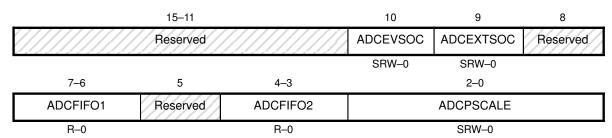
**Note:** R = Read access, W = Write, S = shadowed, -0 = value after reset
