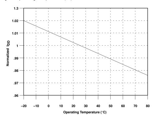
Figure 9–12. Change in Operating Temperature (°C)
