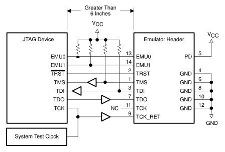
**Note:** When the TMS/TDI lines are buffered, pullup resistors should be used to hold the buffer inputs at a known level when the emulator cable is not connected.
