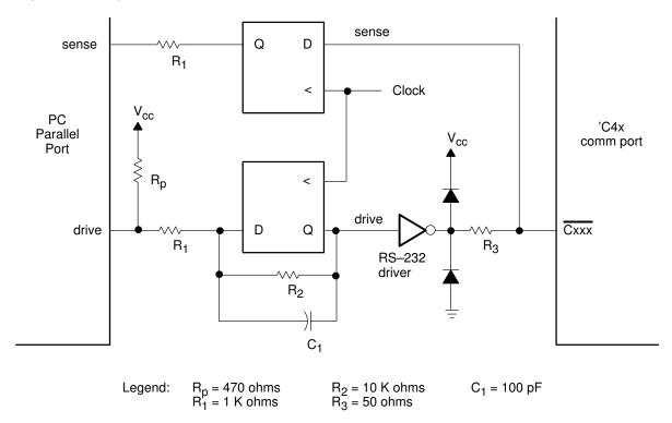
The first improvement is that the signals going to and from the printer port are synchronized using a clock and a simple data latch. By taking samples in time, noise which may be able to corrupt the first sample of a transistion will probably not be enough to corrupt the next sample. By adding a hysteris loop made from resistors R1 and R2, the noise immunity is improved more. Capacitor C1 is an additional analog filter that rejects high-frequency noise.
