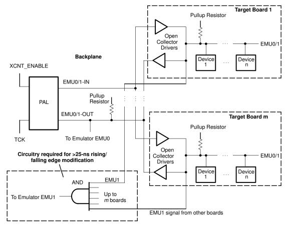
Notes: 1) The low time on EMUx–IN should be at least one TCK cycle and less than 10 μs. Software will set the EMUx–OUT pin to a high state.
