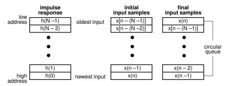
To set up circular addressing, initialize the block-size register BK to block length N. Also, the locations for signal x should start from a memory location whose address is a multiple of the smallest power of 2 that is greater than N. For instance, if N = 24, the first address for x should be a multiple of 32 (the lower 5 bits of the beginning address should be zero). To understand see *Circular Addressing* in the TMS320C4x User's Guide.
