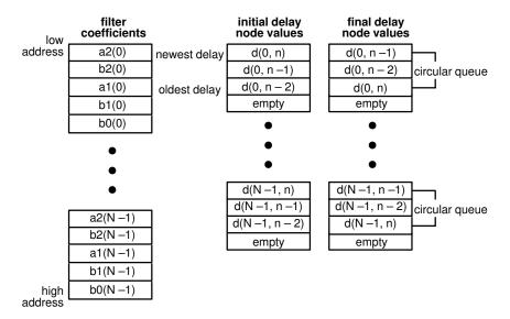
The block size register BK should be initialized to 3, and each set of d values (i.e., d[i,n], i = 0...N-1) should begin at an address that is a multiple of 4 (the last two bits zero), as stated in the case of a single biquad.
