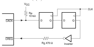
Note that after the port has been reconfigured as an input port, the  $\overline{\text{CREQ}}$  line is active high while the output of the inverter is low. This causes a constant current flow from  $\overline{\text{CREQ}}$  to the inverter.
