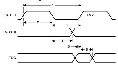
Table 11-2. Emulator Cable Pod Timing Parameters
