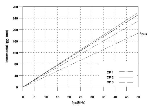
Figure 9-8. Communication Port Current Versus Clock Rate
