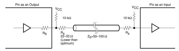
Even though pullup resistors do not help for impedance matching, they are recommended at each end to avoid unintended triggering after reset, when RESET going low is not received on all 'C4x devices at the same time.
