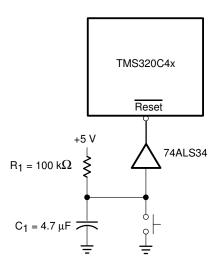
The voltage on the  $\overline{RESET}$  pin is controlled by the  $R_1C_1$  network. After a reset, this voltage rises exponentially according to the time constant  $R_1C_1$ , as shown in Figure 1–2. In Figure 1–1, the 74ALS34 provides a clean  $\overline{RESET}$  signal to the 'C4x.
