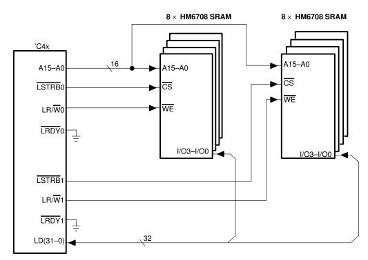
Figure 4-6. 'C4x Interface to Zero-Wait-State SRAMs, Two Strobes
