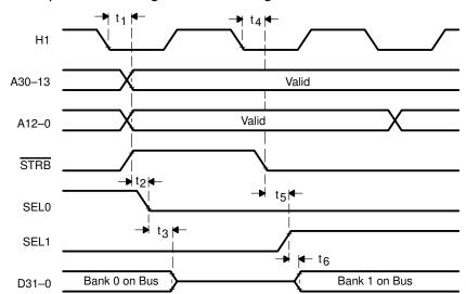
Figure 4-9. Timing for Read Operations Using Bank Switching
