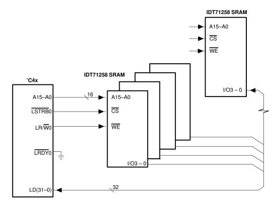
In this circuit implementation, no external logic is necessary to interface the 'C4x to the memory device. Typically, memory devices must be held inactive ( $\overline{\text{CS}}$  inactive) during changes in  $\overline{\text{WE}}$ ; this avoids undesired memory accesses while the address changes. The 'C4x ensures this glueless interface because  $\overline{\text{LSTRB}}$  always frames changes in LR/ $\overline{\text{W}}$ .
