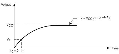
The duration of the low pulse on the  $\overline{RESET}$  pin is approximately  $t_1$ , which is the time it takes for the capacitor  $C_1$  to be charged to 1.5 V. This is approximately the voltage at which the reset input switches from a logic 0 to a logic 1. The capacitor voltage is expressed as
