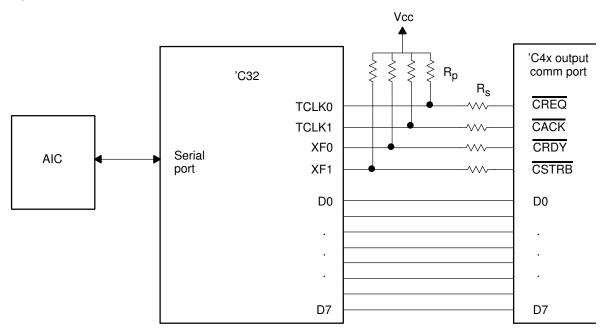
Pullup resistors in the XF0, XF1, TCLK0 and TCLK1 lines are used to prevent undesired glitches due to temporary high-impedance conditions. Serial resistors are also used on the same pins for better impedance matching.
