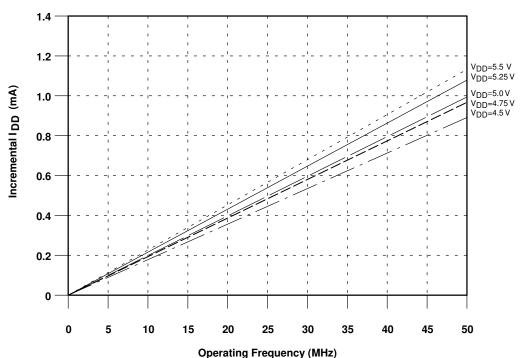
Figure 9–11. Current Versus Frequency and Supply Voltage
