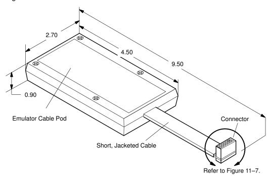
Figure 11-6. Pod/Connector Dimensions
