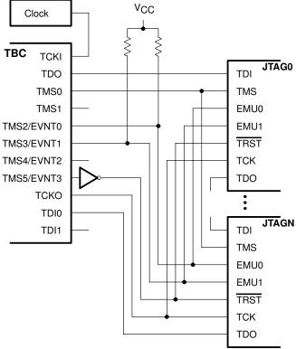
In the system design shown in Figure 1–13, the TBC emulation signals TCKI, TDO, TMS0, TMS2/EVNT0, TMS3/EVNT1, TMS5/EVNT3, TCKO, and TDI0 are used, and TMS1, TMS4/EVNT2, and TDI1 are not connected. The target devices' EMU0 and EMU1 signals are connected to  $V_{\rm CC}$  through pullup resistors and tied to the TBC's TMS2/EVNT0 and TMS3/EVNT1 pins, respectively. The TBC's TCKI pin is connected to a clock generator. The TCK signal for the main JTAG scan path is driven by the TBC's TCKO pin.
