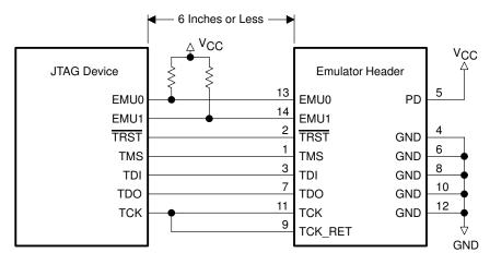
The EMU0 and EMU1 signals must have pullup resistors connected to  $V_{CC}$  to provide a signal rise time of less than 10  $\mu$ s. A 4.7- $k\Omega$  resistor is suggested for most applications.
