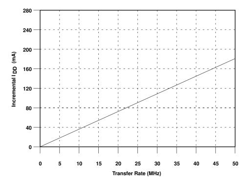
Figure 9-3. Internal Bus Current Versus Transfer Rate
