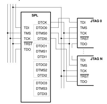
Figure 11-8. Connecting a Secondary JTAG Scan Path to an SPL
