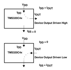
Furthermore, external loads draw supply current ( $I_{DD}$ ) only when outputs are driven high, because when outputs are in the logic zero state, the device is sinking current through  $V_{SS}$ , which is supplied from an external source. Therefore, the power dissipation due to this component will not contribute through  $I_{DD}$  but will contribute to power dissipation with a magnitude of:
