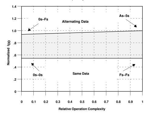
Figure 9-9. Local/Global Bus Current Versus Data Complexity
