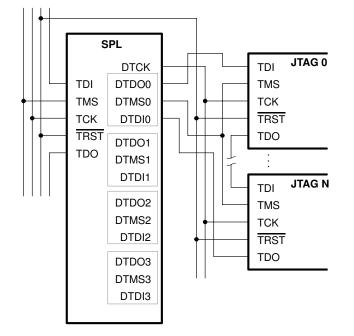
Figure E–10. Connecting a Secondary JTAG Scan Path to a Scan Path Linker
