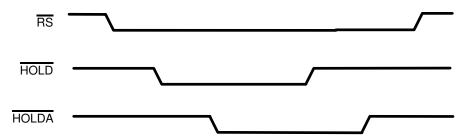
Reset is deasserted before HOLD is deasserted. See Figure 4–15. The CPU will deassert HOLDA regardless of the HOLD signal after the 16 clock cycles required for normal reset operation. Along with the HOLDA signal, the buses will assume normal states. The external system hardware logic should restore the HOLD signal to a high state to avoid conflicts in HOLD logic.
