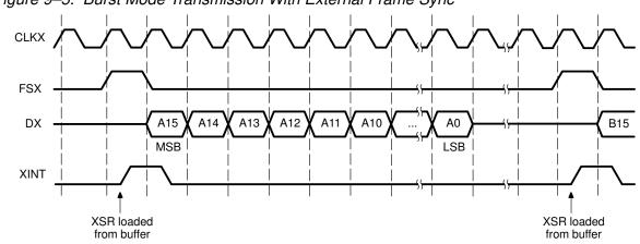
Figure 9–5. Burst Mode Transmission With External Frame Sync
