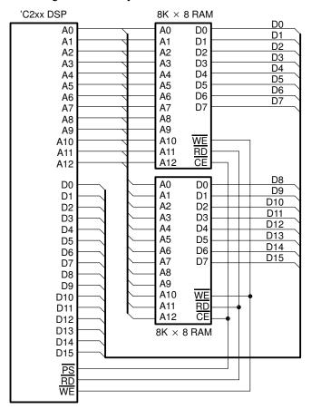
Figure 4–1. Interface With External Program Memory
