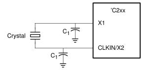
External Oscillator. CLKIN is the output of an external oscillator, which is connected to the CLKIN/X2 pin. The X1 pin must be left unconnected. See Figure 8–2.
