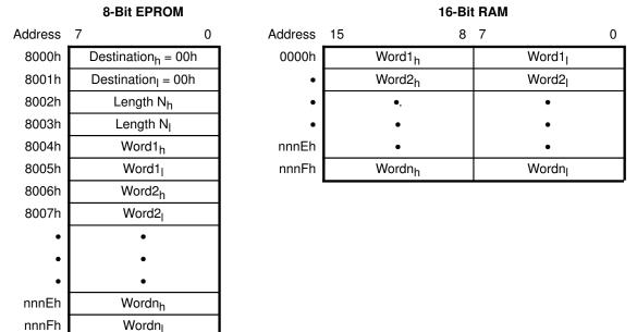
Figure 4–10. Program Code Transferred From 8-Bit EPROM to 16-Bit RAM
