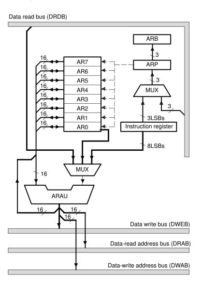
The eight auxiliary registers (AR7–AR0) provide flexible and powerful indirect addressing. Any location in the 64K data memory space can be accessed using a 16-bit address contained in an auxiliary register. For the details of indirect addressing, see Section 6.3 on page 6-9.
