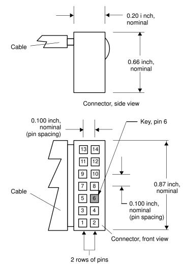
Figure E–9. 14-Pin Connector Dimensions
