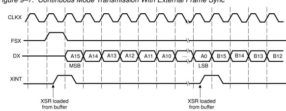
Figure 9–7. Continuous Mode Transmission With External Frame Sync
