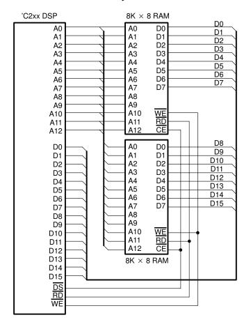
Figure 4–3. Interface With External Local Data Memory
