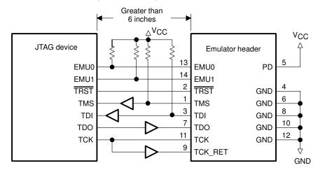
Figure E-5. Emulator Connections With Signal Buffering
