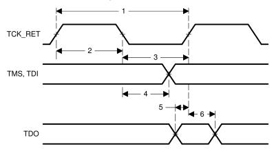
Table E–2. Emulator Cable Pod Timing Parameters
