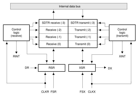
Figure 9–1. Synchronous Serial Port Block Diagram
