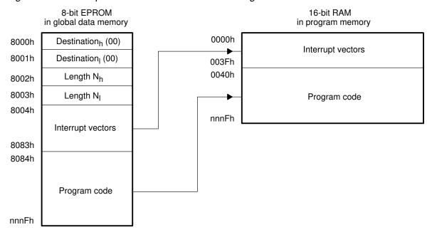
Figure 4–11. Interrupt Vectors Transferred First During Boot Load
