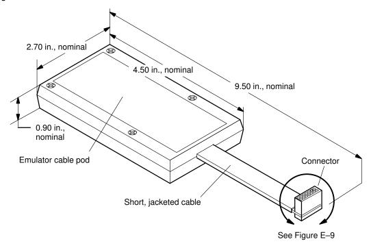
**Note:** All dimensions are in inches and are nominal dimensions, unless otherwise specified. Pin-to-pin spacing on the connector is 0.100 inches in both the X and Y planes.
