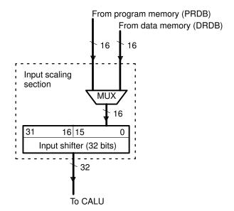
**Input**. Bits 15 through 0 of the input shifter accept a 16-bit input from either of two sources (see Figure 3–2):
