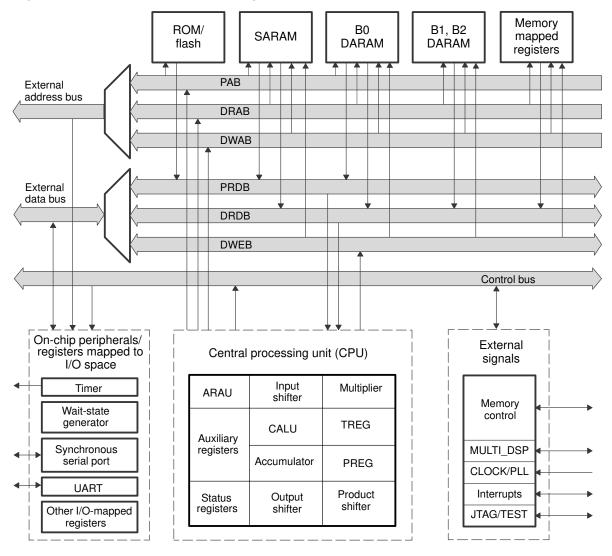
Figure 2–2. Bus Structure Block Diagram
