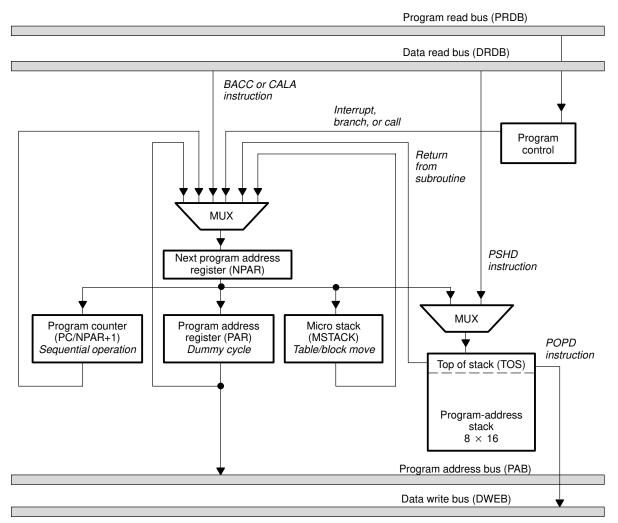
Figure 5–1. Program-Address Generation Block Diagram
