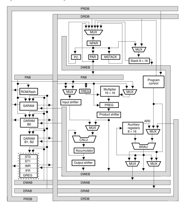
Figure 2–1. Overall Block Diagram of the 'C2xx
