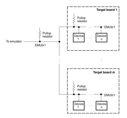
**Note:** The open-collector driver and pullup resistor on EMU1 must be able to provide rise/fall times of less than 25 ns. Rise times of more than 25 ns can cause the emulator to detect false edges during the RUNB command or when the external counter selected from the debugger analysis menu is used. If this condition cannot be met, then the EMU0/1 signals from the individual boards must be ANDed together (as shown in Figure E–14) to produce an EMU0/1 signal for the emulator.
