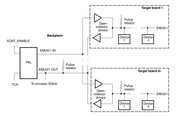
Figure E-11. EMU0/1 Configuration to Meet Timing Requirements of Less Than 25 ns
