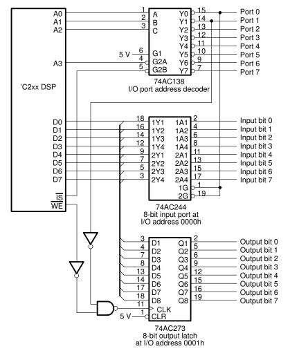
Figure 4–13. I/O Port Interface Circuitry
