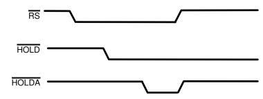
Figure 4–15. Reset Deasserted Before HOLD Deasserted
