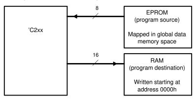
The code for the boot loader is stored on chip. Using the boot loader requires several steps: choosing an EPROM, connecting and programming the EPROM, enabling the boot loader program, and finally, booting.
