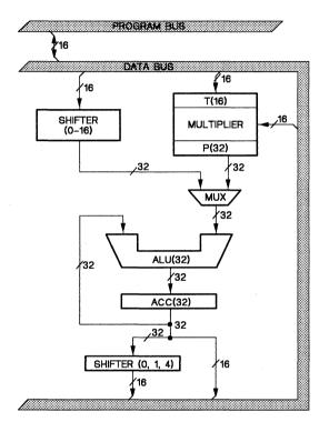
Figure 3-11. Central Arithmetic Logic Unit (CALU)
