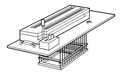
FIGURE 7. EPROM PROGRAMMER ADAPTOR SOCKET
