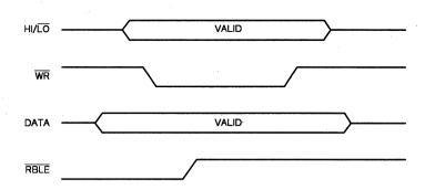
Figure 3-28. External Write Timing to the Coprocessor Port
