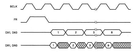
Figure 3-24. Fixed-Data Rate for Internal Framing
