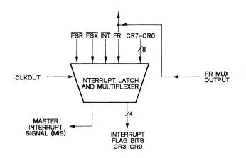
Figure 3-21. Interrupt Latch and Multiplexer
