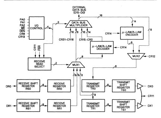
Figure 3-22. Serial Port and Companding Hardware
