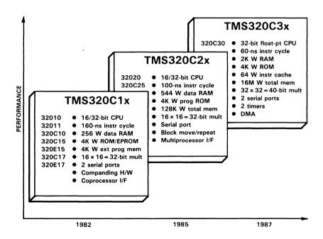
Figure 1-1. TMS320 Device Evolution
