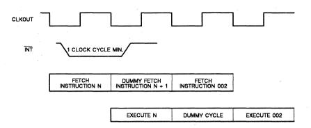
Figure 3-20. Interrupt Timing
