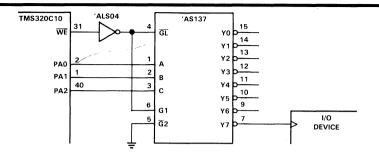
FIGURE 6. I/O DECODE CIRCUIT
