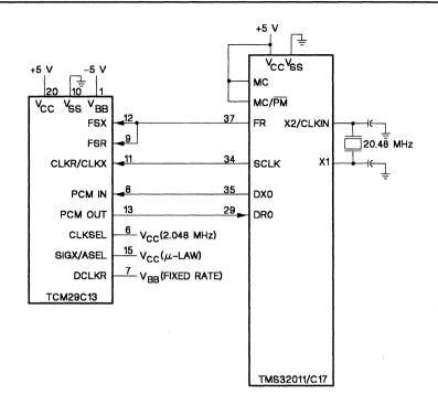
Figure 6-4. Codec Interface for Standalone Serial Operation
