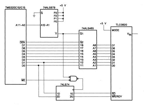
Figure 6-5. A/D Converter to TMS320C10/C15 Interface
