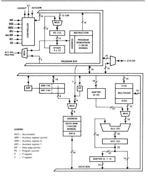
Figure 3-1. TMS32010/C10/C15/E15 Block Diagram
