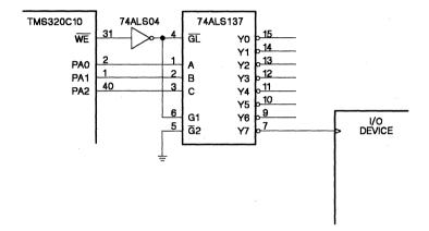
Figure 6-7. I/O Port Interface Circuit
