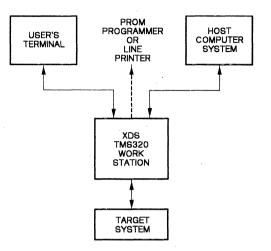
Figure E-3. TMS320C1x XDS/22 System Configuration
