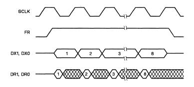
Figure 3-25. Variable-Data Rate for Internal Framing
