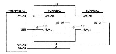
Figure 6-2. EPROM Interface to the TMS32010-14
