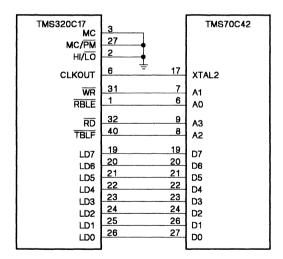
Figure 6-8. TMS320C17 to TMS70C42 Interface
