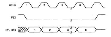
Figure 3-26. Transmit Timing for External Framing
