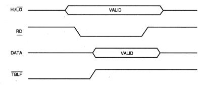
Figure 3-29. External Read Timing from the Coprocessor Port
