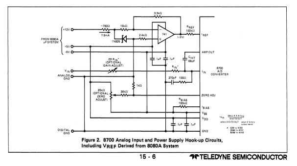
incorporated is a circuit to supply the necessary negative reference, using a temperature-compensated zener diode and an inverting op amp. Note that the  $\pm 5V$  supplies needed for the 8700, as well as the additional +12V used in the reference circuit, are all available from the 8080A system.
