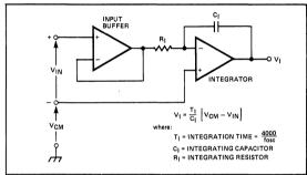
Figure 7: Common-Mode Voltage Reduces Available Integrator Swing. (VCOM ≠ VIN)
