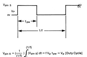
The display may be blanked (all segments OFF) by applying the input code 1111 or by driving the brightness pin with a logic 0. If brightness control is not needed, pin 5 should be tied to 5.0 V.
