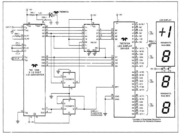
Figure 15: TSC7212A Interface to TSC14433 3 1/2 Digit ADC.
