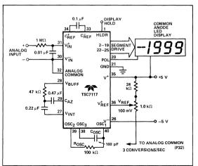
Figure 2: Typical TSC7117 Operating Circuit
