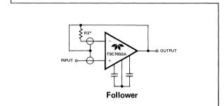
Figure 6: Input Guard Connection
