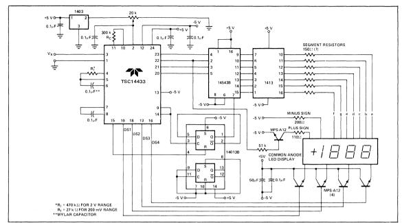
Figure 10: 3 1/2 Digit Voltmeter-Common Anode Displays, Flashing Overrange
