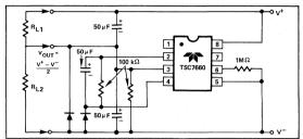
Figure 12: Splitting a Supply in Half.
