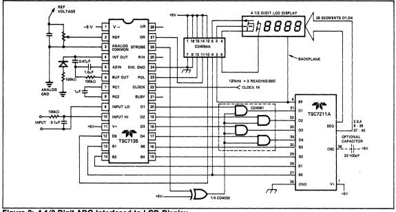
Figure 9: 4 1/2 Digit ADC Interfaced to LCD Display
