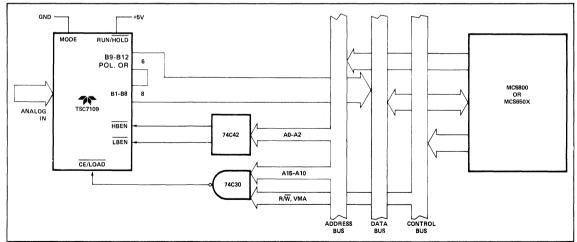
Figure 18: Direct TSC7109 — MC6800 Bus Interface
