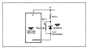
Figure 4: Using an External Reference
