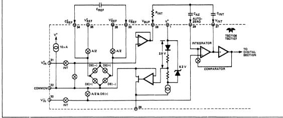
Figure 3: Analog Section of TSC7106/TSC7107
