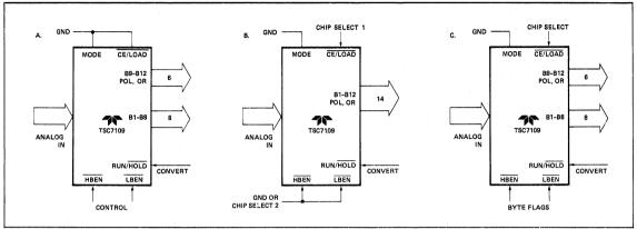
Figure 12: Direct Mode Chip and Byte Enable Combinations
