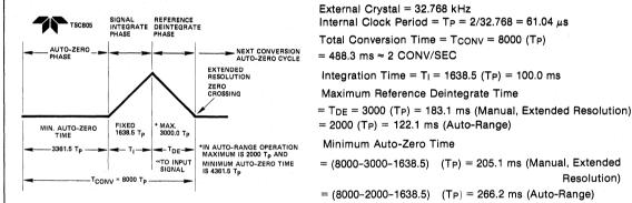
Figure 5: Basic TSC805 Conversion Timing
