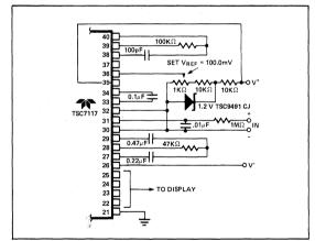
Figure 14: TSC7117 With a 1.2 V External Band-Gap Reference. V<sub>IN</sub> Tied to Common).
