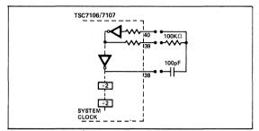
Figure 5: TSC7106/7107 Internal Oscillator/Clock
