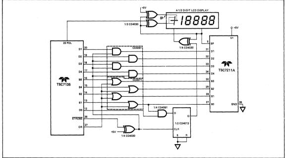
Figure 10: 4 1/2 Digit ADC Interfaced to LCD Display with Digit Blanking on Overrange
