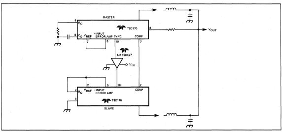
Figure 4: Master/Slave Parallel Operation
