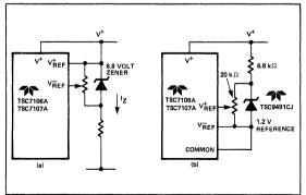
Figure 4: Using an External Reference
