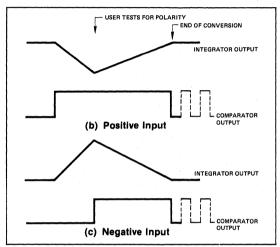
Figure 4b & c: Comparator Output Waveforms
