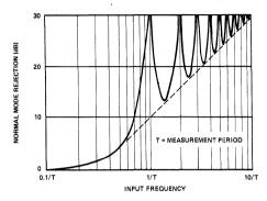
Figure 3: Normal-Mode Rejection of Dual Slope Converter
