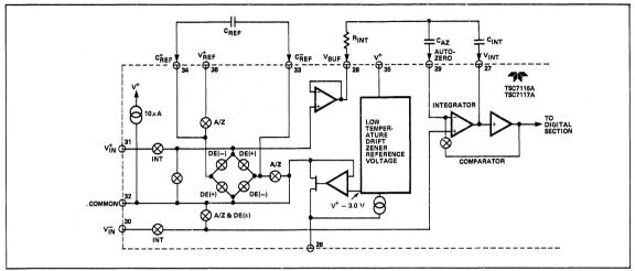
Figure 3: Analog Section of TSC7116A/TSC7117A
