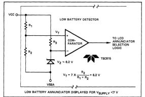
Figure 11: Low Battery Detector
