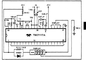
Figure 18: Diode or Resistor Limits Package Power Dissipation
