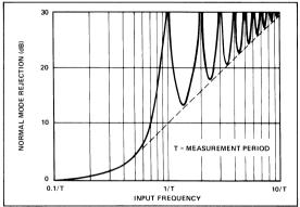
Figure 3B: Normal-Mode Rejection of Dual Slope Converter
