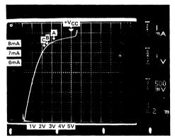
Figure 17: TSC7117 Output Current vs Output Voltage
