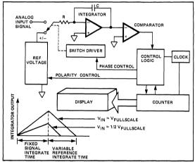
Figure 2: Basic Dual Slope Converter
