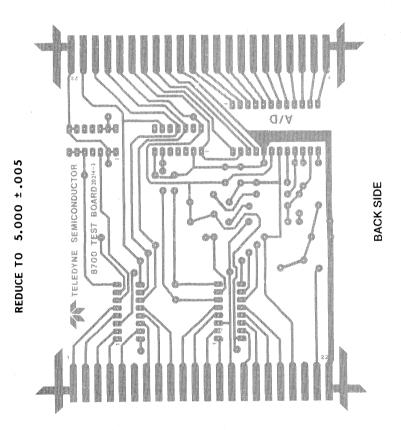
8700 PC BOARD METAL PATTERN PC BOARD FOR 1, 8, 16 CHANNEL DATA ACQUISITION SYSTEM
