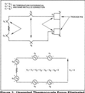
Figure 1: Unwanted Thermocouple Errors Eliminated by Reducing Thermal Gradients and Balancing Junctions.
