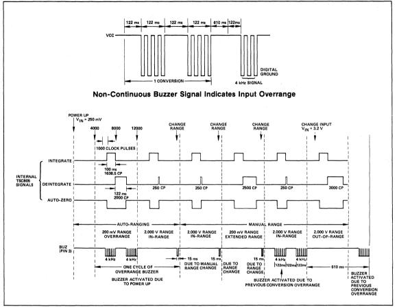
Figure 15: TSC815 Timing Waveform for Buzzer Output
