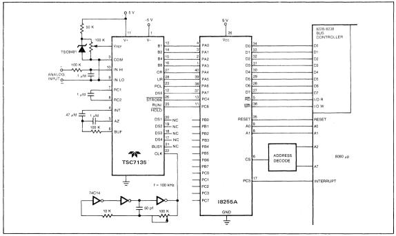
Figure 1: TSC7135 to I/O Port Interface
