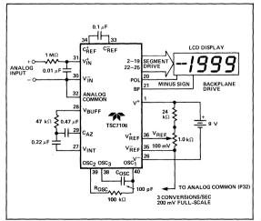
Figure 1: Typical TSC7106 Operating Circuit
