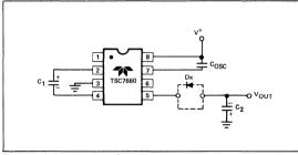
Figure 8: Lowering Oscillator Frequency
