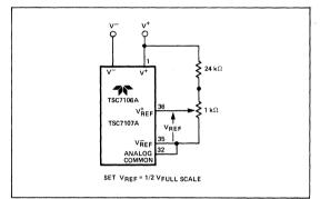
Figure 13: Internal Voltage Reference Connection
