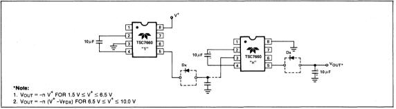
Figure 6: Increased Output Voltage By Cascading Devices
