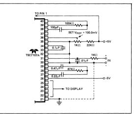
Figure 25: TSC7107A Internal Reference (200 mV Full-Scale, 3 RPS, ViN Tied to GND for Single Ended Inputs).
