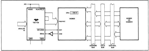
Figure 20: Handshake Interface - TSC7109 to MC6800, MCS650X
