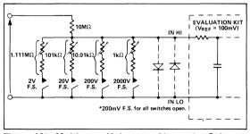
Figure 12b: Multirange Voltmeter, Alternative Scheme
