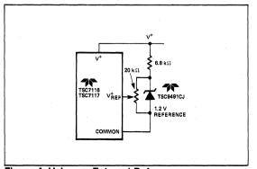
Figure 4: Using an External Reference
