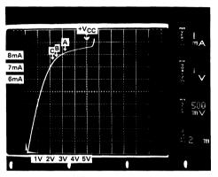
Figure 17: TSC7107 Output Current vs Output Voltage
