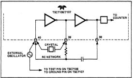
Figure 7: Clock Circuits
