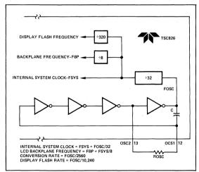
Figure 9: Internal Oscillator Operation
