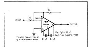
Figure 5: Inverting Amplifier with Optional Clamp
