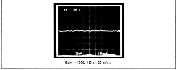
Figure 7: TSC7650A Peak to Peak Noise (0.1 to 10Hz)
