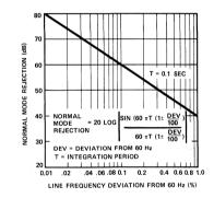
Figure H: Integrating converter normal mode rejection vs. 60 Hz line frequency variations.
