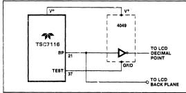
Figure 5: Simple Inverter for Fixed Decimal Point
