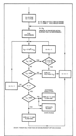
Figure 9: Auto-Range Operation; Voltage Measurement
