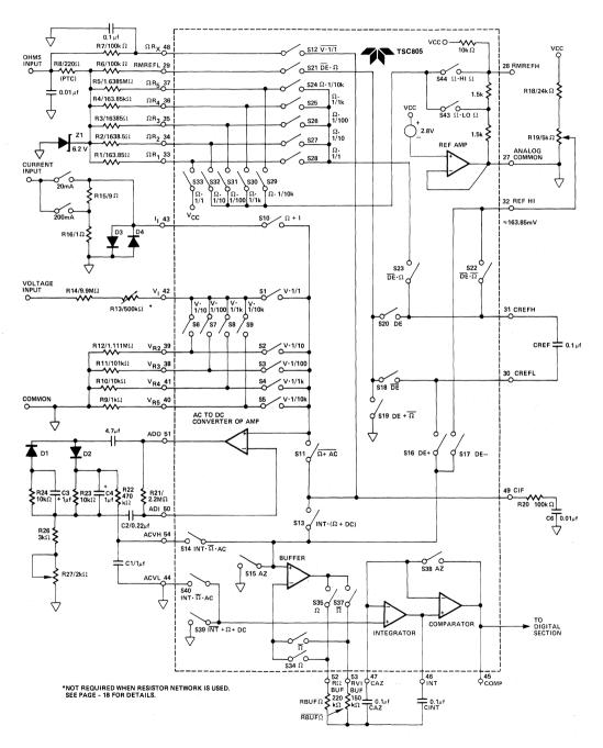
Figure 2: TSC805 Analog Section
