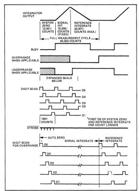
Figure 6: Timing Diagrams for Outputs
