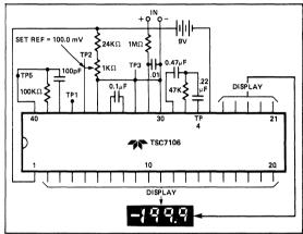
Figure 1: TSC7106 with Liquid Crystal Display
