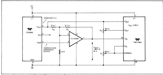
Figure 23: Integrated Circuit Temperature Sensor
