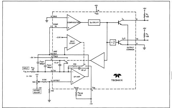
Figure 1: 10 Hz to 10 kHz V/F Converter
