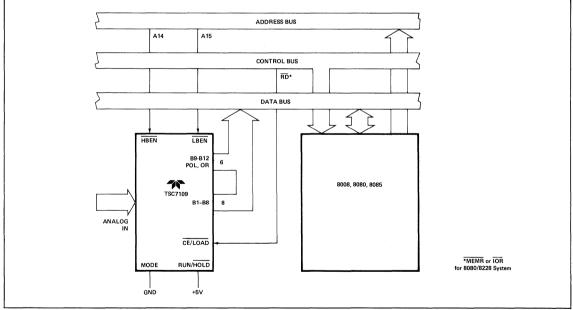
Figure 17: Direct Interface - TSC7109 to 8080/8085
