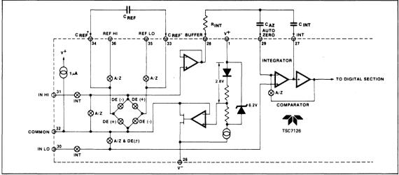
Figure 3: Analog Section of TSC7126.
