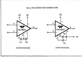
Figure 2: Nulling Capacitor Connection
