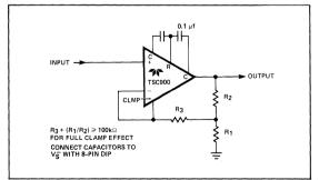
Figure 4: Non-Inverting Amplifier with Optional Clamp
