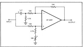
Figure 10: F/V Ripple Eliminator
