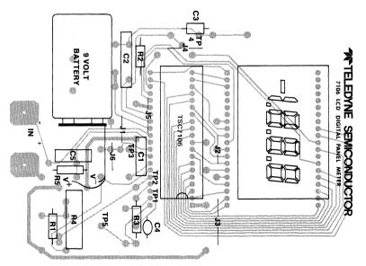
ACTUAL SIZE NOT SHOWN Figure 17: TSC7106 - Circuit Board Layout and Component Placement
