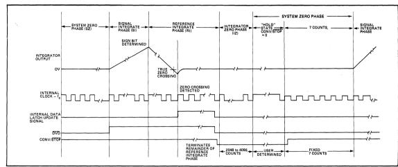
Figure 6: Convert on Command Operation. (CONV/STOP = 0 After Zero Crossing Detected)
