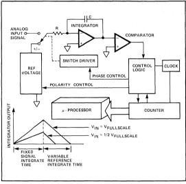
The dual slope converter accuracy is unrelated to the integrating resistor and capacitor values as long as they are stable during a measurement cycle. An inherent benefit is noise immunity. Noise spikes are integrated or averaged to zero during the integration periods. Integrating ADCs are immune to the large conversion errors that plague successive approximation converters in high noise environments.
