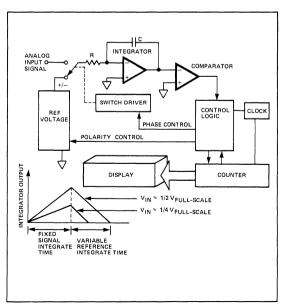
Figure 2: Basic Dual Slope Converter
