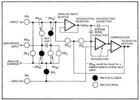
Figure 3C: TSC800 Reference Voltage Integration Cycle
