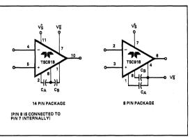
Figure 2: Nulling Capacitor Connection
