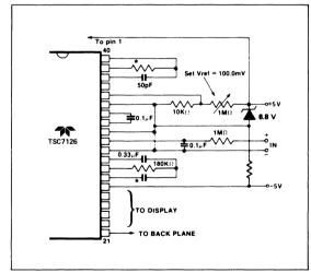
Figure 11: TSC7126 with Zener Diode Reference.
