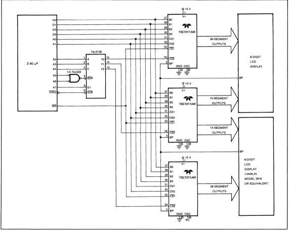
Figure 6. Multiple TSC7211AM Interface to Z-80  $\mu$ P
