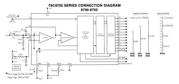
The Teledyne Semiconductor 8700 series are integrating A/D converters. These are available with 8-, 10-, or 12-bit resolutions, with or without three-state outputs, and
