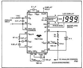
Figure 1: Typical TSC7116A Operating Circuit
