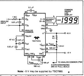
Figure 2: Typical TSC7107A Operating Circuit
