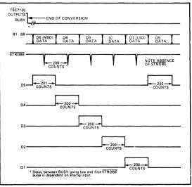
Figure 7: Strobe Signal Pulses Low 5 Times Per Conversion.
