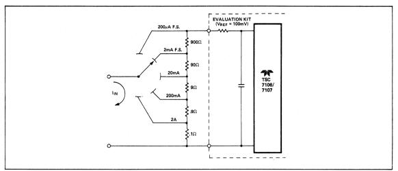
Figure 15: Multirange Current Meter
