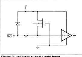
Figure 2: TSC7135 Digital Logic Input
