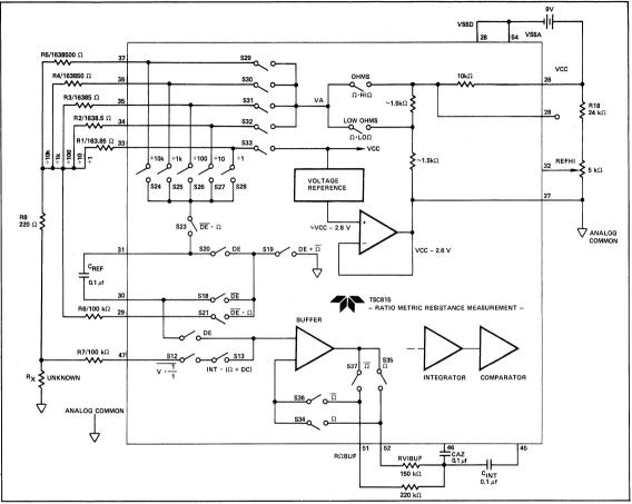
Figure 3: Ratiometric Resistance Measurement Functional Diagram
