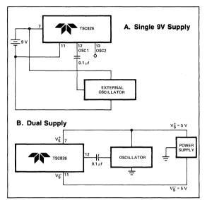
Figure 10: External Oscillator Connection
