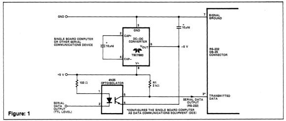
This low cost circuit converts TTL-level signals to an RS-232 level without the expense of a negative power supply. The TSC7660's -5 V output permits the optoisolator to swing to RS-232 levels at up to 9600 baud.
