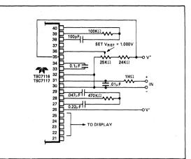
Figure 15: TSC7116/TSC7117: Recommended Component Values for 2.00 V Full-Scale.
