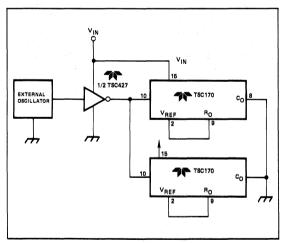
Figure 5: External Clock Synchronization
