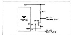
Figure 3: Simple Inverter for Fixed Decimal Point
