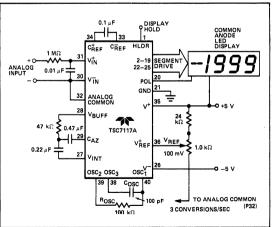
Figure 2: Typical TSC7117A Operating Circuit
