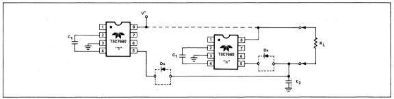
Figure 5: Paralleling Devices Lowers Output Impedance
