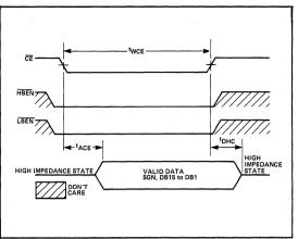
Figure 1B: Parallel Data Transfer – 16-Bit Bytes
