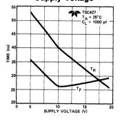
**Delay Time vs Supply Voltage**
