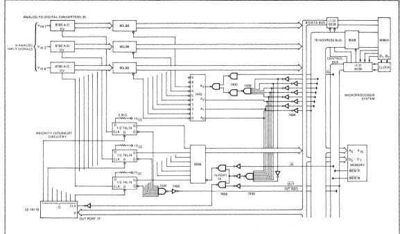
Figure 4. Eight Port A/D Converter System with Maskable Priority Interrupt
