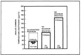
Figure 8: Analog Common Temperature Coefficient
