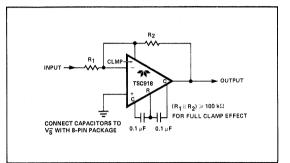
Figure 5: Inverting Amplifier with Optional Clamp
