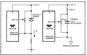
Figure 4: Using an External Reference
