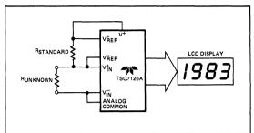
Figure 10: Low Parts Count Ratiometric Resistance Measurement
