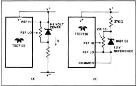
Figure 4: Using an External Reference
