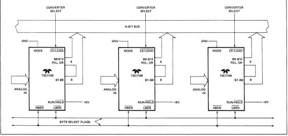
Figure 13: Three-Stating Several TSC7109's to a Small Bus
