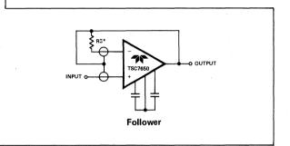
Figure 6: Input Guard Connection
