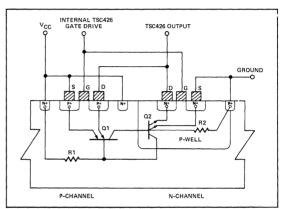
Figure 2: Output Stage IC Layout.
