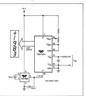
Figure 15: Negative Power Supply Generation with TSC7660.
