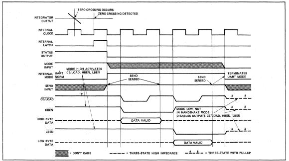
Figure 7: TSC7109 Handshake with Send Input Held Positive
