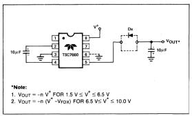
Figure 4: Simple Negative Converter
