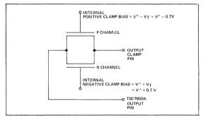
Figure 3: Internal Clamp Circuit
