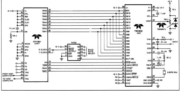
Figure 13: Serial data transmission is easy when the ADC logic includes UART handshaking signals. The TSC300 monitors its DATA REQUEST pin until the UART is ready to receive data.
