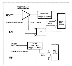
Figure 5: 15-Bit Dynamic Range Converter Eliminates Programmable Gain Amplifier.
