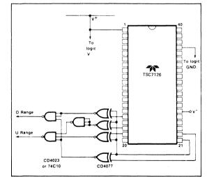
Figure 17: Circuit for Developing Underrange and Overrange Signals from TSC7126 Outputs.
