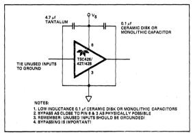
Figure 6: Suggested Bypass Procedure.
