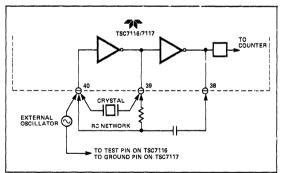
Figure 7: Clock Circuits
