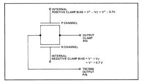
Figure 3: Internal Clamp Circuit
