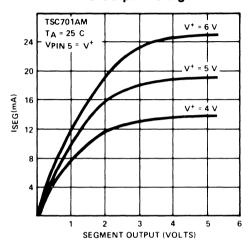
LED Segment Current vs Brightness Control Voltage
