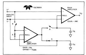
Figure 1: TSC7650A Contains a Nulling and Main Amplifier. Offset Correction Voltages are Stored on Two External Capacitors.
