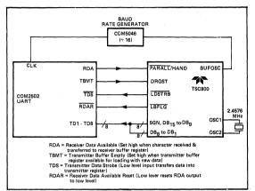
Figure 3B: Typical UART to TSC800 Connection
