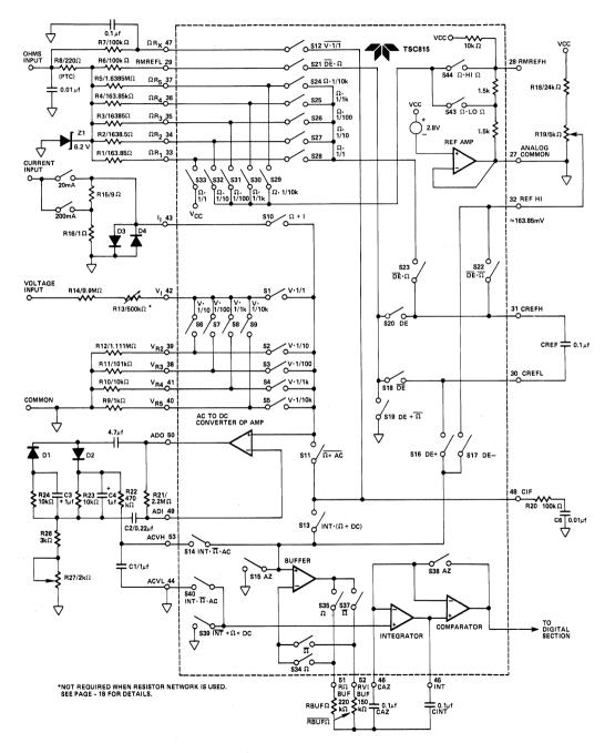
Figure 2: TSC815 Analog Section
