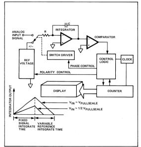
Figure 3A: Basic Dual Slope Converter
