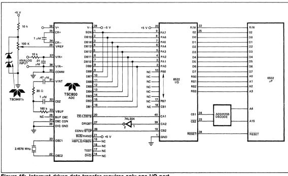
Figure 16: Interrupt-driven data transfer requires only one I/O port.
