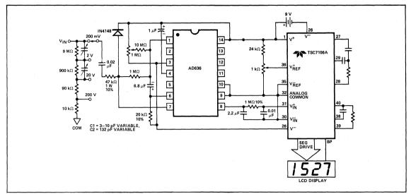
Figure 20: 3 1/2 Digit True RMS AC DMM
