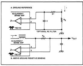
Figure 2: Resistive Sensing
