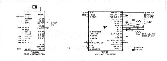
Figure 1B: TSC7109 Parallel Interface with 8048/8049 Microcomputer
