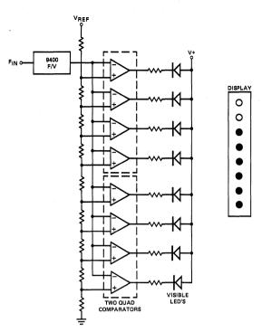
A tachometer can be constructed by using the 9400 in the F/V mode to convert the frequency information (RPM) into a linearly proportional voltage. This voltage is then compared to one of n comparators (8 in this example). When the voltage
