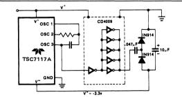
Figure 10: Generating Negative Supply From + 5V
