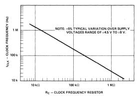
Figure 5: Typical Clock Frequency vs. Resistor (R<sub>C</sub>).
