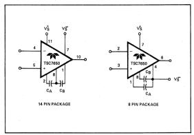
Figure 2: Nulling Capacitor Connection
