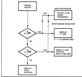
Figure 7: Manual Range Selection; Current Measurement
