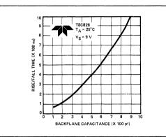
Figure 12: Backplane Driver Rise/Fall Time vs Capacitance
