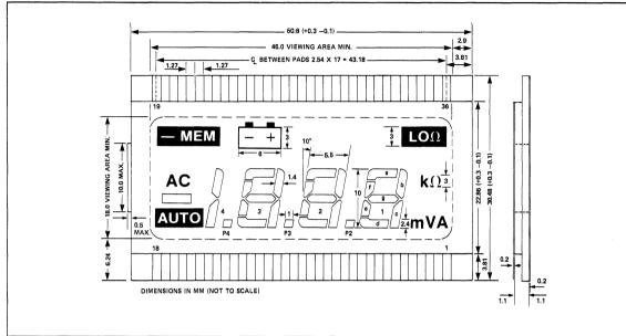
Figure 14: Typical LCD Display Configuration TSC805 Triplex
