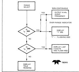
Figure 7: Manual Range Selection; Current Measurement
