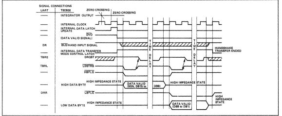
Figure 12: UART interface uses data request signal to control handshake data transfer.
