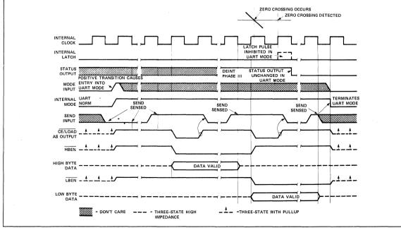
Figure 9: TSC7109 Handshake Triggered by Mode Input
