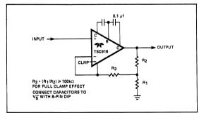
Figure 4: Non-Inverting Amplifier with Optional Clamp
