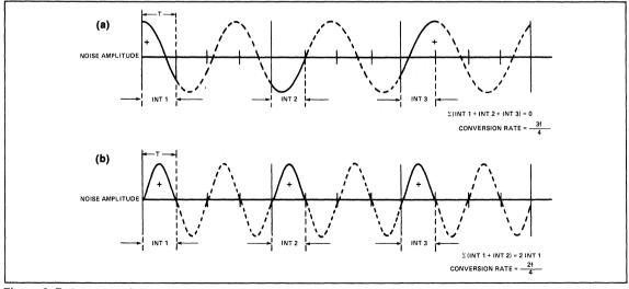
**Figure 3: Data-conversion systems employing a numerical-integration technique** furnish noise rejection when an odd number of samples are summed (a). Adding the results of two conversions, though, can yield twice as much error as does one conversion (b) if the A/D converter and noise frequency are synchronized.
