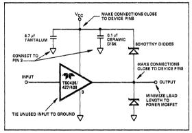
Figure 4: Diode Output Clamp Prevents SCR Action.
