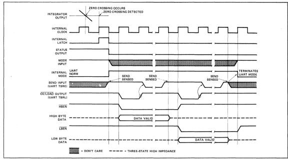
Figure 8: TSC7109 Handshake — Typical UART Interface Timing
