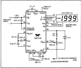
Figure 1: Typical TSC7116 Operating Circuit
