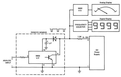
By converting an analog voltage to a linearly proportional pulse train of short duration, it is possible to transmit this data on the same wires that are used to energize the V/F converter.
