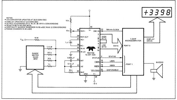
Figure 5: This 3 3/4-digit multimeter uses a numerical-integration technique to reject both 50-and 60-Hz normalmode noise. Although the DMM's display updates at 2.5 samples/sec, conversions take place at 22.5 samples/sec.
