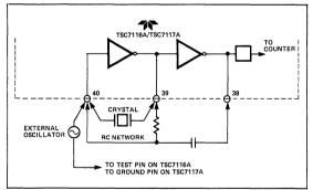
Figure 7: Clock Circuits
