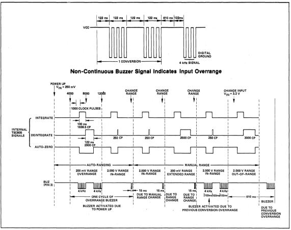
Figure 15: TSC805 Timing Waveform for Buzzer Output
