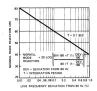
Figure 4: Normal Mode Rejection vs. Input Frequency
