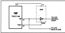
Figure 5: Simple Inverter for Fixed Decimal Point
