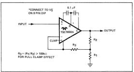
Figure 4: Non-Inverting Amplifier with Optional Clamp
