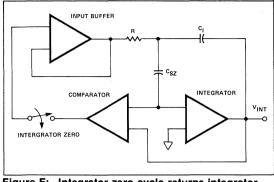
Figure E: Integrator zero cycle returns integrator output to zero volts before system zero cycle is entered.
