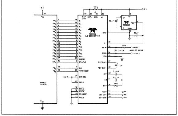
**Figure 6:** You can evaluate numberical integration with the circuit detailed in this schematic. The 6522 peripheralinterface adapter provides clocking and the  $\mu P$  interface for the dual-slope A/D converter.
