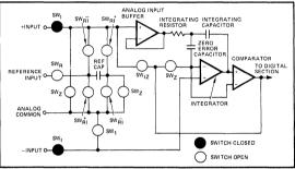
Figure 3C: TSC7135 Input Signal Integration Phase
