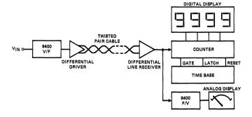
When transmitting analog data over long distances it is advantageous to convert the analog signal into a digital signal which will be less susceptible to noise pick-up. either a pulse or square wave which is transmitted on a pair or wires by use of a line driver and receiver. At the other end the original voltage ( $V_{IN}$ ) can be digitally displayed on a frequency counter or converted back to an analog voltage by use of a 9400 F/V converter.
