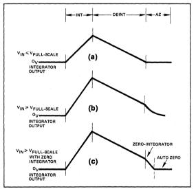
Figure 5: TSC500 Integrator Output Waveforms During:
