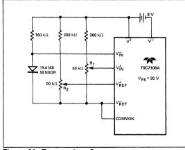
Figure 21: Temperature Sensor
