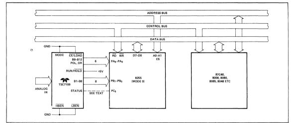
Figure 14: Full-Time Parallel Interface to MCS-48, -80, -85 Microcomputer Systems
