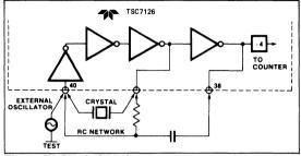
Figure 7: Clock Circuits
