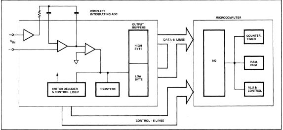
Figure 1: Typical ADC Interface to µC
