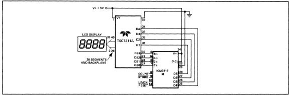
Figure 7: LCD Display Interface to 4 Digit Counter
