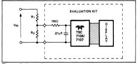
Figure 9: Input Attenuator for  $V_{IN} \ge 2.0 V$
