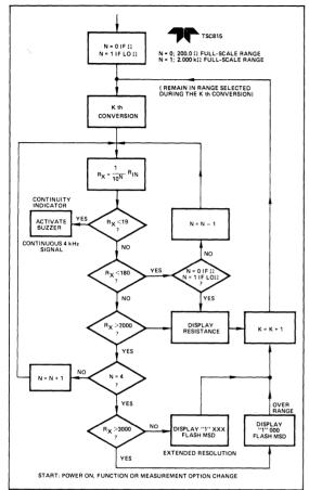
Figure 10: Auto-Range Operation; Resistance Measurement
