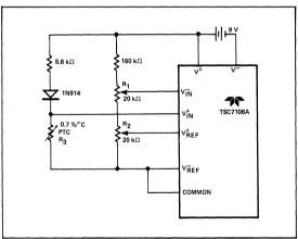
Figure 22: Positive Temperature Coefficient Resistor Temperature Sensor
