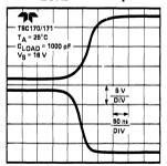
**Output Rise and Fall Time:** CLOAD = 1800 pF 78 TSC170/171 T<sub>A</sub> ≈ 25°C C<sub>LOAD</sub> = 1800 p V<sub>S</sub> = 16V ----50 ns DIV **Oscillator Frequency** (Figure 7) vs Oscillator Resistance 60 TSC170/171 T<sub>A</sub> = 25°C 10 48 4 OSCILLATOR RESISTOR (M2) 35 30 28 20 260 p.F
