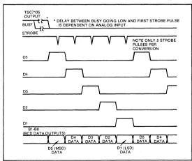
Figure 2: Timing Relationships Between TSC7135 Outputs
