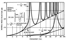
Figure G: Normal Mode Rejection Vs. Input Frequency.
