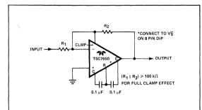
Figure 5: Inverting Amplifier with Optional Clamp
