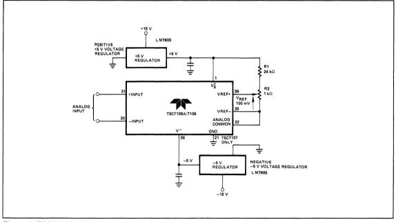
Figure 1: TSC7106A/7106 Operates From ±5 V Power Supplies
