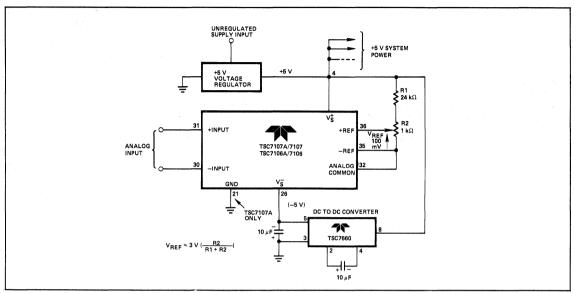
Figure 2: TSC7660 Generates -5 V Power Supply
