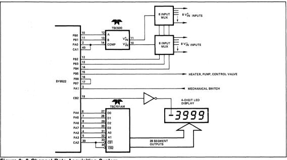
Figure 8: 8-Channel Data Acquisition System
