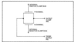
Figure 3: Internal Clamp Circuit
