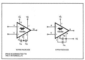
Figure 2: Nulling Capacitor Connection
