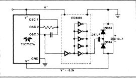
Figure 14: Generating Negative Supply From +5 V
