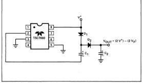
Figure 9: Positive Voltage Multiplier
