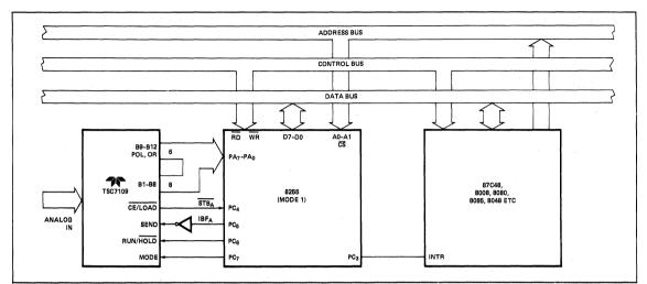
Figure 19: Handshake Interface — TSC7109 to MCS-48, -80, -85
