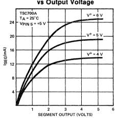
LED Segment Current vs Output Voltage
