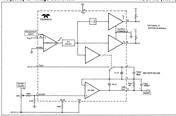
Figure 7: DC — 10 kHz F/V Converter
