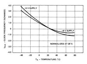
Figure 6: Typical % Change of Clock Frequency vs. Temperature.
