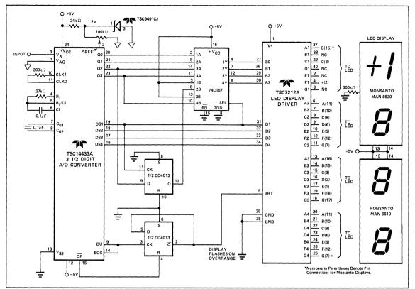
Figure 13: TSC7212A Interface to TSC14433 A 3 1/2 Digit ADC.
