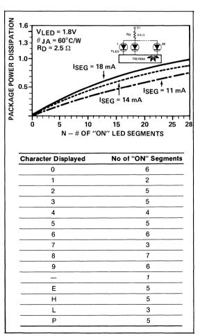
Figure 1: Package Power Dissipation
