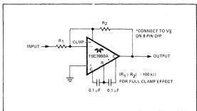
Figure 5: Inverting Amplifier with Optional Clamp
