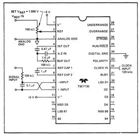
Figure 1: TSC7135 Test Circuit
