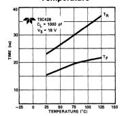
**Delay Time vs Temperature**
