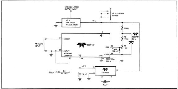
Figure 3: External Reference in ±5 V System
