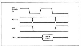
Figure 2. 6502 µP Output Timing Diagram
