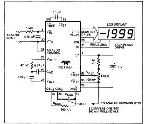
Figure 1: Typical TSC7106A Operating Circuit
