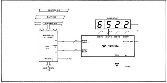
Figure 11: LCD Display Interface to SY6522 VIA
