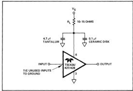
Figure 8: R<sub>L</sub> Current Limiting Protects Device and Will Not Degrade Switching Speed.
