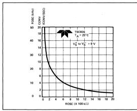
Figure 8: Oscillator Frequency vs. ROSC
