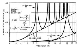
Figure 5: Integrating Converter Normal Mode Rejection vs. 60 Hz Line Frequency Variations.
