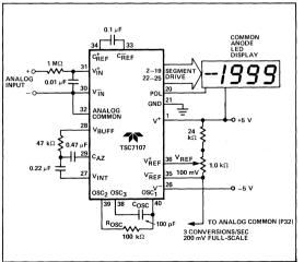
Figure 2: Typical TSC7107 Operating Circuit
