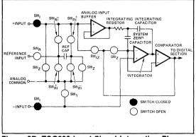
Figure 3B: TSC800 Input Signal Integration Phase
