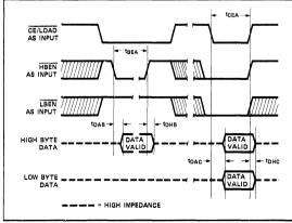
Figure 6: TSC7109 Direct Mode Output Timing
