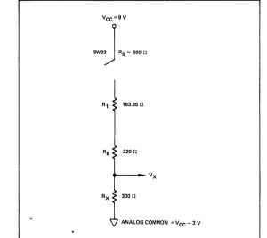
Figure 16: R $\Omega$ BUF Calculation (200  $\Omega$  Manual Operation)
