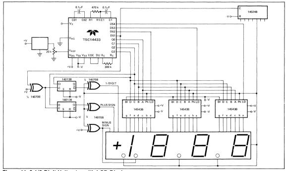
Figure 11: 3 1/2 Digit Voltmeter with LCD Display.
