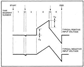
Figure 7: Integrator Waveforms at Pin 6.
