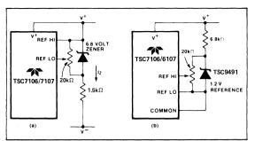
Figure 7: Using an External Reference
