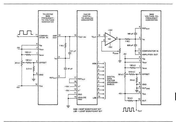
Circuit uses frequency-to-voltage-to-frequency conversion, with intermediate stage of gain between conversions, for multiplying input frequency by any number. Digital-to-analog converter is programmed digitally, by thumbwheel switches or microprocessor, for coarse selection of frequency-multiplying factor; 741 provides fine gain, enables choice of non-integer multiplication values.
