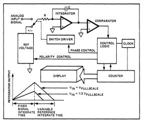
Figure 3: Basic Dual Slope Converter
