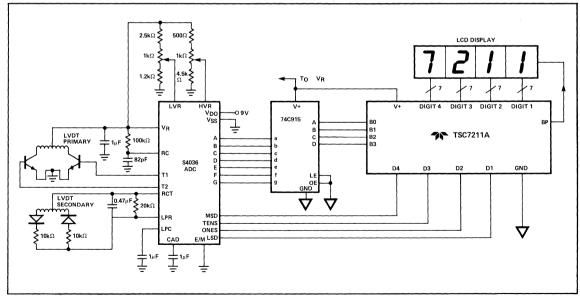
Figure 12: Digital Scale with LCD Readout
