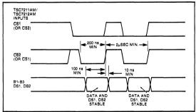
Figure 1. TSC7211AM/TSC7212AM Input Timing Diagram
