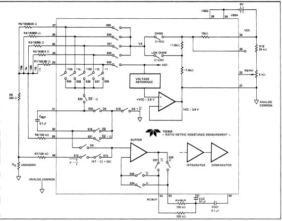
Figure 3: Ratiometric Resistance Measurement Functional Diagram
