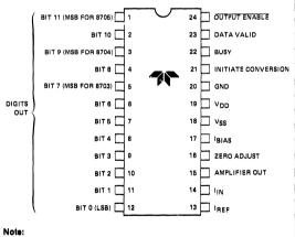
Do not make connections to pin 1, 2, 3 or 4 on 8703; pin 1 or 2 on 8704. These pins are internally connected.
