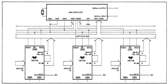
Figure 21: Handshake Interface for Multiplexed Converters
