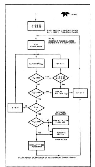
Figure 9: Auto-Range Operation; Voltage Measurement
