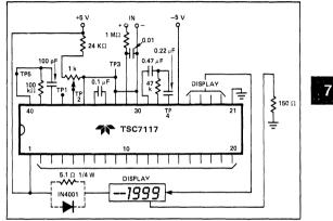
Figure 18: Diode or Resistor Limits Package Power Dissipation
