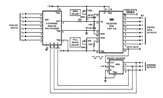
A low-cost data acquisition system with 8 inputs and 8 bits (0.4%) of resolution at the ouput can be built by using the TELEDYNE 8700 CMOS A/D converter and adding the 4051 8 channel CMOS multiplexer and the 4024 binary counter.
