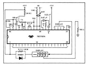
Figure 17: Diode or Resistor Limits Package Power Dissipation.
