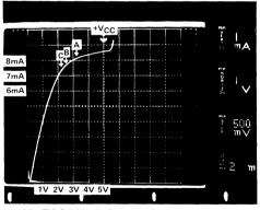
Figure 16: TSC7107A Output Current vs Output Voltage
