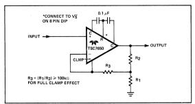
Figure 4: Non-Inverting Amplifier with Optional Clamp
