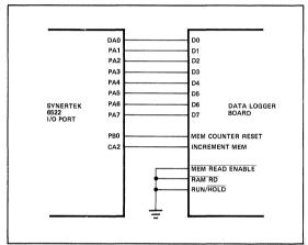
Figure 2: Connecting 13-Bit Remote Data Logger to 6522 i/O Port for Data Readout.
