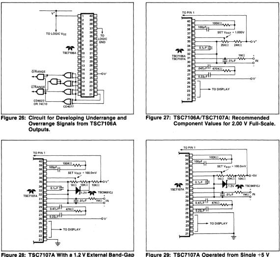
gure 28: TSC/10/A With a 1.2 V External Band-C Reference. Vin Tied to Common).
