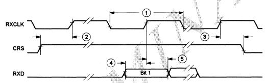
Figure 23 10BASE-T Receive Function Timing
