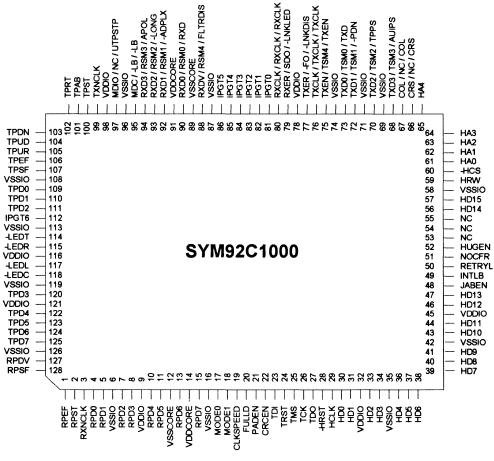
**Figure 1 Pinout Diagram**
