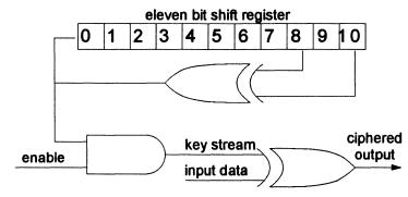
Figure 8 Ciphering Circuit
