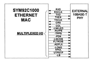
Figure 4 Three Options for Multiplexed I/O
