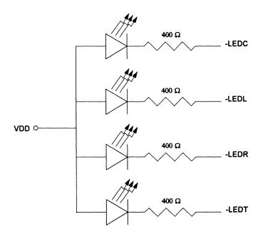
**Figure 5 Typical LED Circuit**
