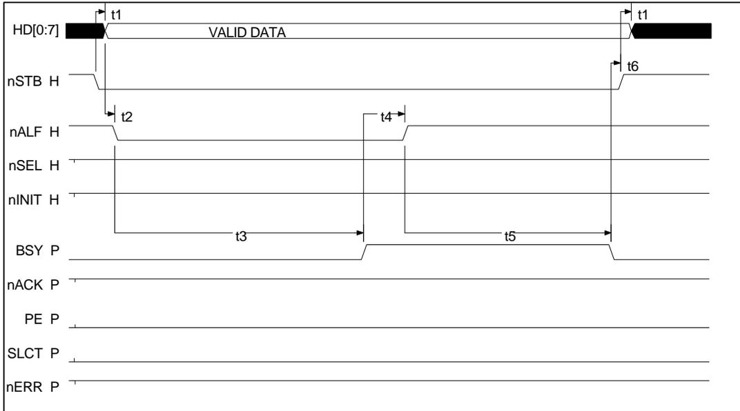
**FIGURE 16 - EPP DATA WRITE TIMING (PARALLEL PORT SIGNALS)**
