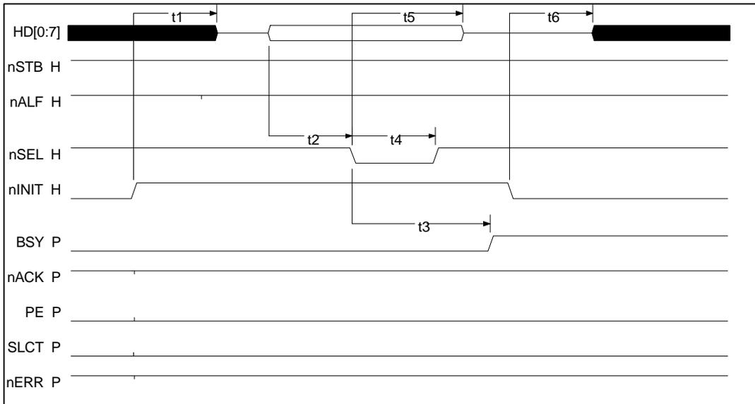
**FIGURE 11 - SPP ADDRESS WRITE TIMING (PARALLEL PORT SIGNALS)**
