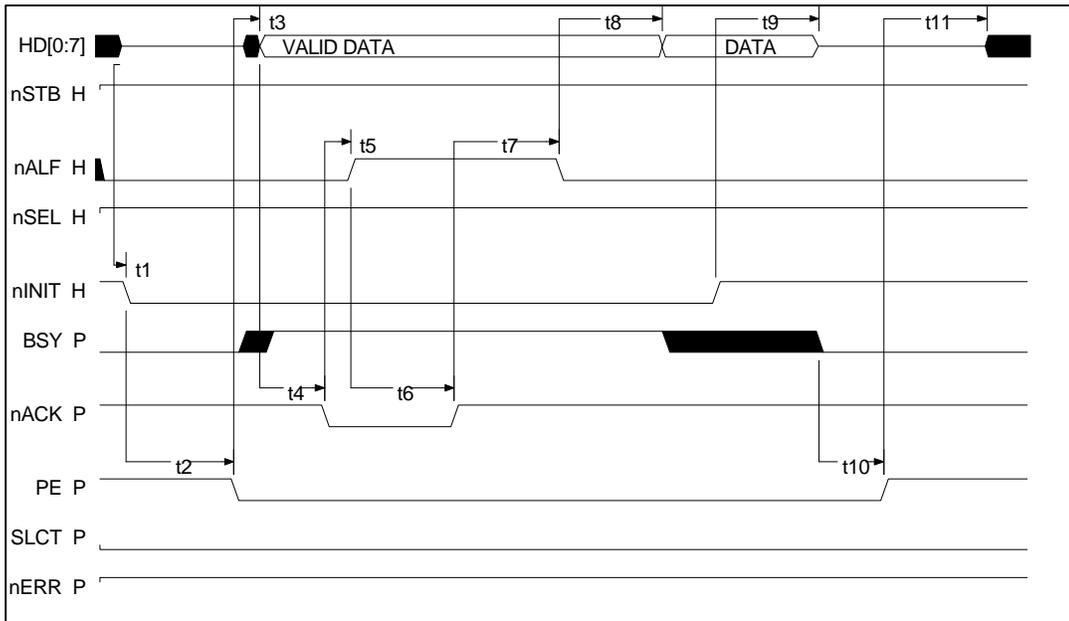
**FIGURE 20 - ECP REVERSE DATA TRANSFER TIMING
