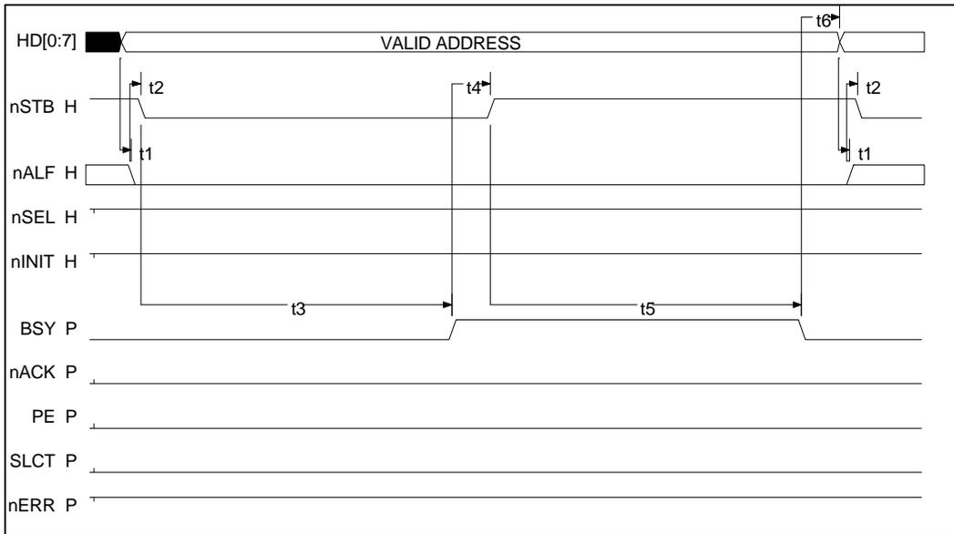
**FIGURE 18 - ECP FORWARD COMMAND TRANSFER TIMING
