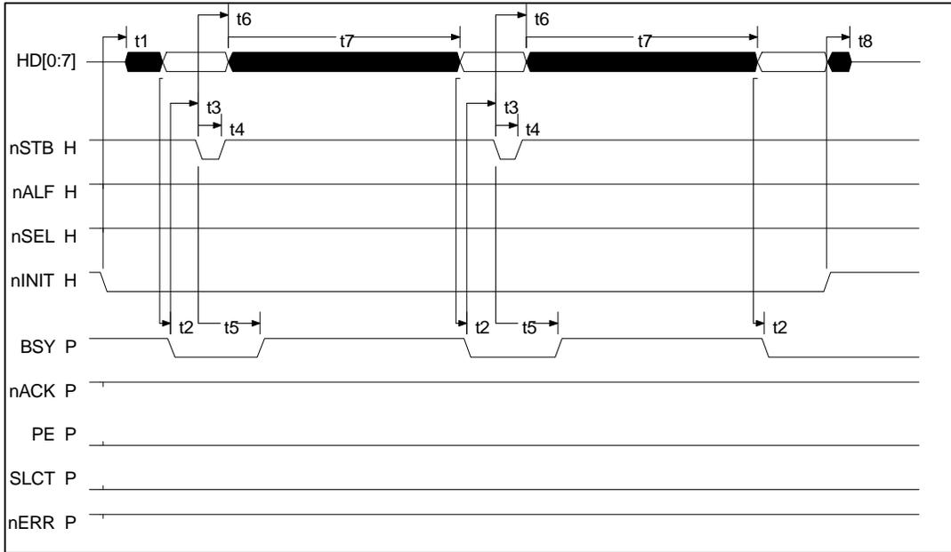
**FIGURE 13 - SPP DATA READ TIMING (PARALLEL PORT SIGNALS)**
