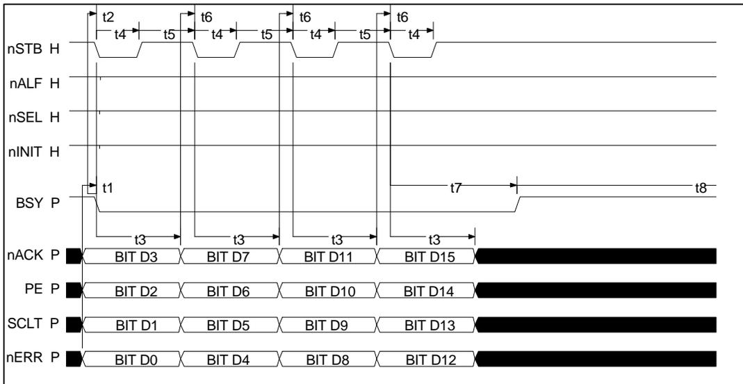
**FIGURE 14 - SPP NIBBLE READ (PARALLEL PORT SIGNALS)**
