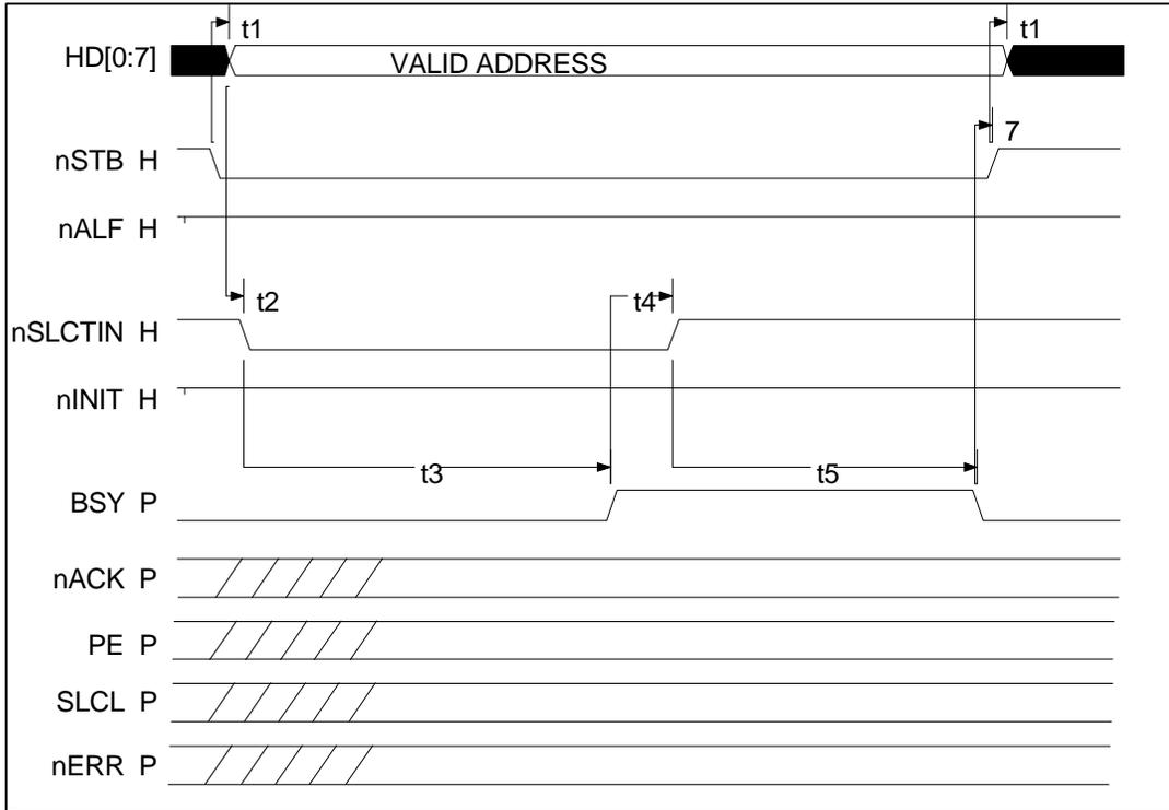
**FIGURE 15 - EPP ADDRESS WRITE (PARALLEL PORT SIGNALS)**
