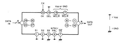
Fig. 1. Circuit of 908 bits delay
