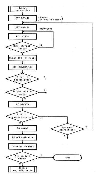
Fig. 3.7 CPU control of the IC during repeated correction
