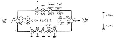
Fig. 1 Circuit of 908 bits delay
