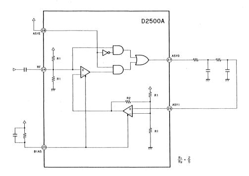
Figure 3-15 Asymmetry correction application circuit example
