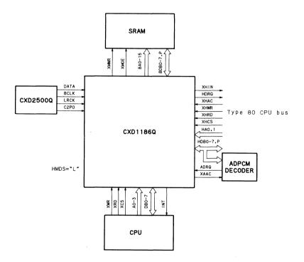
Fig. 4.2 CXD1186Q connection (Type80 CPU bus)
