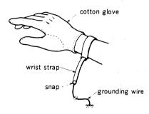
When using a copper wire for grounding, connect a  $1M\Omega$  resistance in series near the hand for safety.
