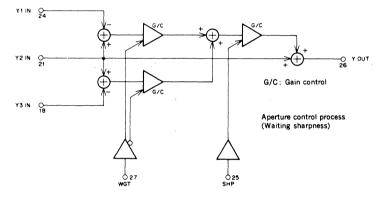
Aperture control process controls preshoot/overshoot ratio through WGT pin (Pin 27) and sharpness level through SHP pin (Pin 25) respectively. This control process is indicated on the above diagram. The basic principle of delay line aperture control is shown on the below diagram.
