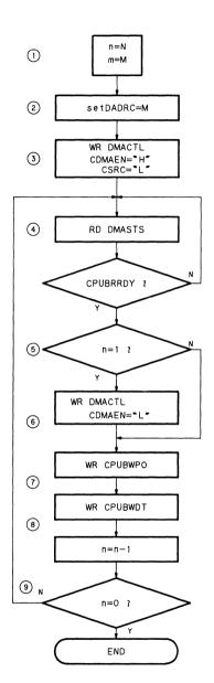
Fig. 5.2 CPU buffer read control
