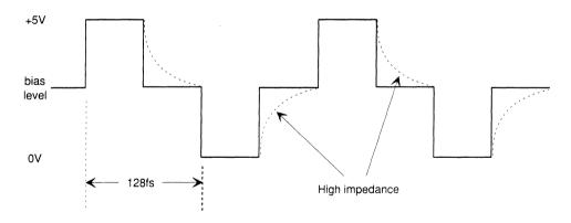
Filtering is necessary to eliminate 128fs component. Attenuation level for stop band frequency component is -45dB level. If it is necessary to increase this level, additional LPF is recommended to be used.
