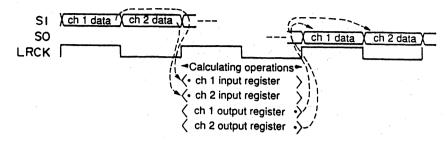
First, during 1LRCK period, ch1/ch2 serial data that is input from SI is latched at ch1/ch2 input register with the rising edge of the following LRCK. Also,during 1LRCK, if the results of the calculating operations are enclosed into ch1/ch2 output registers, those are latched by the shift register at the following rising edge of LRCK to be respectively output as serial data from SO.
