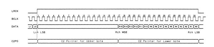
Fig. 2.1.1 (4) CXD2500Q, 64 bit slot mode, timing chart
