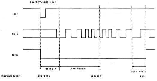
Figure 3-10 (b) Timing chart for 10-track jump
