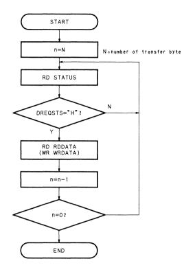
Fig. 4.2.2 I/O mode data transfer
