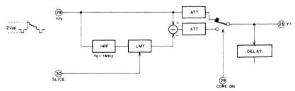
As shown in the above diagram, Y signal is passed through HPF, amplitude limitation is performed and the result substracted from the original signal to execute Y signal coring.
