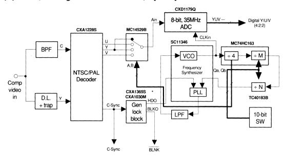
(A). NTSC/PAL Digital Decoder with D1/Square pixel mode selection.
