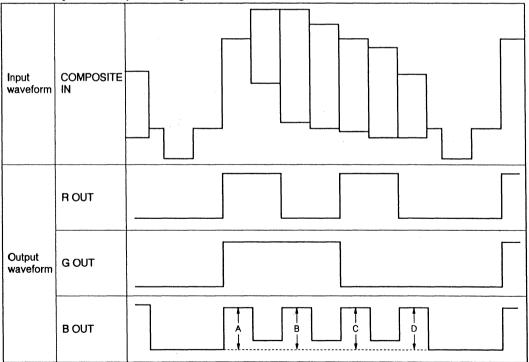
Adjustment Procedure (Input signal: 75% color-bar)
