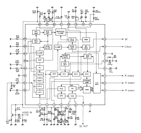
\* Change the C19 input capacitor polarity in accordance with the operating conditions.
