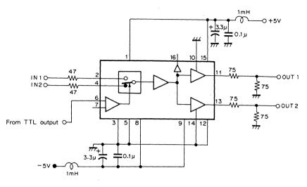
When the TTL output is low, the IN1 signal is output. When it is high, the IN2 signal is output.
