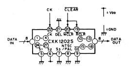
Fig. 3 Circuit of 123 bits delay
