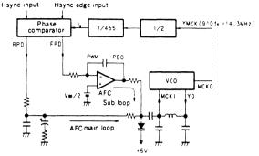
Input H sync, that edge and VCO ( $\approx$  910f<sub>H</sub>) counted down to 1/910 are phase compared. There are 2 such error outputs: RPD: phase comparison output between all sync bottom line and the built-in H counter, and FPD: between sync rising edge and the built-in H counter. RPD output is a lag-lead filter and FPD output is an integrator. Both outputs are converted into DC error respectively.
