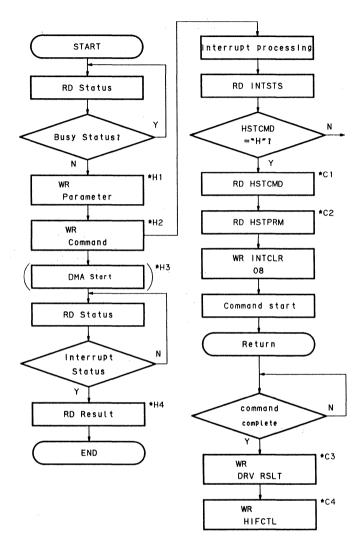
Fig. 4.2.1 Host and Sub CPU control
