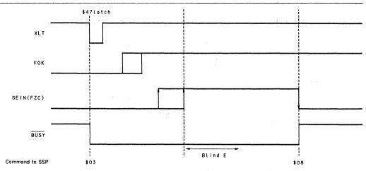
Figure 3-8 (b) Timing chart for auto focus operation
