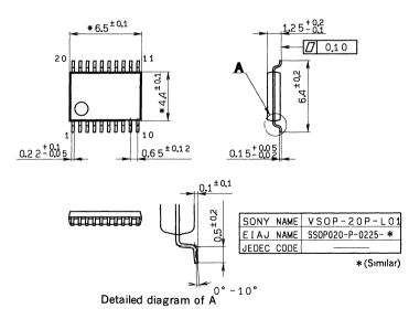
Note) Dimensions marked with \* do not include resin residue.
