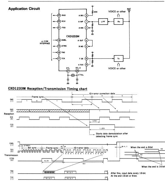
Divide ID+error data into 16-bit and input them from TND as NRZ signal. TCK is input clock. Inputs the first 16-bit within 8.5t. From the next 16-bit, input within 16t.
