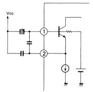
(b) How to form colpitts type oscillation circuits.
