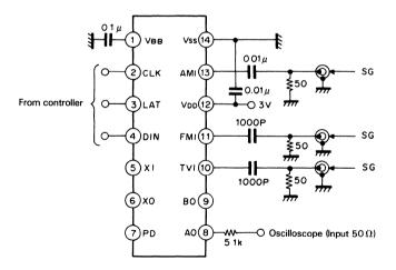
Control input data to CXD1118M. T1-H, T2-H, A-L, B-H SG: HP's 8640B (Input level read directly at 8640B's level meter)
