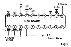
Electrical Characteristics Test Circuit 3 (Current Consumption)
