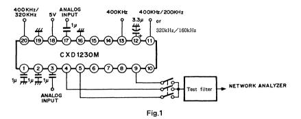
Electrical Characteristics Test Circuit 1 (Frequency Characteristics, Output Voltage)
