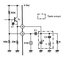
Colpitts type crystal oscillation circuit
