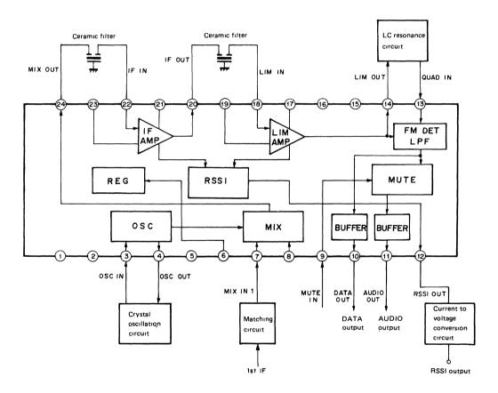
The RSSI output is the currents corresponding to the input levels at the IF amplifier and the limiter. It is possible to convert a current into a voltage by connecting a proper I. V conversion circuit.
