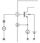
(a) How to input local oscillation signals from an external source.
