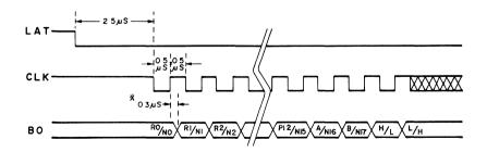
(\* Mark indicates data is output within this timing)
