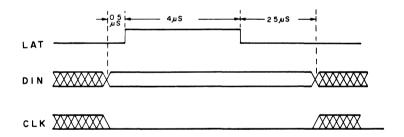
(c) DATA CHECK mode (Shift register data check)
