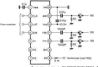
Control input data to CX-7925B/CXD1225M: T1-H, T2-H, A-L, B-H SG: HP's 8640B
