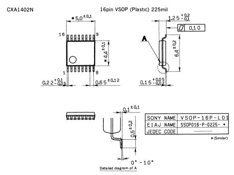
Dimensions marked with \* does not include resin residue
