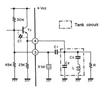
Colpitts type crystal oscillation circuit
