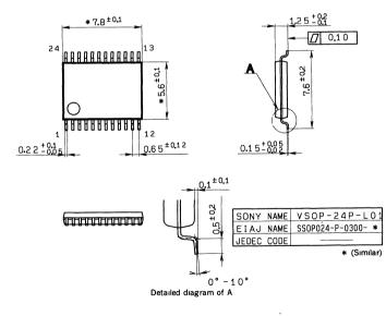
Dimensions marked with \* does not include resin residue
