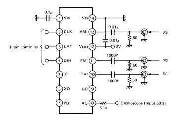
Control input data to CX-7961A/7961A-1 T1-H, T2-H, A-L, B-H SG HP's 8640B (Input level is directly read with the built-in level meter)
