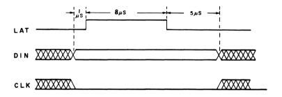
(3) DATA CHECK MODE (DATA check of the shift register)
