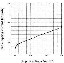
Supply voltage vs. Consumption Current
