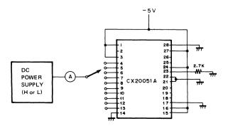
Fig. 2c Block diagram of input current test circuit
