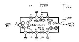
Fig. 3 Circuit of 123 bits delay
