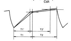
I/Csh should be kept constant for temperature change. If the temperature coefficient for Io/Iset, Iset, and Csh are defined as EI(Ei), Es, and Ec Total temperature coefficient is
