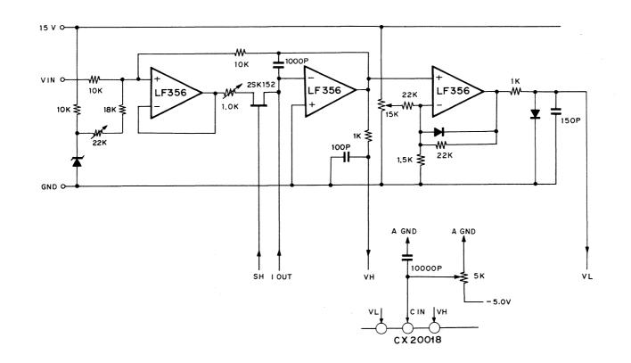
Fig. 7 Application Circuit (Non-inverting Circuit)
