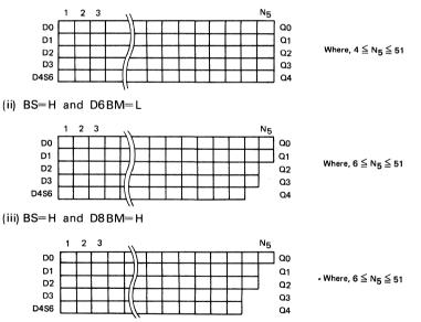
The stage selecting signal determines the number of the output stages after 3 clocks.
