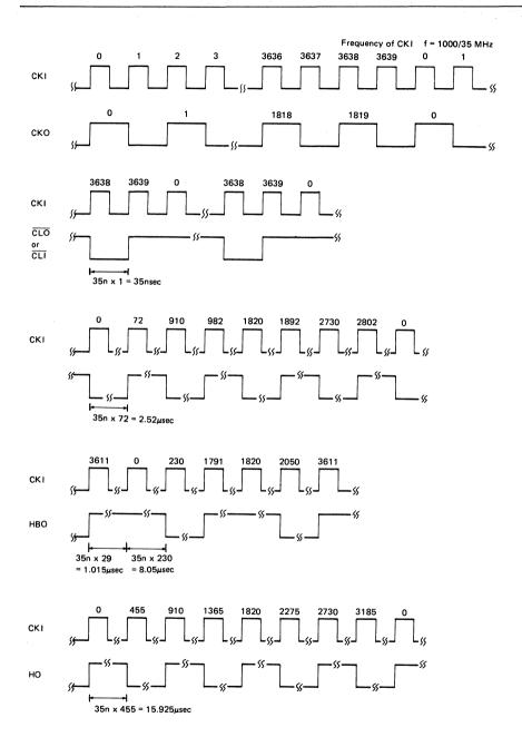
Fig. 5 The respective output timings against the input CKI
