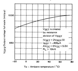
Output zero offset voltage vs. Ambient temperature
