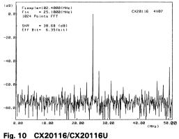
0 CX20116/CX20116U Spectrum with the aid of FFT at 102.4 MHz sampling and 25.1 MHz input.
