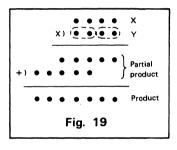
$$Y = -Y_{n} \cdot 2^{n} + Y_{n-1} \cdot 2^{n-1} + Y_{n-2} \cdot 2^{n-2} + \dots + Y_{3} \cdot 2^{3} + Y_{2} \cdot 2^{2} + Y_{1} \cdot 2^{1} + Y_{0} \cdot 2^{0} = (Y_{n-2} + Y_{n-1} - 2Y_{n}) 2^{n-1} + (Y_{n-4} + Y_{n-3} - 2Y_{n-2}) \cdot 2^{n-3} + \dots + (Y_{1} + Y_{2} - 2Y_{3}) \cdot 2^{2} + (Y_{-1} + Y_{0} - 2Y_{1}) \cdot 2^{0} = \sum_{k=0}^{n-1/2} (Y_{2k-1} + Y_{2k} - 2Y_{2k+1}) \cdot 2^{2k}$$
