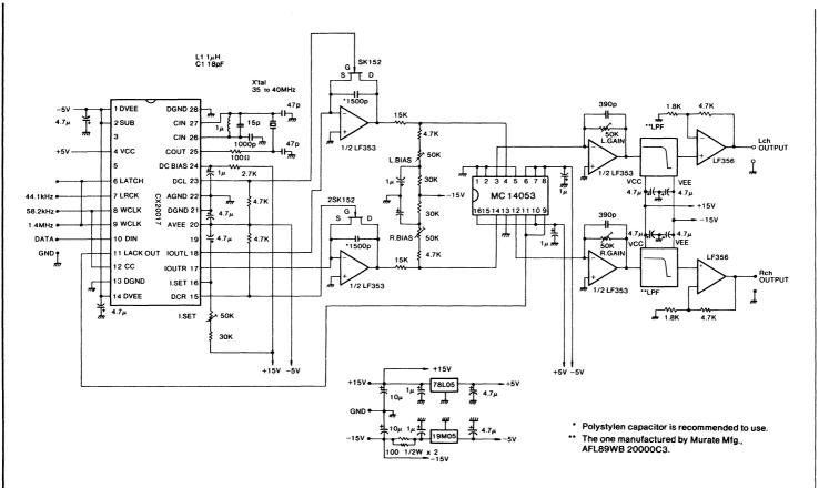
Fig. 1 CX20017PCB Schematic Diagram
