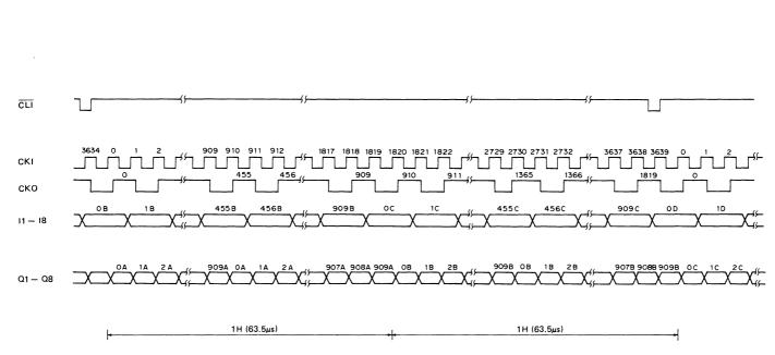
Fig. 2 Double speed conversion timing chart
