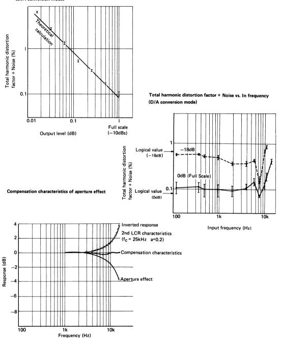
Total harmonic distortion factor + Noise vs. Output level (D/A conversion mode)
