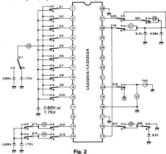
Test Circuit for Differential Linearity Error and Linearity Error
