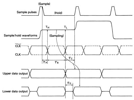
$T_H$  means a timing where  $V_{IN}$  and  $V_{REF}$  are compared and latched by the upper comparator, while  $T_L$  denotes a timing where  $V_{IN}$  and  $V_{REF}$  are compared and latched by the lower comparator.
