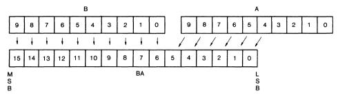
Fig. 6 "BA" Pin Configuration
