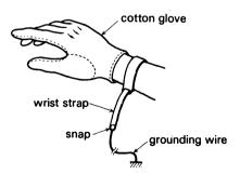
When using a copper wire for grounding, connect a 1M resistance in series near the hand for safety.
