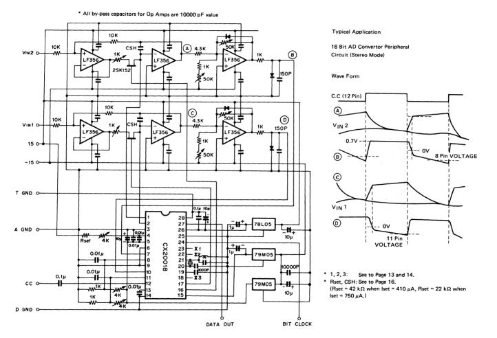
Fig. 5 16 bit A/D Converter Peripheral Circuit (Stereo Mode)
