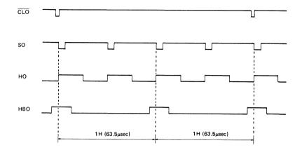
Fig. 4 The phase relationship between the respective outputs
