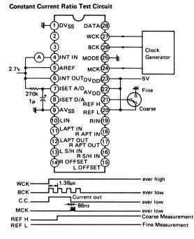
D/A conversion mode/Operational amplifier/ Amplification Gain Test Circuit
