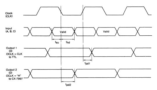
The above timing chart defines tpd, tsu and thd for the clock (CLK). The actual input/output operations are performed with a throughput delay having the number of clocks as shown in the operation mode throughput delay (Fig. 7).
