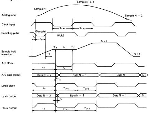
TH is the timing in which the upper level comparator compares VIN and VREF and latch the result. TL is the timing in which the lower level comparator compares VIN and VREF and latches the result.
