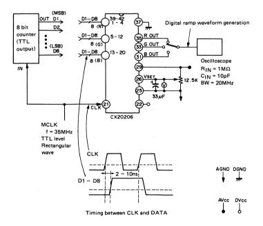
Output voltage full-scale precision, RGB output voltage full-scale ratio, and output zero offset voltage measuring circuits
