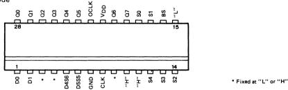
The data is input from D0 and D1 and output from the respective Q0 and Q1 after passing through the stages which specified by the stage selecting signal.
