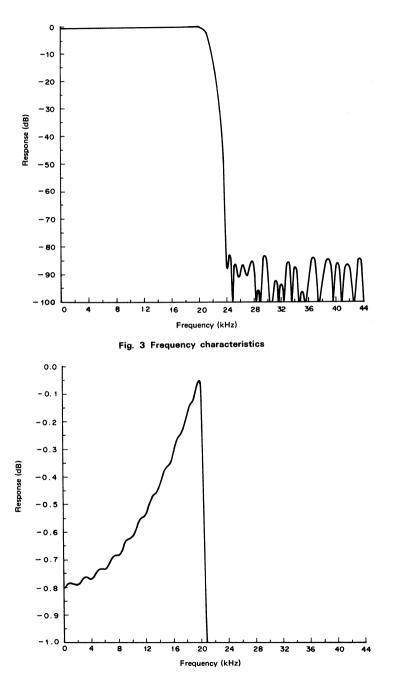
Fig. 4 Band passing characteristics
