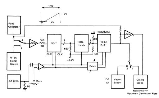
**Differential Non-linearity Measuring Circuit**
