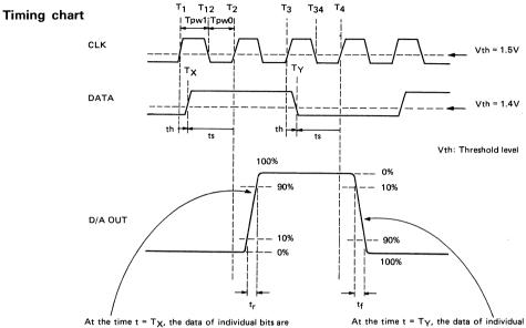
switched and thereafter when the CLK becomes  $L \rightarrow H$  at  $t = T_2$ , the D/A OUT is varied synchronous with it. That is, the D/A OUT is synchronous with the rise of the CLK.
