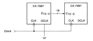
Fig. 4 External Device Interface (1)
