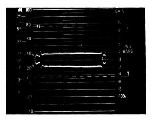
Condition Clock: 20 MHz Signal: NTSC. 40IRE mod. ramp.
