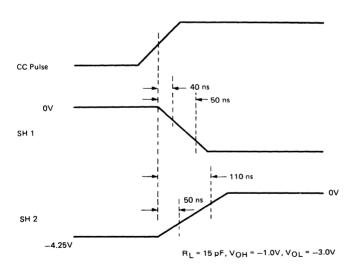
Propagation Delay Times from CC input to SH1, SH2 output
