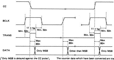
Only MSB is delayed against the CC pulse. Others are delayed against the bit clock. t<sub>M</sub>; One cycle of master clock The counter data which have been converted are transmitted to the shift register with the TRANS pulse. However, due to the circuit structure of the shift register, it cannot be transmitted unless the BCLK and TRANS are simultaneously at high.
