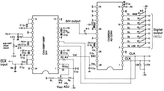
Fig. 5 Connection of CXA 1008P/1008P with CX20052A (1)
