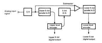
Fig. 1 Configuration of Series-Parallel 10-Bit A/D Converter
