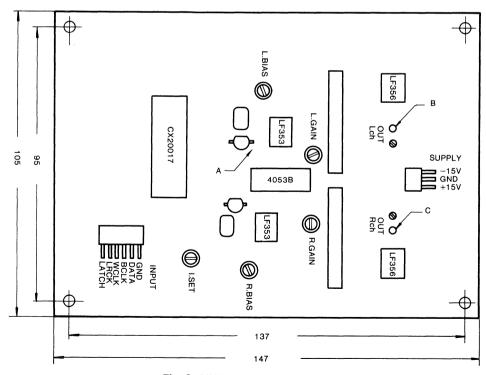
Fig. 8 CX20017PCB Check Points
