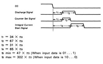
The counter set signal sets data entered in the latch to the counter, and is not output outside. The discharge signal is output from DCL and DCR and is controlled by LRCK. The signal is output from DCL when the level of LRCK is low, and from DCR when the level is high.
