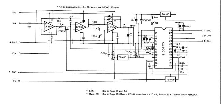
Fig. 6 16 bit A/D Converter Peripheral Circuit (Monaural Mode)
