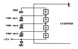
5. For reducing parasitic inductance and resistance, the wider area of GND pattern of the printed circuit board is the better.
