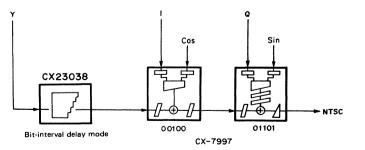
\* When the chroma signal is picked up which has been modulated as shown in Fig. above, the CX23038 of the bit-interval delay mode is used.
