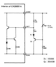
(6) When the analog output level is at full scale 1 Vp-p, the 1LSB becomes approximately 1 mV. In order to obtain the predesignated characteristics, due care should be exercised in the designing of the CX20051A periphery circuit.
