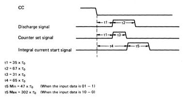
The counter set signal is used to set the data input in the latch to the counter but does not output externally.
