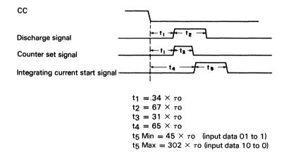
The counter set signal is to set the data input to the latch to the counter and it is not output externally.
