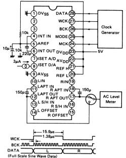
A/D conversion mode/Operational amplifier/ Amplification Gain Test Circuit
