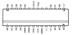
The data is input from D0, D1, D2, D3 and D4S6 and output from Q0, Q1, Q2, Q3 and Q4 respectively, after passing through the stages which is specified by the stage selecting signal. The S0 to S4 and D5S5 are the input pins of the stage selecting signal. Now, assuming that (i) D5S5="H"  $N_5=2^5+2^2\times S2+2S1+S0+4$
