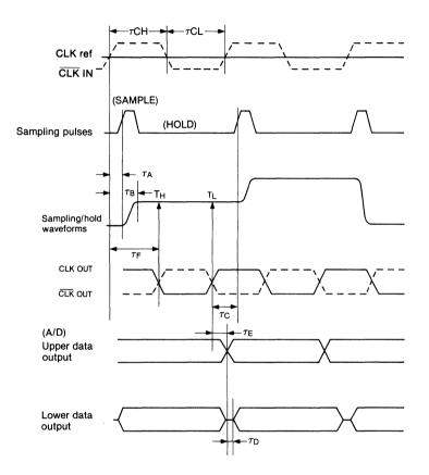
$T_{\rm H}$  shows a timing when the A/D latches upper 4 bits.  $T_{\rm L}$  shows a timing when the A/D latches lower 4 bits.
