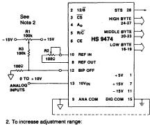
Figure 9a. Bipolar Input Connections with Trim Adjustment
