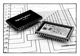
The HS9576 is a versatile building block for highaccuracy, high-speed systems. When used with the HS9716 sample (track)/hold, a high-speed acquisition system is formed which can digitize signals at a rate of 50,000 conversions per second. The HS9576 is available for operation over the commercial (0°C to +70°C) temperature range or -55°C to +125°C with full MIL-STD-883C screening.
