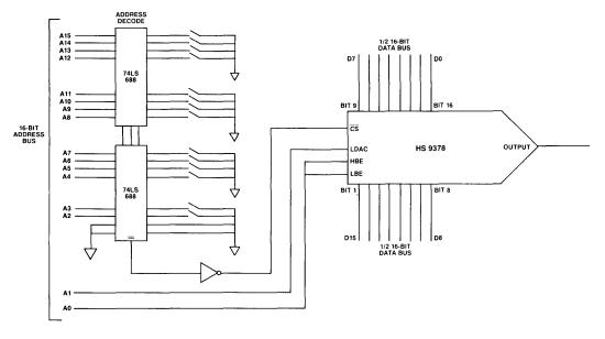
Figure 4. Block Diagram of HS 9378 Interfaced to 16-Bit µ P
