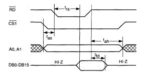
t<sub>as</sub> = address set-up time = 20 ns min.
