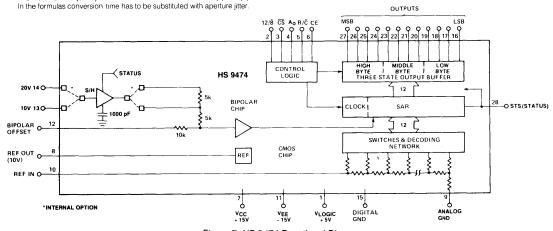
Figure 7. HS 9474 Functional Diagram
