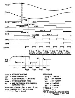
Figure 4B. Pipelined Sequential Data Acquisition System Using HS 9705
