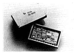
The HS 3860 includes an internal, precision reference supply, a fast output amplifier for minimum settling time, and input registers for easier microprocessor interface.
