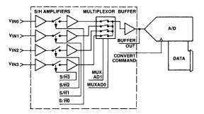
Figure 4A. Pipelined Acquisition DAS Using HS 9705
