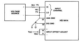
Figure 10. Suggested SPGIA Input Offset Calibration Circuit
