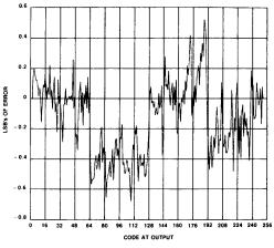
Graph 6. Dc Integral Linearity Error at  $F_{Sample} = 25 \text{ MHz}$
