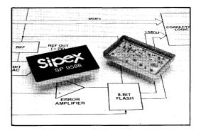
high speed, high accuracy data acquisition systems. The SP9588 is ideal in all applications that require 14-bit performance at relatively high speed with moderately low power consumption.
