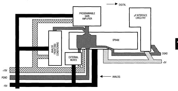
FIGURE 11 PCB LAYOUT FOR THE SP9488
