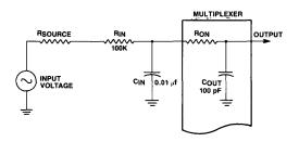
Figure 2. Input Decoupling Yields Poor Settling
