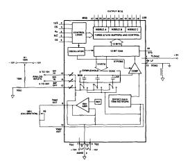
Figure 8. Unipolar Input Connections
