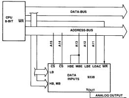
This mode of operation requires 13k bytes of unused addresses. No additional address decoder is necessary. The two chip-select input together with the byte-enable and load-DAC inputs are used to control all functions of the DAC. Through selecting the address-lines the user can vary the addresses used to control the DAC. In the above figure the control signals have the following address-configurations (hex):
