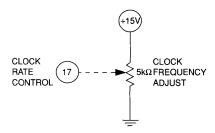
RANGE OF ADJUSTMENT IS TYPICALLY 7.5  $\mu s$  TO 4.0  $\mu s$  FOR 10 BIT AND 6.5  $\mu s$  TO 3.5  $\mu s$  FOR 8 BIT RESOLUTIONS.
