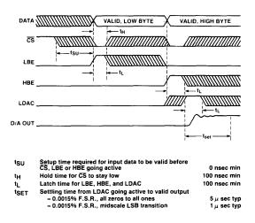
Figure 1. Timing Diagram for Interface to 8-Bit µ P Bus
