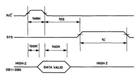
Figure 4. High Pulse For R/C – Outputs Enabled While R/C is High, Otherwise High Impedance
