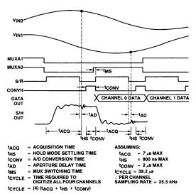
Figure 1A. Simple Sequential Four-Channel DAS
