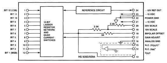
Analog ground and power ground must be externally connected to each other. Power ground is connected to case.
