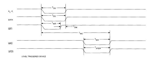
WRITE CYCLE TIMING DIAGRAM
