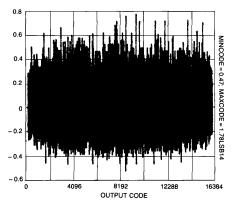
Figure 18. HS 9476 Dynamic Differential Linearity, Fin = 23.456kHz, Fsample = 50kHz
