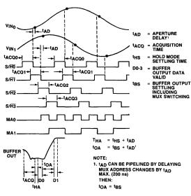
Figure 4. Pipelined Acquisition Sequential Sampling Using HS 9705.
