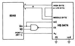
Figure 6. Interfacing the HS 9474 and a 8048 µP
