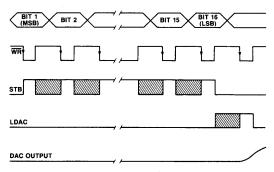
Figure 3. Global Timing for Complete Operation of the HS 9372.
