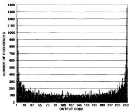
Figure 16. Histogram of HS 1068,  $F_{IN}$  = 8.9 MHz,  $F_S$  = 20 MHz
