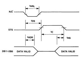
Figure 3. Low Pulse For R/C - Outputs Enabled After Conversion
