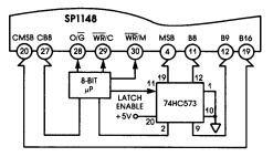
Figure 2. Connections For 8-Bit Bus Interface
