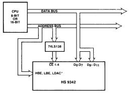
\*For 8-Bit Data Bus, HBE and LBE addressed separately as high byte and low byte. For 16-Bit Data Bus, HBE and LBE are tied together and addressed as one word.
