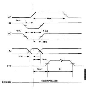
Figure 1. Convert Mode Timing Diagram
