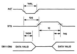
Figure 3. Low Pulse For R/C - Outputs Enabled After Conversion
