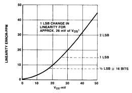
Actual measurement of 26-27mV compares favorably with the calculated value of 28.5mV (Table 2).
