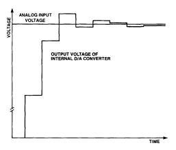
Figure 3. Internal Sequence of an A/D Conversion
