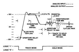
Figure 1. Pictoral Showing Various S/H Characteristics
