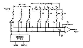
Figure 12 HS 3120 Decoded 12-bit DAC—2MSB's decoded followed by conventional 10-bit R–2R DAC
