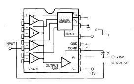
Sample charging rate =  $\frac{l_1}{C}$  V/sec. Hold drift rate =  $\frac{l_2}{C}$  V/sec. Switch pedestal error =  $\frac{Q}{C}$  Volts.
