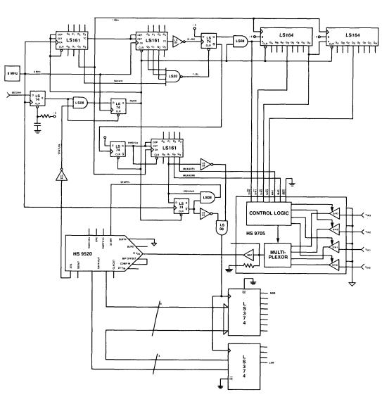
Figure 6. Pipelined Acquisition DAS for 250 kHz Throughput Using HS 9705
