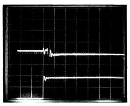
Figure 6. Sample-to-Hold Step (Top), HOLD Command (Bottom) Scale: 20mV/div, vertical; 500 ns/div, horizontal
