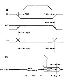
Figure 2. Read Mode Timing Diagram
