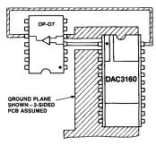
Figure 9 PCB Assembly Layout
