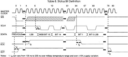
For asynchronous mode, transitions of SCLK, SDATA, EOC, EOT can shift by up to 4 clocks; e.g. the first high to low transition of SCLK may be on clock #6 to #9. The timing relationship between SCLK, SDATA, EOC, and EOT is fixed.
