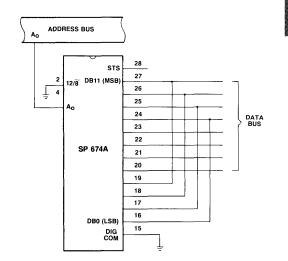
Figure 10. Interfacing the SP 674A to an 8-Bit Data Bus
