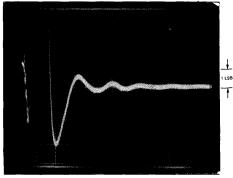
4c. Small Scale Settling. Scale: Vertical 5mV/cm (approx. 1 LSB), Horizontal 1µs/cm. 4c is basically an expanded version of 4b.
