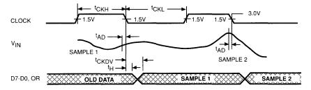
$t_{\mbox{CKDV}}$  and  $t_{\mbox{H}}$  measured at output levels of 0.8 and 2.4 volts.
