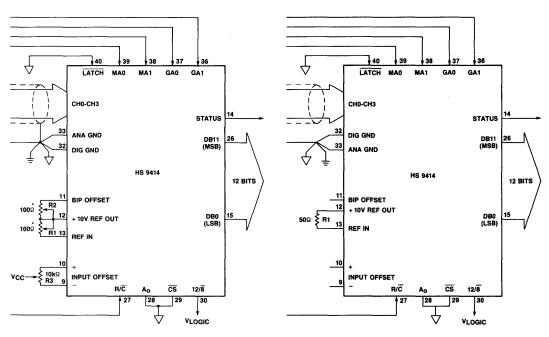
Figure 2a. Bipolar Stand-Alone Connections with Offset and Gain Adjustments
