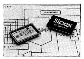
The HS9476 allows analog input ranges of  $\pm$ 5V,  $\pm$ 10V, 0 to +10V, and 0 to +20V. Integral nonlinearity is specified at  $\pm$ 0.003% of FSR maximum, while no missing codes is guaranteed for the full operating temperature range. The HS9476 is available for operation over the commercial (0°C to 70°C) temperature range or  $-55^{\circ}$ C to  $+125^{\circ}$ C with full MIL-STD-883C screening.
