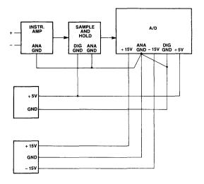
Figure 15. Proper Grounding Technique
