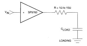
FIGURE 2 CAPACITIVE LOADING
