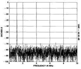
Figure 11. FFT of Ideal 8-Bit Converter
