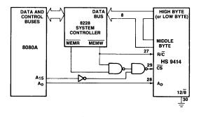
Figure 6. Interfacing the HS 9414 and 8080A µP
