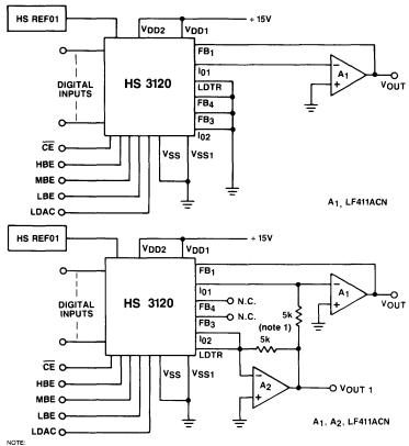
External resistors should be selected for good bipolar offset tempco and need only track well.
