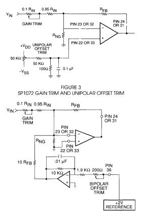
FIGURE 4 SP1072 GAIN TRIM AND BIPOLAR OFFSET TRIM
