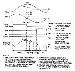
Figure 3. Timing Diagram of Simultaneous Sampling (HS 9704)<sup>2</sup>
