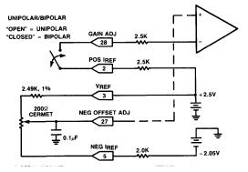
Figure 2. Unipolar/Bipolar Range Offset Adjustment Circuit
