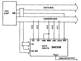
This mode of operation requires 13k bytes of unused addresses. No additional address decoder is necessary. The two chip-select inputs together with the byte-enable and load-DAC inputs are used to control all functions of the DAC. Through selecting the address-lines the user can vary the addresses used to control the DAC. In the above figure the control signals have the following address-configurations (hex):
