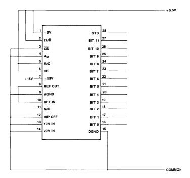
Figure 12. Burn-In Schematic
