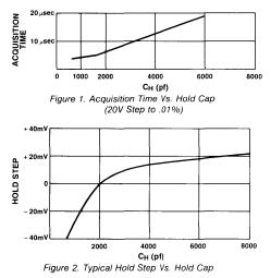
The hold capacitor is connected between pins 12 and 17. If an alternate capacitor is used, the designer must consider the errors that will be introduced. **CAUTION:** Polystyrene capacitors will be damaged if subjected to temperatures above +85°C.
