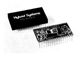
The HS9516 is available with 14-bit ( $\pm 0.003\%$  FSR), 15-bit ( $\pm 0.0015\%$  FSR) or 16-bit ( $\pm 0.0008\%$  FSR) nonlinearity. The B versions are fully screened and tested to MIL-STD-883C and are packaged in a hermetic 32-pin DIP.
