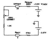
Figure 1. Unipolar Mode – External Offset Adjustment
