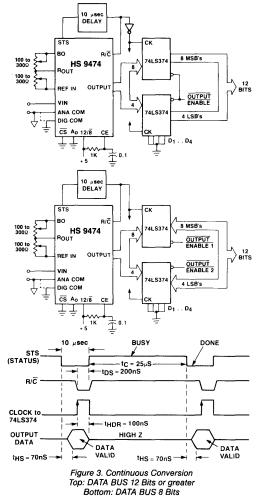
$\overline{CS}$  and  $A_o$  are tied low (0) while 12/ $\overline{B}$  is tied high (1) to select the converter and enable a 12-Bit conversion. Note  $A_o$  is 'don't care' in the truth table.
