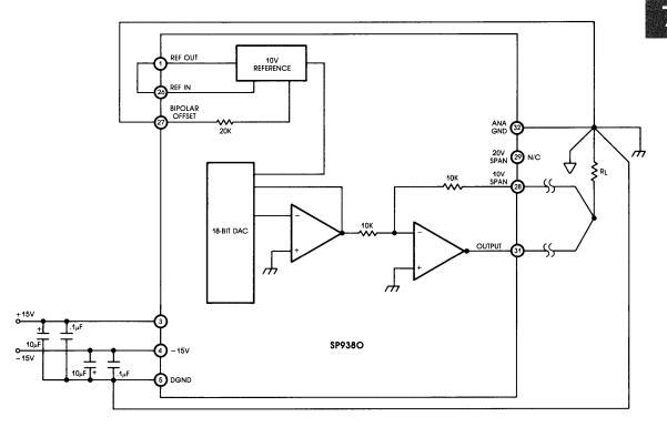
The "holy point" grounding technique consists of choosing a ground reference point where ground returns of different systems' components are connecting. Separate ground returns are provided to minimize the current flow in the path from sensitive points to the system "holy" point. For example, supply currents do not flow in the same return path with an analog signal, or logicgate return currents are not summed into the return from a precision reference.
