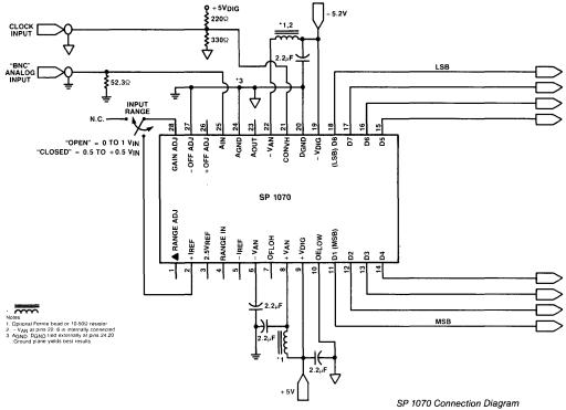
Minimal Power Dissipation Application Circuit
