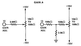
Two Methods Offering A ±1% Swing. Unipolar & Bipolar: Apply a +(F.S. -3/2LSB) analog input and set the potentiometer for a digital output that alternates between 000...0 and 000...1.
