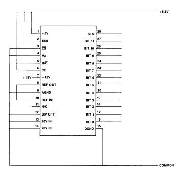
Figure 12. Burn-In Schematic
