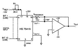
FIGURE 4: Unipolar Operation
