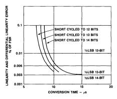
Figure 10. HS 9476 Nonlinearity Vs. Conversion Time
