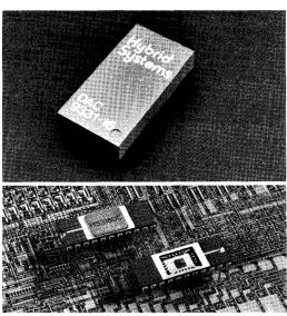
High resolution DAC's developed by Hybrid Systems include: DAC9331-16 (top) industry's first 0.0008% accurate Hybrid DAC and HS 3160 (bottom) 16-bit CMOS MDAC guaranteed monotonic to 14 bits (0.003%) from - 25°C to + 85°C. Figure 1
