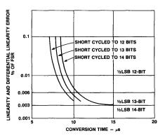
Figure 7. HS 9576 Nonlinearity Vs. Conversion Time
