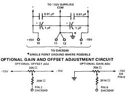
CALIBRATION PROCEDURE (for optional external Gain & Offset adjustment)
