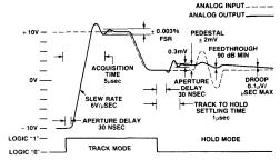
Figure 13. Illustration of the Main S/H Characteristics
