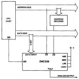
Interfacing the DAC338 to a 16-Bit microprocessor is quite easy, because no multiplexing of the data inputs is necessary. An address decoder and the second chip-select input is used to select the DAC.
