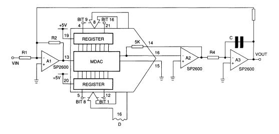
FIGURE 8 DIGITALLY CONTROLLED LOW PASS FILTER
