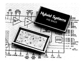
The 9403 is packaged in a 62-pin, hermeticallysealed, ceramic package. Temperature ranges available are 0°C to 70°C for commercial versions and -55°C to 125°C with MIL-STD-883C screening for military grades.
