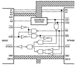
FIGURE 16 INTERFACE OF THE SP9488 TO A 68000 TYPE  $\mu P$
