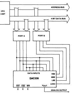
This figure shows how to operate the DAC338 with two 4-Bit ports. The chip-selects are tied to ground allowing continuous operation; they can be used for operating more DAC's at the same port. In the first step data should appear at the port A outputs; in the second step the control flags should appear on port B.
