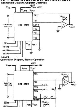
Connection Diagram, Bipolar Operation (for applications where bipolar offset temperature drift ( $\approx$  10 ppm/<sup>o</sup>C) is not critical)
