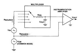
Figure 5. Pseudo-Differential Connection Degrades Common Mode Rejection
