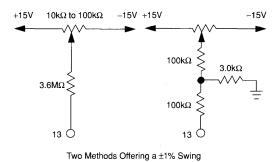
Unipolar & Bipolar: Apply a +(F.S. -3/2 LSB) analog input and set the potentiometer for a digital output that alternates between 000 ... 0 and 000 ... 1.
