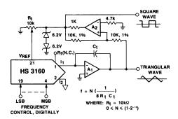
Figure 7. Programmable Function Generator
