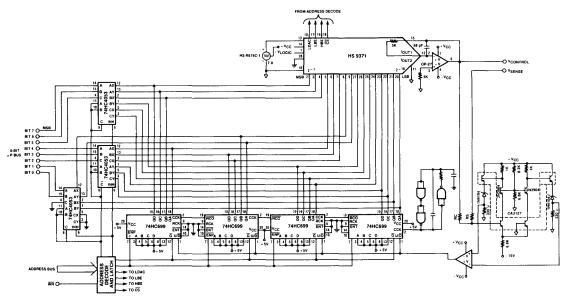
Figure 6. Bus Programmable Sense and Control Servo Loop for Precision Robotics Applications
