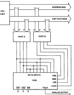
This figure shows how to operate the HS 9338 with two 4-Bit ports. The chip-selects are tied to ground allowing continuous operation; they can be used for operating more DAC's at the same port. In the first step data should appear at the port A outputs; in the second step the control flags should appear on port B.
