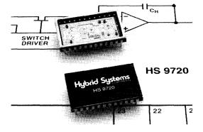
The HS9720 is packaged in a 24-pin DIP and is specified for operation from  $0^{\circ}$ C to  $+70^{\circ}$ C for commercial grades, and  $-55^{\circ}$ C to  $+125^{\circ}$ C for military grades. Full screening to MIL-STD-883C is available.
