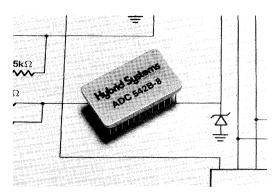
All models can be externally pin-connected for 3 unipolar and 3 bipolar input ranges. Output coding in the bipolar mode is user selectable as either offset binary or 2's complement. ADC541/542 feature an overall temperature coefficient of  $\pm$ 45 ppm/°C and long-term stability of 0.1%/year.
