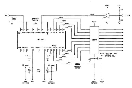
Figure 10. Isolating Digital Ground Noise From Converter Using RL Isolation at Digital Grounds (100Ω Resistors Used to Series Terminate Long Runs) 8
