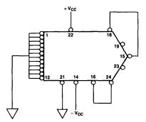
NOTE: Bypass each supply with a  $1\mu$ F tantalum and a  $0.01\mu$ F ceramic to Common.
