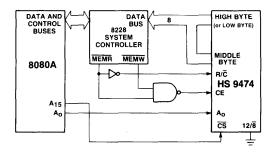
Figure 5. Interfacing the HS 9474 and 8080A μP
