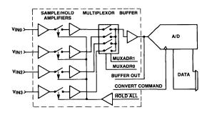
Figure 3A. Simultaneous Sampling DAS Using HS 9704
