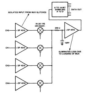
VERY HIGH SPEED BUFFERED DAS FOR MAGNETIC RESONANCE IMAGING ON CAT SCANNER APPLICATIONS
