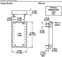
Pin 1 is marked by a dot on the top of the package.
