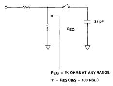
Figure 6. Equivalent SP 674A Input Circuit
