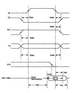
Figure 2. Read Mode Timing Diagram
