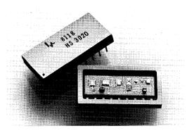
Hybrid Systems guarantees linearity and accuracy not only at room temperature but also at the extremes of the operating range of -55 °C to +125 °C.
