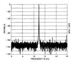
Figure 15. FFT of the HS 9476, Fin = 12.234kHz, Fsample = 50kHz
