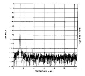
Figure 12. FFT of the SP9480, Fin = 1.123kHz, Fsample = 25kHz
