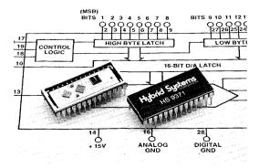
The HS9371 has dual 8-bit input registers for direct interface to 8- or 16-bit bus structures. The pinout of the HS9371 allows the user with an 8-bit bus to run only 8 traces directly underneath the hybrid to connect to the 16-bit input register.
