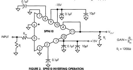
If the expected output voltage swings are small, it is possible to operate the output stages from  $\pm 5V$  supplies; this will reduce power dissipation and junction tempera-
