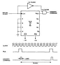
Figure 4. Generation of the CONVERT COMMAND
