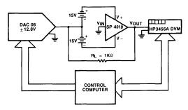
Figure 3. DC Test System
