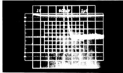
Acquisition Time of a Worst Case 20V Step (Plus to Minus Input) Top trace shows hold command going high in the second horizontal division. Lower trace shows output settling to a 500  $\mu$  V/div. scale.
