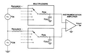
Figure 6. Balanced Differential Approach Preserves Common Mode Balance
