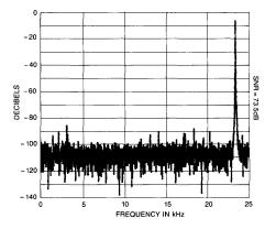
Figure 17. FFT of the HS 9476, Fin = 23.346kHz, Fsample = 50kHz, - 6dB input levels
