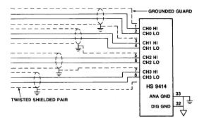
Figure 13. Recommended Input Wiring Layout
