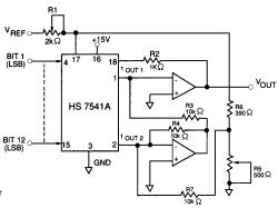
FIGURE 5: Bipolar Operation
