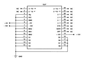
Figure 10. HS 9410 Burn-In Schematic
