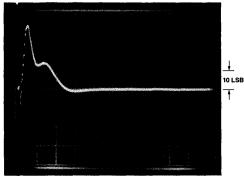
Data not latched. Scale: Vertical 10 LSB/DIV, Horizontal 0.5 s/cm. See improved performance using latches, Fig. 4b.
