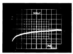
Hold Mode Dielectric Absorption Sag For 5µsec Sample Period Without Dielectric Absorption Compensation
