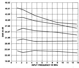
Figure 14. HS 1068 SNR Vs. Frequency Showing 0 to -24 dBInput Levels, F<sub>S</sub>= 20 MHz
