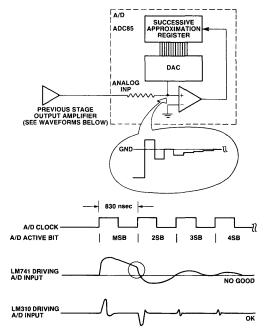
Figure 14. Dynamic Voltage Shifts can Couple Back Thru Input Resistor and Upset Amplifier Output of Previous Stage. The Amplifier Driving the Analog Input must Settle Back between Succesive Bit Cycles.
