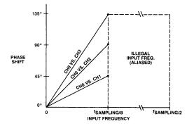
Figure 2. Phase Shift Between Channels Versus Input Frequency in Four-Channel Sequential Sampling DAS (shown below)
