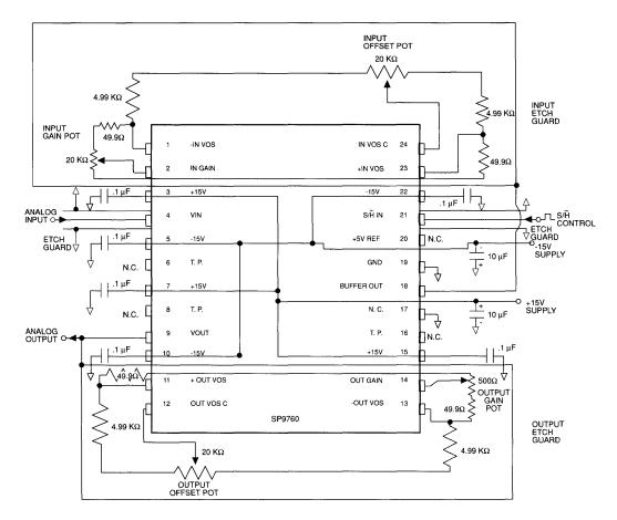
FIGURE 1 SUGGESTED TOPOLOGY AND RELATIVE PLACEMENT OF COMPONENTS
