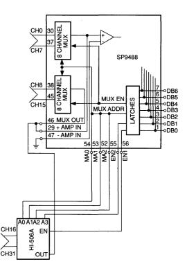
FIGURE 2b INPUT EXPANSION OF THE SP9488 (32 SINGLE-ENDED CHANNELS)
