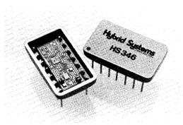
FAST SIGNAL ACQUISITION — a small internal holding capacitor is combined with a high slew rate output amplifier for a fast signal acquisition time of  $2\mu$ s max.
