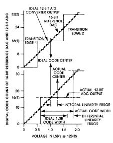
Figure 4. 12-Bit ADC Linearity Testing
