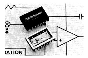
The HS9716/HS9714 comes complete with an internal hold capacitor and is available for use over the 0°C to 70°C temperature range and the -55°C to + 125°C military temperature range. Full screening to MIL-STD-883C is available.
