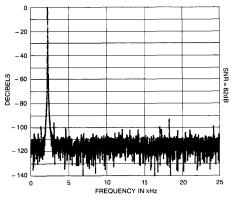
Figure 14. FFT of the HS 9476, Fin = 2.234kHz, Fsample = 50kHz
