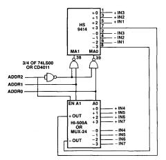
Figure 15. Input Expansion for HS 9414 (From 4 to 7 Channels)
