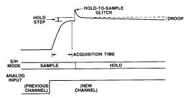
Figure 7b. Typical Sample-and-Hold Output Behavior
