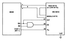
Figure 7. Interfacing the HS 9414 with a 8048 µP.
