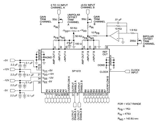
FIGURE 5 SP1072 CONNECTION DIAGRAM CHANNEL A 0 TO 1V INPUT CHANNEL B ±0.5V INPUT
