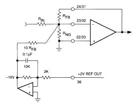
FIGURE 2 TYPICAL BIPOLAR CONNECTIONS
