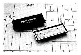
The HS9414 is offered in a ceramic package for commercial ( $0^{\circ}C$  to + 70°C) and military (-55°C to + 125°C) applications with processing available in full compliance with MIL-STD-883C.
