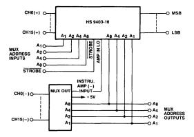
Figure 2. 16-Channel Differential Input Expansion
