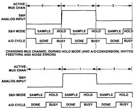
THIS TIMING MINIMIZES FEEDTHRU ERRORS
