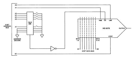
Figure 2. Block Diagram of HS 9378 Interfaced to 8-Bit µP
