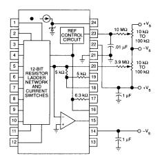
FIGURE 3 EXTERNAL ADJUSTMENT AND VOLTAGE SUPPLY CONNECTION DIAGRAM
