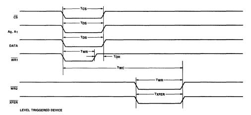
Write Cycle Timing Diagram
