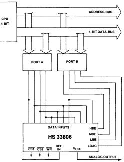
This figure shows how to operate the HS 33806 with two 4-Bit ports. The chip-selects are tied to ground allowing continuous operation; they can be used for operating more DAC's at the same port. In the first step data should appear at the port A outputs; in the second step the control flags should appear on port B.
