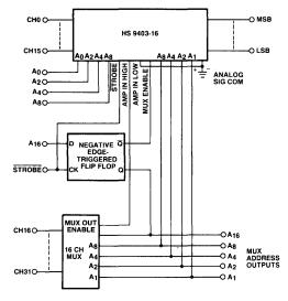
Figure 3. 32-Channel Single-Ended Input Expansion
