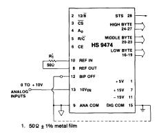
Figure 8b. No Trim Unipolar Input Connections
