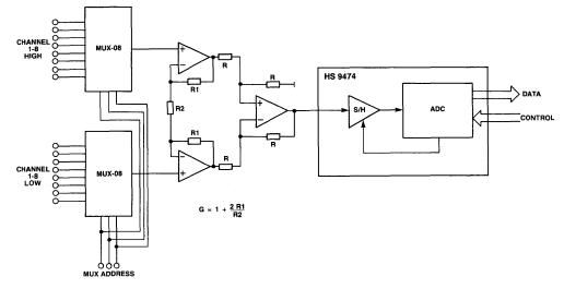
Figure 9. Data Acquisition System with 8 Differential Channels
