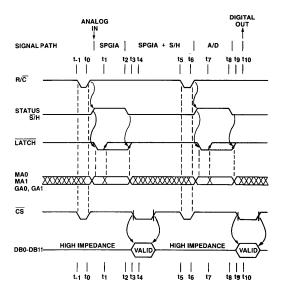
Figure 4. HS 9414 Pipeline Timing for Highest Throughput
