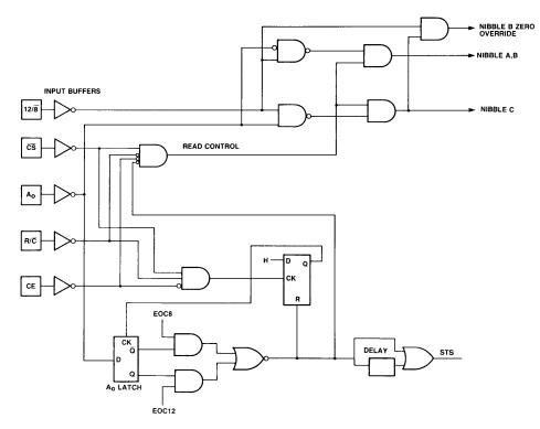
Figure 11. SP 674A Control Logic
