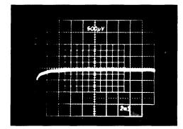
Hold Mode Dielectric Absorption Sag For 5µsec Sample Period With Dielectric Absorption Compensation
