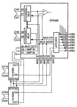
FIGURE 2c INPUT EXPANSION OF THE SP9488 (16 DIFFERENTIAL CHANNELS)
