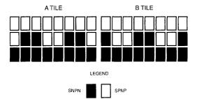
High Gain, high bandwidth complimentary vertical NPN & PNP transistors coupled with precision thin film resistors and capacitors make the SP1000 family ideally suited for implementing cost effective ASIC solutions to high speed and high precision analog signal conditioning and signal processing applications.
