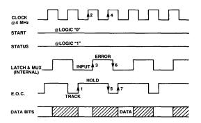
SP 9548 Timing Diagram: Continuous Conversion Mode
