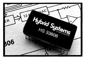
to the DAC register. In addition to these input functions are two chip select inputs and a read/write input allowing direct memory-map configurations. All input controls are static to allow hardwired configurations. The HS33806 is packaged in a hermetically sealed package and is rated -55°C to +125°C. Units are fully screened and processed to MIL-STD-883 requirements.
