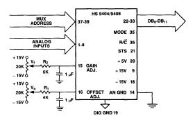
Figure 3. Gain and Offset Input Connections
