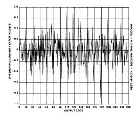
Graph 7. SP1072 Dynamic Diffl $_{\rm in}$  Error at  $F_{\rm in}$  = 5+ MHz, Fs = 25 MHz
