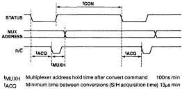
t<sub>ACQ</sub> Minimum time between conversions (S/H acquisition time) 13μs min t<sub>CON</sub> Conversion time for 16-Bit resolution J,K-Models 25μs max S,T-Models 25μs max
