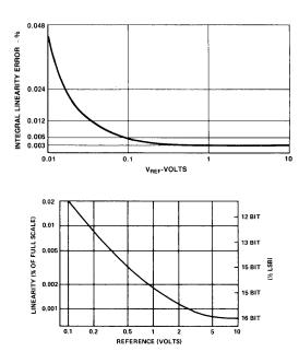
Figure 15 Linearity VS Reference Voltage, HS 3160 (top), DAC9331-16 (bottom)
