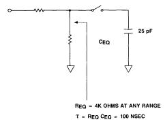
Figure 6. Equivalent HS 574A Input Circuit
