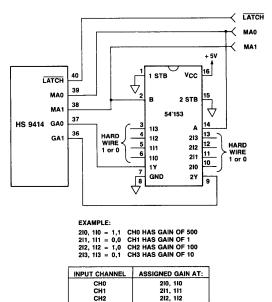
Figure 14. Input Channel Assigned Gain
