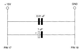
FIGURE 2 RECOMMENDED BYPASS CIRCUIT
