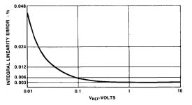
Integral Linearity Error vs. Reference Voltage
