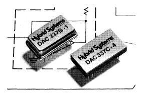
choice of four output voltage ranges: 0 to + 10, 0 to - 10 (unipolar) and  $\pm$  5,  $\pm$  10 (bipolar).
