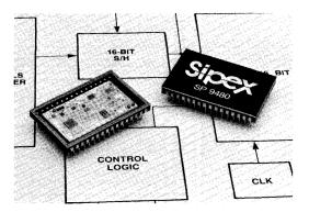
The SP9480 Series is offered in a hermeticallysealed 32-pin package and operates from  $\pm 15V$ and  $\pm 5V$  with a total power consumption of 1200mW. Four basic product grades are available; J and K models are specified over a temperature range of 0°C to  $\pm 70°$ C while the S/B and T/B models are specified over an extended temperature range of  $\pm 55°$ C to  $\pm 125°$ C. Full screening to MIL-STD-883C is available with models specified as "B."
