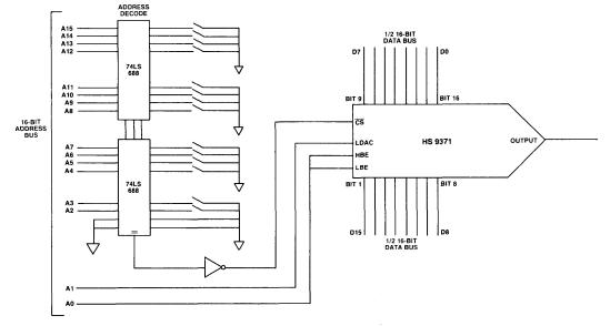
Figure 4. Block Diagram of HS 9371 Interfaced to 16-Bit µP
