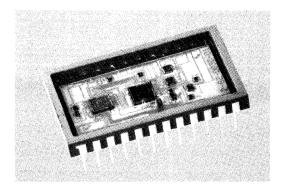
The DAC87A series is pin compatible with the popular DAC87 DAC. An input register is incorporated within the CMOS switch circuit. The latch control for the input register is connected to pin 13. Pin 13 can be connected to +5V or left open and the HSDAC87A will function as a DAC87. In addition pin 13 can be used to 'latch' data into the input registers, see Figure 3.
