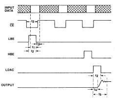
TIME AXIS NOT TO SCALE. ALL STROBES ARE LEVEL TRIGGERED. 1; Data Setup Time. Time data must be stable before strobe (byte enable/LDAC) goes to "0", 11 (min) = 250 nsec. 12; Strobe Width. 12 (min) = 250 nsec. (CE, LBE, HBE, LDAC).
