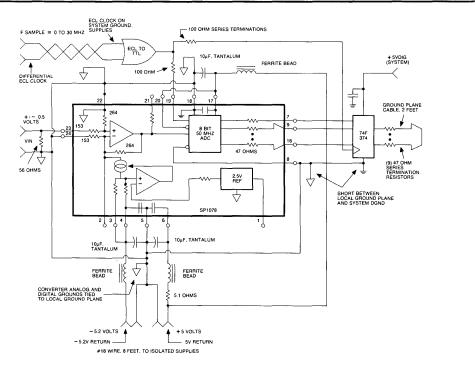
FIGURE 4 BIPOLAR INPUT, NON-INVERTING CIRCUIT FOR OPERATION UP TO FSAMPLE = 30 MHZ
