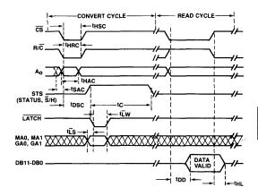
Figure 1a. HS 9414 Interface Timing
