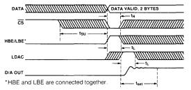
Figure 3. Timing Diagram for Interface to 16-Bit µ P Bus
