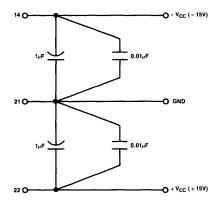
Figure 6. Recommended Power Supply Bypass
