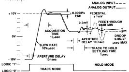
Figure 2. Pictoral Showing Various S/H Characteristics
