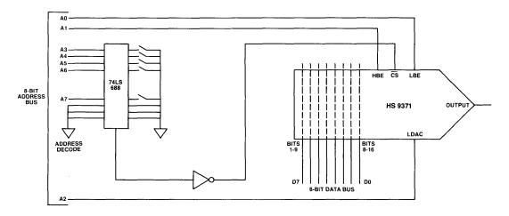
Figure 2. Block Diagram of HS 9371 Interfaced to 8-Bit µP
