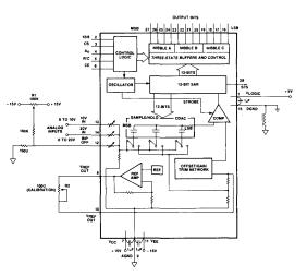
Figure 8. Unipolar Input Connections
