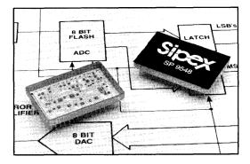
The SP9548 input range, 0 to +5V, has been optimized for high speed applications such as radar, sonar and video digitization, and high speed data acquisition systems. The SP9548 is ideal in all applications that require 12-bit performance at high speed with low power consumption.
