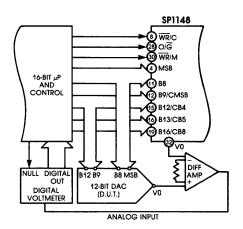
Figure 5. DAC Testing
