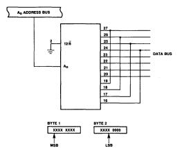
Figure 7. Enabling Data in 8-Bit Mode
