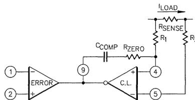
Figure 5. Current Limit With Optimized Frequency Compensation
