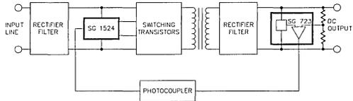
Figure 23. Input/Output Isolation
