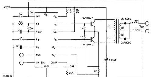
Figure 21. 5V, 25W, DC to DC Converter
