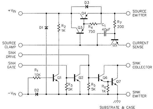
Figure 7. SG1629 Floating Switch Driver Schematic Diagram
