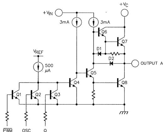
Figure 11. SG1525A Pulse Width Modulator Power Output Stage
