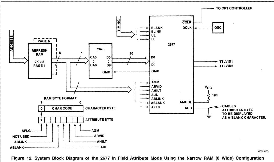
Figure 12. System Block Diagram of the 2677 in Field Attribute Mode Using the Narrow RAM (8 Wide) Configuration
