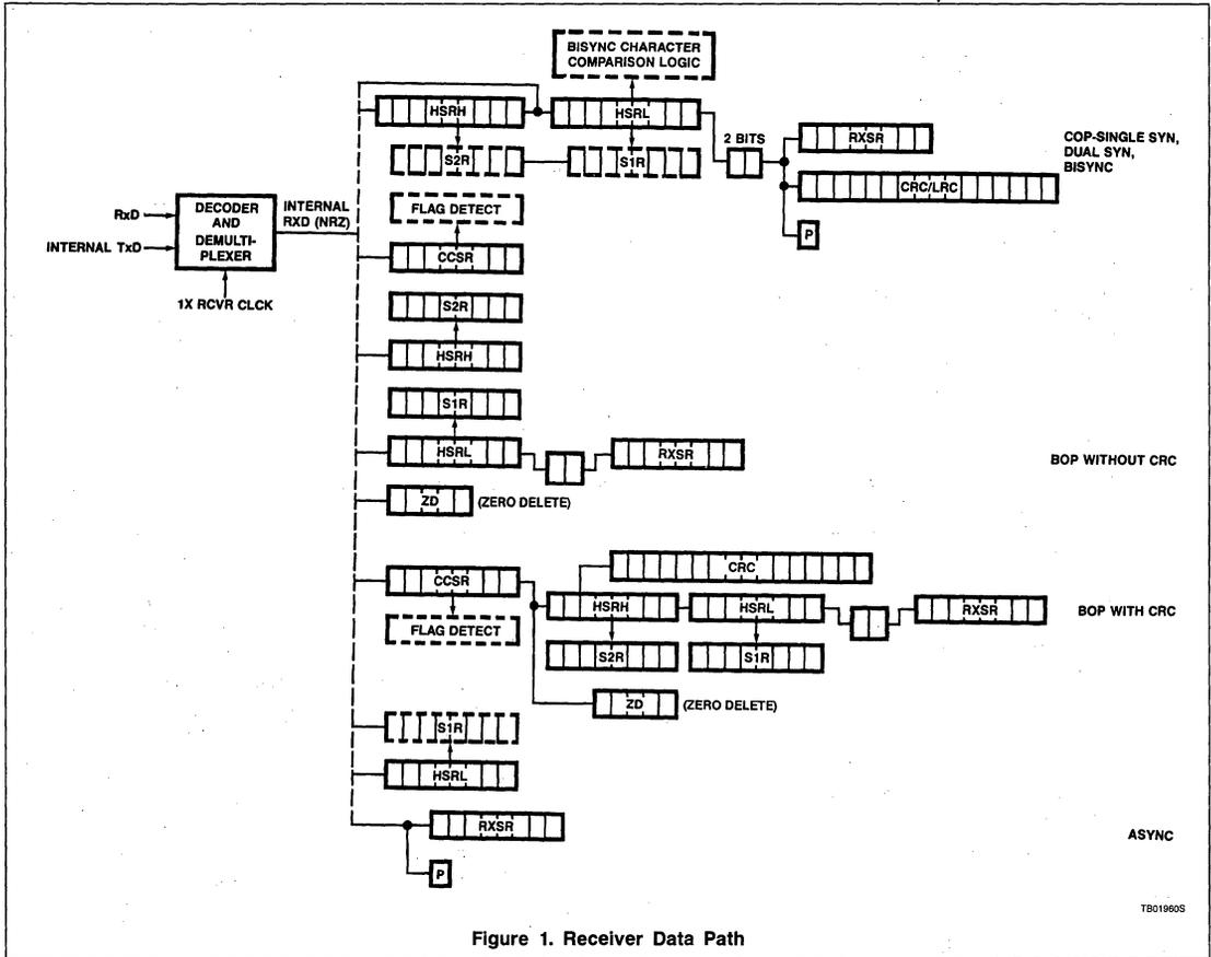
Figure 1. Receiver Data Path
