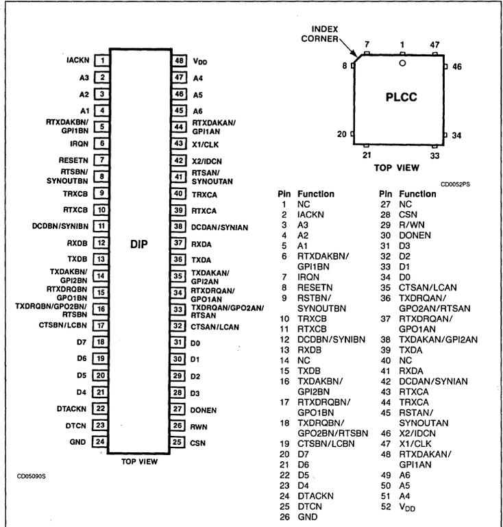
Two modem control inputs (DCD and CTS) and three modem control outputs (RTS and two general purpose) are provided. Because the modem control inputs and outputs are general purpose in nature, they can be optionally programmed for other functions.
