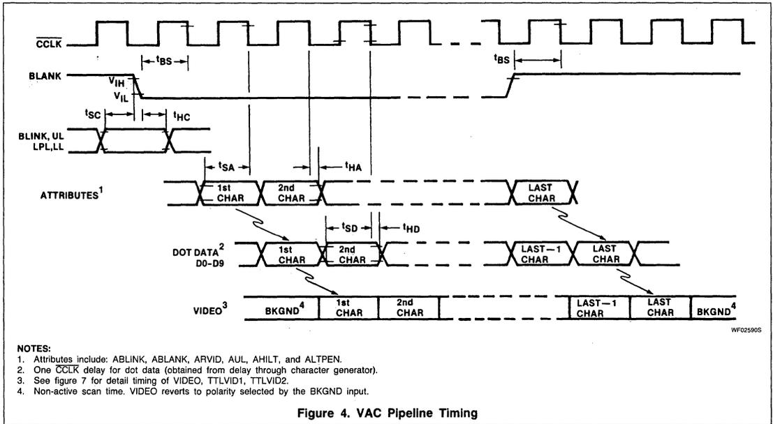
Figure 4. VAC Pipeline Timing
