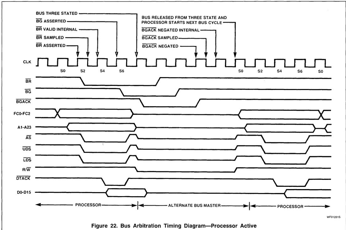
Figure 22. Bus Arbitration Timing Diagram—Processor Active
