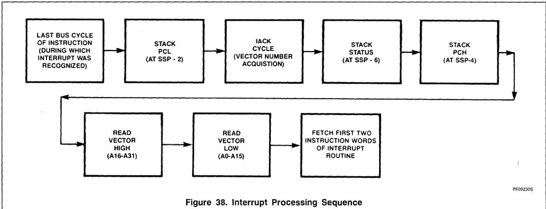
Figure 38. Interrupt Processing Sequence
