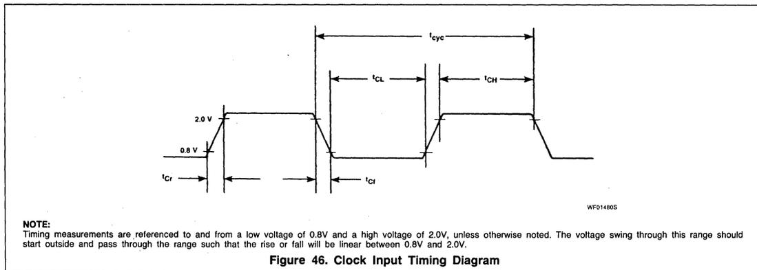
NOTE: Timing measurements are referenced to and from a low voltage of 0.8V and a high voltage of 2.0V, unless otherwise noted. The voltage swing through this range should start outside and pass through the range such that the rise or fall will be linear between 0.8V and 2.0V.
