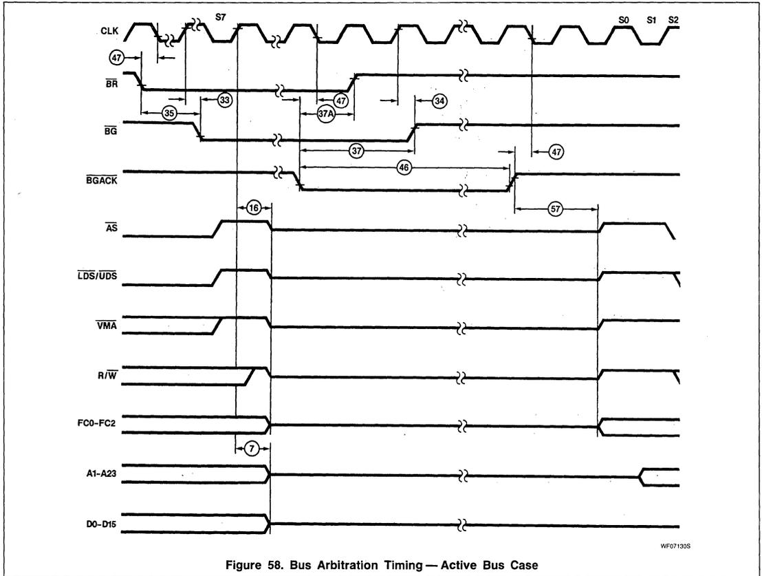
Figure 58. Bus Arbitration Timing — Active Bus Case
