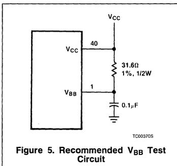
**Figure 5. Recommended  $V_{BB}$  Test Circuit**
