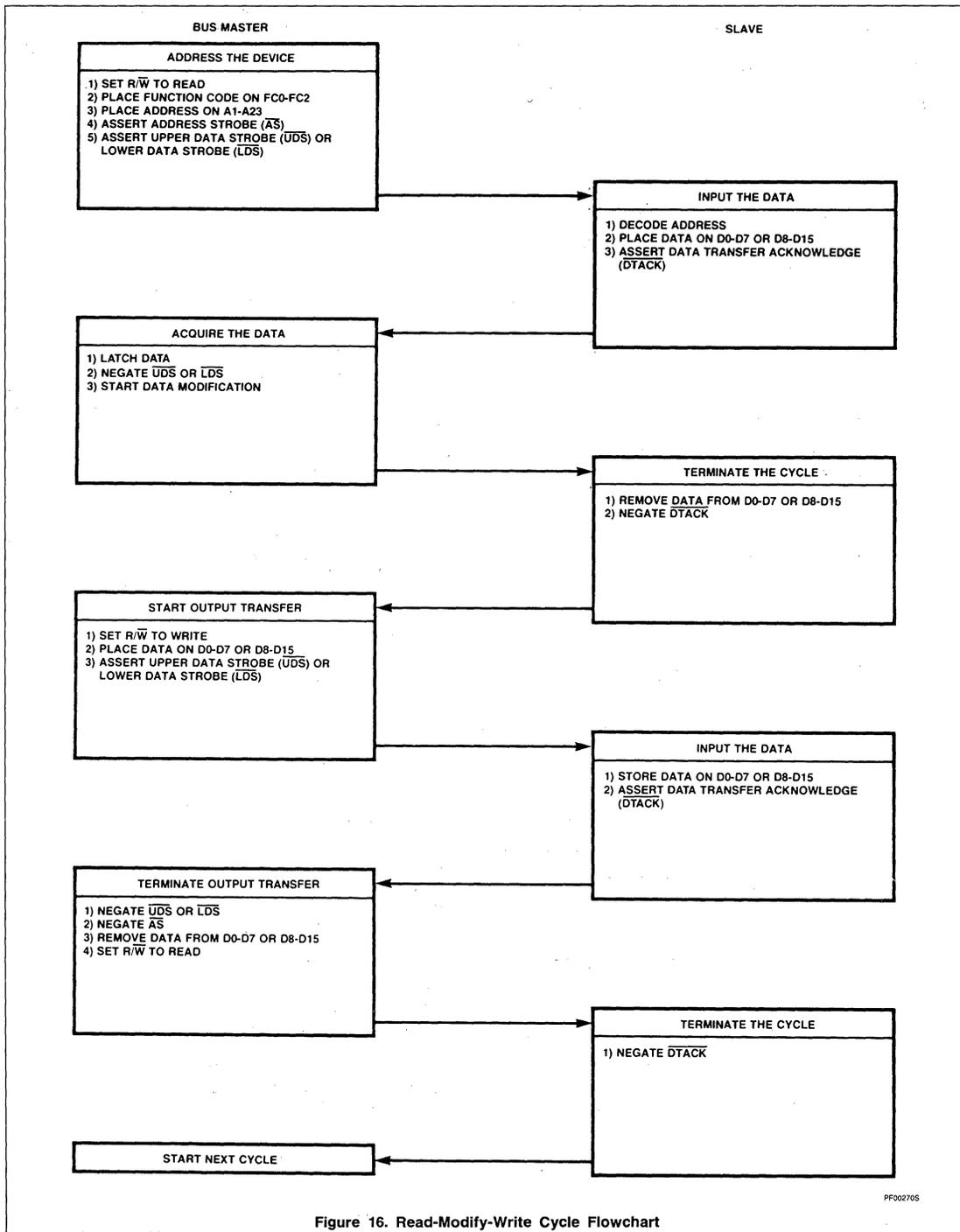
Figure 16. Read-Modify-Write Cycle Flowchart
