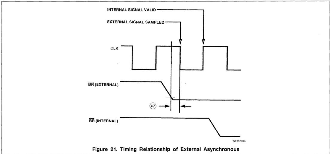
Figure 21. Timing Relationship of External Asynchronous
