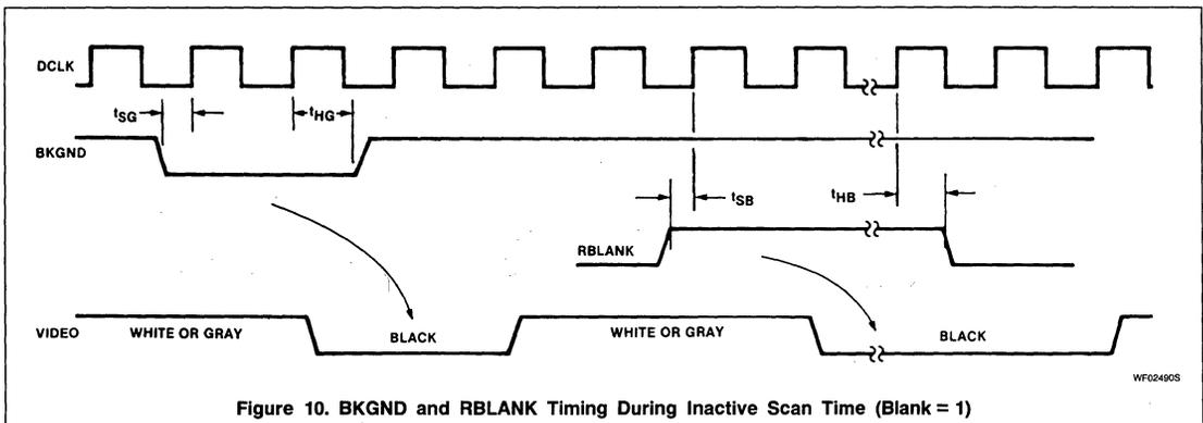
Figure 10. BKGND and RBLANK Timing During Inactive Scan Time (Blank = 1)
