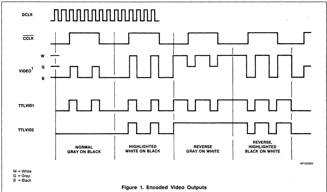
Figure 1. Encoded Video Outputs
