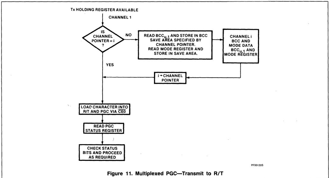
Figure 11. Multiplexed PGC—Transmit to R/T
