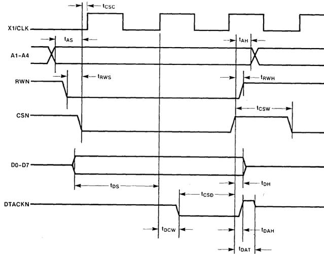
Figure 3. Bus Timing (Write Cycle)
