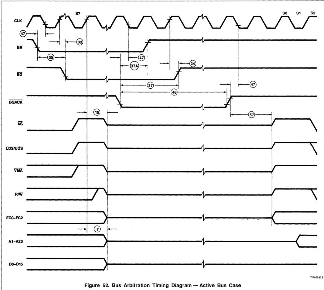
Figure 52. Bus Arbitration Timing Diagram — Active Bus Case
