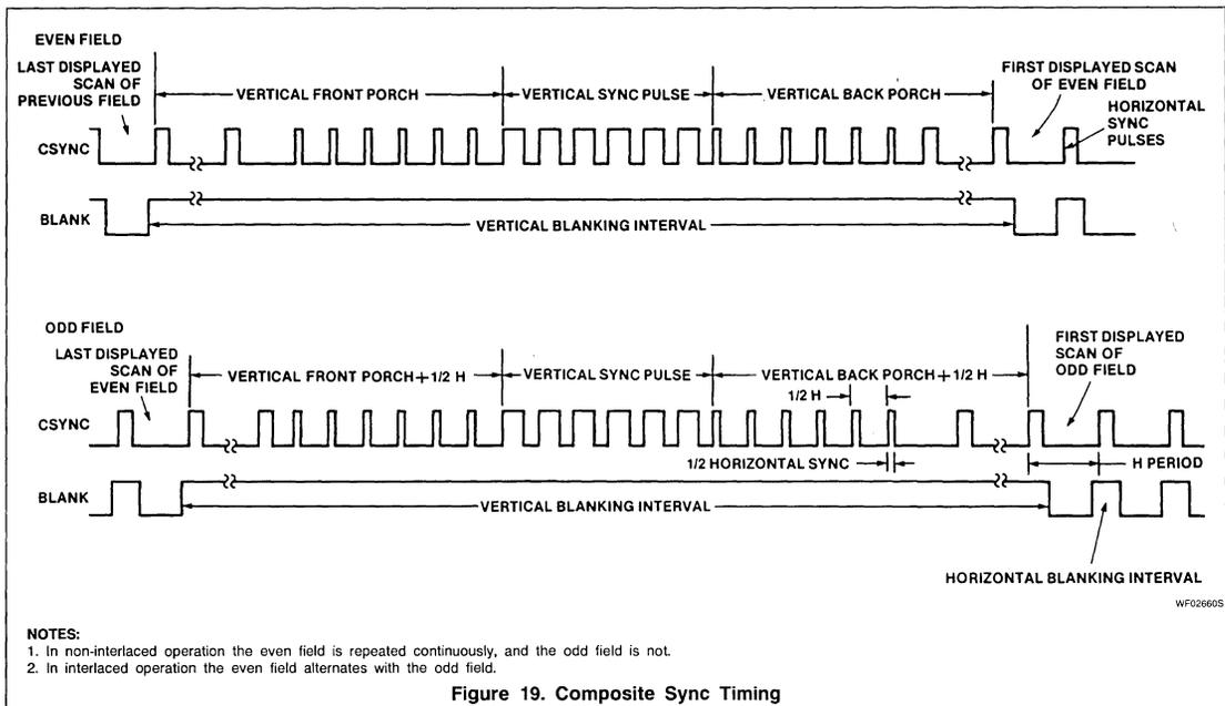
Figure 19. Composite Sync Timing
