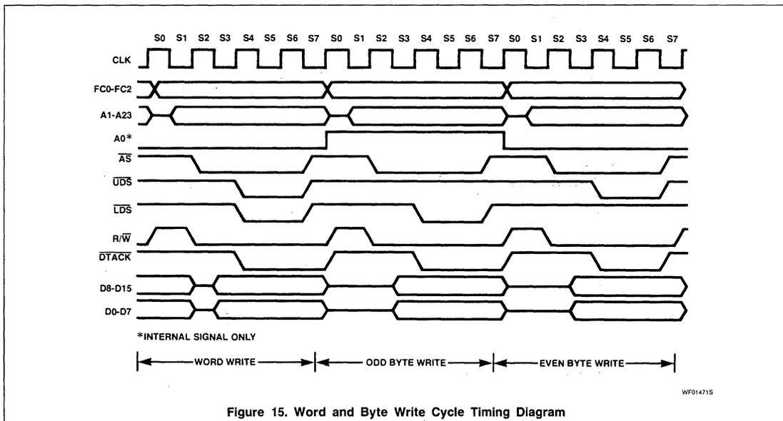
Figure 15. Word and Byte Write Cycle Timing Diagram
