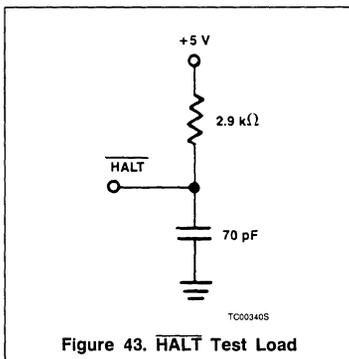
Figure 43. HALT Test Load
