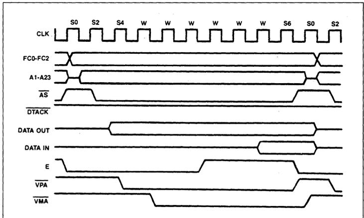
Figure 39. SCN68000 to Synchronous Peripheral Timing — Best Case
