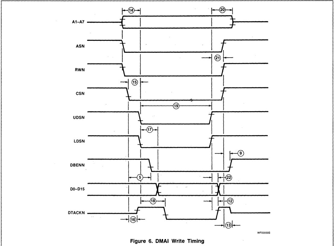
Figure 6. DMAI Write Timing
