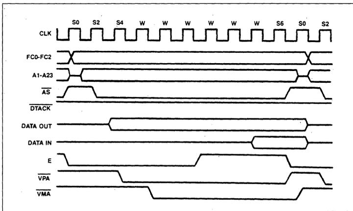
Figure 44. SCN68010 to Synchronous Peripheral Timing Diagram — Best Case
