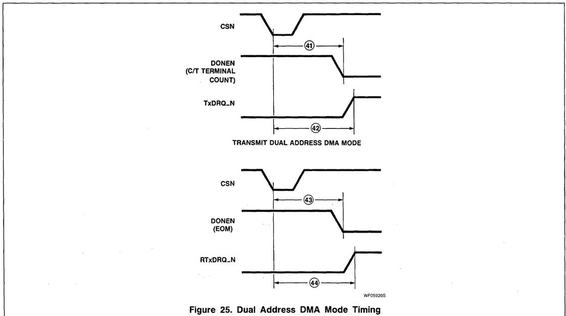
Figure 25. Dual Address DMA Mode Timing
