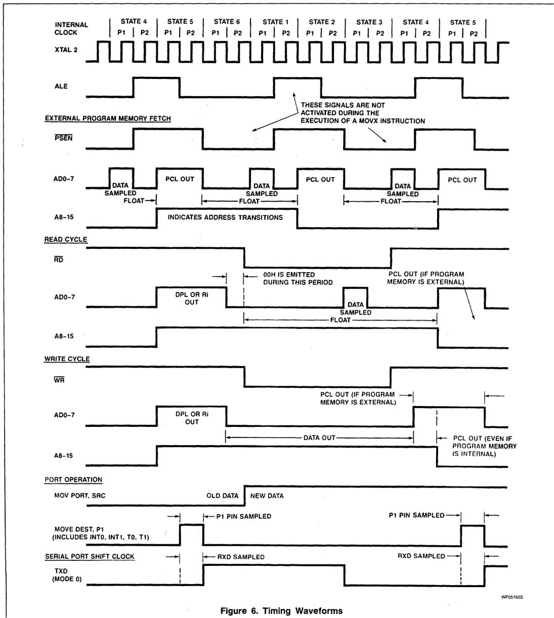
Figure 6. Timing Waveforms
