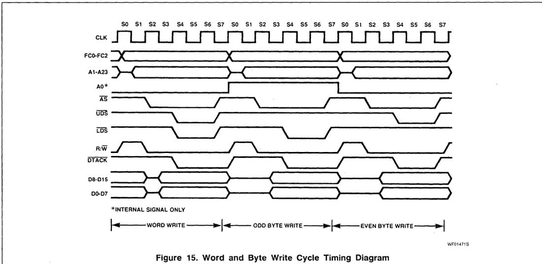
Figure 15. Word and Byte Write Cycle Timing Diagram
