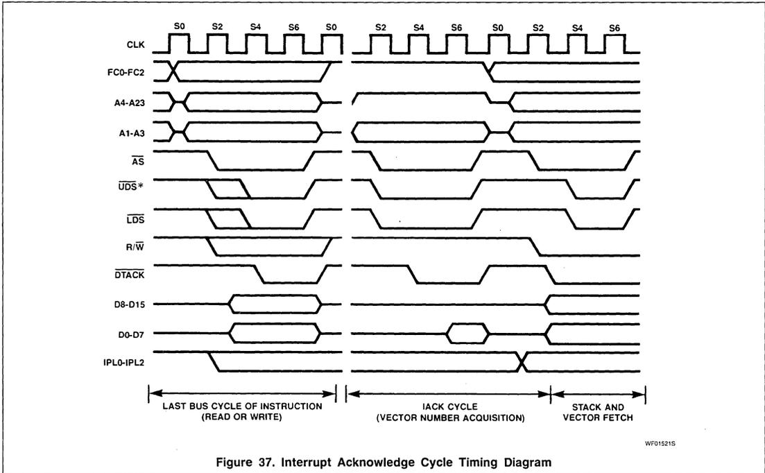
Figure 37. Interrupt Acknowledge Cycle Timing Diagram
