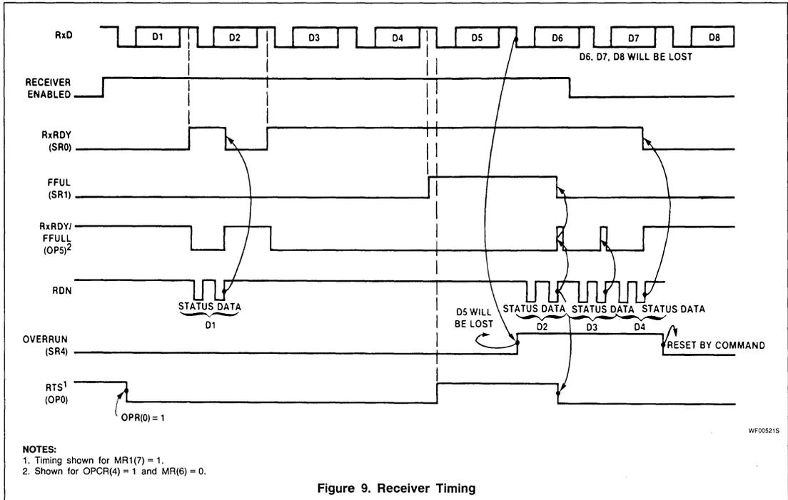
Figure 9. Receiver Timing
