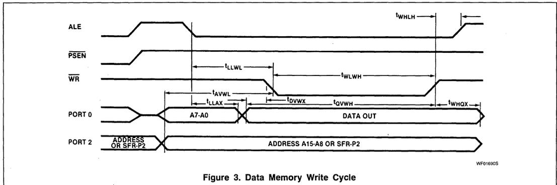
Figure 3. Data Memory Write Cycle
