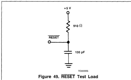
Figure 49. RESET Test Load
