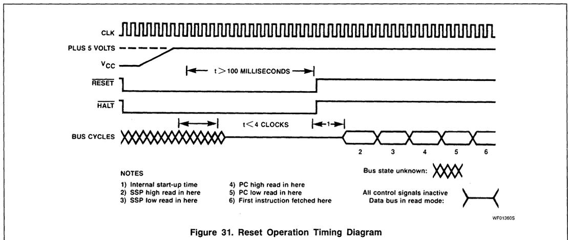
Figure 31. Reset Operation Timing Diagram
