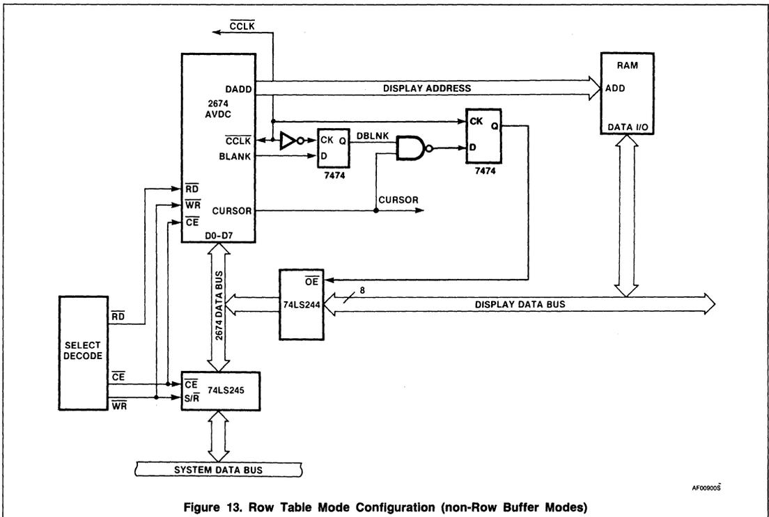
Figure 13. Row Table Mode Configuration (non-Row Buffer Modes)
