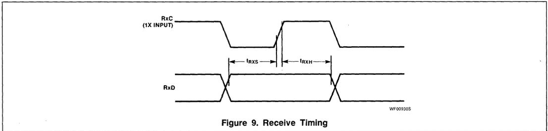
Figure 9. Receive Timing
