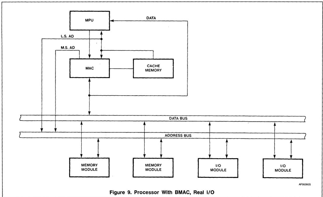
Figure 9. Processor With BMAC, Real I/O
