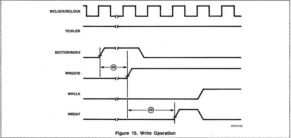
Figure 15. Write Operation
