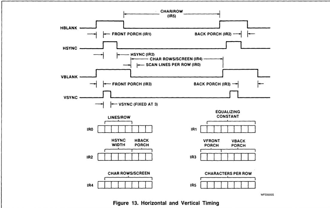
Figure 13. Horizontal and Vertical Timing
