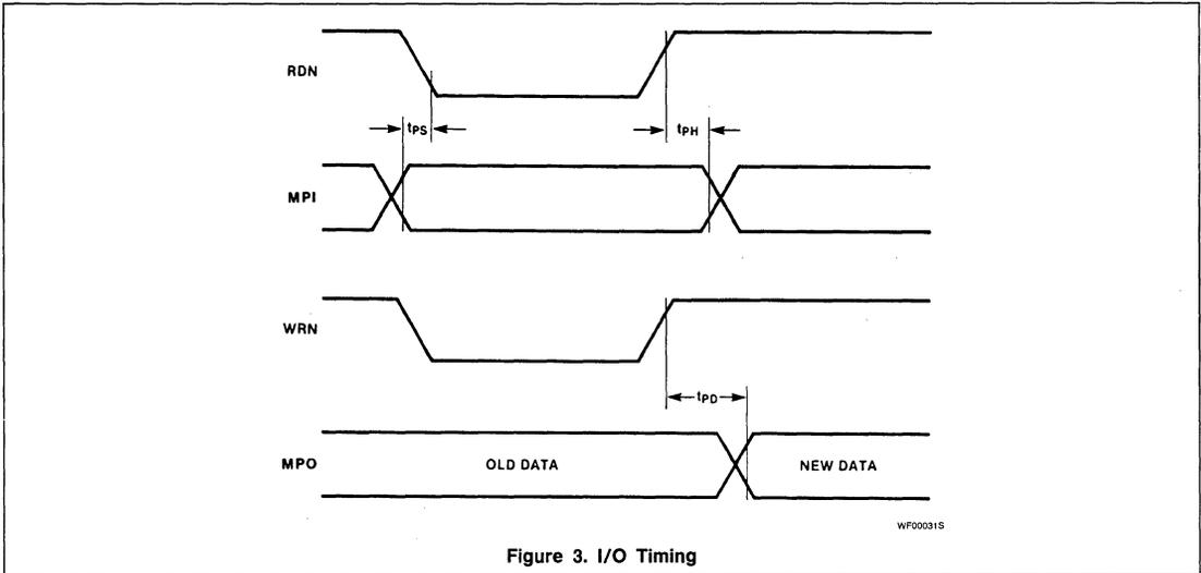
Figure 3. I/O Timing
