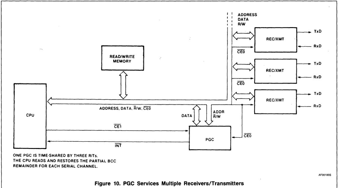
Figure 10. PGC Services Multiple Receivers/Transmitters
