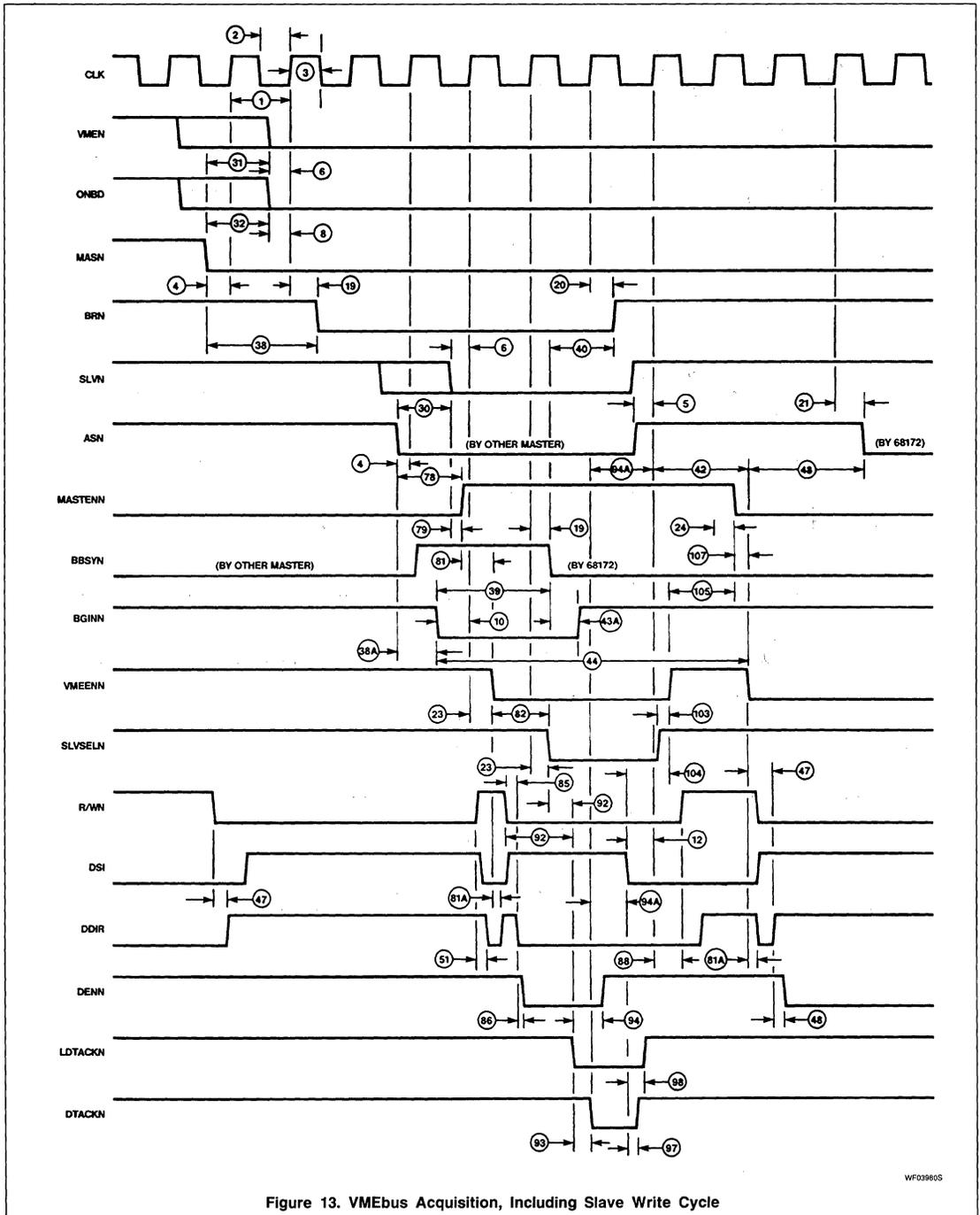
Figure 13. VMEbus Acquisition, Including Slave Write Cycle
