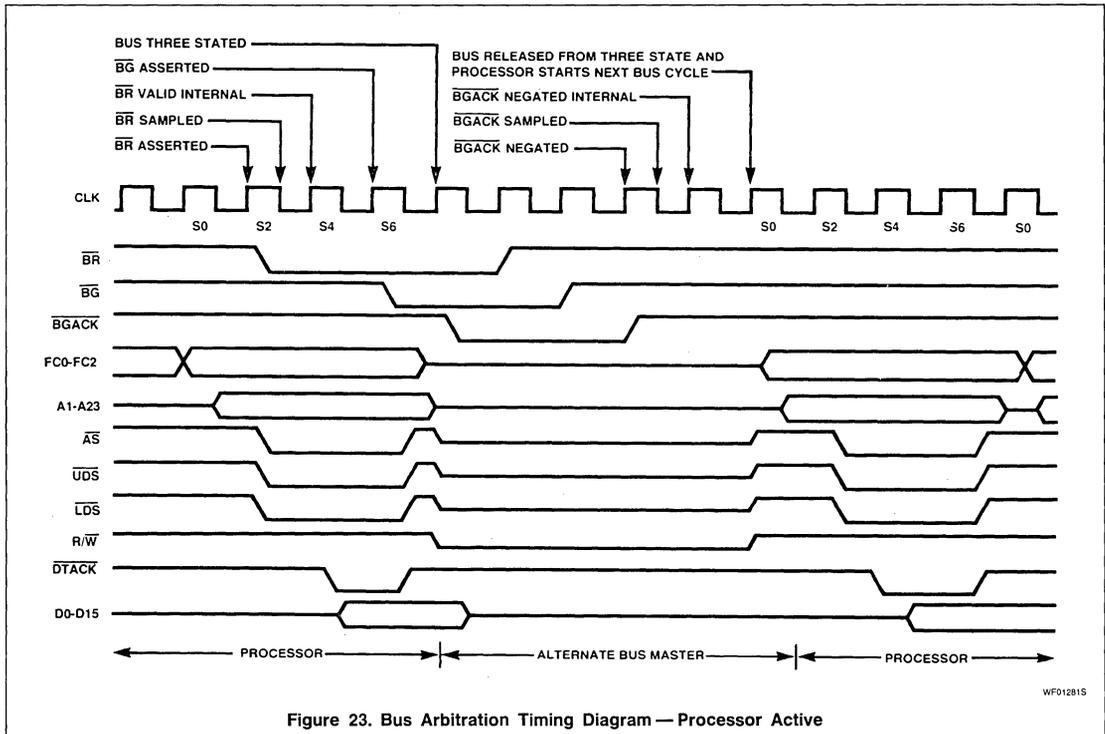
Figure 23. Bus Arbitration Timing Diagram — Processor Active
