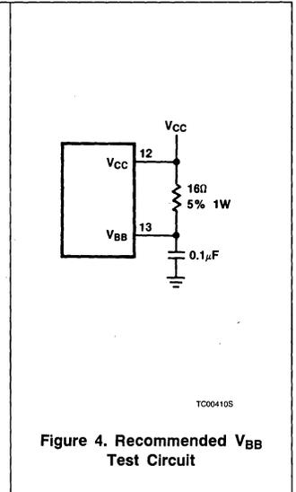
Figure 4. Recommended V<sub>BB</sub> Test Circuit
