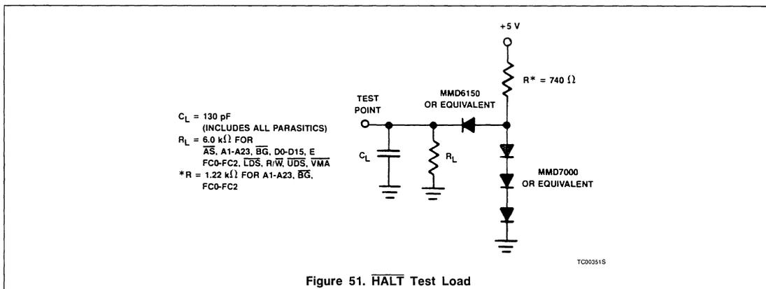
Figure 51. HALT Test Load
