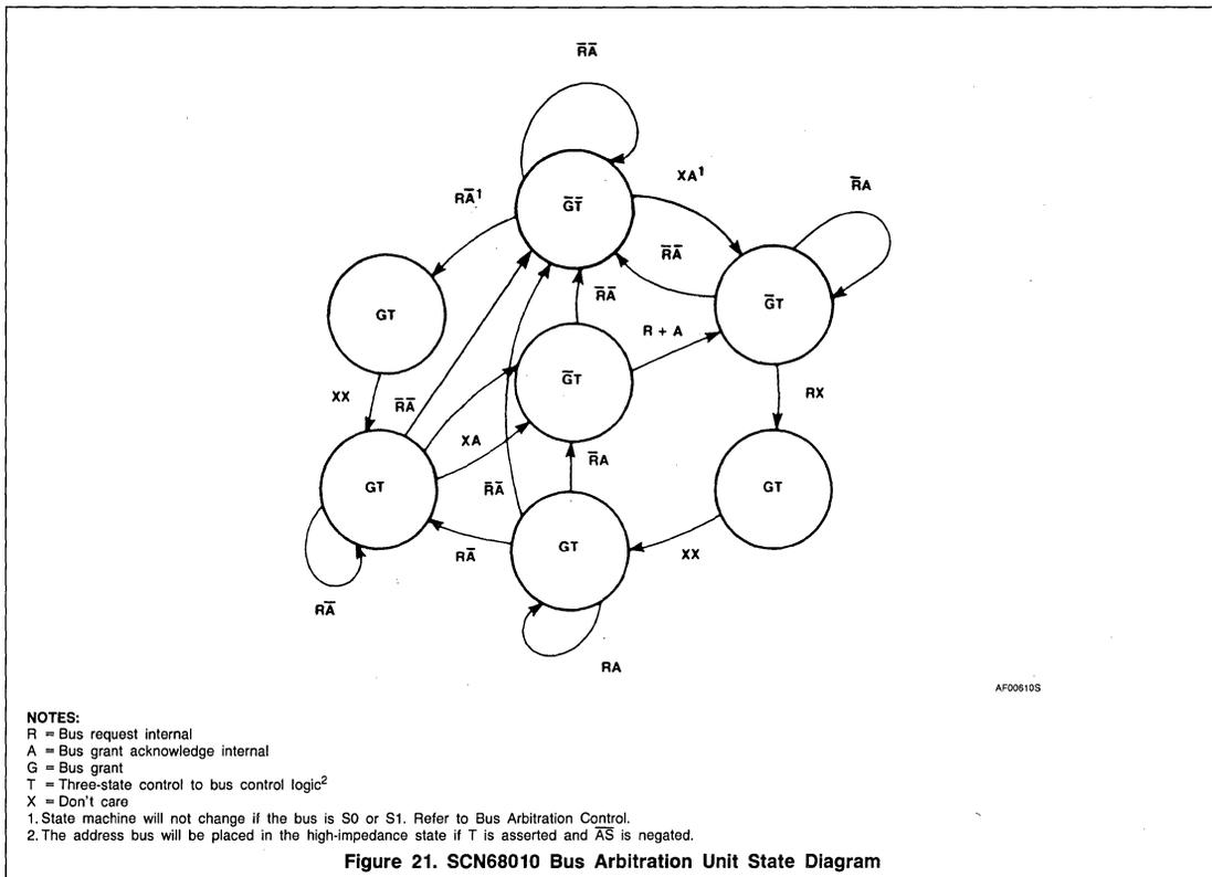
Figure 21. SCN68010 Bus Arbitration Unit State Diagram
