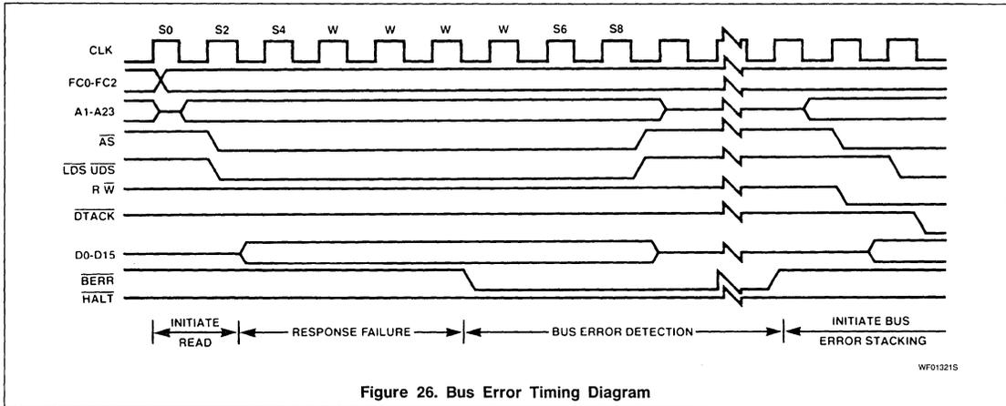
Figure 26. Bus Error Timing Diagram
