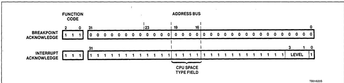
Figure 18. SCN68010 CPU-Space Address Encoding
