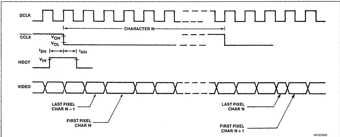
Figure 11. Half Dot Shift Timing
