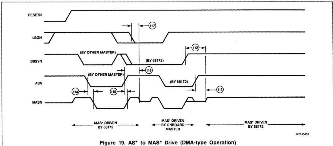
Figure 19. AS\* to MAS\* Drive (DMA-type Operation)
