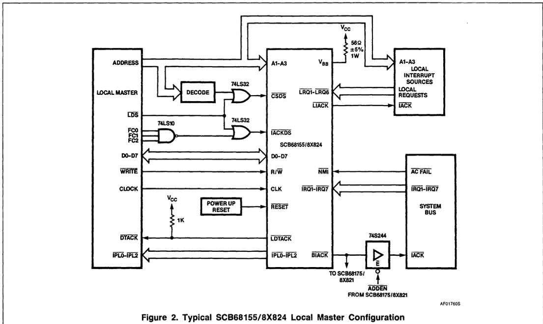
Figure 2. Typical SCB68155/8X824 Local Master Configuration
