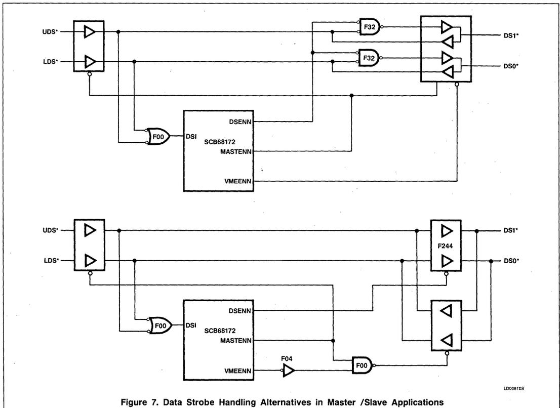
Figure 7. Data Strobe Handling Alternatives in Master /Slave Applications
