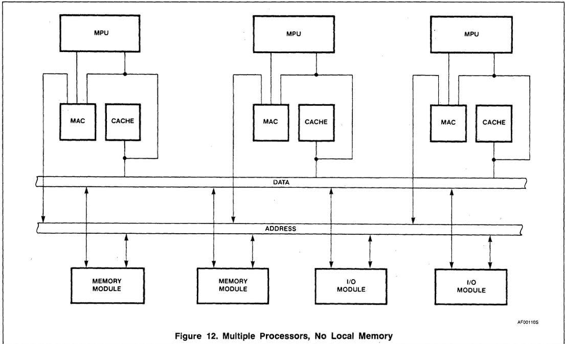
Figure 12. Multiple Processors, No Local Memory
