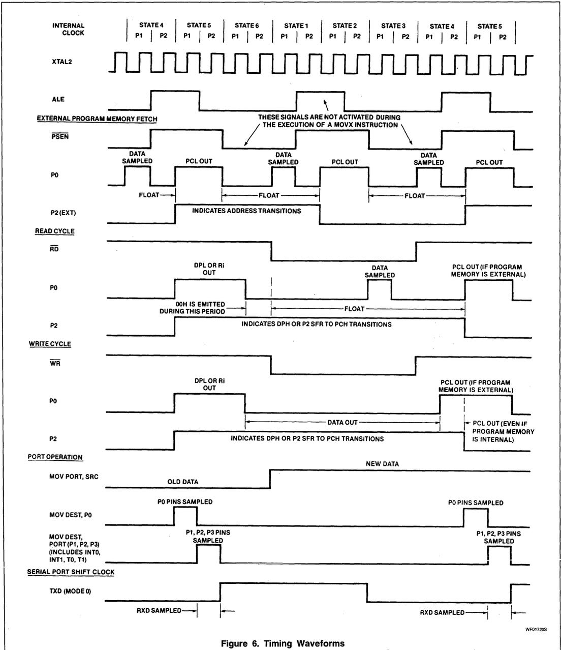
Figure 6. Timing Waveforms
