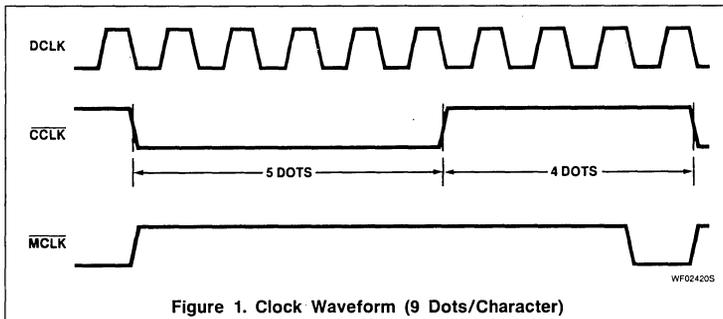
Figure 1. Clock Waveform (9 Dots/Character)
