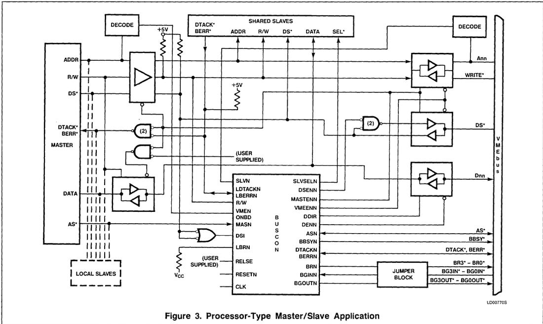
Figure 3. Processor-Type Master/Slave Application
