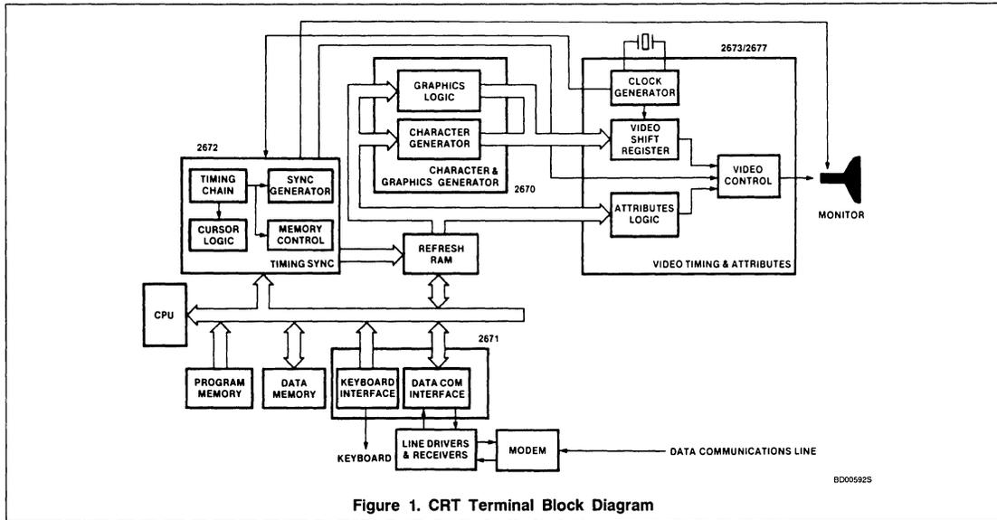
Figure 1. CRT Terminal Block Diagram
