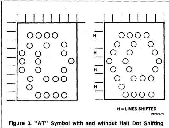
Figure 3. "AT" Symbol with and without Half Dot Shifting
