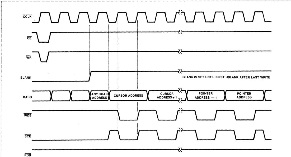
Figure 5. Write from Cursor to Pointer Command Timing
