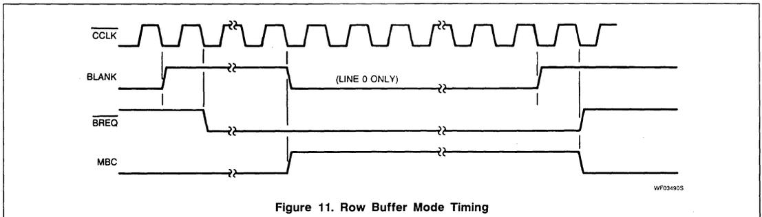
Figure 11. Row Buffer Mode Timing
