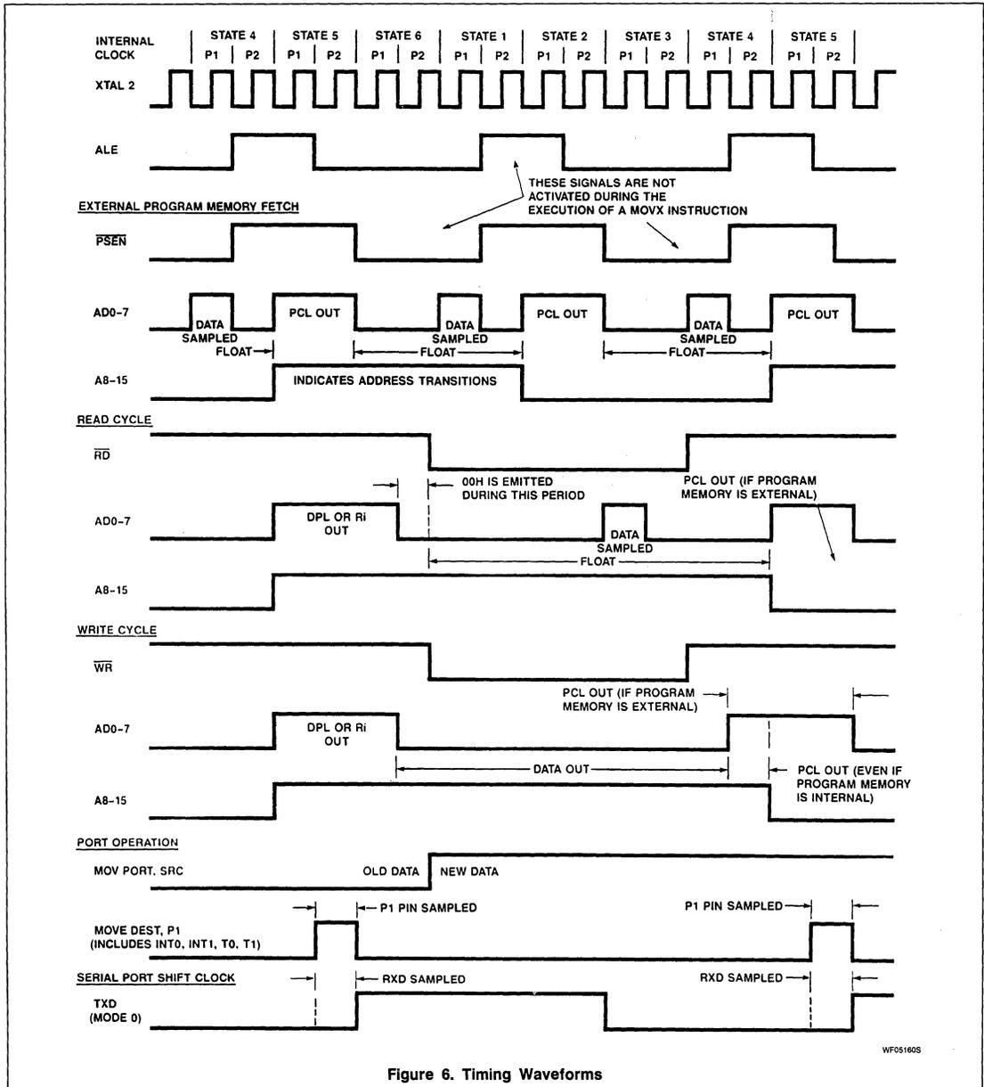
Figure 6. Timing Waveforms
