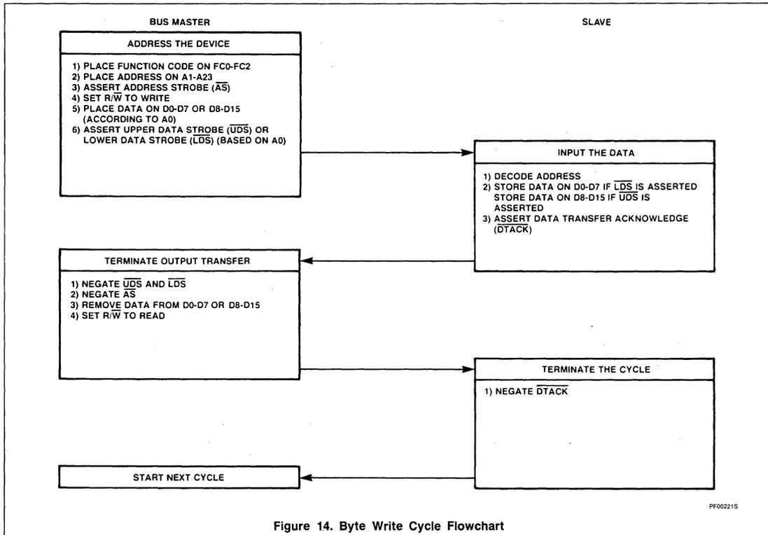
Figure 14. Byte Write Cycle Flowchart
