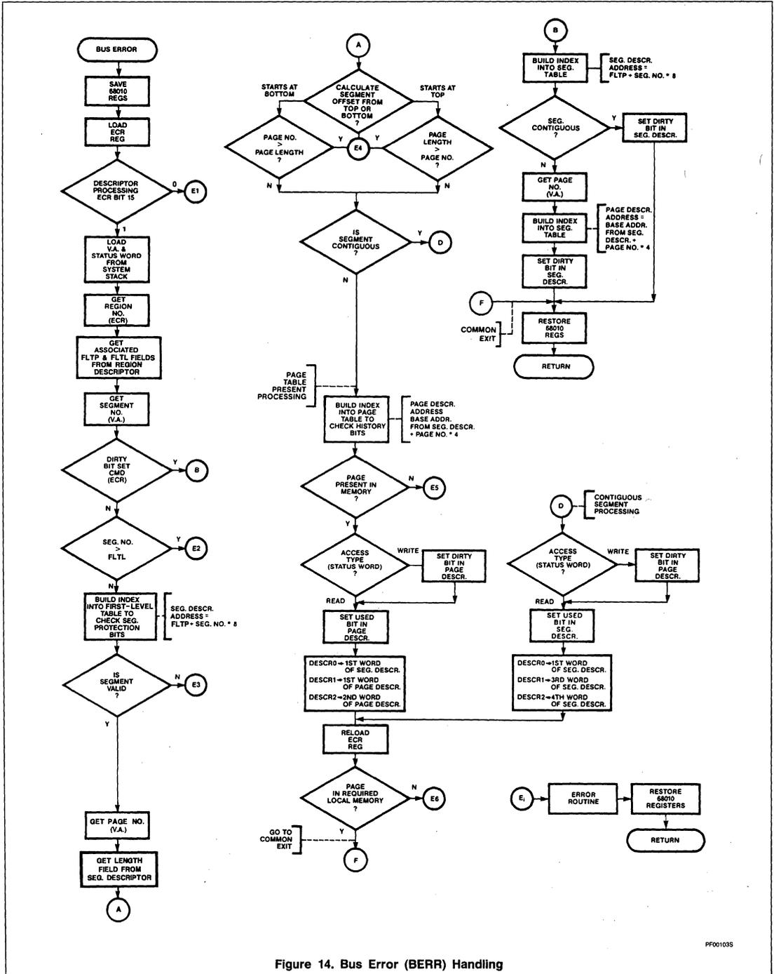
Figure 14. Bus Error (BERR) Handling
