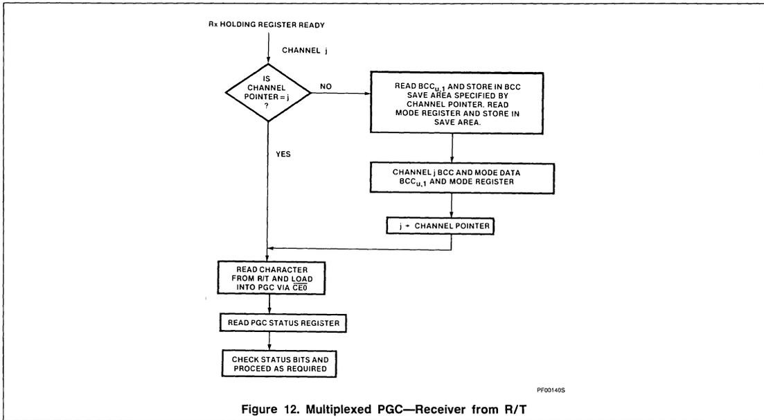
Figure 12. Multiplexed PGC—Receiver from R/T
