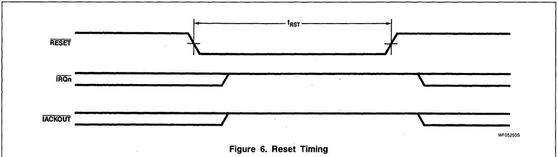
Figure 6. Reset Timing
