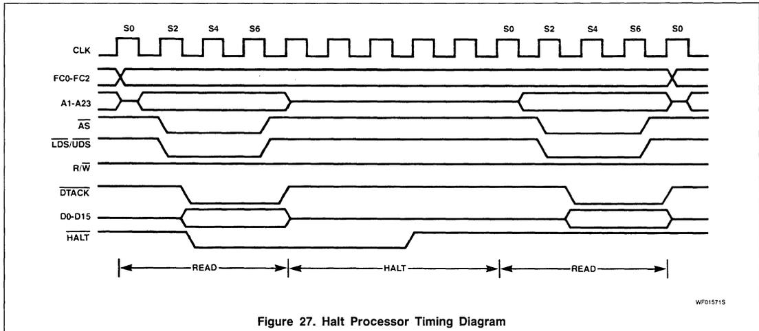
Figure 27. Halt Processor Timing Diagram
