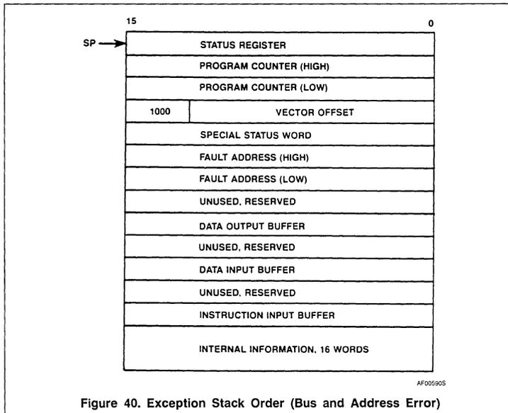
Word patterns with bits 12–15 equaling 1010 or 1111 are distinguished as unimplemented instructions and separate exception vectors are given to these patterns to permit efficient emulation. This facility allows the operating system to detect program errors, or to emulate unimplemented instructions, such as the 68881 floating-point coprocessor instructions, in software.
