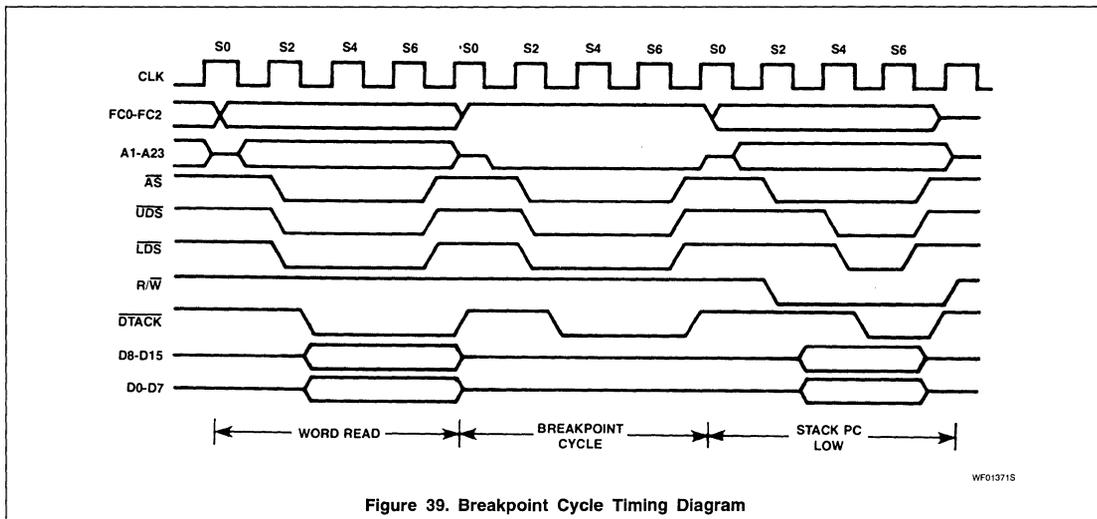
Figure 39. Breakpoint Cycle Timing Diagram
