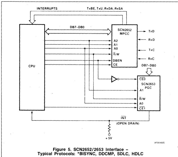
Figure 5. SCN2652/2653 Interface - Typical Protocols: \*BISYNC, DDCMP, SDLC, HDLC
