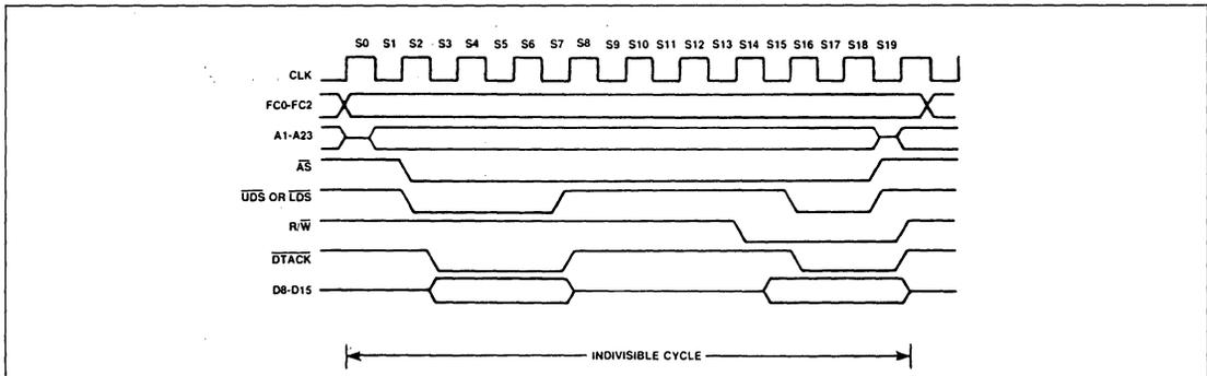
Figure 17. Read-Modify-Write Cycle Timing Diagram
