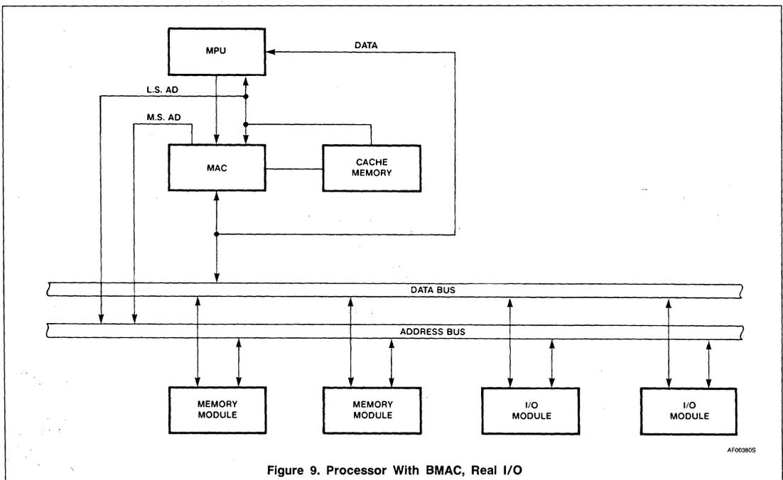
Figure 9. Processor With BMAC, Real I/O
