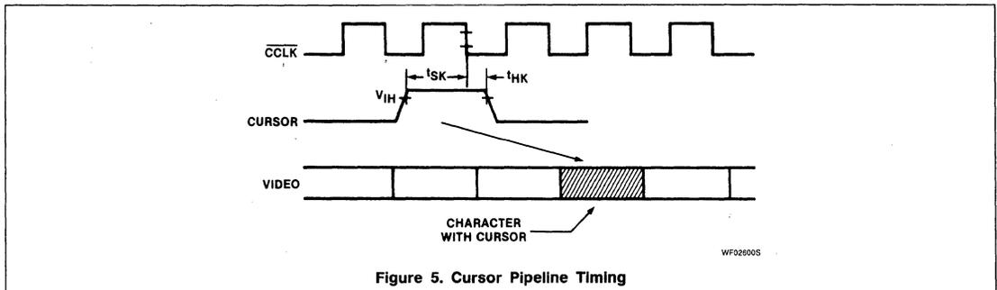
Figure 5. Cursor Pipeline Timing
