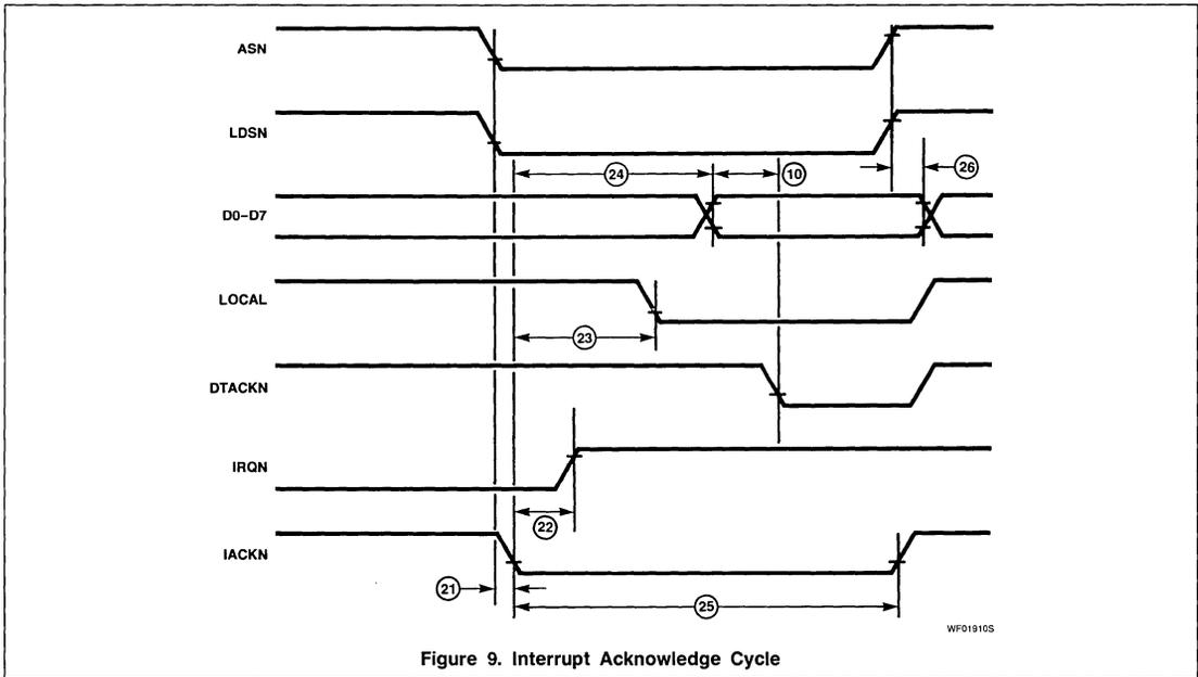
Figure 9. Interrupt Acknowledge Cycle
