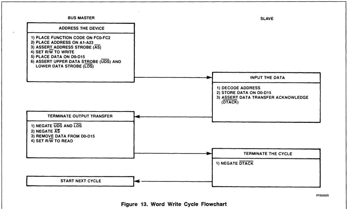
Figure 13. Word Write Cycle Flowchart
