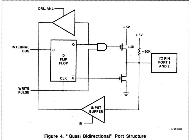
Figure 4. "Quasi Bidirectional" Port Structure
