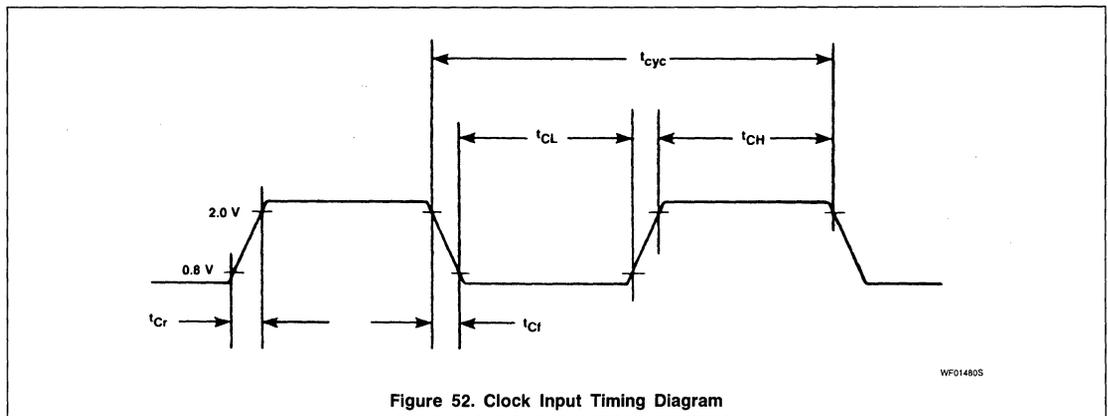
Figure 52. Clock Input Timing Diagram
