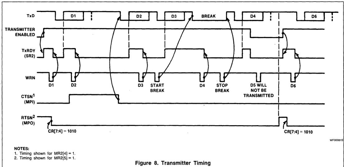
Figure 8. Transmitter Timing
