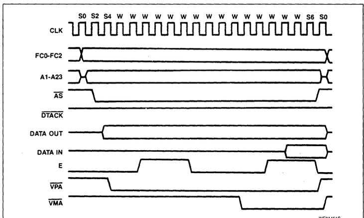
Figure 40. SCN68000 to Synchronous Peripheral Timing—Worst Case
