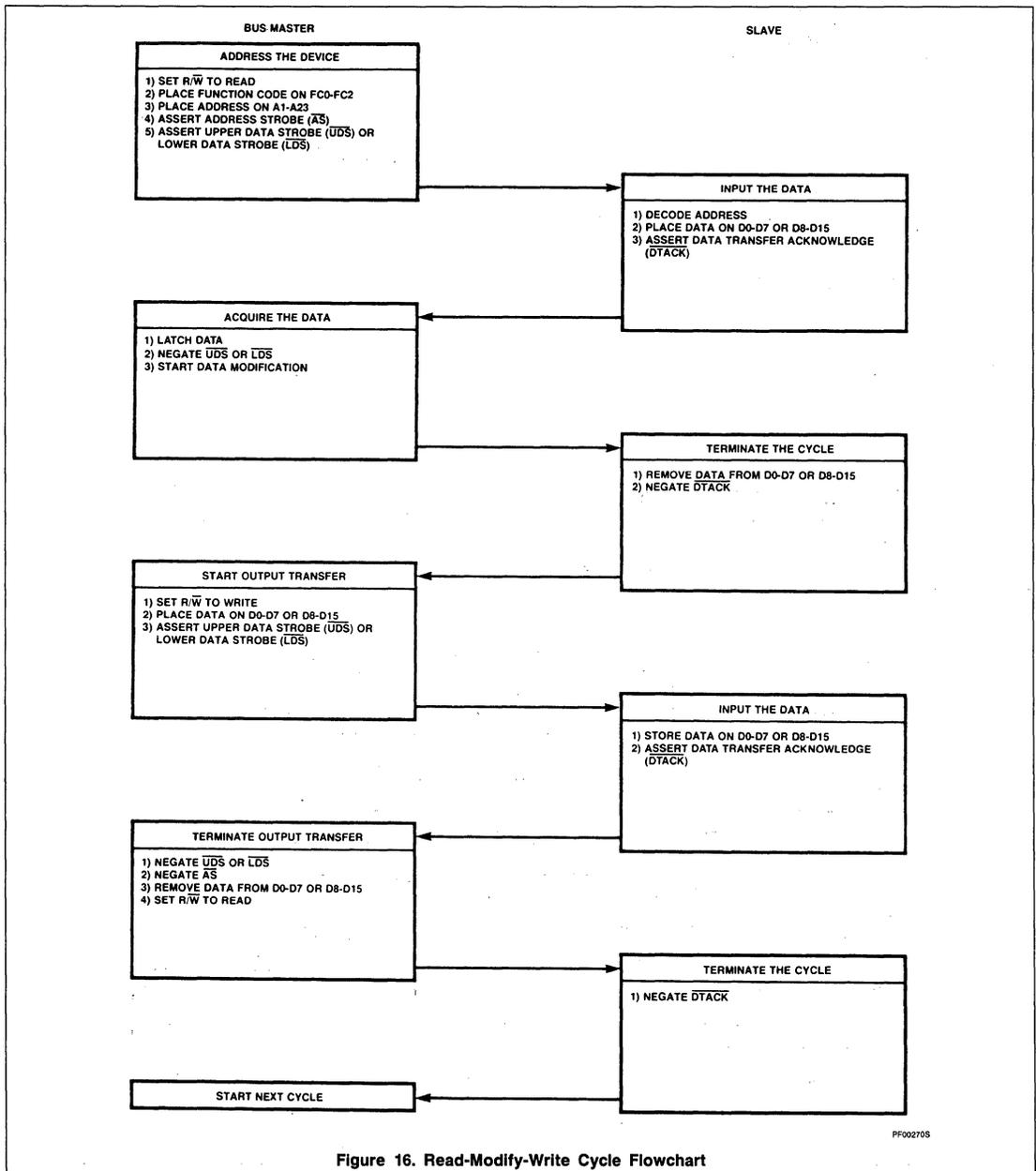
Figure 16. Read-Modify-Write Cycle Flowchart
