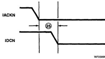
Figure 22. Interrupt Daisy Chain Timing
