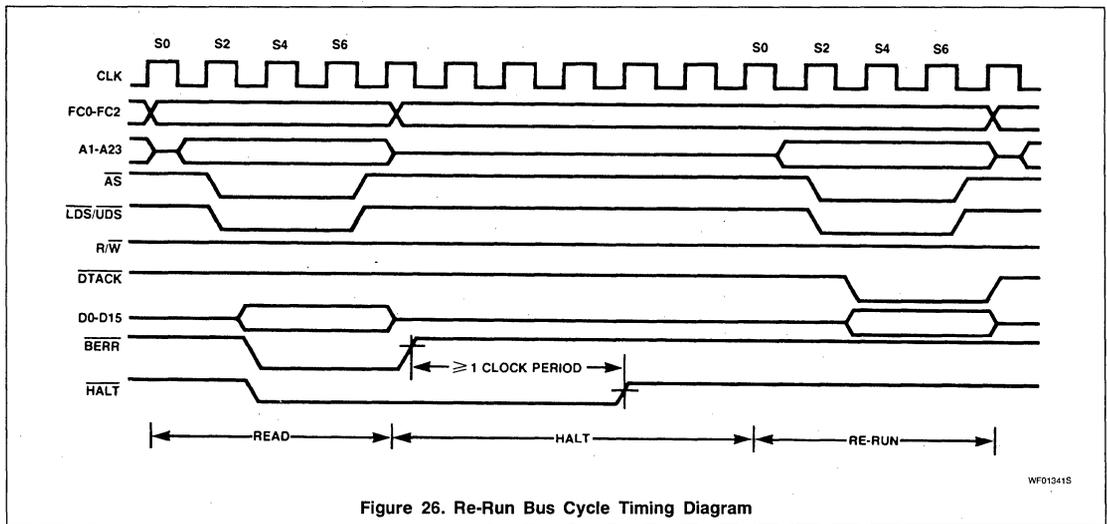
Figure 26. Re-Run Bus Cycle Timing Diagram
