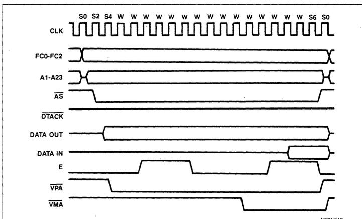
Figure 45. SCN68010 to Synchronous Peripheral Timing Diagram — Worst Case
