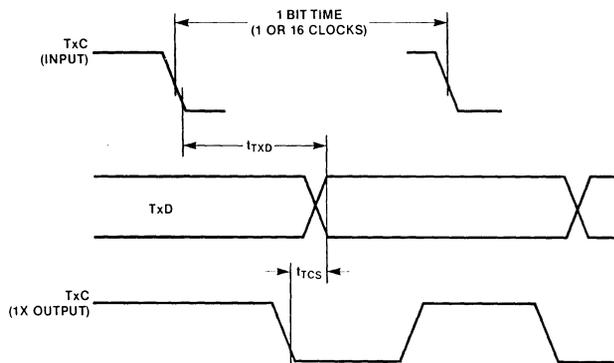
Figure 8. Transmit Timing
