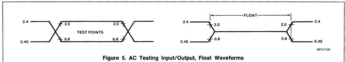
Figure 5. AC Testing Input/Output, Float Waveforms
