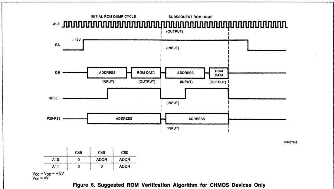
Figure 6. Suggested ROM Verification Algorithm for CHMOS Devices Only
