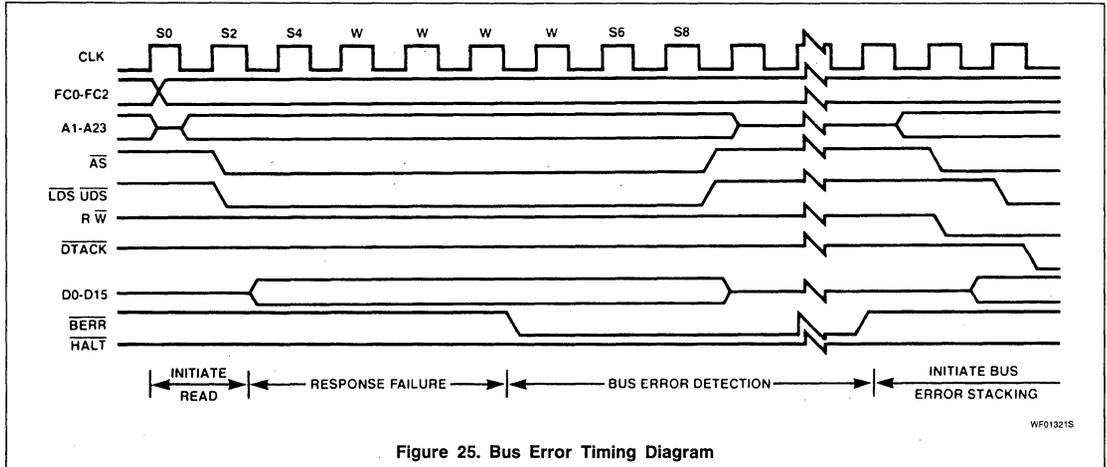
Figure 25. Bus Error Timing Diagram
