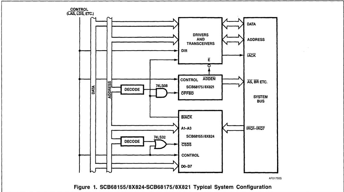
Figure 1. SCB68155/8X824-SCB68175/8X821 Typical System Configuration
