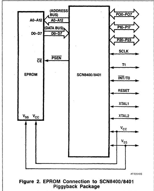
Figure 2. EPROM Connection to SCN8400/8401 Piggyback Package
