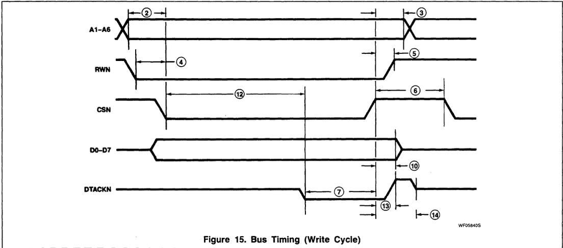
Figure 15. Bus Timing (Write Cycle)
