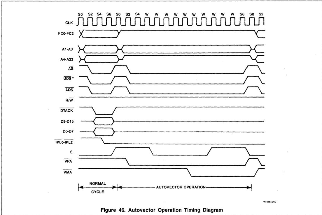
Figure 46. Autovector Operation Timing Diagram
