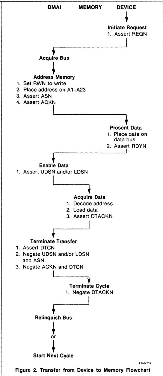
Figure 2. Transfer from Device to Memory Flowchart
