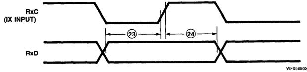
Figure 21. Receive Timing
