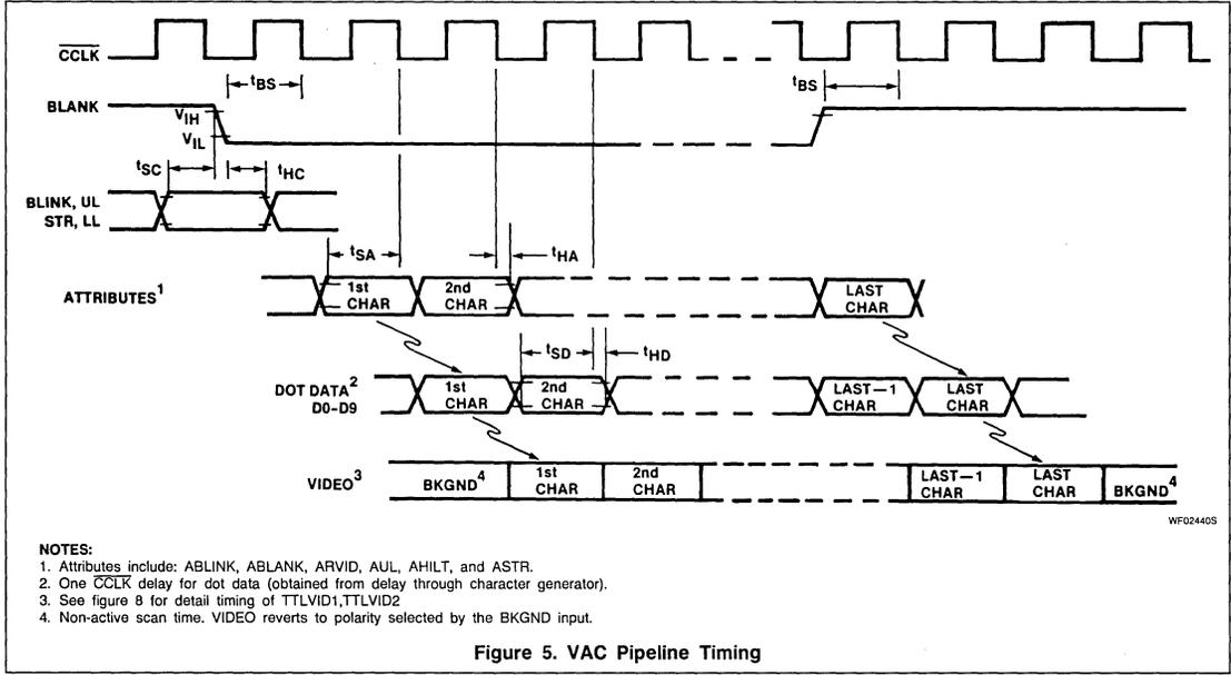
Figure 5. VAC Pipeline Timing
