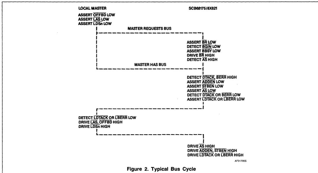
control of the host bus may only be transferred while  $\overline{AS}$  is high. The SCB68175/8X821 will cycle  $\overline{STBEN}$  as required for a read-modify-write cycle.
