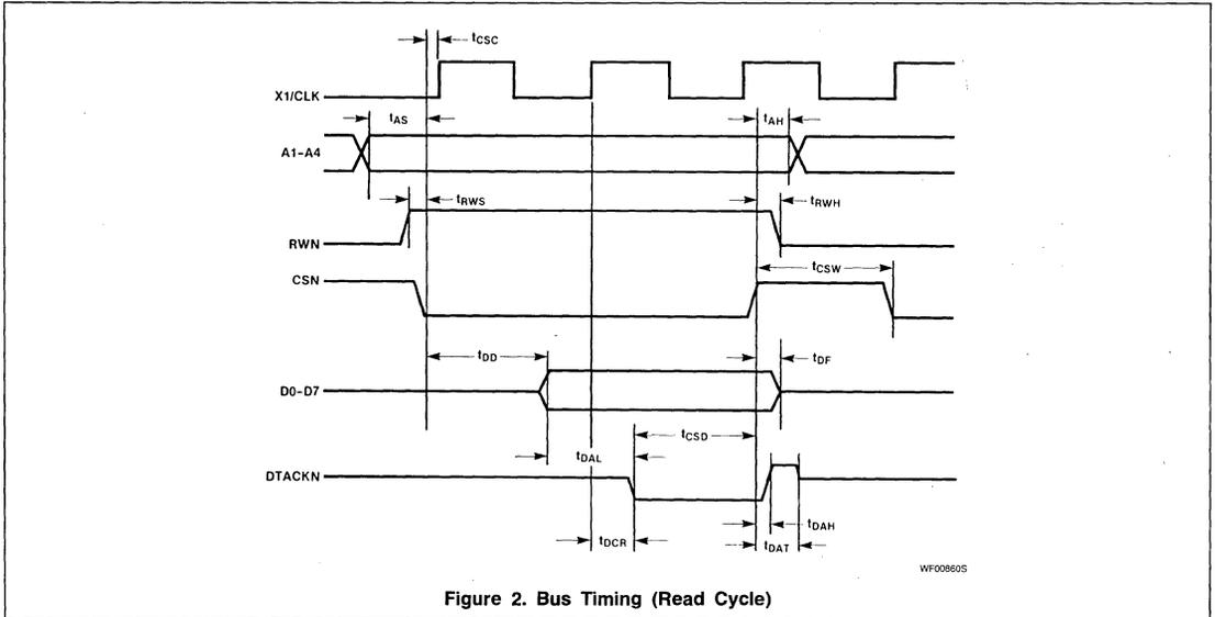
Figure 2. Bus Timing (Read Cycle)
