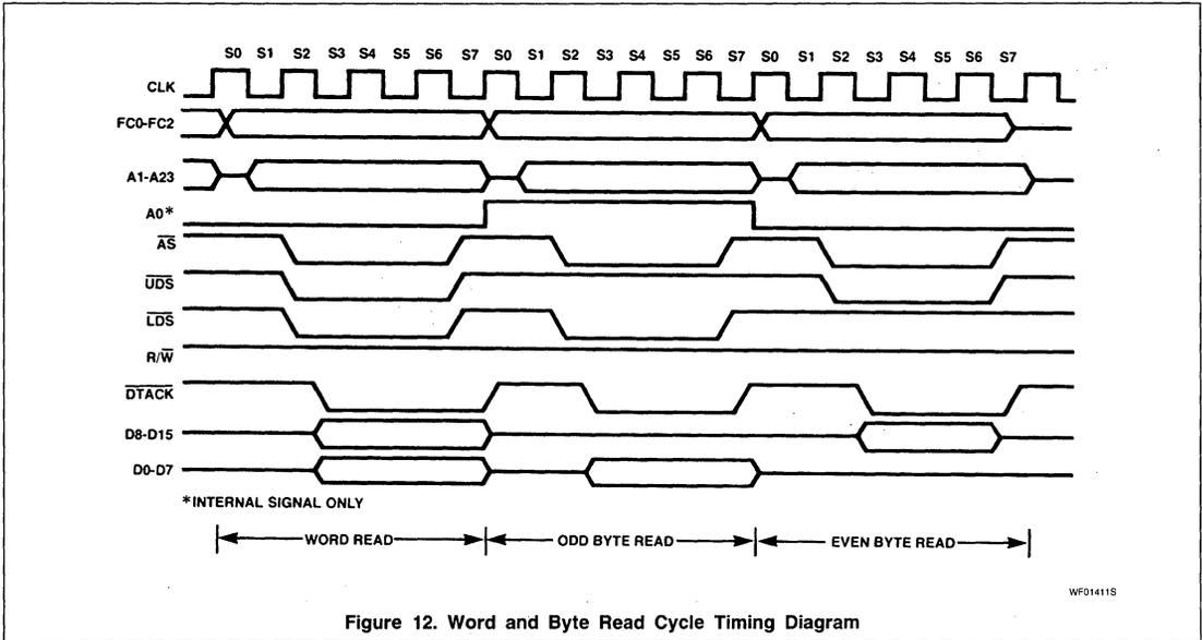
Figure 12. Word and Byte Read Cycle Timing Diagram
