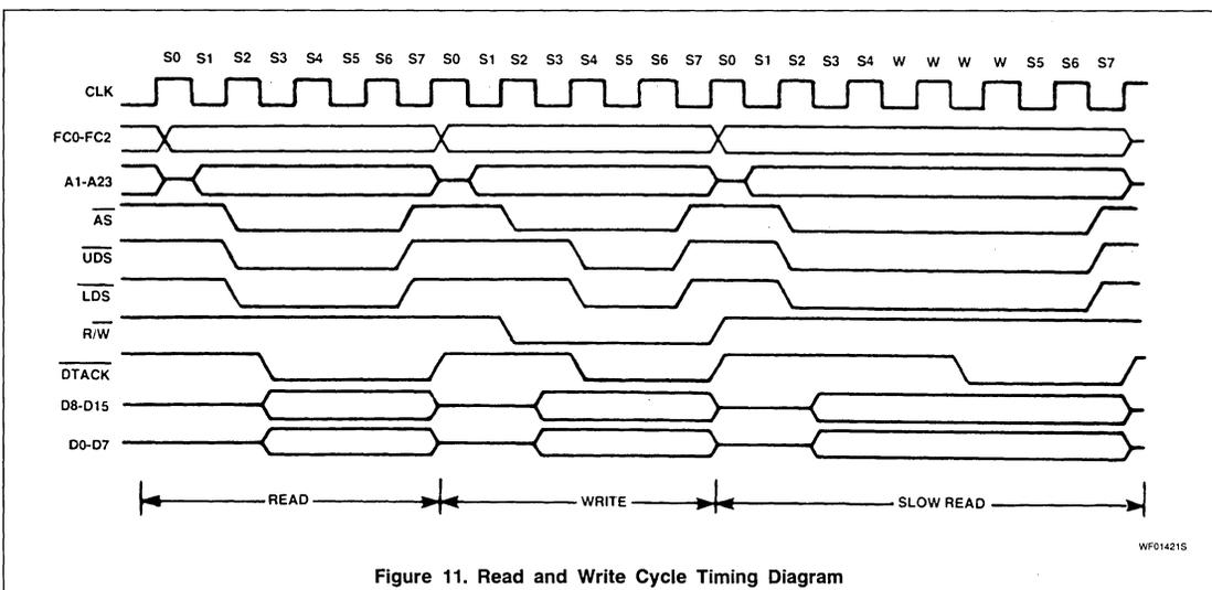
Figure 11. Read and Write Cycle Timing Diagram
