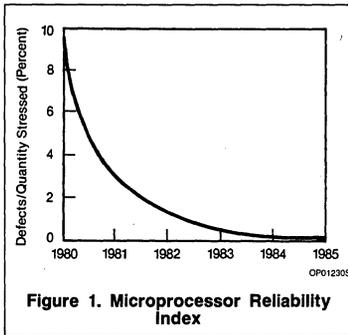
Figure 1 shows the relative improvement in Sure III performance for the Microprocessor Division for the past five years. This curve combines all the stress tests and plots the overall percentage defective by year. Clearly, the reliability of our product line is improving, and more importantly, it is consistent and predictable.
