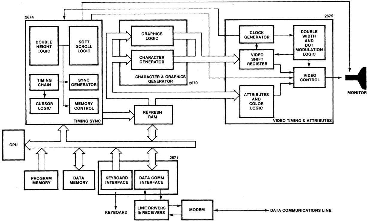
Figure 1. CRT Terminal Block Diagram
