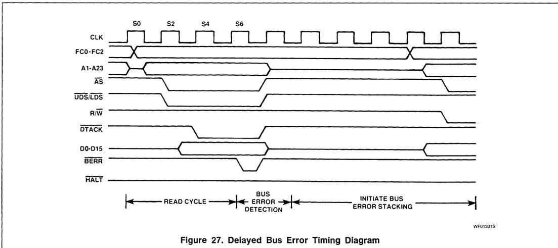
Figure 27. Delayed Bus Error Timing Diagram
