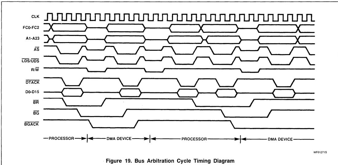
Figure 19. Bus Arbitration Cycle Timing Diagram
