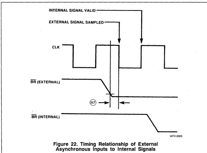
Figure 22. Timing Relationship of External Asynchronous Inputs to Internal Signals
