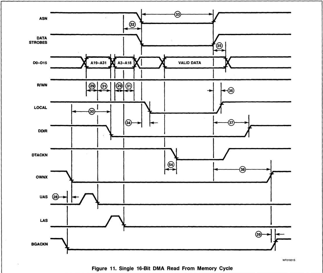
Figure 11. Single 16-Bit DMA Read From Memory Cycle
