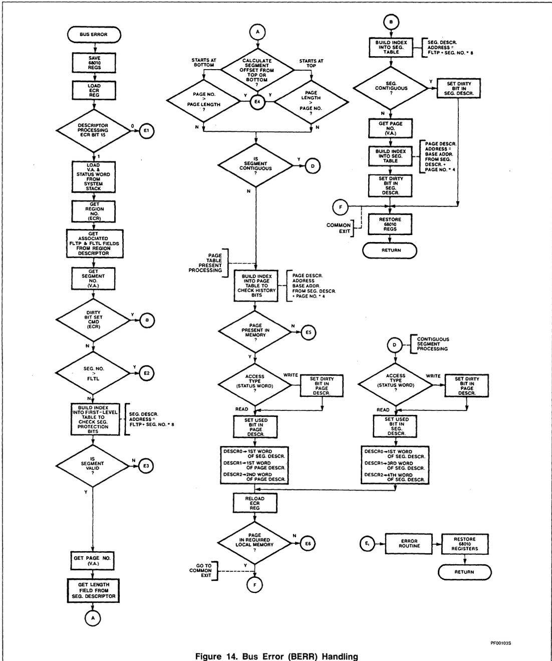
Figure 14. Bus Error (BERR) Handling
