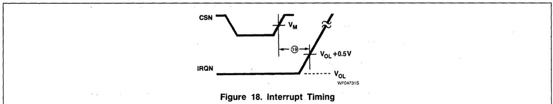
Figure 18. Interrupt Timing
