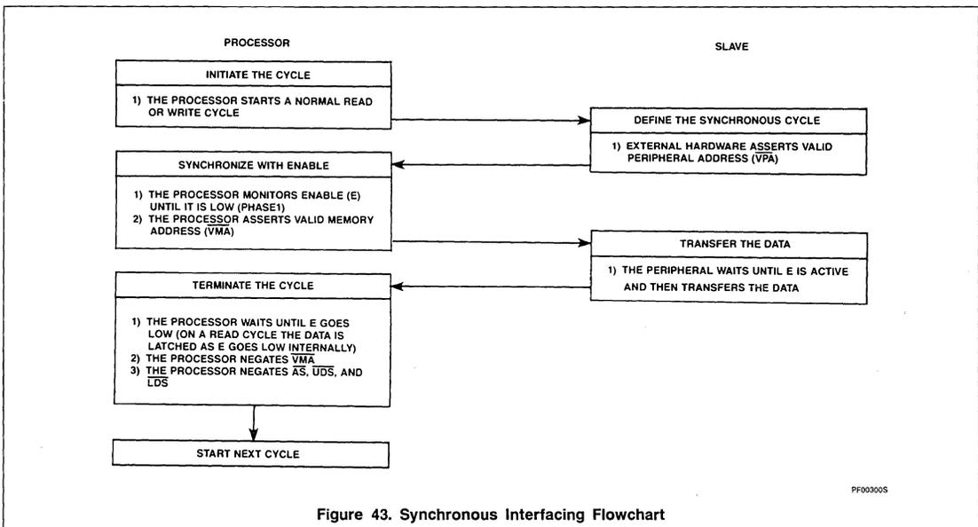
Figure 43. Synchronous Interfacing Flowchart
