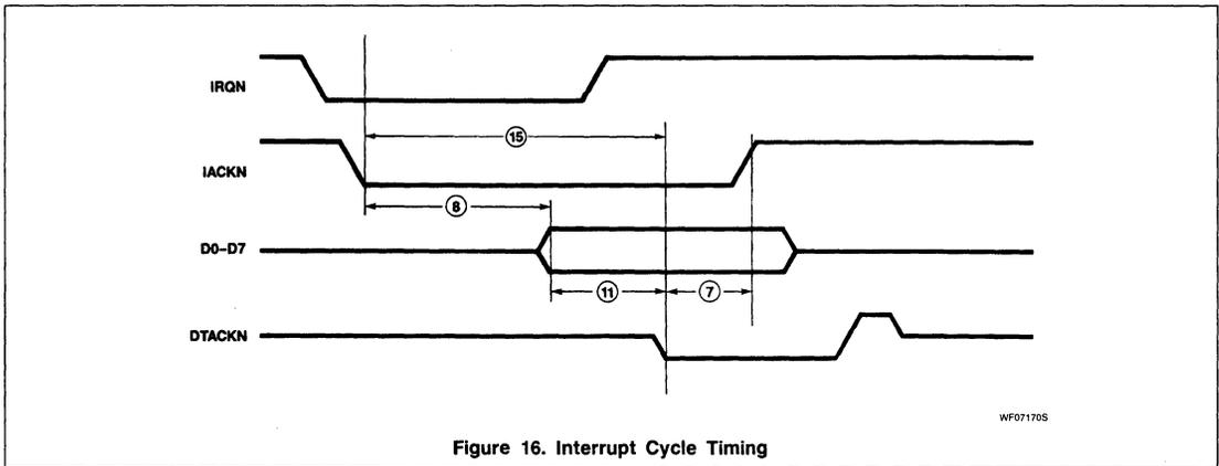
Figure 16. Interrupt Cycle Timing
