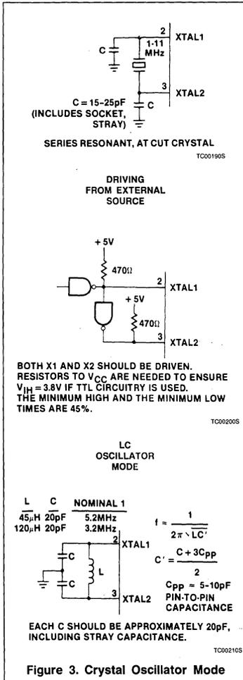
Figure 3. Crystal Oscillator Mode
