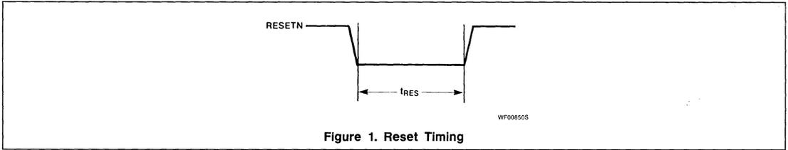
Figure 1. Reset Timing
