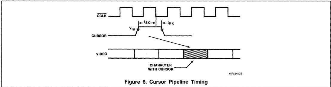
Figure 6. Cursor Pipeline Timing
