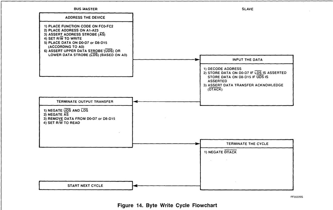
Figure 14. Byte Write Cycle Flowchart
