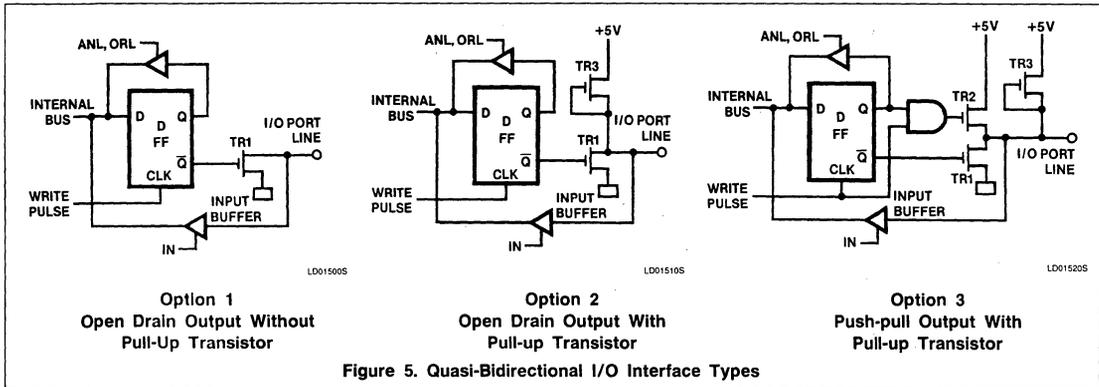
Figure 5. Quasi-Bidirectional I/O Interface Types
