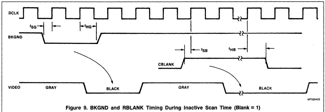
Figure 9. BKGND and RBLANK Timing During Inactive Scan Time (Blank = 1)
