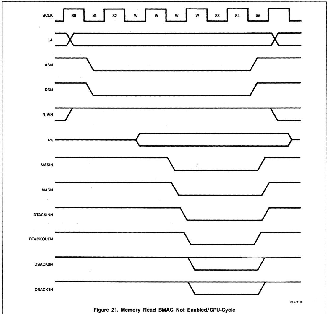
Figure 21. Memory Read BMAC Not Enabled/CPU-Cycle
