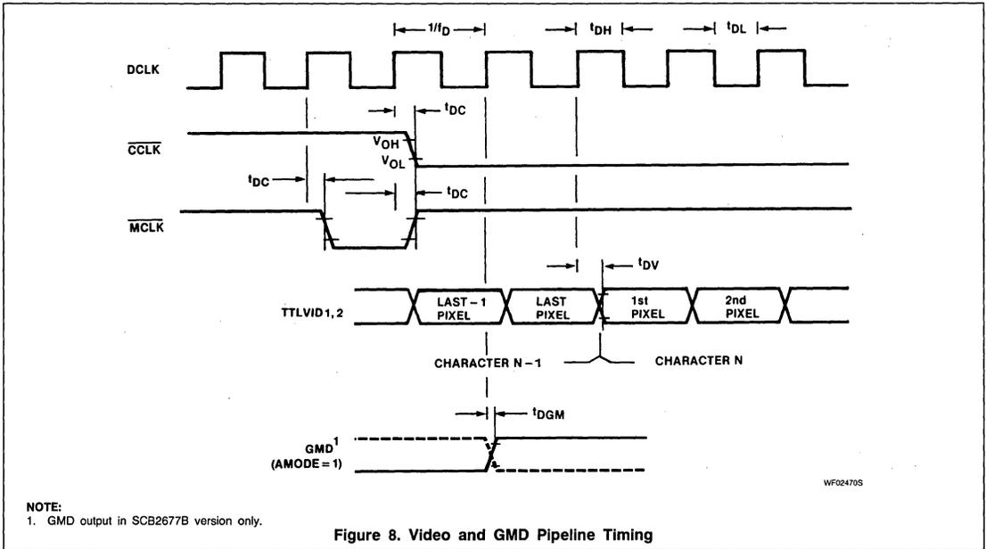
Figure 8. Video and GMD Pipeline Timing
