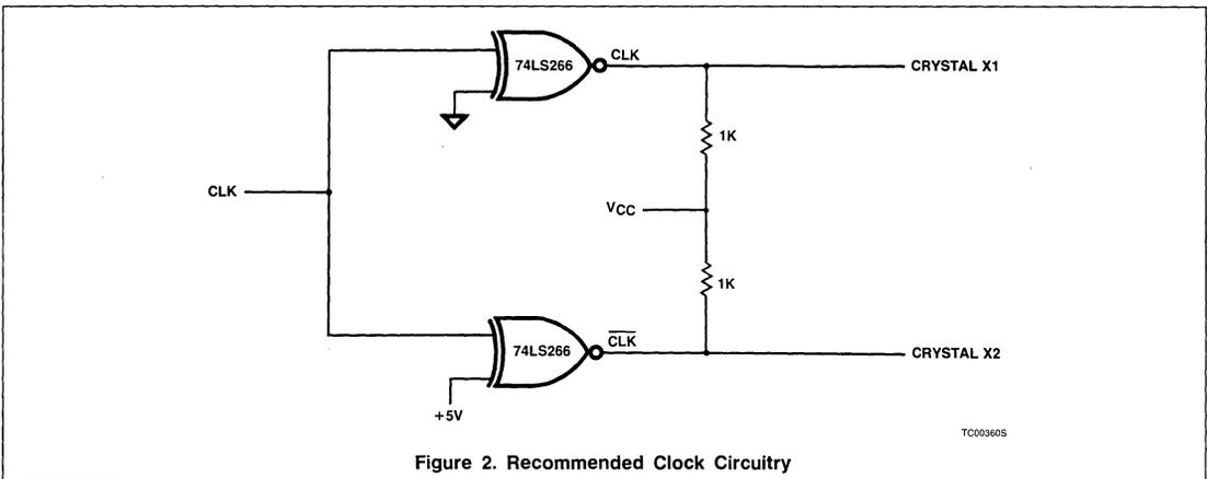
Figure 2. Recommended Clock Circuitry
