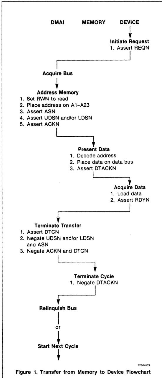
Figure 1. Transfer from Memory to Device Flowchart
