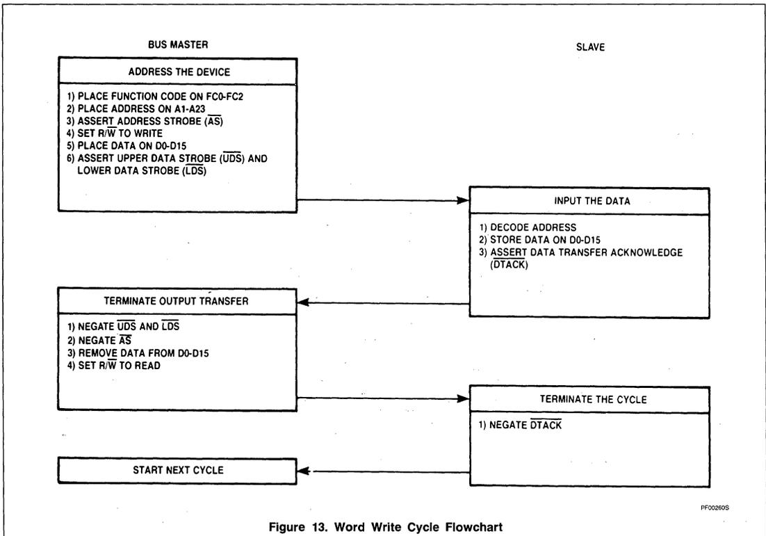
Figure 13. Word Write Cycle Flowchart
