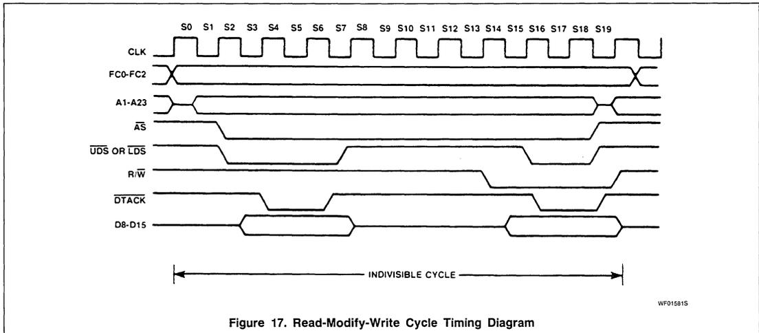
Figure 17. Read-Modify-Write Cycle Timing Diagram
