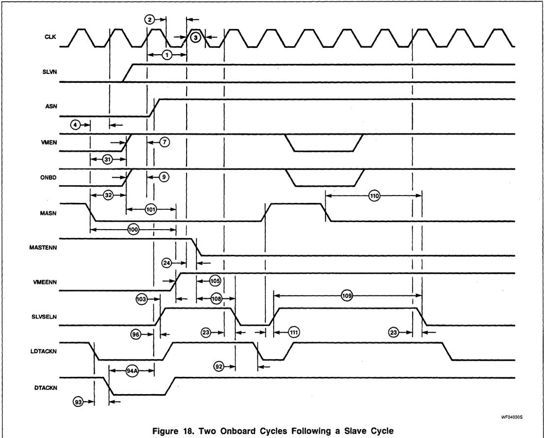
Figure 18. Two Onboard Cycles Following a Slave Cycle
