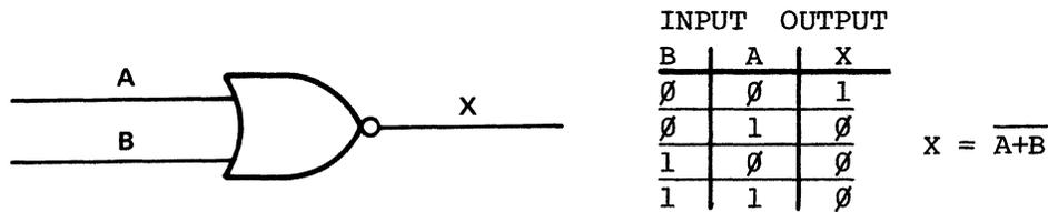
Figure 2.15 SYMBOL AND TRUTH TABLE FOR NOR GATE
