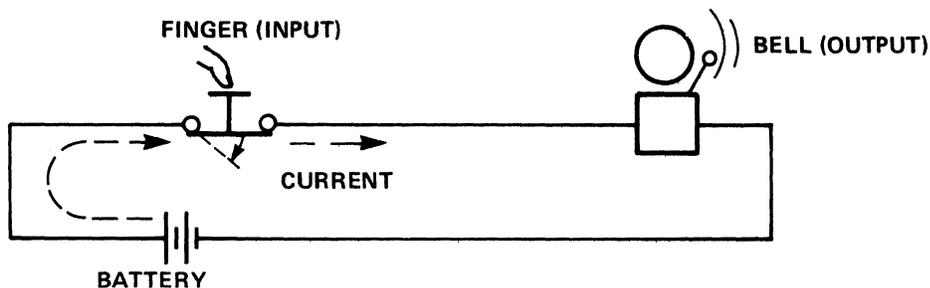
Figure 2.2 ALARM CIRCUIT
