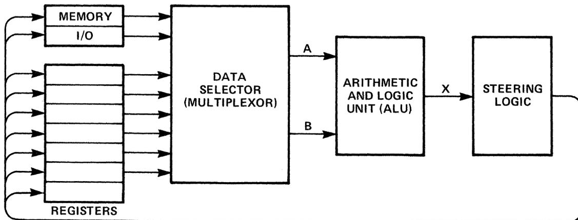
Figure 4.3 ARITHMETIC AND LOGIC SYSTEM BLOCK DIAGRAM
