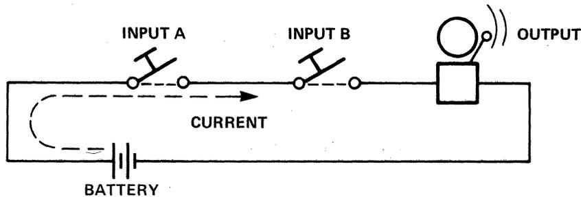
Figure 2.5 AND CIRCUIT
