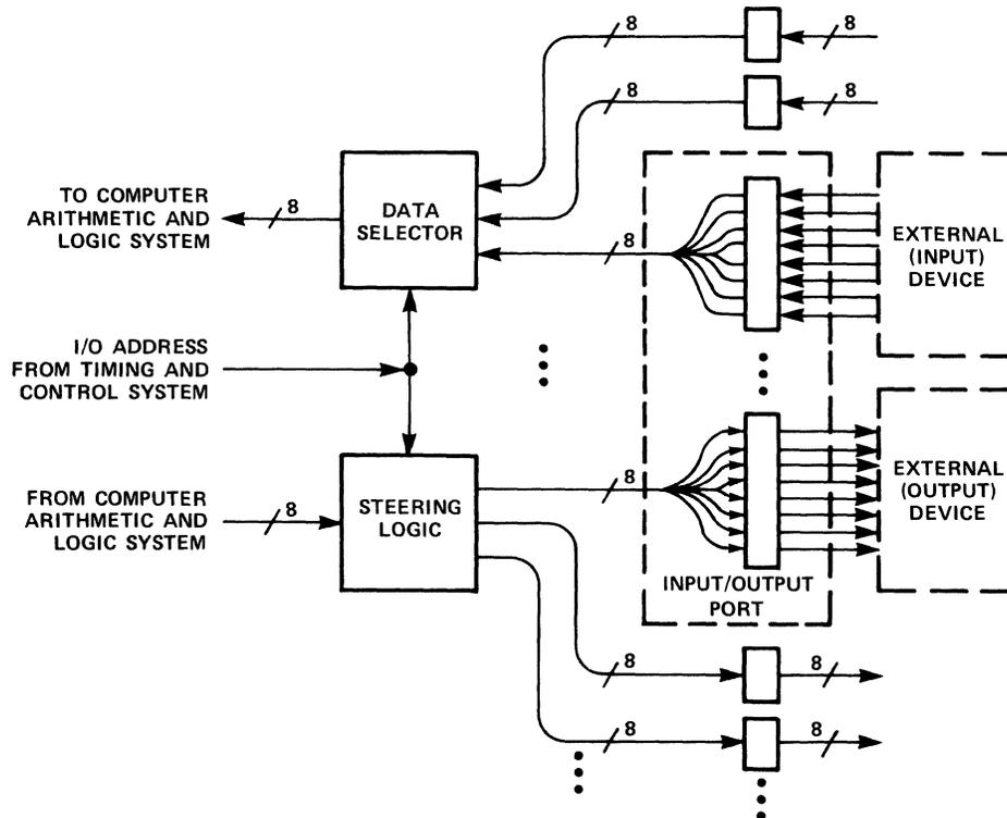
Figure 4.5 INPUT/OUTPUT SYSTEM
