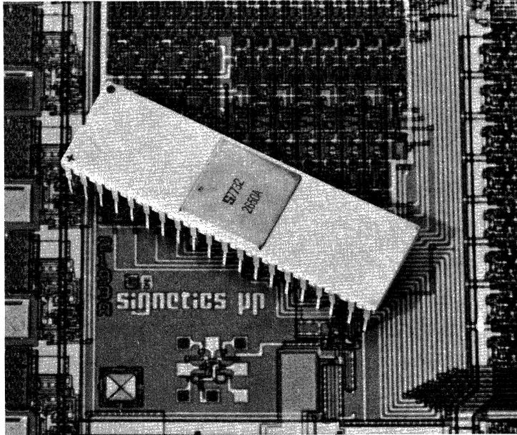
Figure 1.1 THE 2650 MICROPROCESSOR
