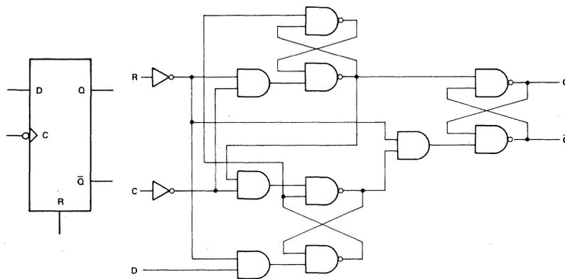
Figure 2.16 LOGIC SYMBOL AND SCHEMATIC FOR D-TYPE FLIP/FLOP
