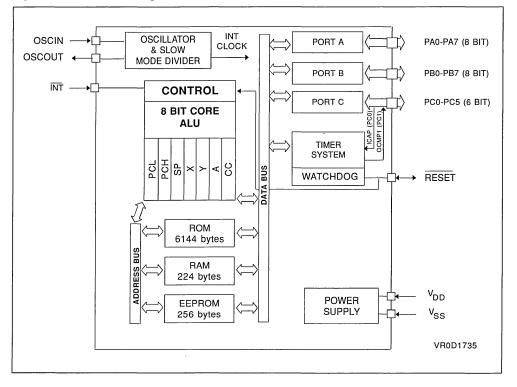
Figure 1. ST7294 Block Diagram
