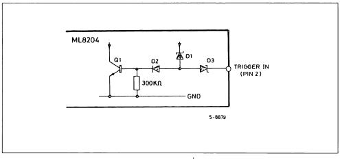
Figure 5a : Enabling Oscillation of the ML8204 for Supply Voltages less than V<sub>s1</sub>.
