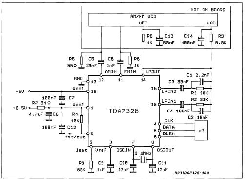
\*) C7 must be connected as closed as possible between pin 10 and pin 13
