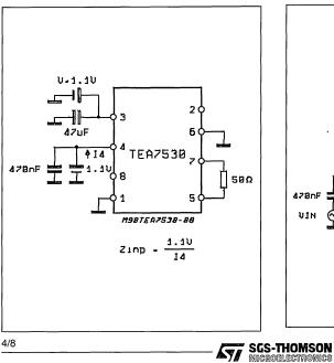
Figure 8: Anti-loading Feedback System at G = GATT
