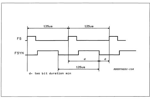
Figure 11: FSYN in comparison with FS when FSYN is different from FS.
