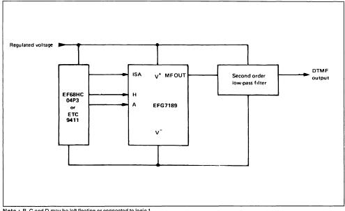
Note : B, C and D may be left floating or connected to logic 1.
