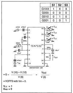
Figure 10 : Antiacoustic Feedback System at G011.
