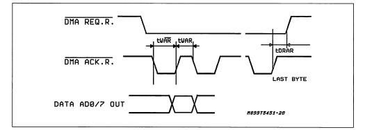
Figure 20: DMA frame transmission timing
