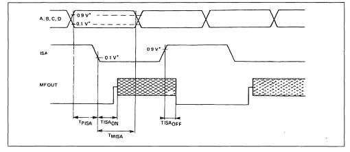
Figure 7 : Serial Operating Mode.
