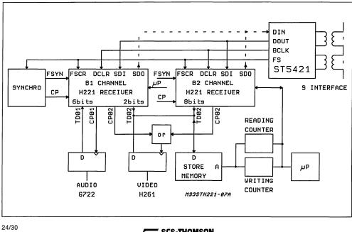
**SGS-THOMSON** MICROELECTRONICS Figure 8: Application Interface Configuration can change every 20ms.
