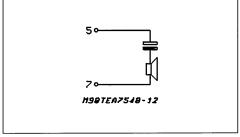
Two loudspeaker connection methods are possible, using the amplifier in either symmetrical or asymmetrical mode.
