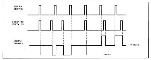
Figure 10: Simplified schematic of PFD outputs.
