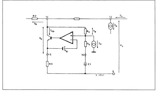
Figure 6 : Circuit Configuration of the Shunt Regulator.
