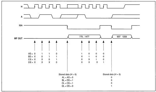
Notes: 1. With ISA at logic 0, H, A, B, C and D signals cannot modify the generated DTMF pair. As a result, in serial operating mode, it is possible to enter AS, BS, CS and DS data while another DTMF pair is being generated.
