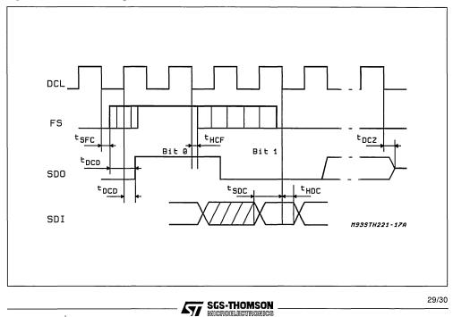
Figure 17: Application Side Signals.
