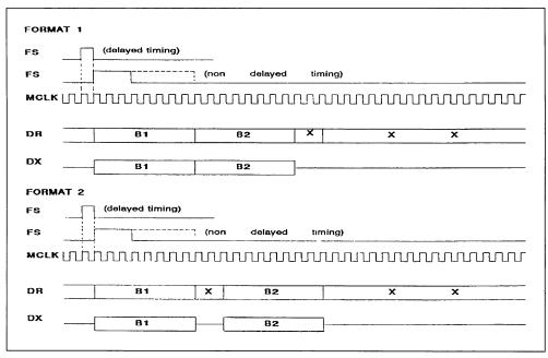
Figure 2: GCI Interface Frame Structure
