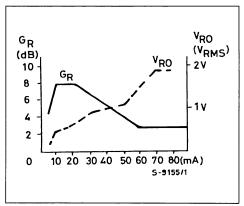
Figure 6 : DC Characteristic Measured between Line and GND.
