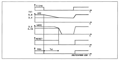
TD is fixed by the VMC value, C10 on VMC, and the ST6 current consumption. Example:  $V_{MC} = 5V$ ,  $C_{10} = 470\mu$ F,  $I_{ST6+ TEA7090} =$   $450\mu A \Rightarrow T_D$  = 1.67s by this way the TEA7090+ ST6 drive a long ground key duration.
