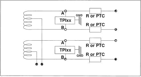
This component use an internal diagram which allows to have symetrical characteristics with a good balanced behaviour.
