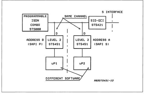
Figure 7: LAPB and LAPD protocol on the same D channel handlended with 2 different µPs
