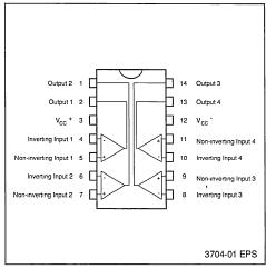
The TS3704 is a micropower CMOS quad voltage comparator with extremely low consumption of  $9\mu$ A typ / comparator (20 times less than bipolar LM339). The push-pull CMOS output stage allows power and space saving by eliminating the external pull-up resistor required by usual open-collector output comparators.
