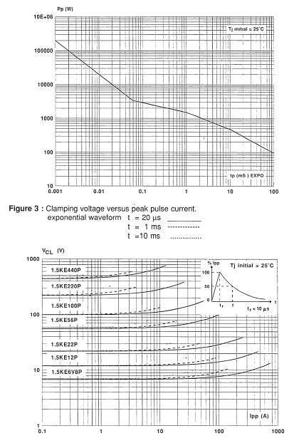
Figure 2 : Peak pulse power versus exponential pulse duration.
