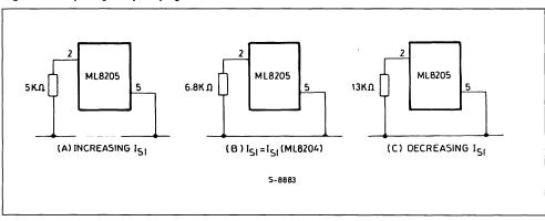
Figure 8 : Adjusting  $I_{si}$  by Varying  $R_{SL}$ .
