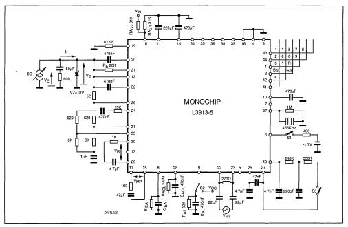
Figure 6: DTMF Distortion French Specification.
