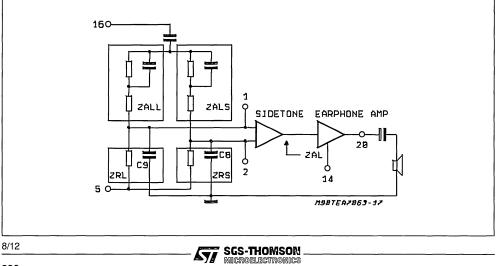
In this condition an internal connection is activated from line DTMF output (pin 16) to Receive Output (pin 20) with an attenuation GRS = 38.5dB to provide acoustic feedback of the DTMF emission.
