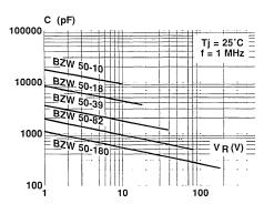
C (pF) 100000 Tj = 25°C f = 1 MHz BZW 50-10B 10000 BZW 50-18B Ξ. BZW 50-39B BZW 50-82B 1000 BZW 50-180B VR(V) 100 10 100 1
