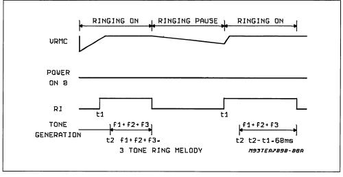
During the delay t2-t1, the microcontroller can analyse the line ring frequency and then sends to the serial data input the code corresponding to the chosen ringing output level.
