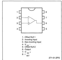
The TS271 is a low cost, low power single operational amplifier designed to operate with single or dual supplies. This operational amplifier uses the SGS-THOMSON silicon gate LIN MOS process giving it an excellent consumption-speed ratio. This amplifier is ideally suited for low consumption applications.
