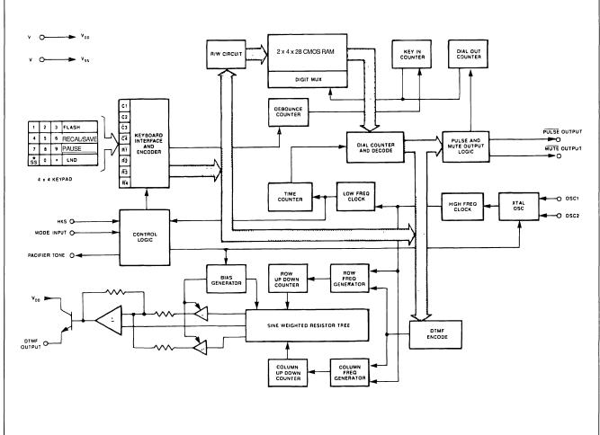
Figure 3 : MK53732 Block Diagram.
