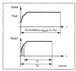
Pin reset: It is the power on reset output.
