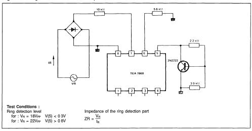
Figure 3 : Ring Detection Level and Impedance.
