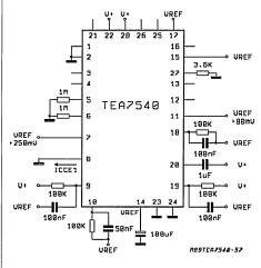
$V^+$  = 3V pin 7 is forced to transmit mode pin 11 is forced to maximum gain
