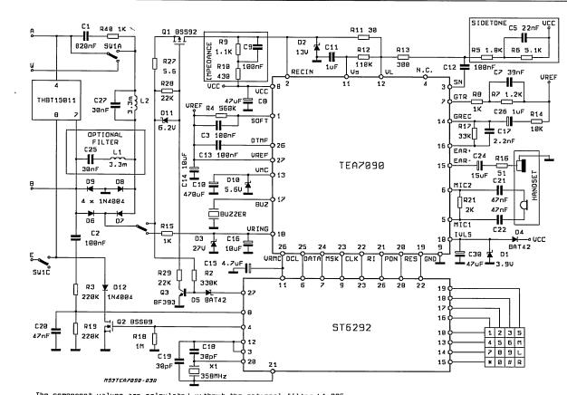
The component values are calculated without the optional filter L1.C25. In case this filter is connected, the sum of C25+C9 should be equal to 100nF. The filter L1.C25 is useful only if the filter L2.C27 has a low Q. The Sidetone is for 2Kms Line + 2ref for Germany.
