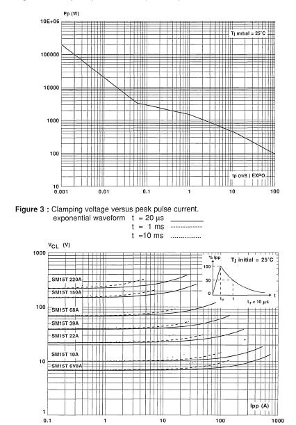
Figure 2 : Peak pulse power versus exponential pulse duration.
