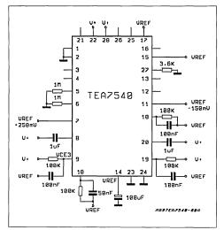
V<sup>+</sup> = 3V pin 7 is forced to transmit mode
