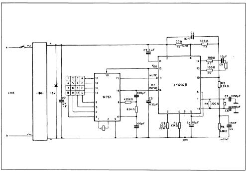
Figure 11 : Application Circuit with Multifrequency (Europe I STD).
