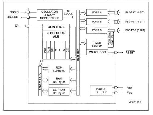
Figure 1. ST7293 Block Diagram
