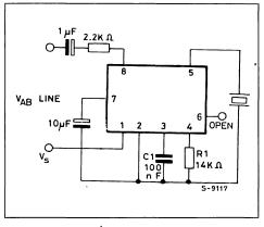
$R_1 \approx \frac{-3.56 \text{ x } 10^4}{F_1 \text{ (HZ)}} \text{ x } \left(1 - 0.12 \text{ x } \ln \frac{F_1}{2543}\right)$
