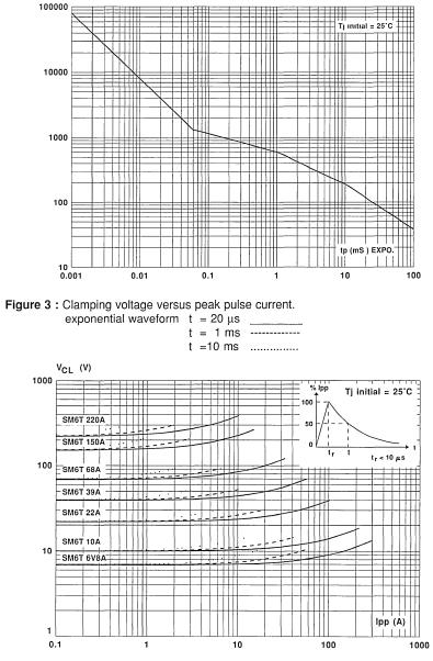
Figure 2 : Peak pulse power versus exponential pulse duration.
