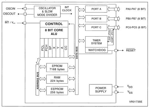
Figure 1. ST72E94 Block Diagram
