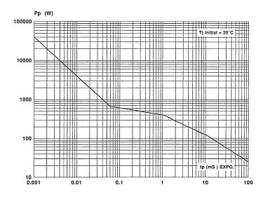
Figure 2 : Peak pulse power versus exponential pulse duration.
