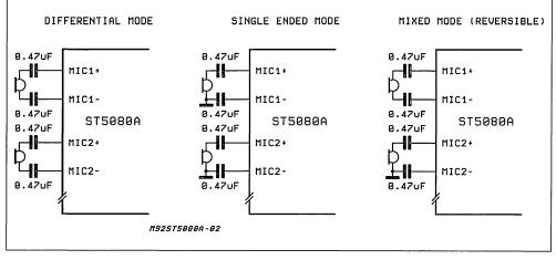
The 4 connection modes (since the MIXED MODE is symmetrical with respect to MIC1 and MIC2) allow one microphone at a time to be selected via the V<sub>S</sub> bit (bit 7 of Control Register CR4).
