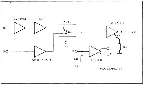
2.1. A.G.C. IN TRANSMISSION. The transmission gain between Microphone Input (pin 8) and Vline (pin 20) is internally decreased of 6dB when the line current varies from 27mA to 42mA with a constant AC load of 600 ohms.
