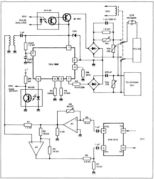
Figure 10 : Complete DAA Interface Circuit with TEA7868.
