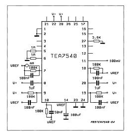
$V^{\star}\!=\!3V$  pin 11 is forced to 100mV to force the transmit mode
