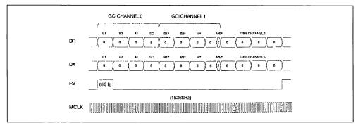
appropriate. During the assigned time slot,  $D_X$  output shifts data out from the voice data register on the rising edges of MCLK. Serial voice data is shifted into  $D_R$  input during the same time slot on the falling edges of MCLK.
