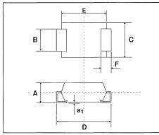
FOOTPRINT DIMENSIONS (Millimeter). SOD 15 Plastic.
