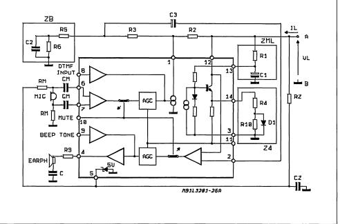
The L3281 is an electronic speech circuit developed to replace hybrid circuits in telephone sets that can be operated in parallel with other phones.
