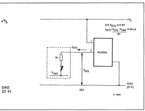
Figure 7a : Gating the ML8204 from CMOS.
