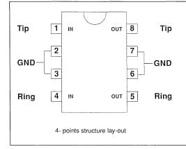
1) Connect pins 2, 3, 6 and 7 to ground in order to guarantee a good surge current capability for long duration disturbances.
