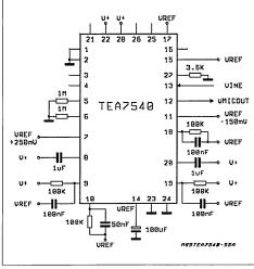
$V^* = 3V$ pin 7 is forced to transmit mode pin 11 is forced to minimum gain Input signal on pin 13 VINE = 1.5mVpp output voltage VMICOUT measured on pin 12
