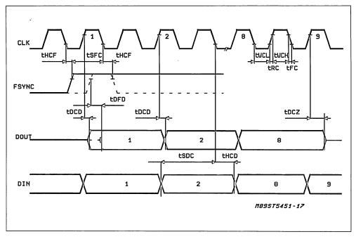
Figure 15: Single Clock Diagram
