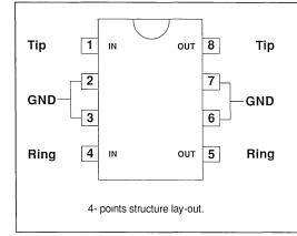
1) Connect pins 2, 3, 6 and 7 to ground in order to guarantee a good surge current capability for long duration disturbances.
