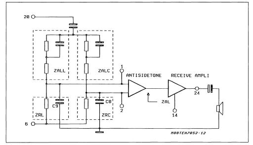
3.1. A.G.C. IN RECEIVE. As described for the transmission chain, also the receiving gains Gr, from pins 1 and 2 to pin 24, have a reduction of 6dB when lline moves from 27mA to 42mA.
