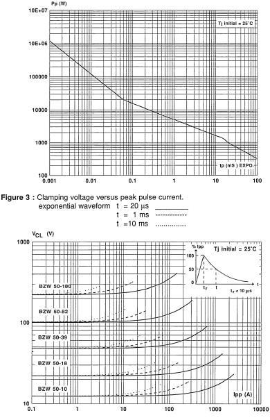
**Note :** The curves of the figure 3 are specified for a junction temperature of 25 °C before surge. The given results may be extrapolated for other junction temperatures by using the following formula :  $\Delta V$  (BR) =  $\alpha T$  (V(BR)) \* [Ta -25] \* V (BR).
