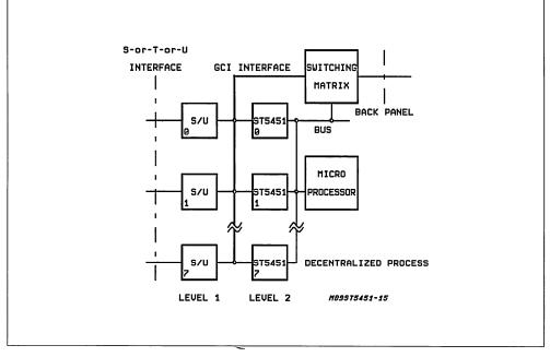
Figure 9: Decentralized D channel handling in NT2 or LT
