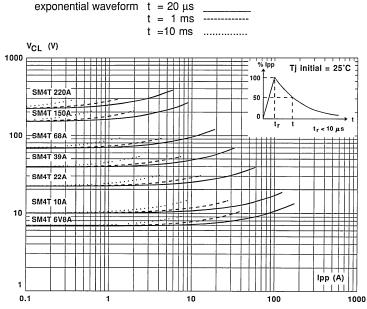
**Note** : The curves of the figure 3 are specified for a junction temperature of 25 °C before surge. The given results may be extrapolated for other junction temperatures by using the following formula :  $\Delta V$  (BR) =  $\alpha T$  (V(BR)) • [Ta -25] • V (BR).
