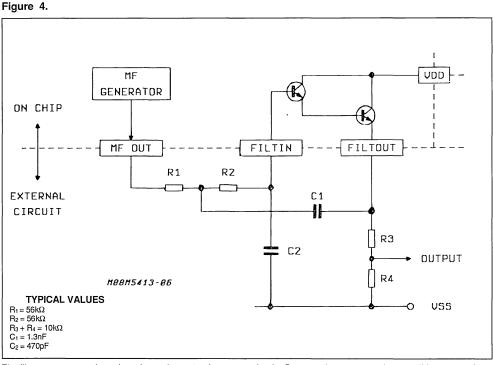
The filter components shown have been chosen to give a second order Butterworth response with a cut-off frequency of about 3.5kHz. The pass-band insertion loss is nominally 0.5dB.
