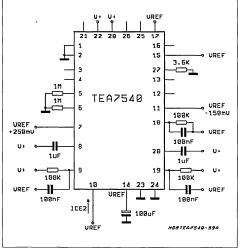
V<sup>+</sup> = 3V pin 7 is forced to transmit mode pin 11 is forced to minimum gain
