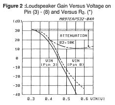
$R_2 = 10 \text{ K} \Rightarrow \text{ATT} = 20 \text{ dB}$
