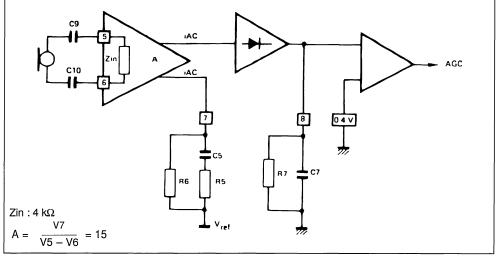
The first filter is generated by the capacitors on pins 5 and 6; the second filter by the R-C network on pin 7.
