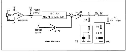
Figure 9: Equivalent Receiving Circuit.
