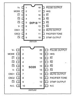
Figure 1 : Pin Connections (top view).
