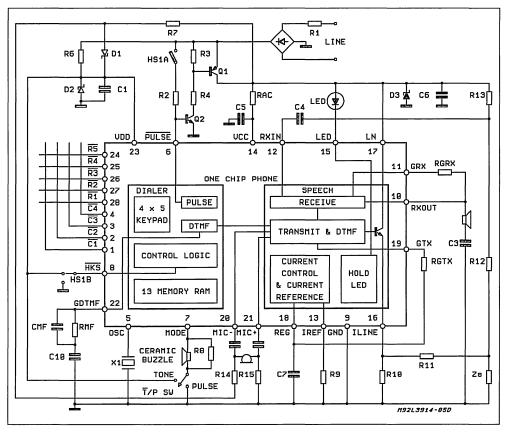
When mated with a tone ringer, a complete telephone can be produced with just two ICs.
