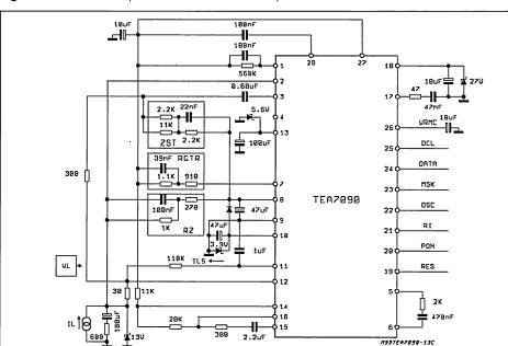
Figure 13: Test1 Circuit (VL/IVRMC/VRMC/IVMC/ILS)
