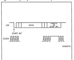
Figure 46. Serial Expansion Mode
