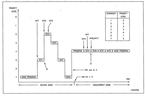
External Interrupts. Up to 8 external interrupts are available on the ST9036 as alternate function inputs of I/O pins. These may be selected to be triggered on rising or falling edges and can be independently masked. The eight interrupt sources are grouped into four pairs or channels which can be assigned to independent interrupt priority levels. Within each
