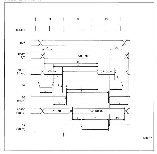
**EXTERNAL WAIT TIMING TABLE** ( $V_{DD}=5V\pm10\%$ ,  $T_{A}=-40^{\circ}C$  to +85°C, Cload = 50pF, INTCLK = 12MHz, Push-pull output configuration, unless otherwise specified)
