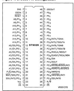
Figure 2. ST9027 Pin Configuration
