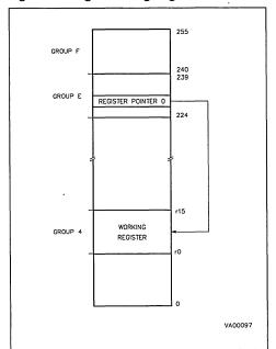
Figure 11. Dual Working Register Banks
