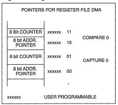
After the transfer of the complete block of data to/from the MFT, the count registers reach the zero value and an end of block interrupt occurs so that the ST9 may process the new data. In many cases, the time taken to reload the data tables and to re-trigger the DMA action causes speed limitations, especially in those applications requiring a continu-
