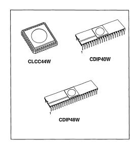
Figure 1. ST90E26,T26 Pin Configuration
