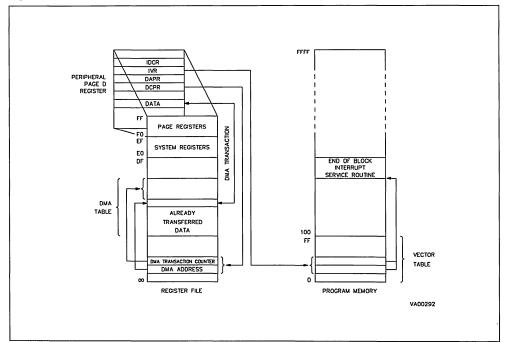
Figure 18. DMA Between Registers and Peripheral
