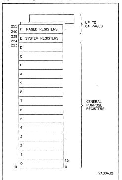
Figure 7. Page Pointer Mechanism
