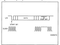
Figure 47. Serial Expansion Mode
