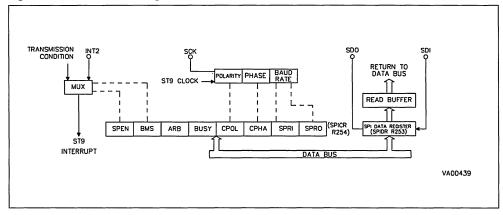
ard serial bus protocol. The SPI uses 3 lines comprising Serial Data Out (SDO), Serial Data In (SDI) and the Synchronous Serial Clock (SCK) which are available as Alternate Functions of I/O pins. Additional I/O pins may act as device selects or IM-bus address ident signals. The functional diagram of the SPI is shown in figure 41.
