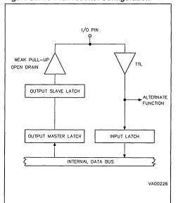
Figure 33. I/O Port Alternate Function Config.
