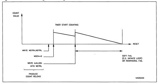
then be retriggered, causing the reloading of the timer value, by the operation of writing of the byte sequence 0AAh, 055h to the WDTLR register. If this is not done before the Watchdog counts to zero, the Watchdog Timeout condition occurs. This causes a Hardware Reset of the ST9040. The Watchdog reset signal is not output on the external RESET pin.
