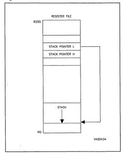
Figure 13. External Stack Pointers
