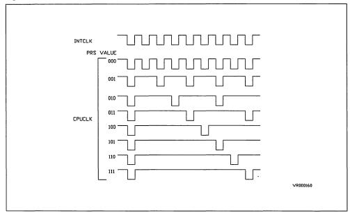
Figure 26. External Memory Interface Timing with CPUCLK Prescaling and 5 Added Wait States
