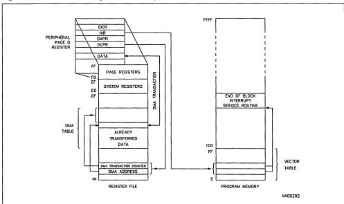
Figure 18. DMA Between Registers and Peripheral
