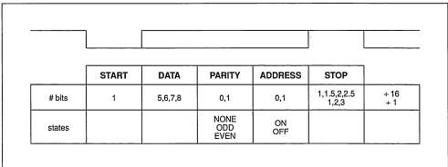
Figure 45. Byte Synchronous Output
