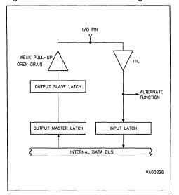
Figure 38. I/O Port Alternate Function Config.
