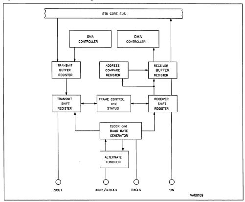
latched on the rising edge of the external synchronised clock input on the RXCLK pin. This mode may be used to access external synchronous peripherals.
