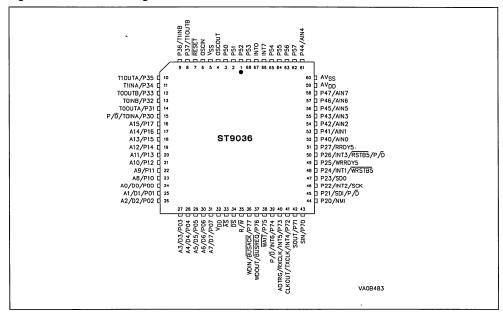
Figure 2. ST9036 Pin Configuration
