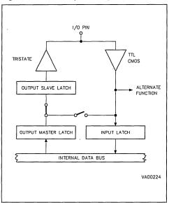
Figure 31. I/O Port Output Configuration
