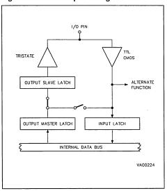
Figure 33. I/O Port Output Configuration
