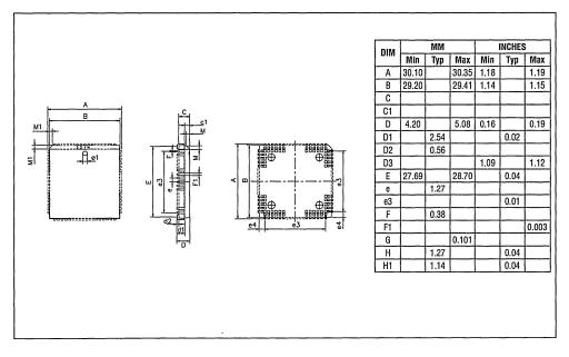
Figure 6. 84-Lead Window Ceramic Leaded Chip Carrier (L)
