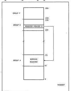
Figure 11. Dual Working Register Banks
