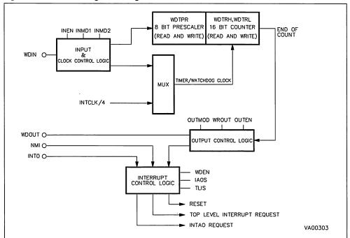
Figure 35. Timer/Watchdog Block Diagram
