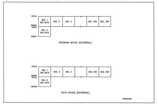
When the Address Expansion is selected, several I/O port configuration registers take an alternative function. The Port Data Registers for I/O ports 2 and 3 (Registers E2h and E3h) become the Bank Switch Data Segment Register and Bank Switch Program Segment Register respectively. The values held in these registers are output on Port 2 whenever a memory access is made to either data or program spaces with A15 high. This allows Port 2 bits to represent either extended address lines
