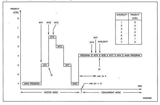
**External Interrupts.** Up to 8 external interrupts are available on the ST9040 as alternate function inputs of I/O pins. These may be selected to be triggered on rising or falling edges and can be independently masked. The eight interrupt sources are grouped into four pairs or channels which can be assigned to independent interrupt priority levels.
