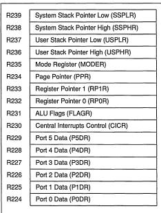
Figure 11. Single Working Register Bank
