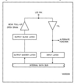
Figure 37. I/O Port Alternate Function Config.
