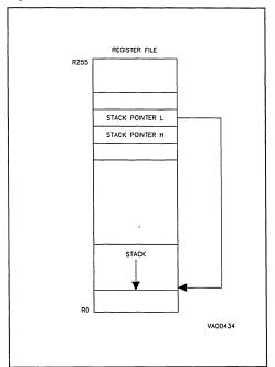
Figure 13. External Stack Pointers
