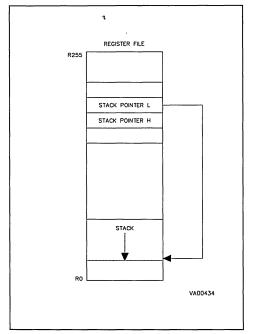
Figure 15. External Stack Pointers
