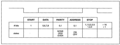
Figure 46. Byte Synchronous Output
