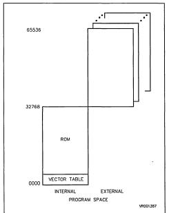
will access the Data Space. When a separate Data Space is not required, data may stored in external RAM or ROM memory within the Program Space.
