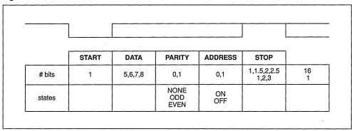
Figure 50. Byte Synchronous Output
