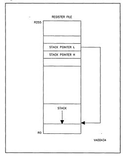
Figure 13. External Stack Pointer
