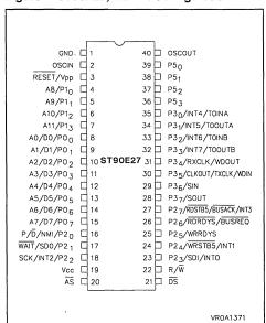
Figure 3. ST90E28,T28 Pin Configuration
