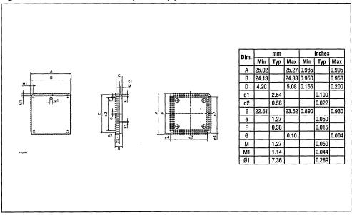
Figure 6. 68-Lead Window Ceramic Leaded Chip Carrier (L)
