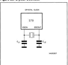
The conceptual schematic of the ST9 internal clock circuit is shown in figure 22.
