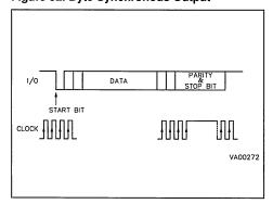
Figure 53. Serial Expansion Mode
