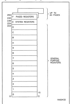
Figure 8. Page Pointer Mechanism
