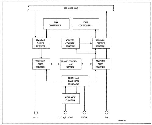
50). For a second synchronous mode, CLKOUT is activated only for the data section of the word (figure 51) on serial data output, and input data is latched on the rising edge of the external synchronised clock input on the RXCLK pin. This mode may be used to access external synchronous peripherals.
