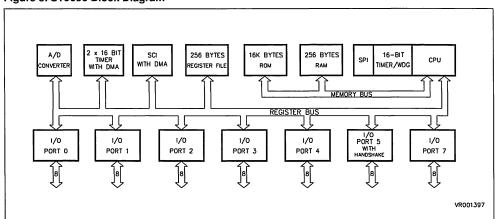
Figure 3. ST9036 Block Diagram
