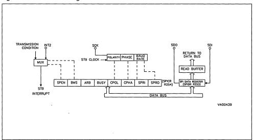
(SDI) and the Synchronous Serial Clock (SCK) which are available as Alternate Functions of I/O pins. Additional I/O pins may act as device selects or IM-bus address ident signals. The functional diagram of the SPI is shown in figure 46.
