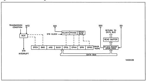
(SDI) and the Synchronous Serial Clock (SCK) which are available as Alternate Functions of I/O pins. Additional I/O pins may act as device selects or IM-bus address ident signals. The functional diagram of the SPI is shown in figure 48.
