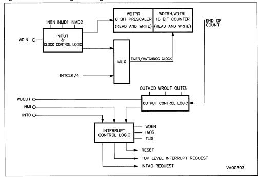
Figure 36. Timer/Watchdog Block Diagram
