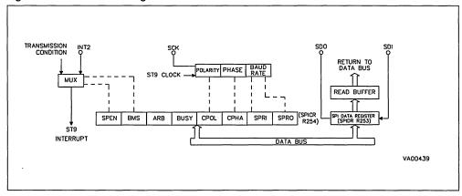
ard serial bus protocol. The SPI uses 3 lines comprising Serial Data Out (SDO), Serial Data In (SDI) and the Synchronous Serial Clock (SCK) which are available as Alternate Functions of I/O pins. Additional I/O pins may act as device selects or IM-bus address ident signals. The functional diagram of the SPI is shown in Figure 42.
