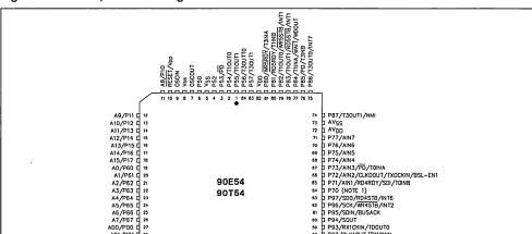
Figure 2. ST90E54,T54 Pin Configuration
