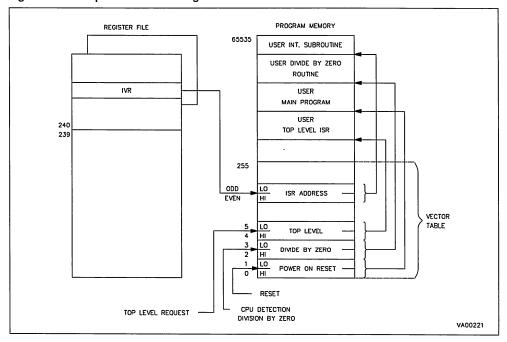
interrupt sources may occur within a peripheral, the peripheral interrupt vector source may be encoded by hardware set bits within the IVR register. This means that the vector address defined in the peripheral IVR is the base address for a block of vectors servicing that peripheral. The address pointed to by the vector is loaded into the Program Counter and execution restarts from this point.
