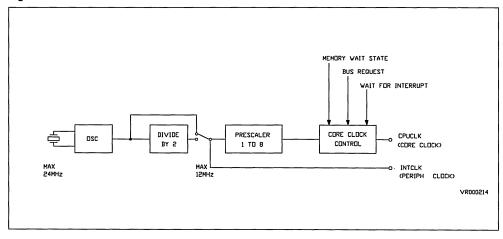
section is named INTCLK, the internal clock which drives the timebases of the on-chip clock for the ST9036 peripherals (eg the Multifunction Timer, Timer/Watchdog, Serial Communications Interface) and also the input of the CPU prescaler section. The CPU of the ST9 includes the instruction execution logic and may run at different rates
