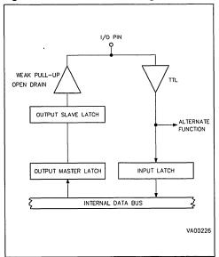
Figure 33. I/O Port Alternate Function Config.
