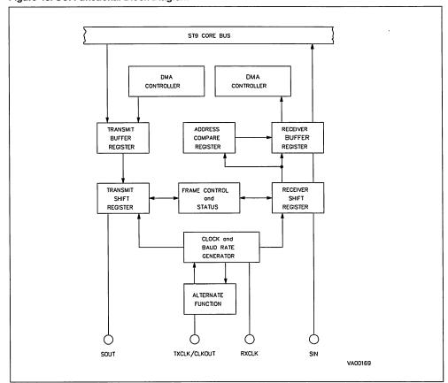
Figure 43. SCI Functional Block Diagram
