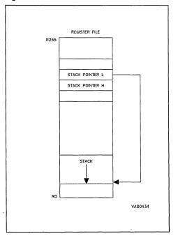
Figure 14. External Stack Pointers
