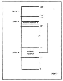
Figure 11. Dual Working Register Banks
