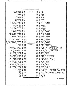
Figure 2. ST9030 Pin Configuration
