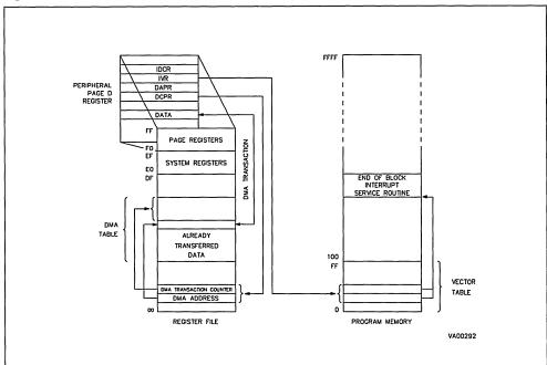
Figure 19. DMA Between Registers and Peripheral
