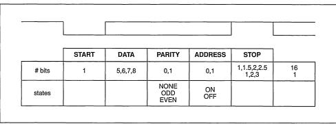
Figure 48. Byte Synchronous Output
