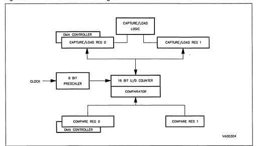
Figure 38. Multifunction Timer Block Diagram
