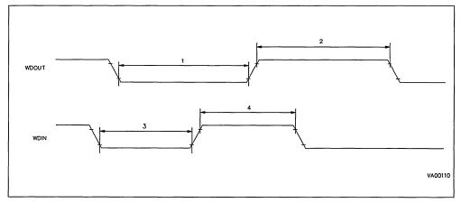
SPI TIMING TABLE (VDD =  $5V \pm 10\%$ , TA = -40°C to +85°C, Cload = 50pF, INTCLK = 12MHz, Output Alternate Function set as Push-pull)
