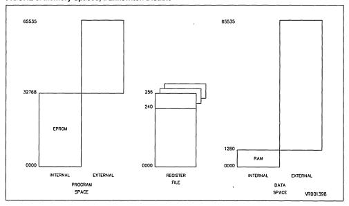
Figure 4. Memory Spaces, Bankswitch Enabled
