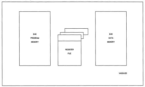
Figure 4. Memory Spaces, Bankswitch Enabled
