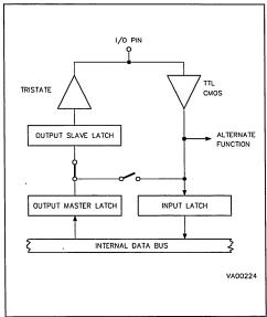
Figure 31. I/O Port Output Configuration
