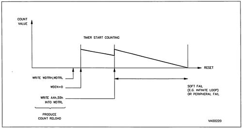
timer prescaler and timer reload value before enabling the Watchdog mode. The Watchdog Timer must then be retriggered, causing the reloading of the timer value, by the operation of writing of the byte sequence 0AAh, 055h to the WDTLR register. If this is not done before the Watchdog counts to zero, the Watchdog Timeout condition occurs. This causes a Hardware Reset of the ST9036. The Watchdog reset signal is not output on the external Reset pin.
