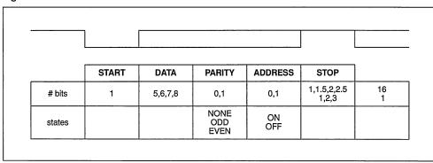
Figure 52. Byte Synchronous Output
