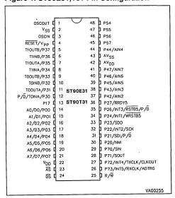
Figure 2. ST90E30,T30 Pin Configuration
