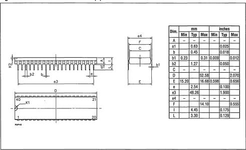
Figure 52. 48-Pin Plastic Dual In Line (B)
