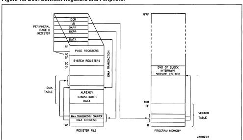
Figure 18. DMA Between Registers and Peripheral
