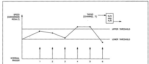
Figure 58. Analog Watchdog Used in Motor Speed Control
