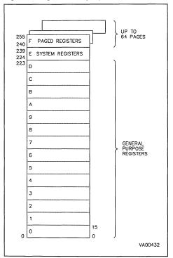
Figure 8. Page Pointer Mechanism
