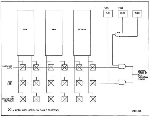
a dummy read from the EEPROM memory (STBY must be active). This triggers the charge pump to generate the high voltage necessary to program the fuse. The Write Fuse bits must be held to a "1" state for the whole of the programming cycle, the end of programming may be monitored on the TLCK or HLCK bit.
