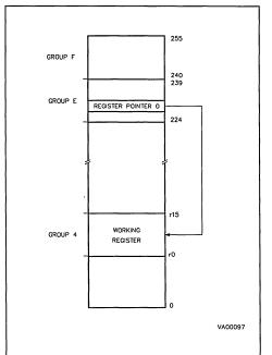
Figure 13. Dual Working Register Bank
