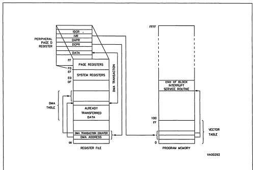
Figure 20. DMA Between Registers and Peripheral
