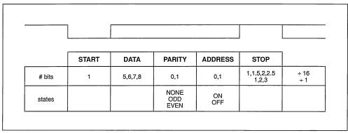
Figure 46. Byte Synchronous Output
