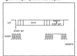
Figure 49. Serial Expansion Mode
