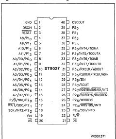
Figure 3. ST9028 Pin Configuration
