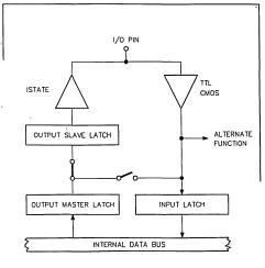
Figure 30. I/O Port Output Configuration
