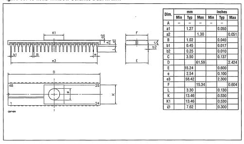
Figure 56. 44-Lead Window Ceramic Leaded Chip Carrier
