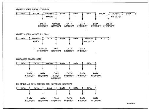
When DMA is active the Receive Data Pending bit (RDP), and the Transmit status bit (THE/TSE) interrupt sources are replaced by the DMA End Of Block Interrupt sources for transmit and receive, respectively.
