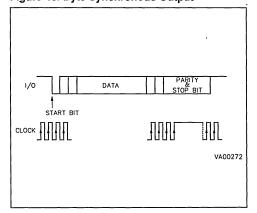
Figure 47. Serial Expansion Mode
