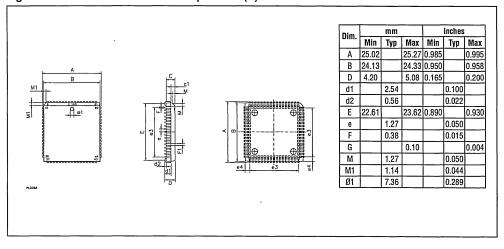
Figure 54. 80-Lead Plastic Quad Flat Package (q)
