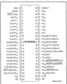
Figure 2. ST90E27,T27 Pin Configuration
