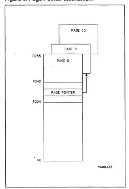
register, the Page Pointer (PPR, R234) within the system register group must be loaded with the relevant page number using the SPP instruction. Subsequently any access to registers in the top group (R240-R255) will refer to the selected page. This remains set until the next change to the Page Pointer register (by the SPP instruction).
