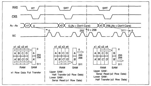
Figure 7. Split Read Transfer Normal Usage
