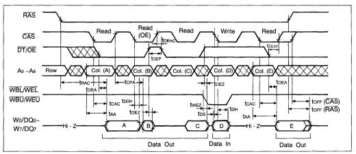
Figure 1. Extended Data Output Example
