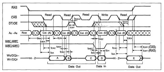
Figure 1. Extended Data Out Example
