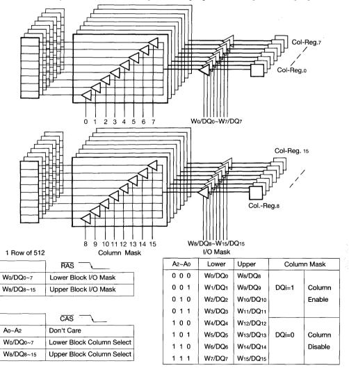
Figure 5. Block Write Scheme
