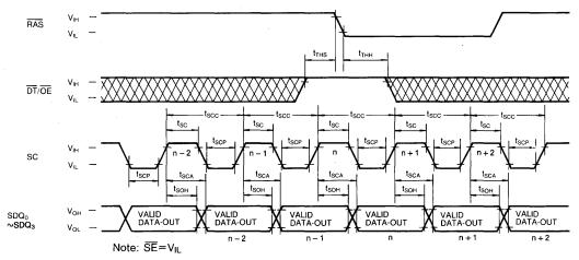
SERIAL READ CYCLE (SE Controlled Outputs)
