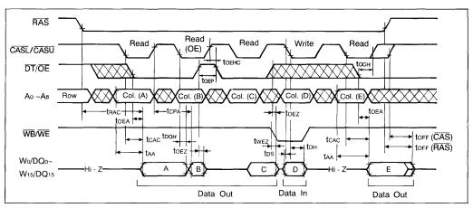
Figure 1. Extended Data Output Example
