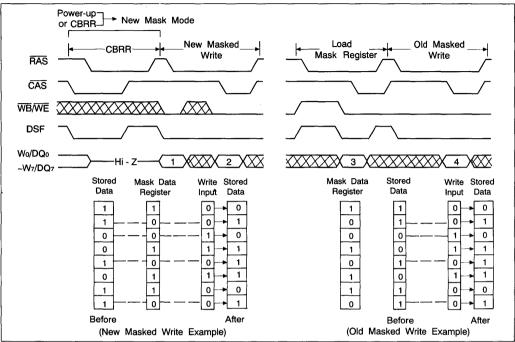
Figure 3. New Mask Write Cycle and Old Mask Write Cycle Example 2.
