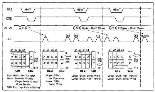
Figure 12. Masked Split Write Transfer Normal Usage
