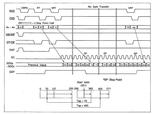
Figure 12. Stop Register Timing
