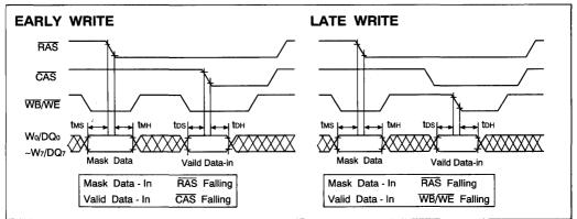
Figure 1. New Mask Write Cycle Example 1. (Early Write & Late Write)
