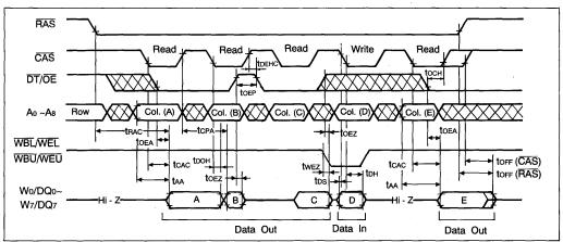
Figure 1. Extended Data Output Example
