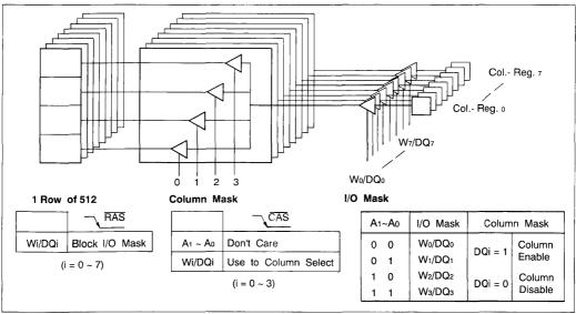
Figure 4. Block Write Scheme
