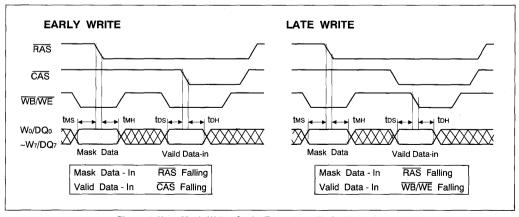
Figure 2. New Mask Write Cycle Example 1 (Early Write & Late Write)
