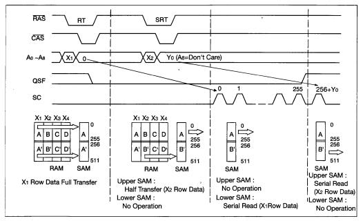
Figure 8. Split Read Transfer Normal Usage (Case 2)
