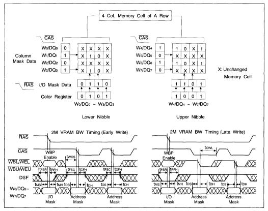
Figure 6. Block Write Example and Timing
