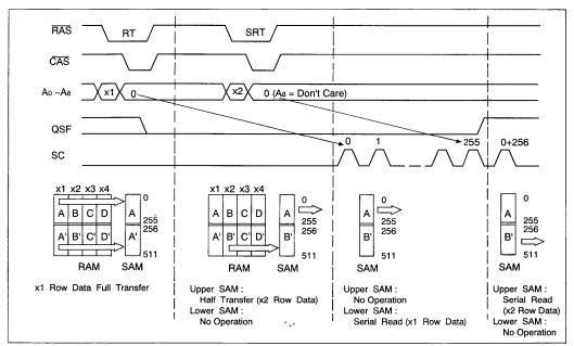
Figure 7. Split Read Transfer Normal Usage
