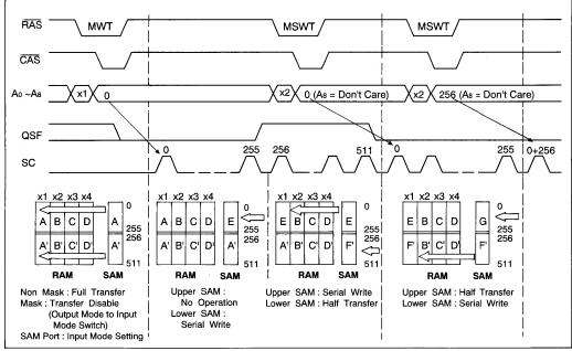
Figure 11. Masked Split Write Transfer Normal Usage
