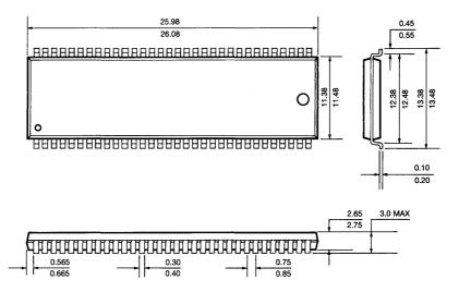
70(64) Pin Plastic Thin Small Out Line Package (Type II Forward)
