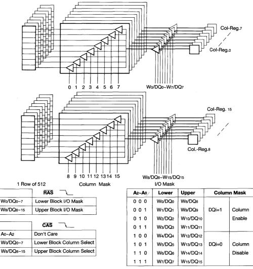
Figure 5. Block Write Scheme
