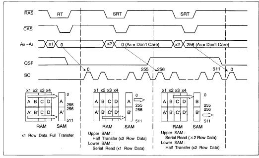
Figure 6. Split Read Transfer Normal Usage
