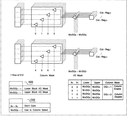
Figure 5. Block Write Scheme
