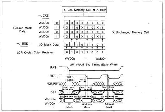
Figure 4. Block Write Example and Timing
