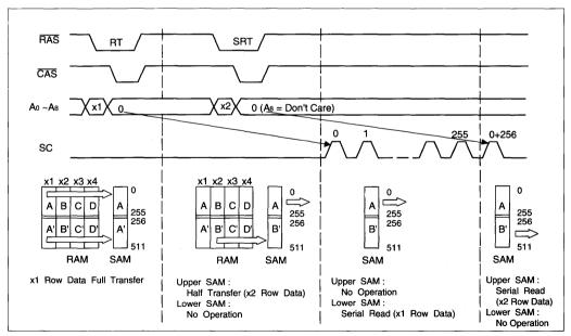
Figure 8. Split Read Transfer Normal Usage
