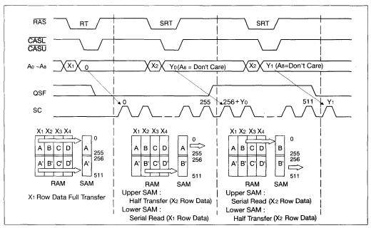
Figure 6. Split Read Transfer Normal Usage (Case1)
