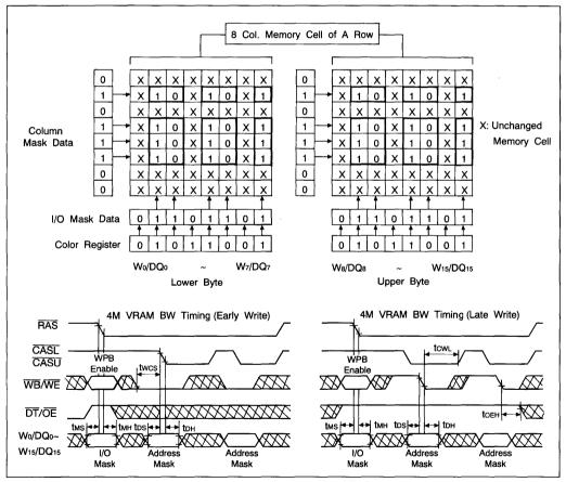
Figure 5. Block Write Example and Timing
