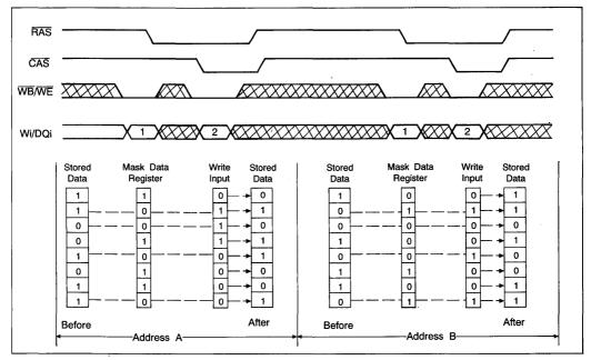
Figure 2. New Mask Write Cycle Example 2.
