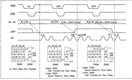
Figure 5. Split Read Transfer Normal Usage
