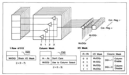
Figure 3. Block Write Scheme
