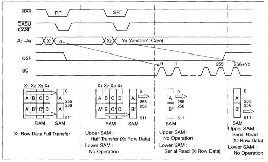
Figure 7. Split Read Transfer Normal Usage (Case 2)
