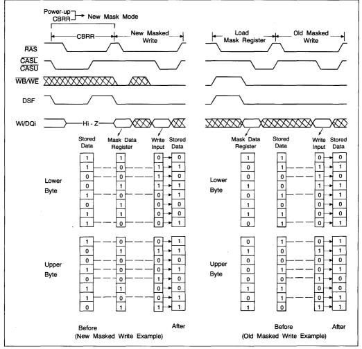
Figure 3. New Masked Write Cycle and Old Masked Write Cycle Example
