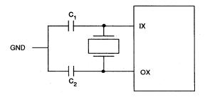
$C1 = C2 = 20 \text{ pf for } C_L = 20 \text{ pf}$  $C1 = C2 = 47 \text{ pf for } C_L = 32 \text{ pf}$
