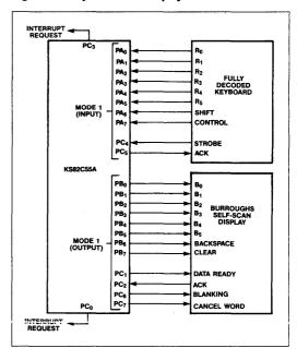
Figure 16: Keyboard and Display Interface
