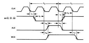
CENL, CMDLY, DEN Characteristics with MB = 0 and CEN = 1 During Write Cycle
