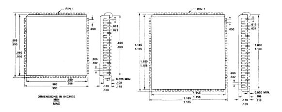
Figure 53. 68-Pin PLCC Package
