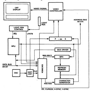
The KS68C45S CRT Controller (CRTC) provides an interface for computers to raster-scan type CRT displays.
