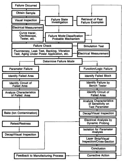
Failure Analysis Procedure Flow Chart
