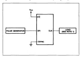
Figure 10: Ready to Clock (Using EFI)
