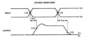
AC Testing inputs are driven at 3.0V for a logic "1" and 0.0V for a logic "0". Timing measurements are made at 2.4V for a logic "1" and 0.8V for a logic "0" at the outputs.
