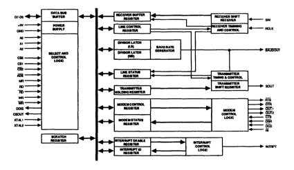
Figure 1 : BLOCK DIAGRAM OF KS82C450/KS82C50A
