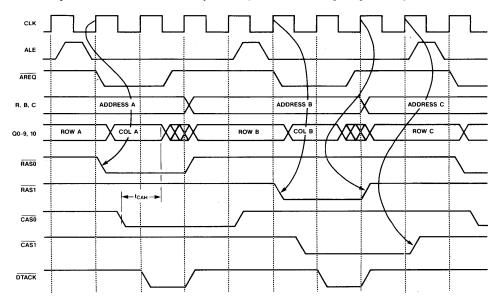
Figure 15. DTACK During Mode 0 Accesses, RAS Initially Asserted
