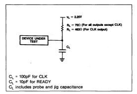
Figure 8: Clock High & Low Time (Using EFI)
