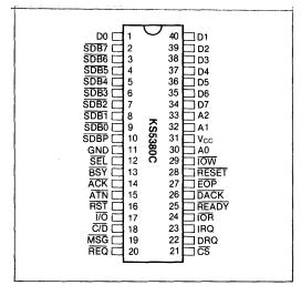
Figure 4. Physical Layout of the KS5380C SCSI Bus Controller (DIP-40 Version)
