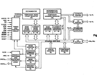
Figure 1: KS82C37A Block Diagram
