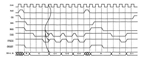
Figure 10. Burst Mode Access with Page Mode DRAMs (ECAS2 = 1, R6 = 1 During Programming)
