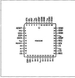
Figure 2. Physical Layout of the KS53C80 SCSI Bus Controller (PLCC Version)
