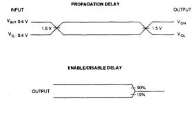
A.C. Testing: All input signals must switch between V $_{\mu}$  0.4 V and V $_{m}$  + 0.4 V TR and TF must be  $\leq$  15 ns.
