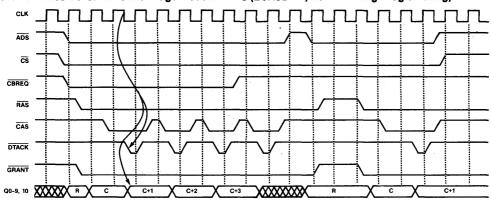
Figure 13. 68030 Burst Mode with Page Mode DRAMs (ECAS2 = 1, R6 = 1 During Programming)
