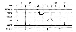
Figure 22 shows two 68040 Burst Mode burst cycles. The DRC has been programmed to assert DTACK on the first rising CLK edge after CAS is asserted. In the first cycle, WAITIN was sampled active on the clock edge that negated DTACK. DTACK is rising edge triggered, so WAITIN is continually sampled on rising CLK edges until it is negated. Since the DRC was programmed to assert
