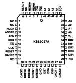
Figure 2: 44 Pin PLCC Configuration
