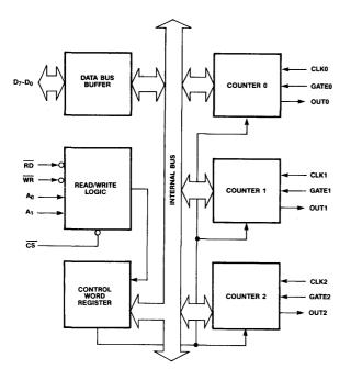
Figure 2: KS82C54 Block Diagram
