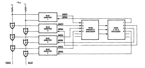
Figure 9. Connections for Serial Priority Resolving Technique
