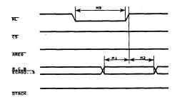
Figure 44. REFRESH, Single Access Mode Burst Mode
