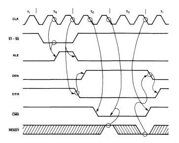
Figure 10. Idle-Write-Idle Bus Cycles with 2 Wait States in Multibus Mode (MB = 1)
