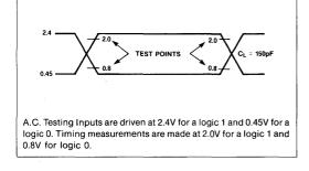
Figure 25: AC Testing Load Circuit
