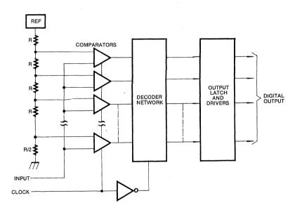
Fig. 1 Flash (Parallel) A/D Converter
