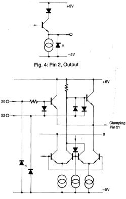
Fig. 6: Pins 20 and 22, Inputs
