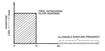
Fig. 2 Shown in the shaded area is an ideal, low pass, anti-aliasing filter responce.
