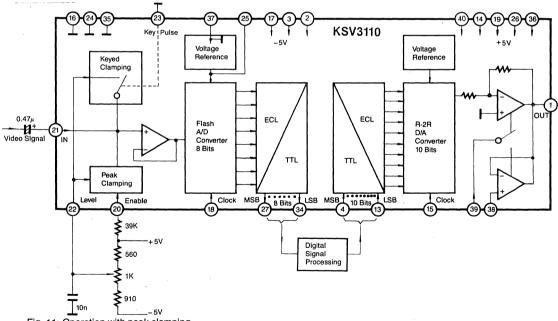
Fig. 11: Operation with peak clamping
