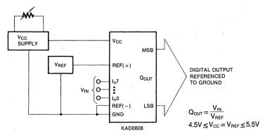
Fig. 10 Ground Referenced Conversion System Using Trimmed Supply
