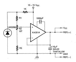
Fig. 12 Typical Reference and Supply Circuit
