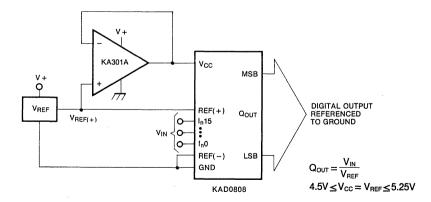
Fig. 6 Ground Referenced Conversion System with Reference Generating V<sub>cc</sub> Supply
