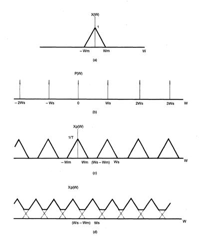
Fig 3. Effect in the frequency domain of sampling in the time domain:
