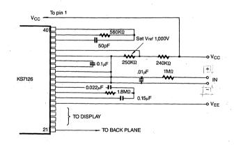
Figure 18: Recommended Component Values for 2.00V Full-Scale, One Reading Per Second. \* Values depend on clock frequency. See Figure 10, 12,15
