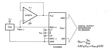
Fig. 11 Ground Referenced Conversion System with Reference Generating V<sub>cc</sub> Supply
