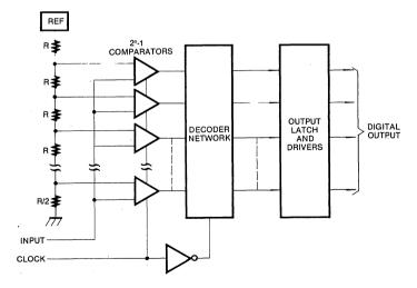
Fig. 3 Flash (Parallel) A/D Converter
