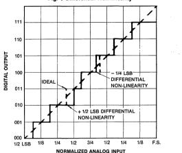
Fig. 6 Differential Non-linearity
