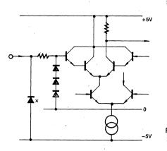
Fig. 10: Pin 38, Input x=protection diode
