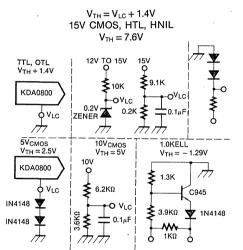
Do not exceed negative logic input range of DAC. Fig. 9 Interfacing with Various Logic Families
