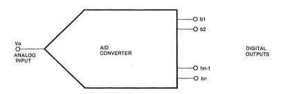
Fig. 1 Symbolic Block Diagram of A/D Converter
