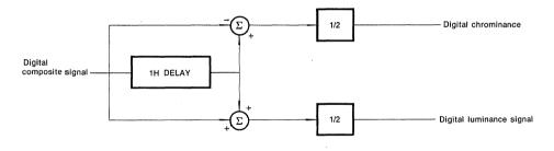
Fig. 4 Digital Comb Filter
