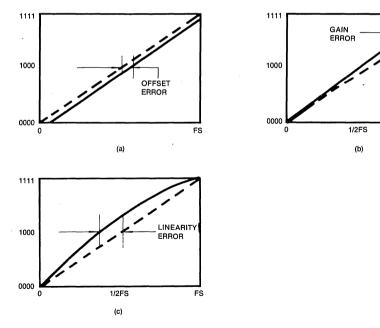
Fig. 1 Errors for an A/D Converter; (a) Offset; (b) Gain; (c) Linearity
