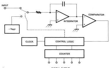
DIGITAL OUTPUT Fig. 6 Functional Block Diagram of Dual-Slope A/D Converter.
