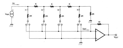
Fig. 11 R-2R Ladder D/A Converter
