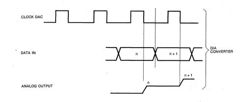
(The Timing Diagram of D/A Part)
