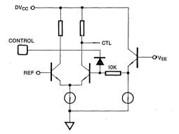
Fig. 4 Pin 19-26, Digital Input
