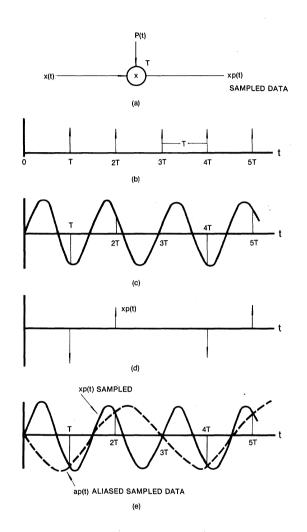
Fig. 1 When sampling, many signals may be found to have the same set of data points. These are called aliaes of each other.
