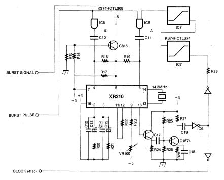
(The Clock Generator Circuit)
