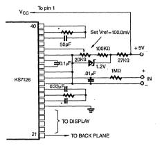
Figure 13: KS7126 Operated From Single +5V Supply. An External Reference Must Be Used.
