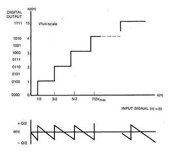
Fig. 8 Quantization characteristics.
