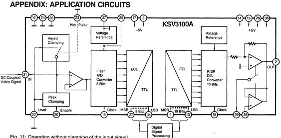
Fig. 11: Operation without clamping of the input signal
