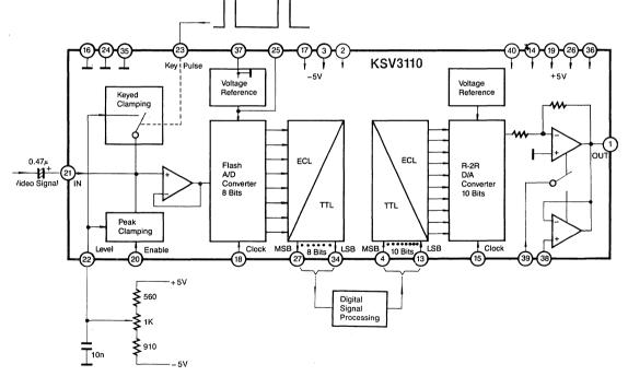
Fig. 13: Operation with keyed clamping
