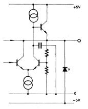
Fig. 8: Pin 25, Reference Voltage Pin
