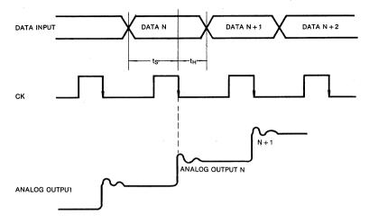
Fig. 11 KSV3110 Timing Diagram (D/A)
