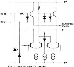
Fig. 7 Pins 22 and 24, Inputs
