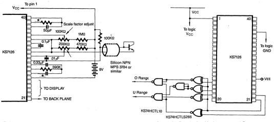
Figure 16: KS7126 Used as a Digital Centigrade Thermometer. A Silicon Diode-Connected Transistor Has a Temperature Coefficient of About 2mV/°C. Figure 17: Circuit for Developing Underrange and Overrange Signals from KS7126 Outputs.
