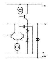
Fig. 8: Pin 25, Reference Voltage Pin
