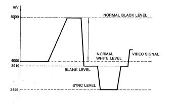
Fig. 10 With Inverse Signal Input
