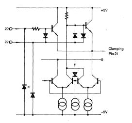
Fig. 6: Pins 20 and 22, Inputs
