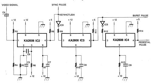
(The Pulse Generator Circuit)
