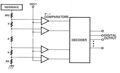
Fig. 4 Functional Block Diagram of Flash A/D Converter
