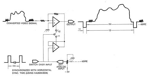
Add horizontal sync. pulse of video signal to the converted composited signal; result is the stabilized sync. pulse
