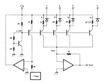
Fig. 10 Weighted Current Source D/A Converter
