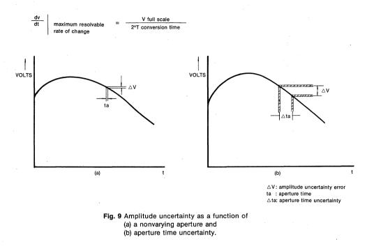
If for example V full scale = 10.24 volts, T conversion time = 10ms, and n = 10 or 1024 bits of resolution then the maximum rate of change resolvable by the A/D converter would be Q volt/sec. If the input signal has a faster rate of change than 1 volt/sec, 1 LSB changes cannot be resolved within the sampling period.
