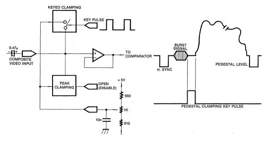
Fig. 7 Operating Keyed Clamping
