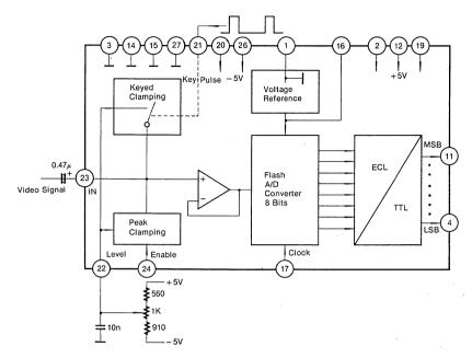
Fig. 11: Operation with keyed clamping
