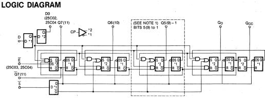
NOTE 1: Cell logic is repeated for register stages Q5 to Q1 KS25C02, KS25C03 2: Numbers in parenthesis are for KS25C04
