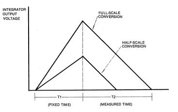
Fig. 7 Integrator Output Waveform for Dual-Slop A/D Converter
