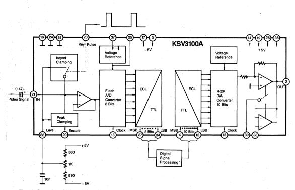
Fig. 13: Operation with keyed clamping
