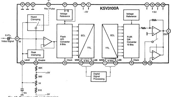
Fig. 12: Operation with peak clamping
