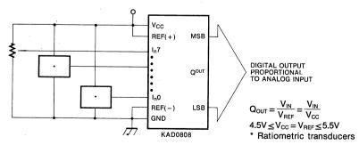
Fig. 9 Ratiometric Conversion System
