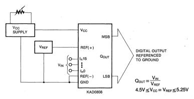
Fig. 5 Ground Referenced Conversion System Using Trimmed Supply
