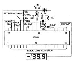
Figure 2: KS7126 Clock Frequency 48 KHz (3 readings/sec.)
