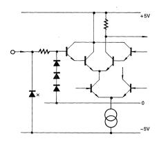
Fig. 10: Pin 38, Input x=protection diode
