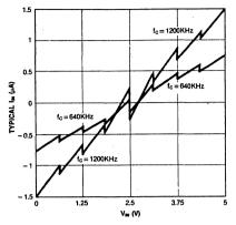
Fig. 1 Comparator  $I_{IN}$  vs  $V_{IN}$  ( $V_{CC} = V_{REF} = 5V$ )
