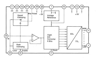
Fig. 4 KSV3208 Block Diagram
