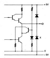
Fig. 4: Pin 4 to 11, Outputs
