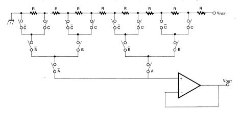
Fig. 12 3-Bit D/A Converter Example Using Voltage-Scaling Principle
