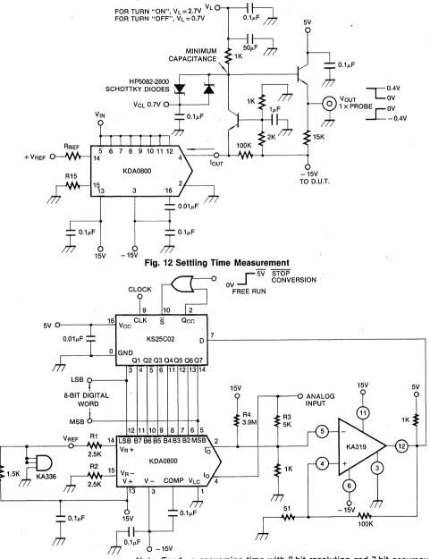
Note. For 1 μs conversion time with 8-bit resolution and 7-bit accuracy, an KA361 comparator replaces the KA319 and the reference current is doubled by reducing R1, R2 and R3 to 1.25KΩ and R4 to 2MΩ.
