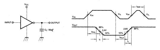
Fig. 1 AC Test Circuit
