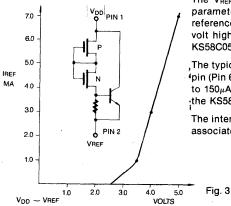
The V<sub>REF</sub> output provides a reference voltage that tracks internal parameters of the KS58C05. V<sub>REF</sub> provides a negative voltage reference to the V<sub>DD</sub> supply. Its magnitude will be approximately 0.6 volt higher than the minimum operating voltage of each particular KS58C05.
