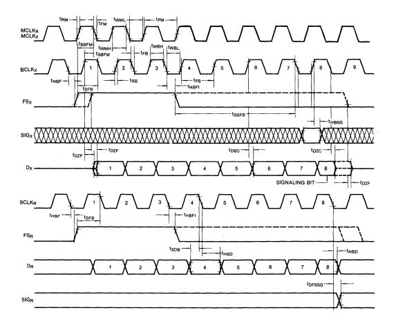
Fig. 3 Long Frame Sync Timing
