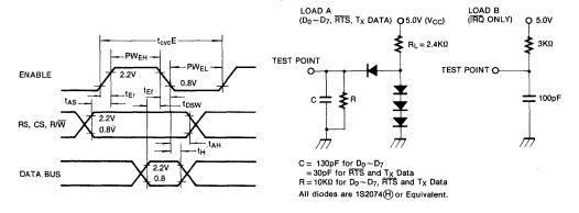
Fig. 8 Bus Write Timing Characteristics (Write information into UART)
