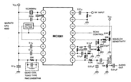
In the above typical application, the audio signal is recovered using a conventional quadrature FM detector. The absence of an input signal is indicated by the presence of noise above the desired audio frequencies. This "noise band" is monitered by an active filter and a detector. A squelch trigger circuit indicates the presence of noise (or a tone) by an output which can be used to control scanning. At the same time, an internal switch is operated which can be used to mute the audio.
