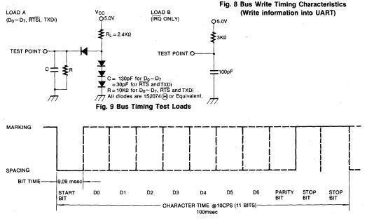
Fig. 10 110 Baud Serial ASCII Data Timing
