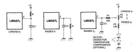
Fig. 7 Detection Band Skew Adjustment
