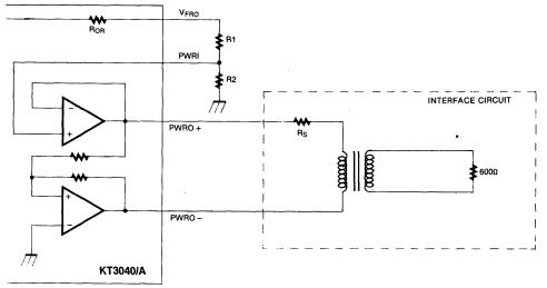
Typical Connection of Output Driver Amp
