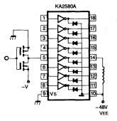
Telecommunication Relay Driver (Negative Logic)
