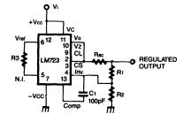
Note: R1•R2/(R1+R2)for minimum temperature drift. R3 may be eliminated for minimum component count.
