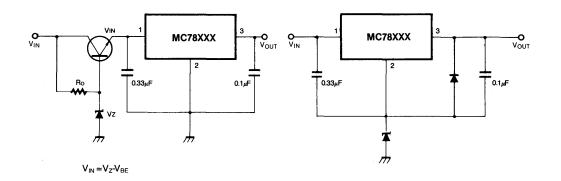
Fig. 20 High Input and Output Voltage
