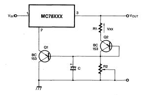
Note: Q2 is connected as a diode in order to compensate the variation of the Q1 VBE with the temperature. C allows a slow rise-time of the  $V_0$
