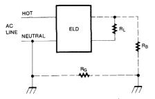
Explain: An unintentional electrical path,  $R_B$ , between the load terminal of the hot line and the ground, as shown by the dashed lines.
