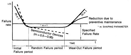
Figure 3. Failure Rate Curve ("Bath Tub Curve")
