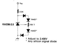
Fig. 7 Trimmed 4V to 6V reference with temperature coefficient of breakdown voltage independent
