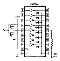
Telecommunicaiton Relay Driver (Positive Logic)
