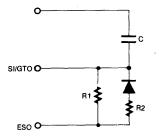
$$\begin{split} t_{GTP} &= (RpC) In(V_{DD}/V_{DD} - V_{TST}) \\ t_{GTA} &= (R1C) In(V_{DD}/V_{TST}) \\ Rp &= R1R2/(R1 + R2) \\ (a) \ Decreasing \ t_{GTP}(t_{GTP} < t_{GTA}) \end{split}$$
