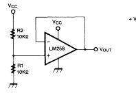
Fig. 14 Non-Inverting DC Gain
