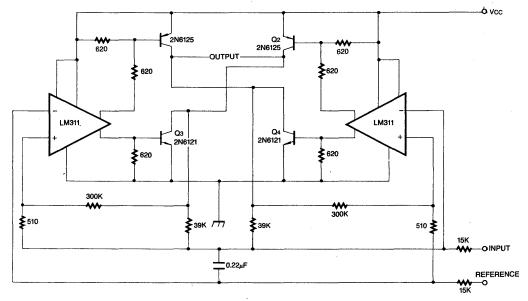
Fig. 2 Relay Driver with Strobe
