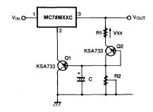
Note: Q2 is connected as a diode in order to compensate the variation of the Q1 VBE with the temperature. C allows a slow rise-time of the Vo
