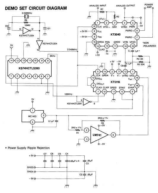
NOTE: All unused input connected to GNDD or V<sub>CC</sub>, only in HCT series.
