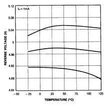
Fig. 9 5.0V REFERENCE WITH MINIMUM
