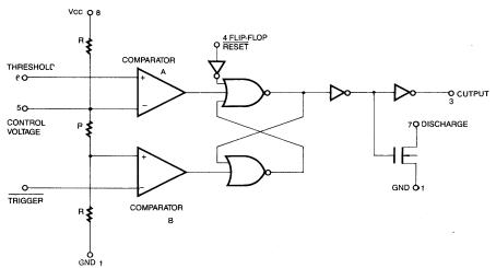
This block diagram reduces the circuitry down to its simplest equivalent components. Tie down unused inputs.  $R = 100K\Omega \pm 20\%$  Typ.
