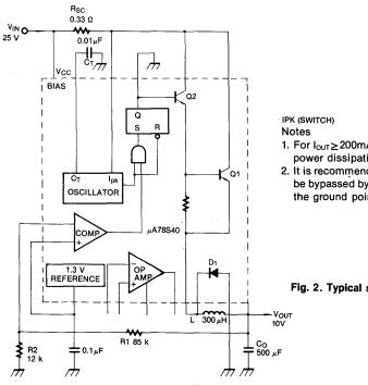
For I<sub>OUT</sub>≥200mA use external diode to limit on chip power dissipation.
