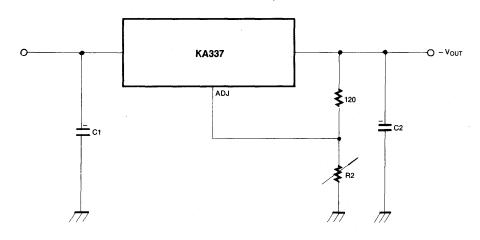
\*  $-V_{OUT} = -1.25V (1 + R2/120\Omega) + (-I_{adj} * R2)$
