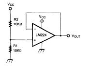
Fig. 14 Non-Inverting DC Gain
