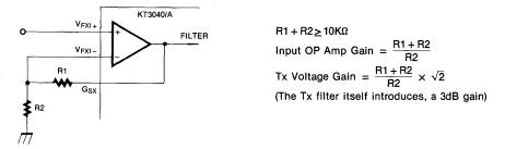
The Tx input stage is followed by a prefilter which is a two-pole RC active low pass filter designed to attenuate high frequency noise before the input signal enters the switched capacitor band pass filter. A band pass filter provides rejection of 200Hz or lower noise which may exist in the signal path, and stopband attenuation which exceeds the D3 and D4 specifications as well as the CCITT G712 recommendations.
