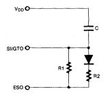
$$\begin{split} t_{GTP} = (R1C) In(V_{DD}/V_{DD} - V_{TST}) \\ t_{GTA} = (RpC) In(V_{DD}/V_{TST}) \\ Rp = R1R2/(R1 + R2) \\ (a) \ Decreasing \ t_{GTA}(t_{GTP} > t_{GTA}) \end{split}$$
