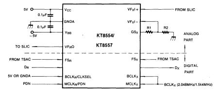
Note : XMIT gain =  $20 \times \log(\frac{R1 + R2}{R2})$ , (R1 + R2) > 10K $\Omega$ .
