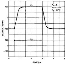
Fig. 12 INVERTING LARGE SIGNAL PULSE RESPONSE
