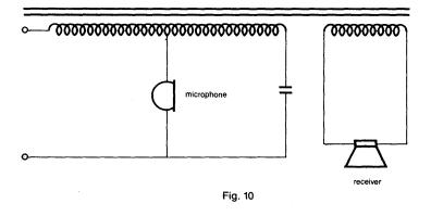
A traditional speech circuit is equivalently equal to the circuit as described in Fig. 7. The microphone is composed of carbon powder. It converts the sound presure into the variation of resistance and so a AC signal is generated when the bias current flows through the microphone and a subscriber is talking. The current actuated by microphone does not affect receiver because it is compensated by the coil polarity.
