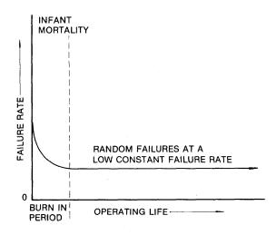
eliability theory assumes that devices fail according to the above curve. When a group of devices is manufactured a small portion of the units will be inherently weaker than the average. These weak units will probably fail during the first few hours of operation—hence the term "infant mortality." If the units are burned-in however, thereby allowing the weak units to fail, there is a much lower probability that those finally put into system use will fail.
