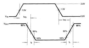
Fig. 2 Switching Waveforms
