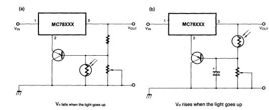
Fig. 25 Light Controllers (Vo min = VXX + VBE)
