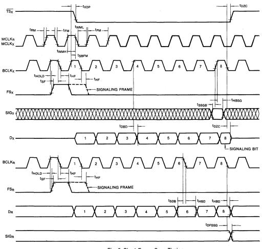
Fig. 2. Short Frame Sync Timing
