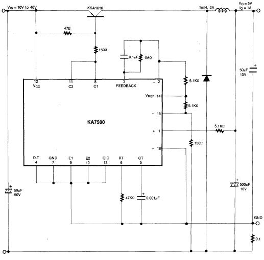
Fig. 1 PULSE WIDTH MODULATED STEP-DOWN CONVERTER
