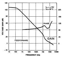
Fig. 17 LARGE SIGNAL FREQUENCY RESPONSE
