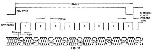
Note: All rise and fail times are measured from 0.4V and 2.4V. All delay times are measured from 1.4V.
