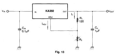
C<sub>in</sub>: C<sub>in</sub> is required if regulator is located an appreciable distance from power supply filter.
