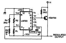
Fig. 6 Positive voltage regulator
