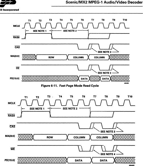
Figure 6-12. Fast Page Mode Write Cycle
