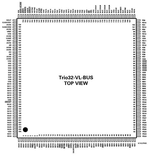
Figure 3-2. Trio32 VL-Bus Configuration Pinout
