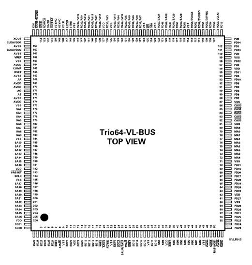
Figure 3-4. Trio64 VL-Bus Configuration Pinout
