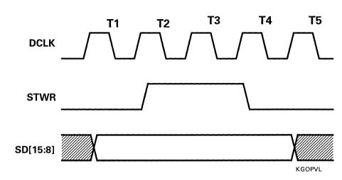
Figure 10-9. General Output Port Timing (VL-Bus)
