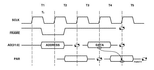
Figure 6-7. Read Parity Operation
