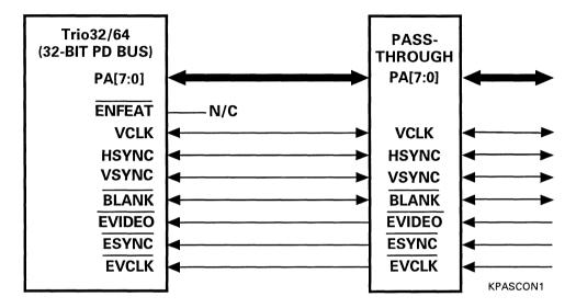
Figure 10-12. Pass-Thru Feature Connector (32-bit PD)
