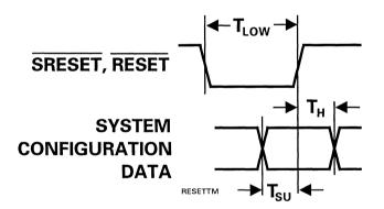
Figure 4-4. Reset Timing
