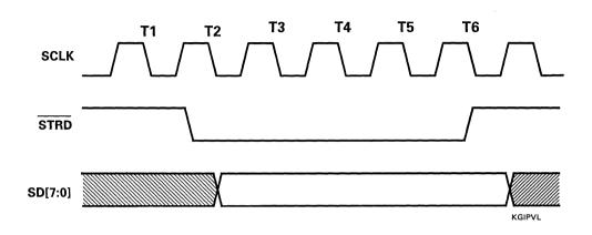
Figure 10-7. General Input Port Timing (VL-Bus)
