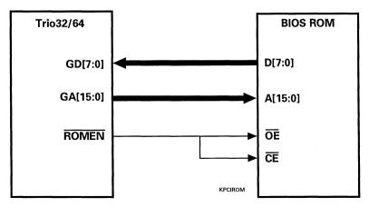
Figure 10-1. BIOS ROM PCI Configuration Interface
