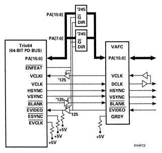
Figure 10-11. VAFC Implementation (64-bit PD Bus)
