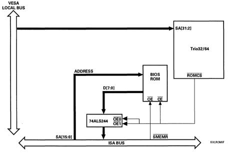
Figure 10-2. BIOS ROM VL-Bus Configuration Interface
