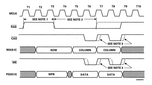
Figure 7-5. Fast Page Mode Write Cycle
