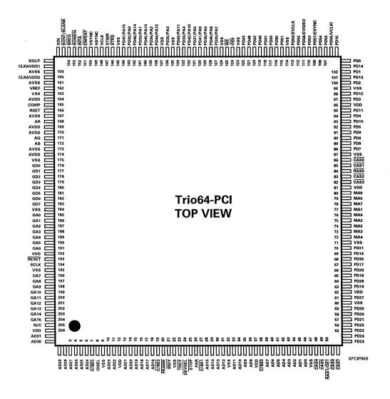
Figure 3-3. Trio64 PCI Bus Configuration Pinout
