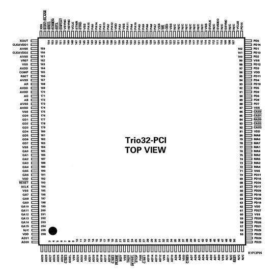
Figure 3-1. Trio32 PCI Bus Configuration Pinout
