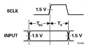
Figure 4-2. Input Timing
