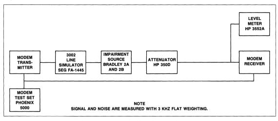
**BER Performance Test Set-up**
