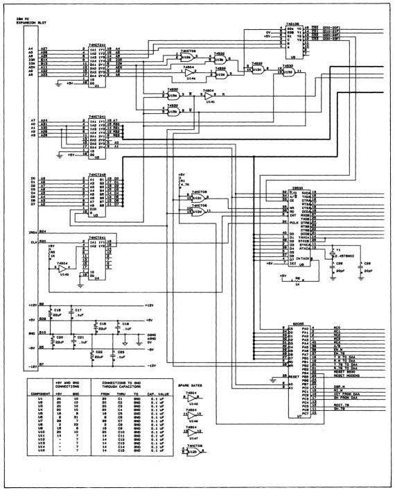
Figure 3. International Modem Schematic
