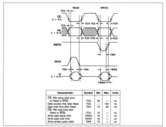
Figure 2. Microprocessor Interface Timing Diagram
