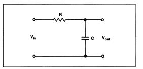
Figure 18. Equivalent Analog RC-Network
