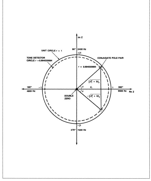
Figure 4. Z-Plane Pole-Zero Diagram
