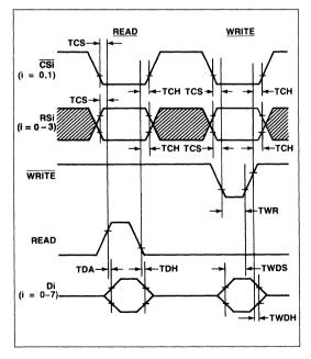
**Microprocessor Interface Timing Diagram**
