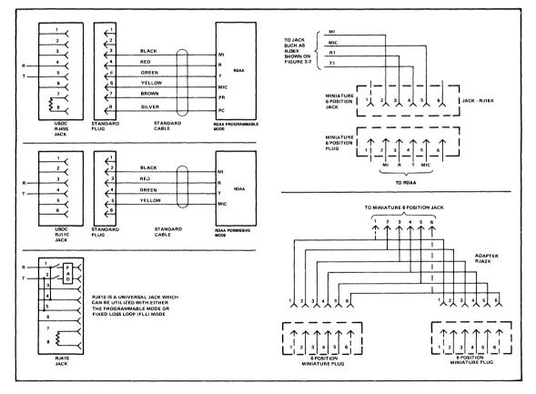
Figure 4. Standard Jacks, Plugs and Cable Color Codes
