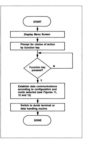
Figure 9. Flowchart - Main Operation
