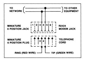
Figure 4. RJ11 Telephone Jack
