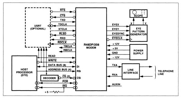
Figure 1. R48DP/208 Functional Interconnect Diagram
