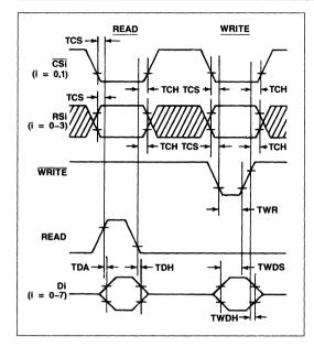
Microprocessor Interface Timing Requirements
