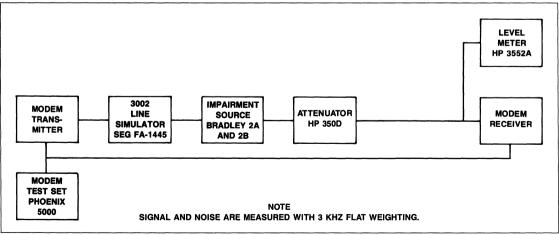
**BER Performance Test Set-up**
