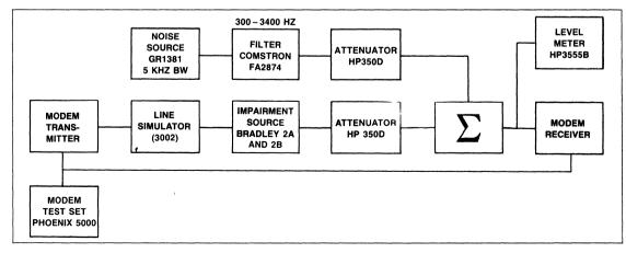
Figure 6. BER Performance Test Set-up
