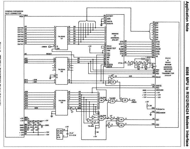
Figure 2. IBM PC to R1212/R2424 Modem Schematic
