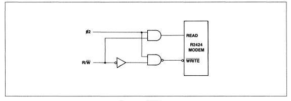
Figure 3. R/W to READ WRITE Conversion Logic
