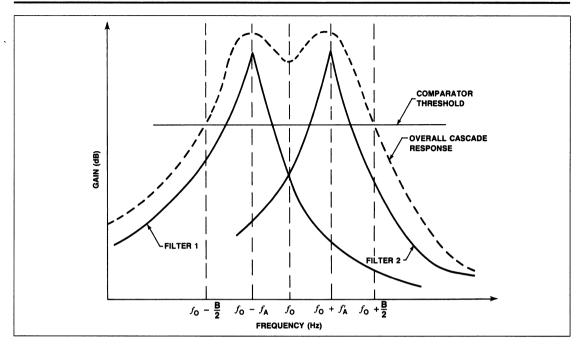
Figure 5. Graphical Representation of Bandwidth (B) and Offset Frequencies ( $f_A$  and  $f'_A$ )
