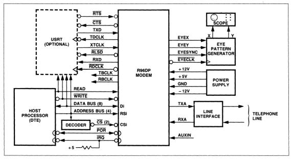
Figure 1. R96DP Functional Interconnect Diagram
