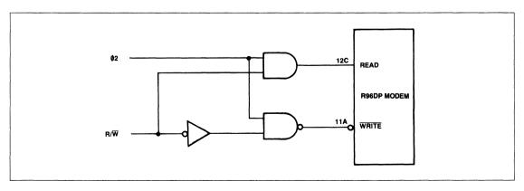
Figure 3. R/W to READ WRITE Conversion Logic
