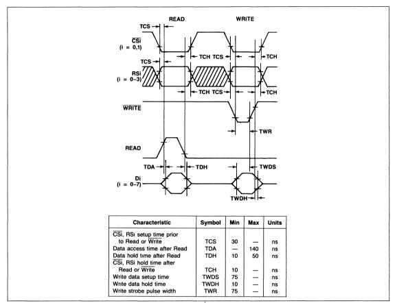
Figure 2. Microprocessor Interface Timing Diagram
