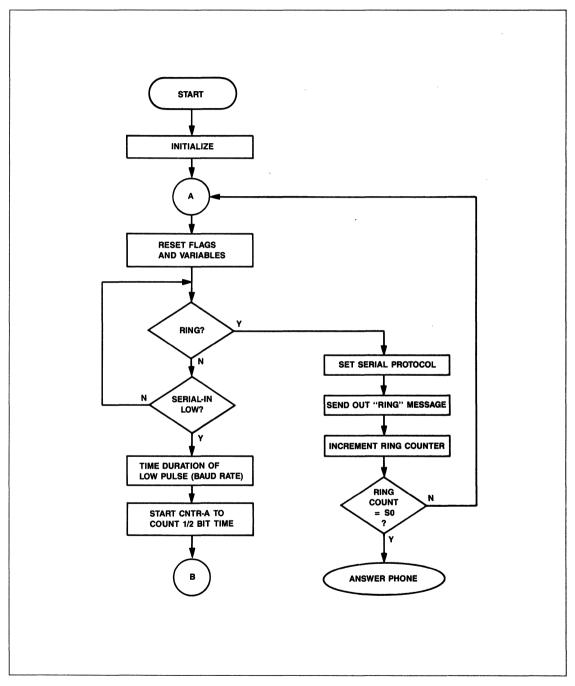
Figure 5. Command Mode Flowchart
