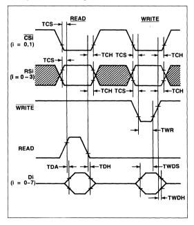
**Microprocessor Interface Timing Diagram**
