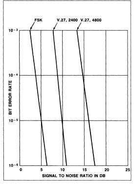
Typical Bit Error Rate (Back-to-Back, Level – 20 dBm)
