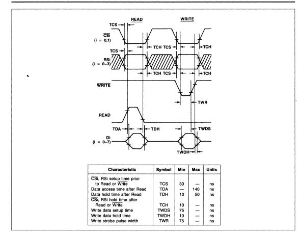
Figure 2. Microprocessor Interface Timing Diagram
