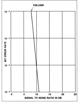
Typical Bit Error Rate (Back-to-Back, Level – 20 dBm)
