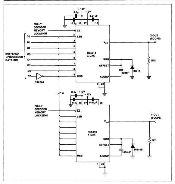
Figure 11. Typical Microprocessor Bus Eye Pattern Generator
