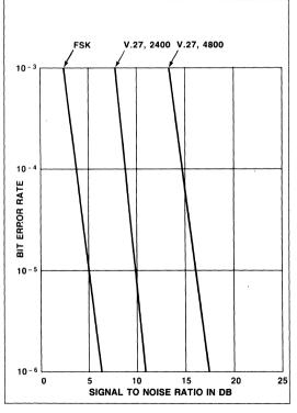
Typical Bit Error Rate (Back-to-Back, Level – 20 dBm)
