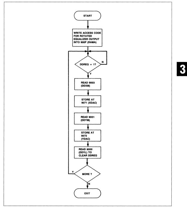
Figure 7. Eye Pattern Generation Flowchart
