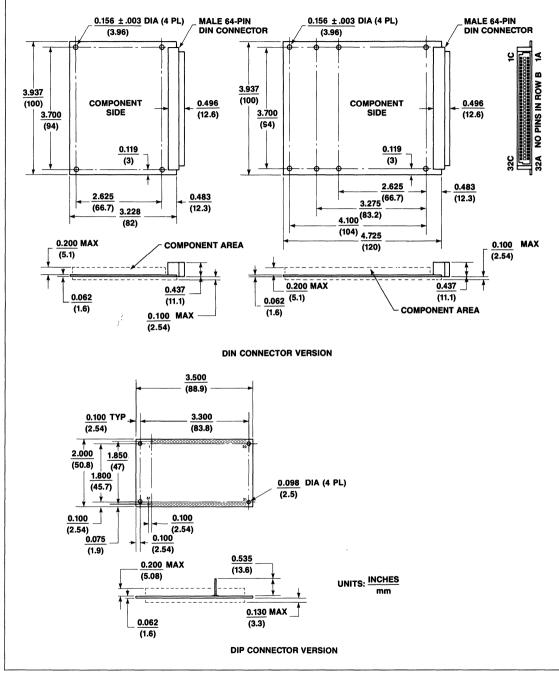
Figure 13. Modem Printed Circuit Board Dimensions
