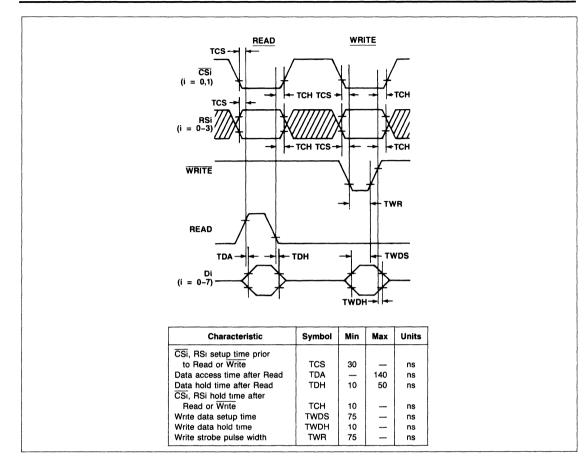
Figure 2. Microprocessor Interface Timing Diagram
