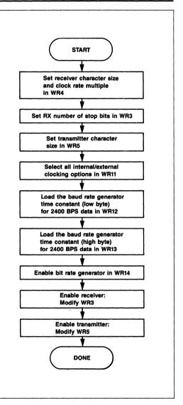
Figure 6. Flowchart — Basic Devices Setup: 8530
