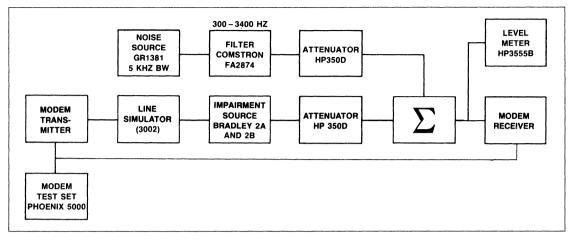
Figure 8. BER Performance Test Set-up
