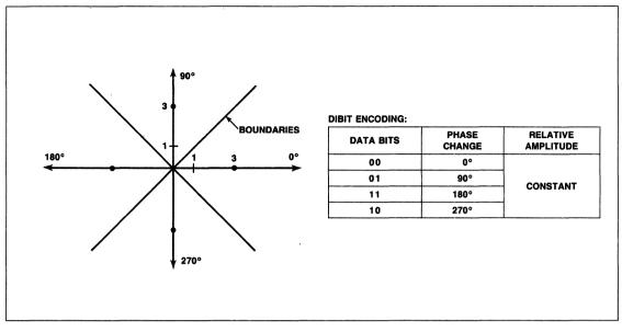
Figure 7. Ideal Eye Pattern-V.29/4800 bps and V.27/BIS/TER/2400 bps
