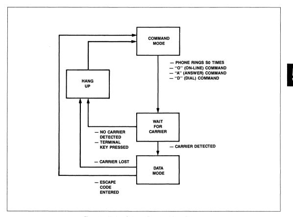
Figure 4. Modem Software Functional State Diagram
