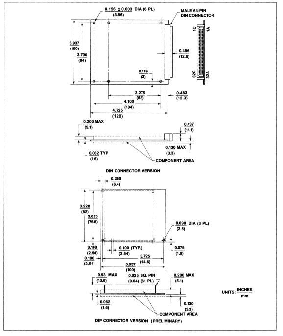
Figure 9. R96DP Modem Dimensions and Pin Locations
