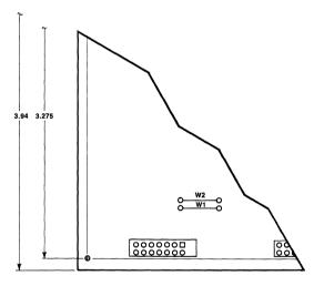
Figure 1. RDAA Module Jumper Selection Location
