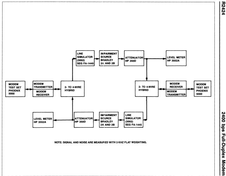
Figure 14. 2-Wire Full-Duplex Bit Error Rate Performance Test Setup (Bidirectional)
