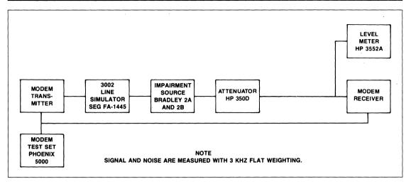
Figure 8. BER Performance Test Set-up
