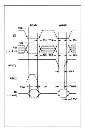
**Microprocessor Interface Timing Waveforms**
