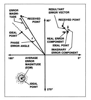
Figure 16. Error Vector Phase Error/EQM
