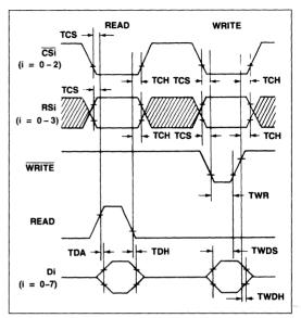
Figure 2. Microprocessor Interface Timing Diagram
