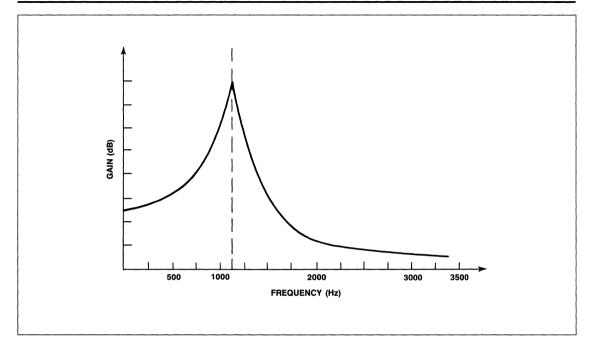
Figure 2. Typical Single Filter Response
