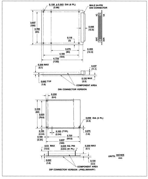
Figure 9. R48DP/208 Modem Dimensions and Pin Locations
