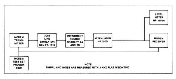
**BER Performance Test Set-up**
