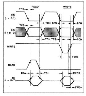
Microprocessor Interface Timing Diagram
