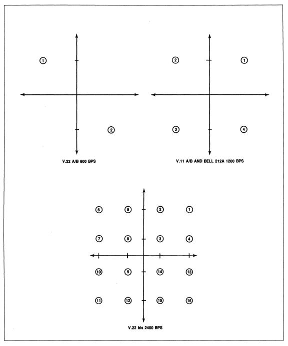
Figure 23. Scaled Signal Points
