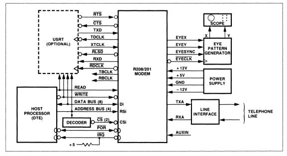
Figure 1. R208/201 Functional Interconnect Diagram
