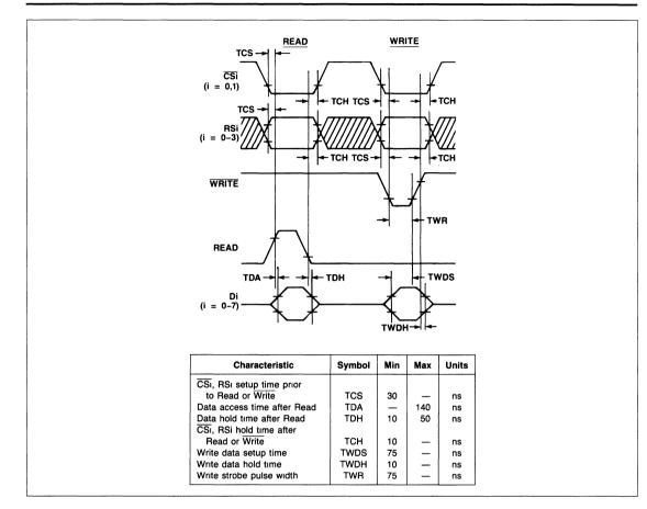
Figure 2. Microprocessor Interface Timing Diagram
