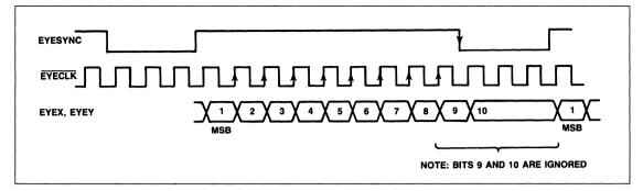
Figure 14. Serial Eye Pattern Signal Timing
