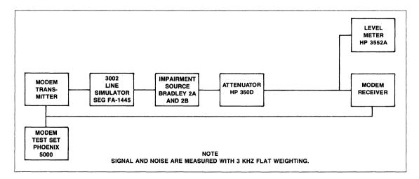
**BER Performance Test Set-up**
