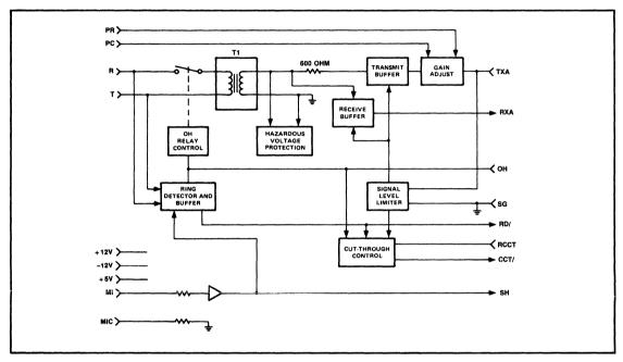
Figure 3. RDAA Functional Block Diagram
