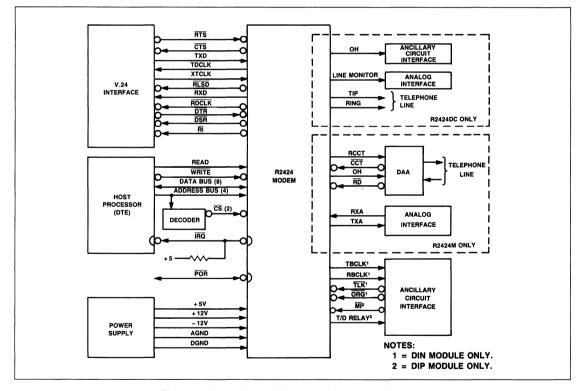
Figure 1. R2424 Modem Functional Interconnect Diagram
