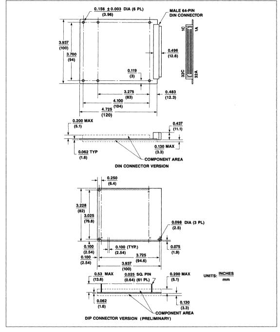
Figure 8. R48DP Modem Dimensions and Pin Locations
