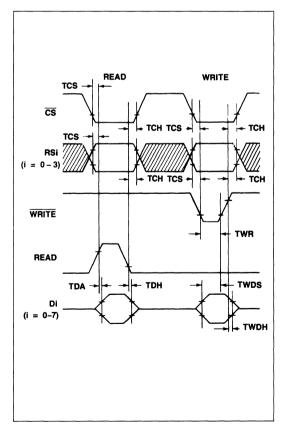
**Microprocessor Interface Timing Waveforms**
