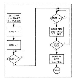
Figure 11. Auto Dial Sequence Flow Diagram
