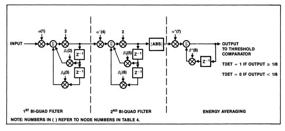
Figure 2. Tone Detector Diagram
