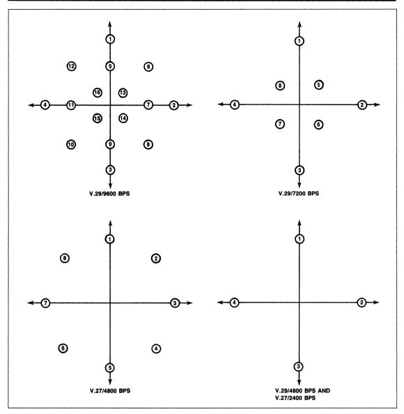
Figure 22. Scaled Signal Points
