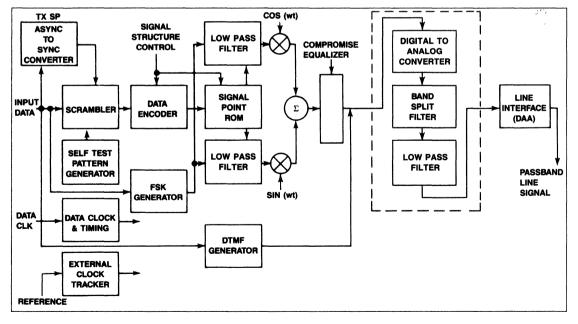
Figure 1. R1212/R2424 Processing Flow Diagram
