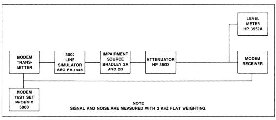
**BER Performance Test Set-up**
