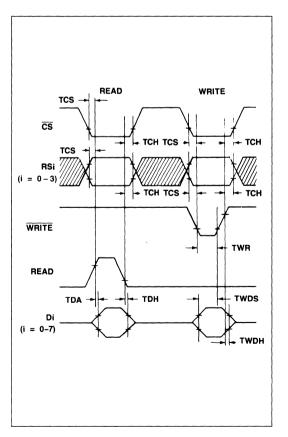
**Microprocessor Interface Timing Waveforms**
