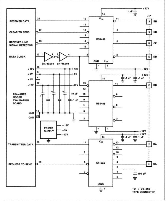
Figure 4. RS-232 Buffer Circuit
