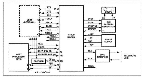
Figure 1. R48DP Functional Interconnect Diagram
