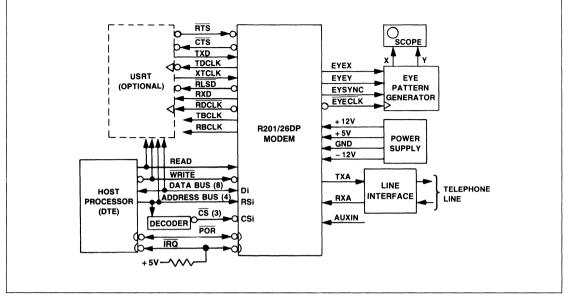
Figure 1. R201/26DP Functional Interconnect Diagram
