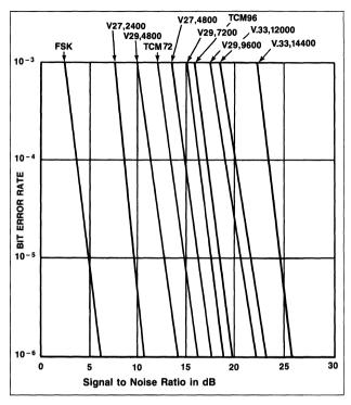
Typical Bit Error Rate (Back-to-Back, Level – 20 dBm)
