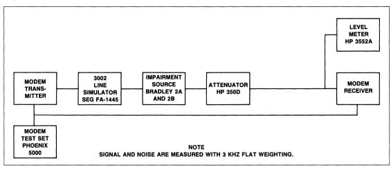
**BER Performance Test Set-up**
