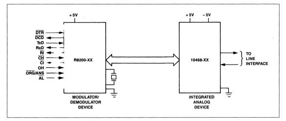
R212DP/DS Modem Device Set Interface Diagram
