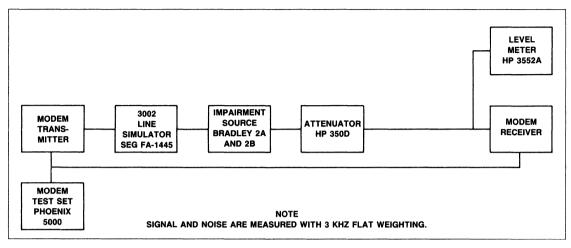
**BER Performance Test Set-up**
