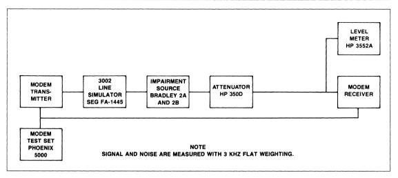
Figure 8. BER Performance Test Set-up
