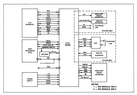
Figure 1. R1212 Modem Functional Interconnect Diagram
