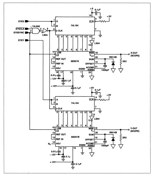
Figure 13. Serial Eye Pattern Generator
