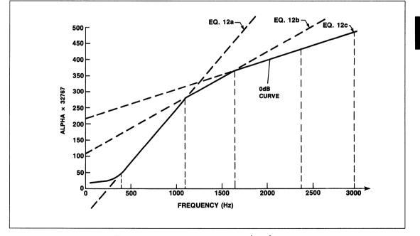
Figure 6.  $\alpha$  versus Center Frequency for  $|H(f_0)| = 0$ dB
