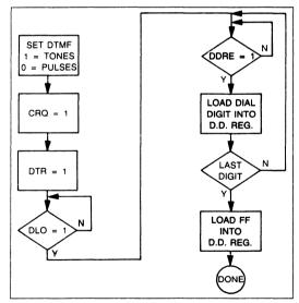
Figure 13. Auto Dial Sequence Flow Diagram
