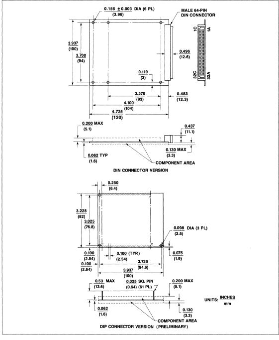
Figure 9. R208/201 Modem Dimensions and Pin Locations
