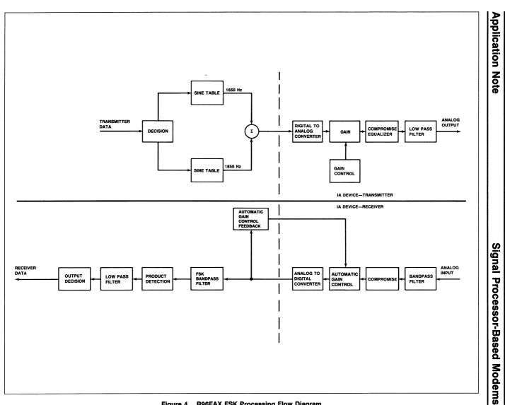
Figure 4. R96FAX FSK Processing Flow Diagram
