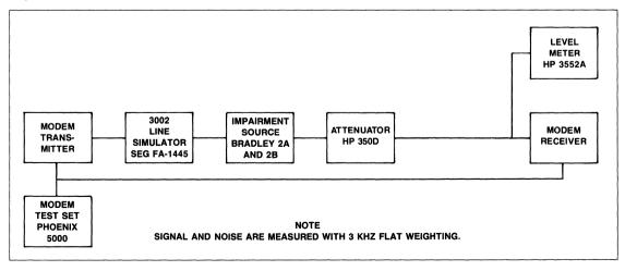
**BER Performance Test Set-up**
