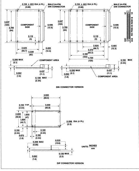
Figure 15. R2424 Modem Dimensions and Pin Locations
