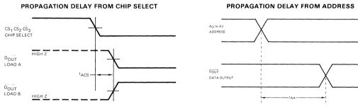
(ALL TIME MEASUREMENTS REFERENCED TO 1.5 V)
