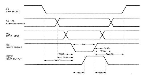
(ALL TIME MEASUREMENTS REFERENCED TO 1.5 V)
