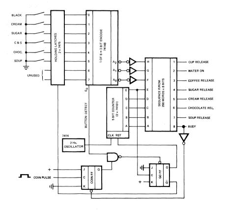
Figure 7. Coffee Machine ROM/Counter Sequencer.
