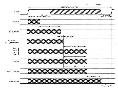
Notes: 1. This delay is the max.  $t_{pd}$  of the register containing A, B, D, and I. For the Am2918, use 13ns.
