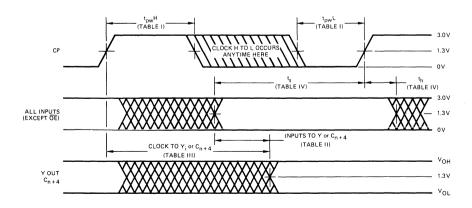
Figure 1. Switching Waveforms. See Tables for Specific Values.
