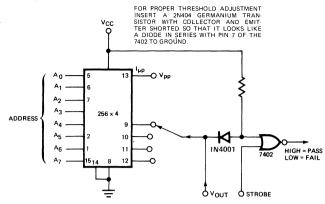
THE 1N4001 DIODE PROTECTS THE INPUT OF THE 7402 FROM THE HIGH PROGRAMMING VOLTAGES
