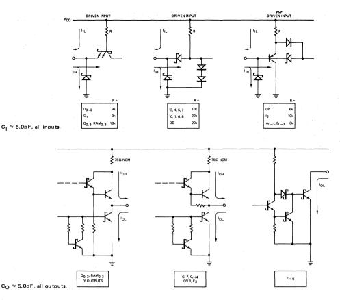
Figure 3. Am2901 Input/Output Current Interface Conditions.
