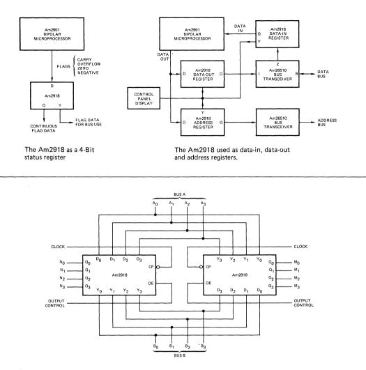
The Am2918 can be connected for bi-directional interface between two buses. The device on the left stores data from the A-bus and drives the A-bus. The device on the right stores data from the B-bus and drives the A-bus. The output control is used to place either or both drivers in the high-impedance state. The contents of each register are available for continuous usage at the N and M ports of the device.
