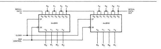
8-Bit serial to parallel converter with three-state output (W) and direct access to the register word (X).
