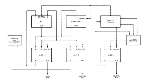
The Am2915 is a universal Bus Transceiver useful for many system data, address, control and timing input/output interfaces.
