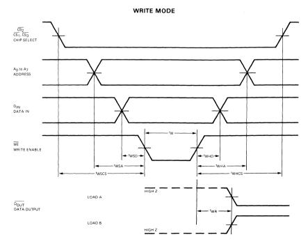
(ALL TIME MEASUREMENTS REFERENCED TO 1.5 V)
