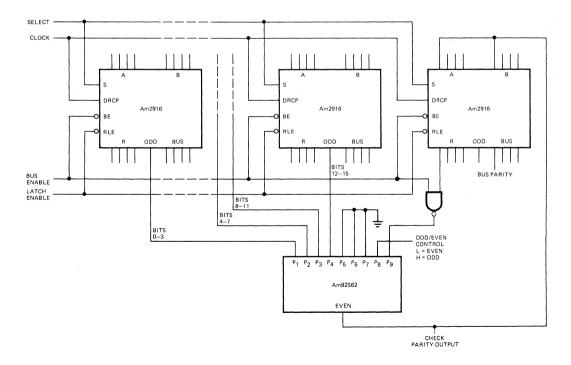
Generating or checking parity for 16 data bits.
