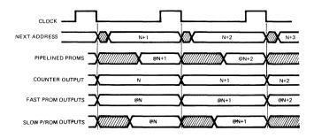
Figure 19. 2909 Sequencer Timing Diagram.
