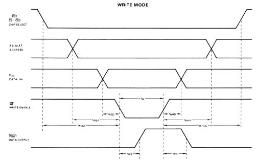
(ALL TIME MEASUREMENTS REFERENCED TO 1.5 V)
