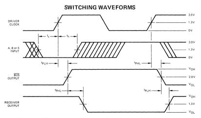
Note: Bus to Reciver output delay is measured by clocking data into the driver register and measuring the  $\overline{\text{BUS}}$  to R combinatorial delay.
