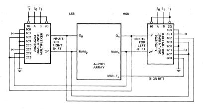
Figure 19. Three-State Multiplexers Used on Shift I/O Lines.
