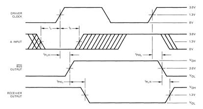
Note: Bus to Receiver output delay is measured by clocking data into the driver register and measuring the BUS to R combinatorial delay.
