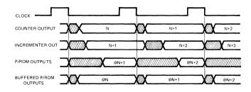
Figure 10. Pipelined Counter /ROM Timing Diagram.
