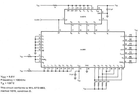
Figure 4. Am2901 Burn-In Circuit.
