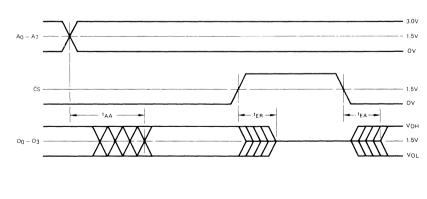
Note: Level on output while  $\overline{\mathsf{E}}$  is HIGH is determined externally.
