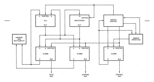
The Am2905 is a universal Bus Transceiver useful for many system data, address, control and timing input/output interfaces.
