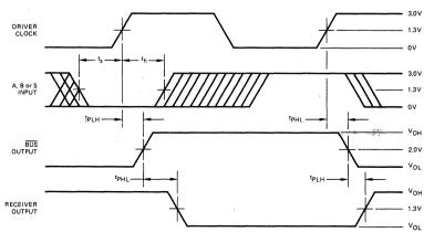
Note: Bus to Receiver output delay is measured by clocking data into the driver register and measuring the  $\overline{\text{BUS}}$  to R combinatorial delay.
