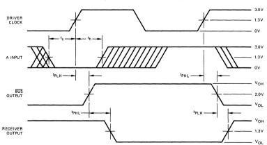
Note: Bus to Reciever output delay is measured by clocking data into the driver register and measuring the BUS to R combinatorial delay.
