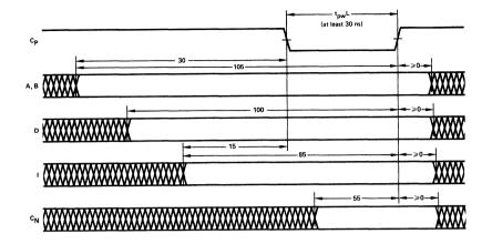
Figure 1. Minimum Cycle Times from Inputs. Numbers Shown are Minimum Data Stable Times for Am2901 DC, in ns. See Table III for Detailed Information.
