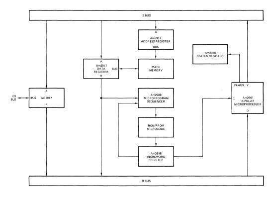
The Am2917 can be used as an I/O Bus Transceiver and Main Memory I/O Transceiver in high-speed Microprocessor Systems.
