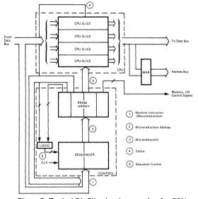
Figure 2. Typical Bit-Slice Implementation for CPU and Control.
