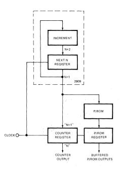
Figure 11. 2909 Pipelined System.
