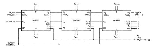
Figure 16. Three Am2901's used to Construct 12-Bit CPU with Ripple Carry. Corresponding A, B, and I Pins on all Devices are Connected Together.
