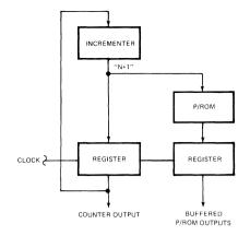
Figure 9. Pipelined Counter /ROM System.
