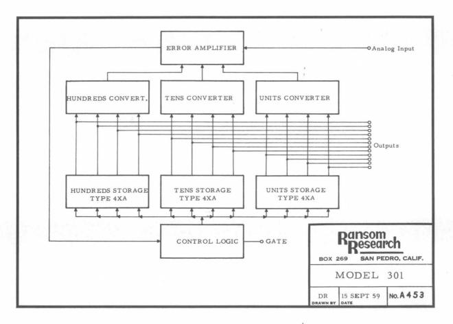
Figure 1. Block Diagram, Model 301 A/D Converter
