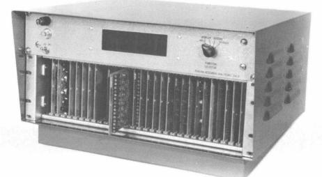
TypicalSeries 300 A/D Converter shown with front panel removed.
