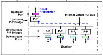
Figure 5-1. System Reset Propagation Example
