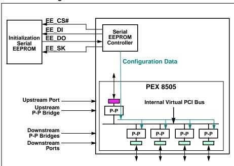
Figure 6-1. Serial EEPROM Connections
