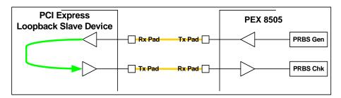
Figure 14-3. Cable Loopback
