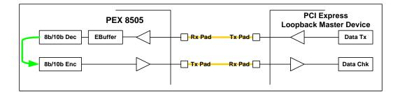
Figure 14-6. Digital Loopback Slave Mode
