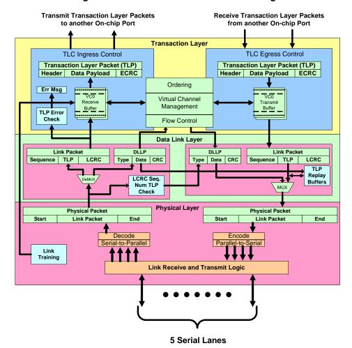
Figure 9-1. Data Formation and Flow Through
