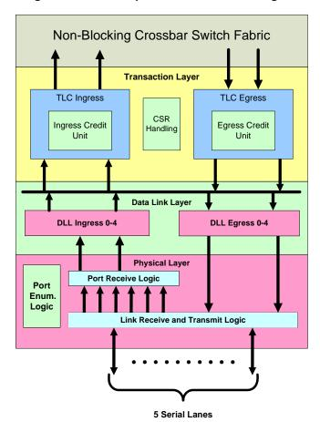
Figure 4-4. PCI Express Station Block Diagram
