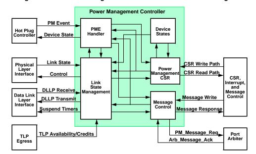
Figure 12-1. Power Management Controller Functional Block Diagram
