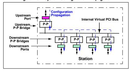
Figure 4-3. System Configuration Propagation
