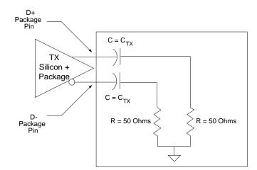
Figure 15-1. Compliance Test/Measurement Load
