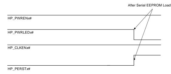
**Note:**  $HP\_PWRLEDx\#$  is not asserted if the serial EEPROM or  $I^2C$  interface clears the Power Indicator Present bit (offset 7Ch[4]) to 0.
