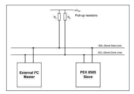
Figure 7-1. Standard Devices to I<sup>2</sup>C Bus Connection Block Diagram
