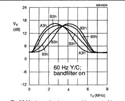
Fig.38 Maximum luminance peaking control in 60 Hz / S-VHS mode as a function of four aperture centre frequencies controllable by subaddress byte 06.
