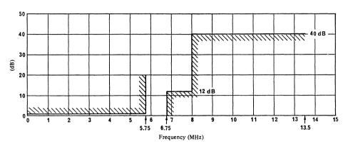
a) Template for insertion loss/frequency characteristic
