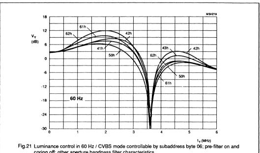
coring off; other aperture bandpass filter characteristics.
