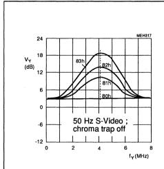
Fig.31 4.1 MHz luminance peaking control control as a function of four different aperture factors controllable by subaddress byte 06; pre-filter off; coring off and bandpass filter on.
