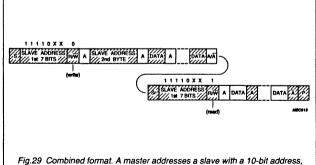
Fig.29 Combined format. A master addresses a slave with a 10-bit address, then transmits data to this slave and reads data from this slave
