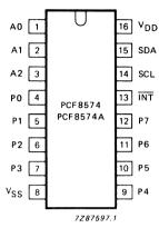
Fig.2 Pinning diagram.
