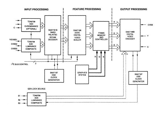
Figure 3. 8-Bit Video Window Graphics with Encoder Gen-Locked to an External Source
