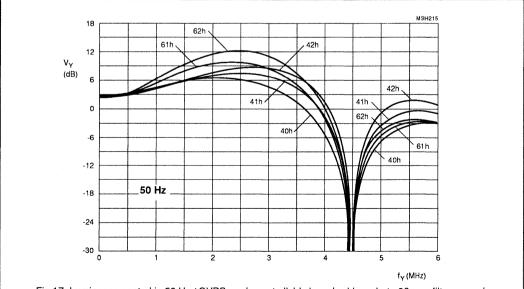
Fig.17 Luminance control in 50 Hz / CVBS mode controllable by subaddress byte 06; pre-filter on and coring off; other aperture bandpass filter characteristics.
