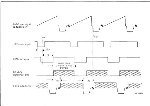
Fig.10 Horizontal timing. t<sub>Rint</sub> = pipeline delay of RAM interface adjustable from -5 to +58 pixel clocks (PIXCLK); t<sub>ofs</sub> = propagation delay of external GENLOCK line adjustable from -17 to +46 pixel clocks.
