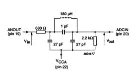
Fig.18 Example of an economical low-pass filter for U and V signals.
