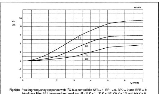
bandpass filter BF1 bypassed and peaking off; (1) K = 1, (2) K = 1/2, (3) K = 1/4 and (4) K = 0.
