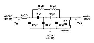
This filter can be adapted to various applications with respect to performance requirements. An input and output impedance of at least 680  $\Omega$  and 2.2 k $\Omega$  respectively must in any event be applied.
