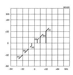
Fig.16 Coring function adjustment by subaddress 06 to affect the bandfilter output signal. The thresholds are related to the 13-bit word width in the luminance processing part and influence the 1LSB to 3LSB (Y0 to Y2) with respect to the 8-bit luminance output
