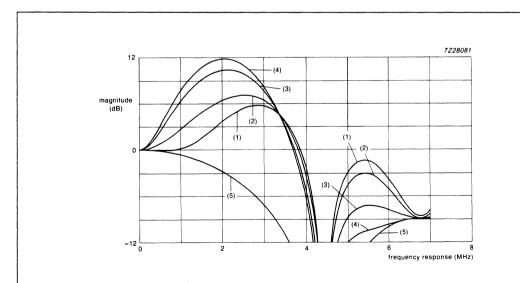
Fig.13 Magnitude of the frequency response of the unlimited summation signal (combining Channel 1 and Channel 2); PAL mode; prefilter OFF; Responses 1 to 5 show various comb-filter combinations programmable by bits BP2 and BP1, via the I<sup>2</sup>C-bus.
