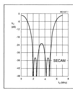
Fig.22 Frequency response of chroma stop filter in colour-difference mode for 50 Hz SECAM.
