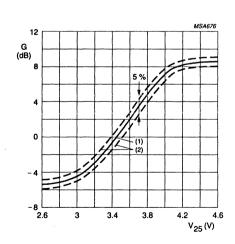
(1)Typical value ( $V_{CCA} = V_{CCD} = 5 \text{ V}$ ;  $T_{amb} = 25^{\circ}\text{C}$ )(2)Minimum and maximum values (temperature and supply)
