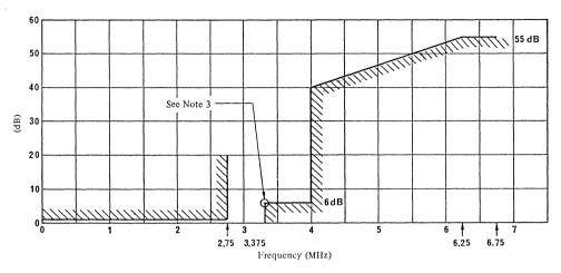
a) Template for insertion loss/frequency characteristic
