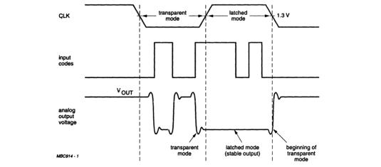
During the transparent mode (CLK = LOW), any change of input data will be seen at the output. During the latched mode (CLK = HIGH), the analog output remains stable regardless of any change at the input. A change of input data during the latched mode will be seen on the falling edge of the clock (beginning of the transparent mode).
