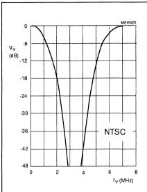
Fig.21 Frequency response of chroma stop filter in colour-difference mode for 60 Hz NTSC. Filter is only active in fast switching mode, but bypassed in RGB mode. The selected filter is dependent on actual detected colour standard.
