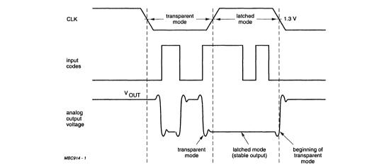
During the transparent mode (CLK = LOW), any change of input data will be seen at the output. During the latched mode (CLK = HIGH), the analog output remains stable regardless of any change at the input. A change of input data during the latched mode will be seen on the falling edge of the clock (beginning of the transparent mode).
