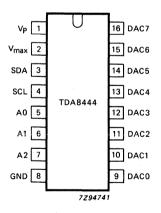
Fig. 2 Pinning diagram.
