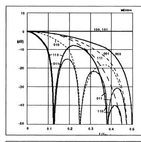
Fig.27 Horizontal frequency characteristic of luminance signal (Y) dependent on HF2 to HF0 bits (subaddress 24).
