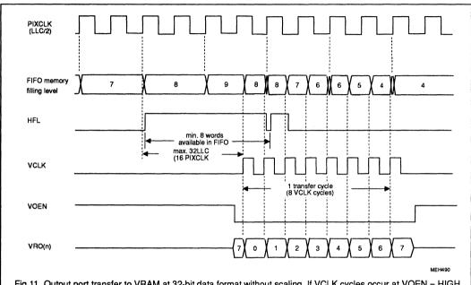
Fig.11 Output port transfer to VRAM at 32-bit data format without scaling. If VCLK cycles occur at VOEN = HIGH, the FIFO register is unchanged, but the outputs VRO(31-0) remain in 3-state position.
