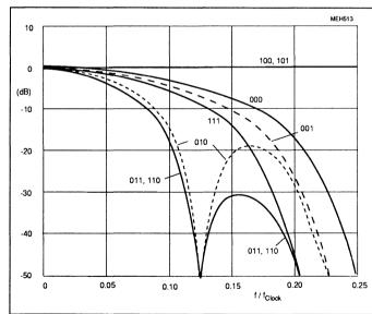
Fig.14 Horizontal frequency characteristic of chrominance signals (UV) without UV interpolation dependent on HF2 to HF0 bits (subaddress 04).
