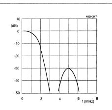
Fig.5 Overall transfer characteristics 4:1:1 input data.
