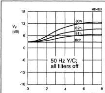
Fig.35 4.1 MHz luminance peaking control in 50 Hz / S-VHS mode as a function of four different aperture factors controllable by subaddress byte 06.
