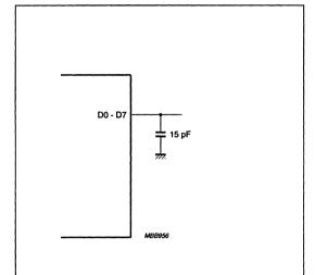
Fig.7 Load circuit for timing measurement.
