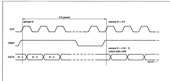
When the HREF period is a whole multiple of 4 clock periods, the output data is valid without any clock delay. The internal circuit always gives an internal delay of 4 clock periods as illustrated in Fig.5.
