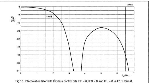
Fig.10 Interpolation filter with I<sup>2</sup>C-bus control bits IFF = 0; IFC = 0 and IFL = 0 in 4:1:1 format, and control bits IFF = 1; IFC = 0 and IFL = 0 in 4:2:2 format; 13.5 MHz data rate.
