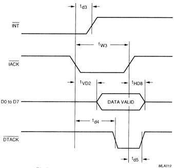
Fig.8 Interrupt timing; 68000-mode.
