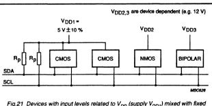
Fig.21 Devices with input levels related to  $V_{DD}$  (supply  $V_{DD1}$ ) mixed with fixed input level devices (supply  $V_{DD2,3}$ ) on the  $l^2C$ -bus
