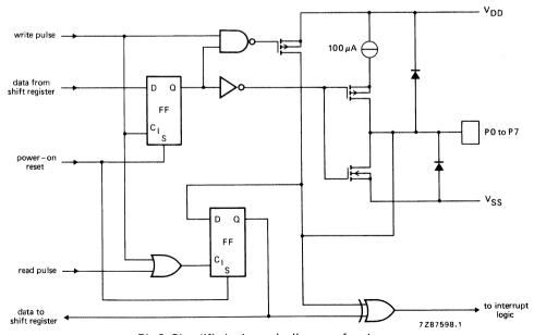
Fig.3 Simplified schematic diagram of each port.
