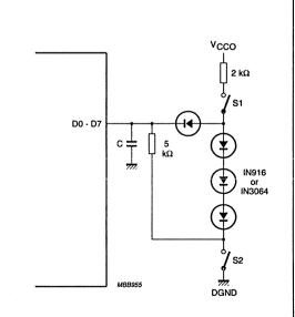
Fig.6 Load circuit for timing measurement; 3-state outputs ( $\overline{CE}$ :  $f_i = 1$  MHz;  $V_{Vi} = 3$  V); see Table 3.
