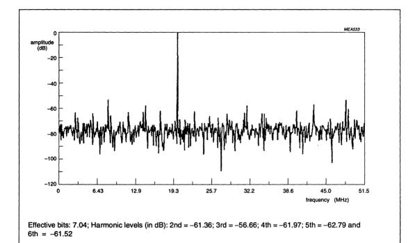
Fig.12 Fast fourier transformer ( $f_{CLK} = 100 \text{ MHz}$ ;  $f_i = 20 \text{ MHz}$ ).
