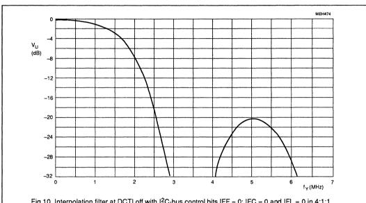
Fig.10 Interpolation filter at DCTI off with  $I^2C$ -bus control bits IFF = 0; IFC = 0 and IFL = 0 in 4:1:1 format and control bits IFF = 1; IFC = 0 and IFL = 0 in 4:2:2 format; 13.5 MHz data rate.
