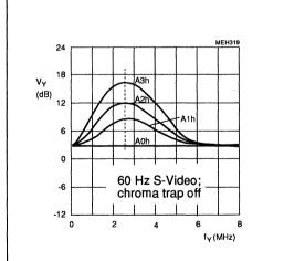
Fig.34 2.6 MHz luminance peaking control control as a function of four different aperture factors controllable by subaddress byte 06; pre-filter off; coring off and bandpass filter on.
