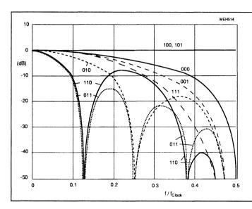
Fig. 13 Horizontal frequency characteristic of luminance signal (Y) dependent on HF2 to HF0 bits (subaddress 04).
