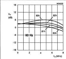
Fig.24 Luminance control in 60 Hz / S-VHS mode controllable by subaddress byte 06; pre-filter off and coring off; different aperture bandpass ffilter characteristics.
