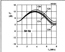
Fig.24 Luminance control in 50 Hz / S-VHS mode controllable by subaddress byte 06; pre-filter on and coring off; different aperture bandpass filter characteristics.
