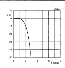
Fig.7 Overall transfer characteristics 4:4:4 input data (SCBW-bit = 1).
