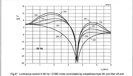
coring off; maximum and minimum aperture bandpass filter characteristics.
