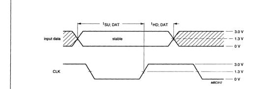
The shaded areas indicate when the input data may change and be correctly registered. Data input update must be completed within 0.3 ns after the first rising edge of the clock ( $t_{SU;DAT}$  is negative; -0.3 ns). Data must be held at least 2 ns after the rising edge ( $t_{HD;DAT}$  = +2 ns).
