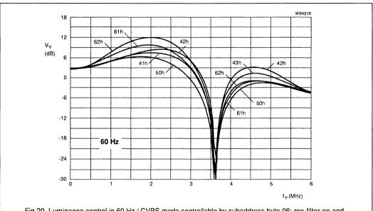
Fig.20 Luminance control in 60 Hz / CVBS mode controllable by subaddress byte 06; pre-filter on and coring off; other aperture bandpass filter characteristics.
