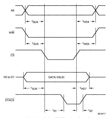
Fig.6 Bus timing; 68000-mode write cycle.
