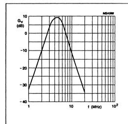
Fig.5 Band pass filter nominal frequency response (PAL mode).
