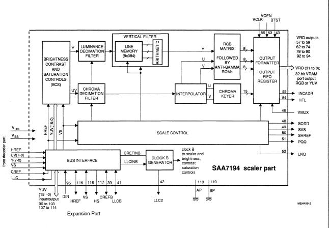
Fig.1(b) Block diagram of brightness, contrast, saturation controls and scaler part; (continued from Fig.1(a)).
