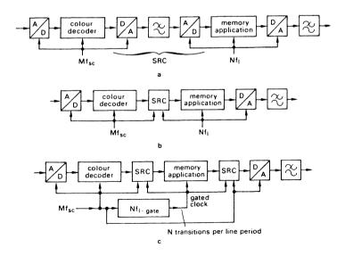
Fig. 1. Application of sample rate converters: a. anolog sample rate converter, b. digital sample rate converter and two clocks coupled to video signal, c. two digital sample rate converters and single clock.
