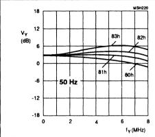
Fig.23 Luminance control in 50 Hz / S-VHS mode controllable by subaddress byte 06; pre-filter off and coring off; different aperture bandpass filter characteristics.
