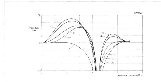
Fig.14 Magnitude of the frequency response of the unlimited summation signal (combining Channel 1 and Channel 2); PAL mode; prefilter ON; Responses 1 to 5 show various comb-filter combinations programmable by bits BP2 and BP1, via the I<sup>2</sup>C-bus.
