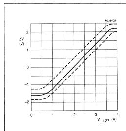
Fig.5 Difference between black level and measuring level at the RGB outputs (AV) as a function of the brightness control input voltage  $(V_{11})$ .
