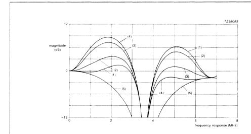
Fig.15 Magnitude of the frequency response of the unlimited summation signal (combining Channel 1 and Channel 2); NTSC mode; prefilter OFF; Responses 1 to 5 show various comb-filter combinations programmable by bits BP2 and BP1, via the I<sup>2</sup>C-bus.
