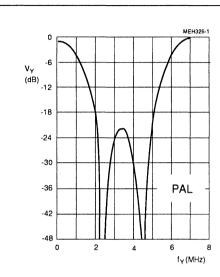
Fig.20 Frequency response of chroma stop filter in colour-difference mode for 50 Hz PAL. Filter is only active in fast switching mode, but bypassed in RGB mode. The selected filter is dependent on actual detected colour standard.
