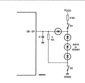
Fig.9 Load circuit for timing measurement; 3-state outputs (OF:  $f_i = 1 \text{ MHz}$ ;  $V_{OF} = 3 \text{ V}$ ).
