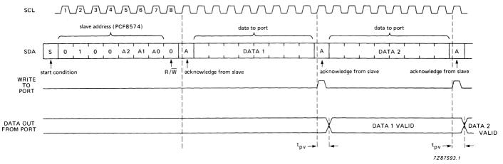
Fig. 10 WRITE mode (output port).
