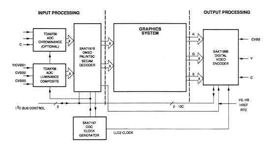
Figure 5. RTC Genlock Mode (Uses Single CGC)
