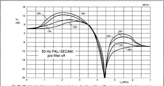
Fig.25 Maximum luminance peaking control as a function of <u>four different aperture centre frequencies</u> controllable by subaddress byte 06; aperture factor 1; coring off; chroma trap on; pre-filter off; and bandfilter on.
