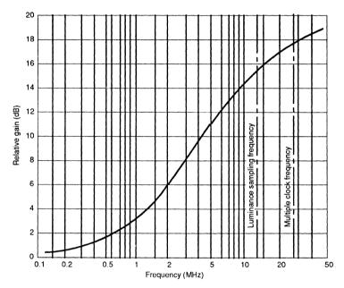
FIGURE 5 — Line receiver equalization characteristic for small signals
