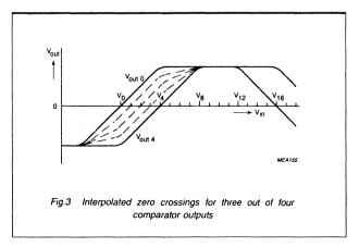
By using this interpolation technique, three out of every four comparators are eliminated, thereby reducing the number required for an 8-bit folding and interpolating ADC from 255 to 64. The interpolation technique also reduces the number of taps required on the precision reference resistor ladder from 255 to 64 and reduces the number of folding amplifiers required from 16 to 4.
