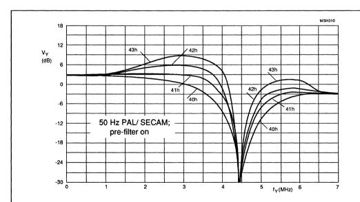
Fig.24 3.8 MHz luminance peaking control as a function of <u>four different aperture factors</u> controllable by subaddress byte 06; coring off; chroma trap on; pre-filter on and bandfilter on.
