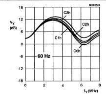
Fig.25 Luminance control in 60 Hz / S-VHS mode controllable by subaddress byte 06; pre-filter on and coring off; different aperture bandpass filter characteristics.
