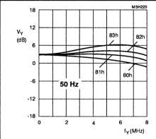
Fig.22 Luminance control in 50 Hz / S-VHS mode controllable by subaddress byte 06; pre-filter off and coring off; different aperture bandpass filter characteristics.
