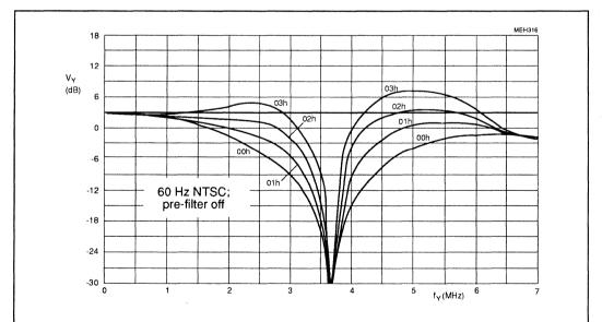
Fig.30 4.1 MHz luminance peaking control as a function of <u>four different aperture factors</u> controllable by subaddress byte 06; coring off; chroma trap on; pre-filter off and bandfilter on.
