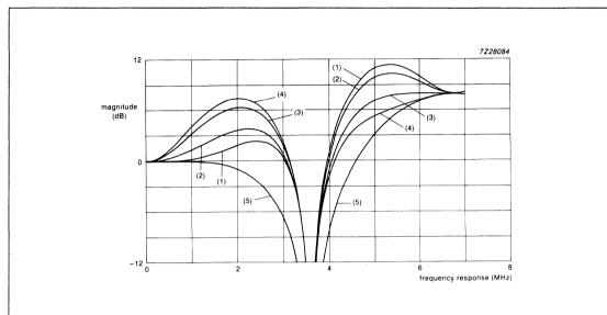
Fig.16 Magnitude of the frequency response of the unlimited summation signal (combining Channel 1 and Channel 2); NTSC mode; prefilter ON; Responses 1 to 5 show various comb-filter combinations programmable by bits BP2 and BP1, via the I<sup>2</sup>C-bus.
