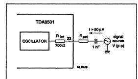
Fig.11 Tuning circuit for external signal source.
