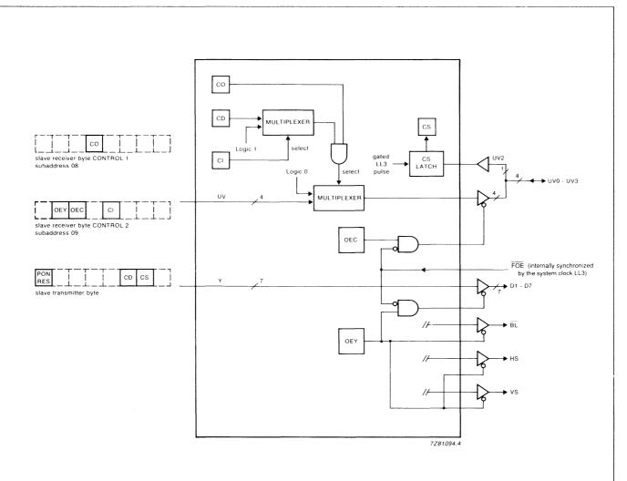
Fig.6 Schematic diagram of control signals at the output interface.
