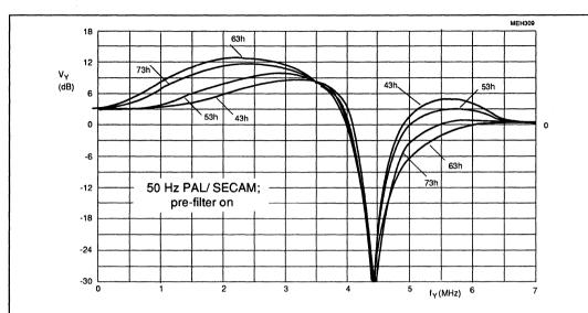
Fig.23 Maximum luminance peaking control as a function of <u>four different aperture centre frequencies</u> controllable by subaddress byte 06; aperture factor 1; coring off; chroma trap on; pre-filter on; and bandfilter on.
