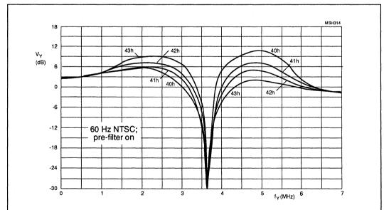
Fig.28 3.8 MHz luminance peaking control as a function of <u>four different aperture factors</u> controllable by subaddress byte 06; coring off; chroma trap on; pre-filter on and bandfilter on.
