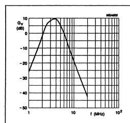
Fig.7 Band pass filter nominal frequency response (NTSC mode).
