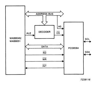
Fig.11 Application diagram using the MAB8048/MAB8051.
