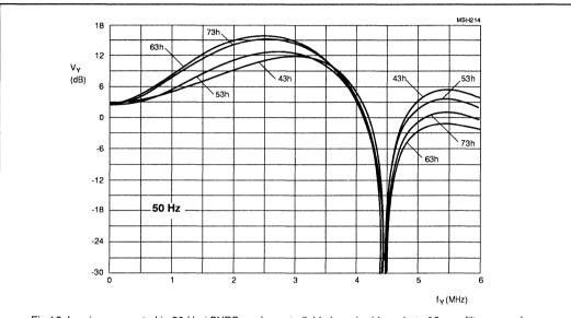
Fig.16 Luminance control in 50 Hz / CVBS mode controllable by subaddress byte 06; pre-filter on and coring off; maximum aperture bandpass filter characteristic.
