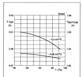
Fig.3 Influence of ambient temperature on  $V_{TOP}$  and  $V_{BOTTOM}$  under 5 V supply.
