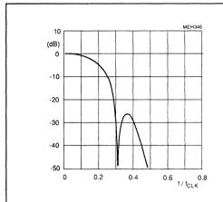
Fig.4 Transfer characteristics of 4:4:4 to 4:2:2 decimator.
