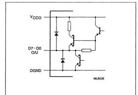
Fig.7 TTL data and overflow/underflow outputs.
