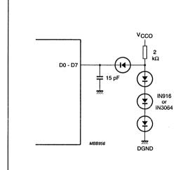
Fig.5 Load circuit for timing measurement; data outputs ( $\overline{CE} = LOW$ ).
