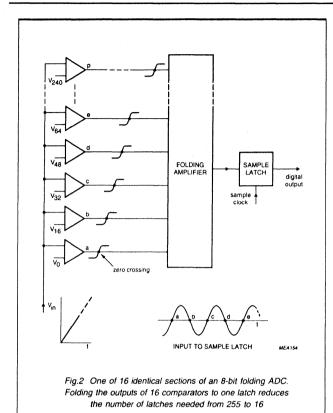
and chip area for this ADC configuration are also considerably reduced, its overall performance actually improves. Furthermore, since it has only 16 connections between the analog and digital circuitry instead of 255, kick-back noise is much reduced.
