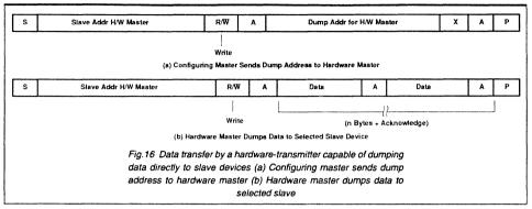
transmitter is set in the slavereceiver mode after the system reset. In this way, a system configuring master can tell the hardware master-transmitter (which is now in slave-receiver mode) to which address data must be sent (Fig.16). After this programming procedure, the hardware master remains in the master-transmitter mode.
