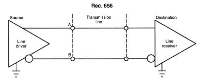
FIGURE 3 - Line driver and line receiver interconnection
