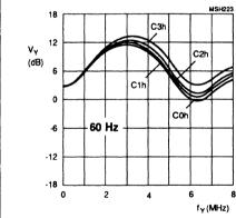
Fig.26 Luminance control in 60 Hz / S-VHS mode controllable by subaddress byte 06; pre-filter on and coring off; different aperture bandpass filter characteristics.
