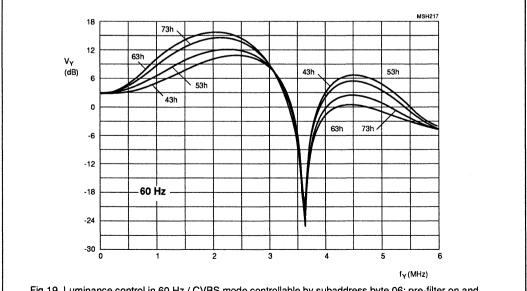
Fig.19 Luminance control in 60 Hz / CVBS mode controllable by subaddress byte 06; pre-filter on and coring off; maximum aperture bandpass filter characteristic.
