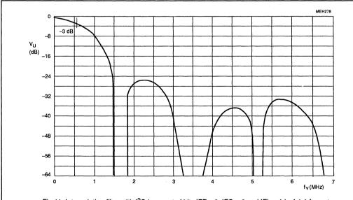
Fig.11 Interpolation filter with I<sup>2</sup>C-bus control bits IFF = 0; IFC = 0 and IFL = 1 in 4:1:1 format, and control bits IFF = 1; IFC = 0 and IFL = 1 in 4:2:2 format; 13.5 MHz data rate.
