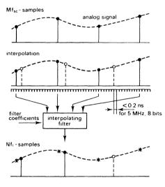
Fig. 2. Principle of sample rate conversion.
