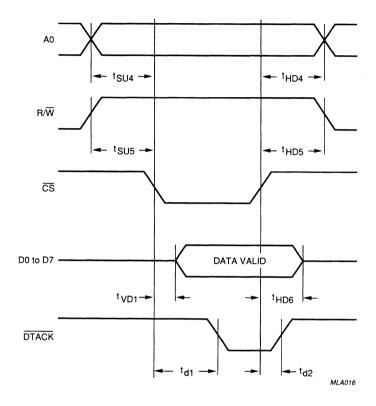
Fig.5 Bus timing; 68000-mode read cycle.
