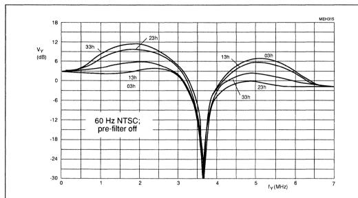
Fig.29 Maximum luminance peaking control as a function of <u>four different aperture centre frequencies</u> controllable by subaddress byte 06; aperture factor 1; coring off; chroma trap on; pre-filter off; and bandfilter on.
