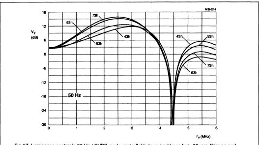
Fig.17 Luminance control in 50 Hz / CVBS mode controllable by subaddress byte 06; pre-filter on and coring off; maximum aperture bandpass filter characteristic.
