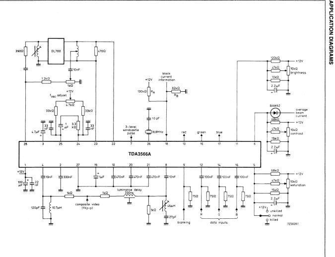
Fig.8 Application diagram showing the TDA3566A for a PAL decoder.
