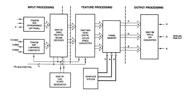
Figure 2. 8-Bit RGB Frame Buffer with Analog RGB Output
