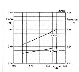
Fig.4 Influence of supply voltage on  $V_{\text{TOP}}$  and  $V_{\text{BOTTOM}}$  under 25 °C ambient temperature.
