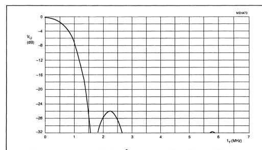
Fig.11 Interpolation filter at DCTI off with  $I^2C$ -bus control bits IFF = 0; IFC = 0 and IFL = 1 in 4:1:1 format and control bits IFF = 1; IFC = 0 and IFL = 1 in 4:2:2 format; 13.5 MHz data rate.
