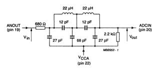
This filter can be adapted to various applications with respect to performance requirements. An input and output impedance of at least 680  $\Omega$  and 2.2 k $\Omega$  respectively must in any event be applied.
