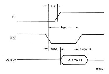
Fig.7 Interrupt timing; 80XX-mode.
