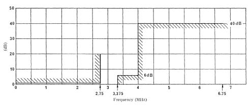
a) Template for insertion loss/frequency characteristic
