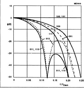
Fig.28 Horizontal frequency characteristic of chrominance signals (UV) without UV interpolation dependent on HF2 to HF0 bits (subaddress 24).
