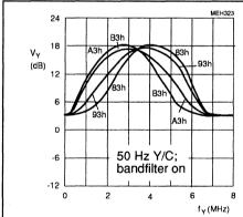
Fig.37 Maximum luminance peaking control in 50 Hz / S-VHS mode as a function of four aperture centre frequencies controllable by subaddress byte 06.
