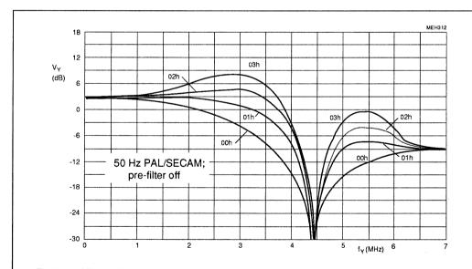
Fig.26 4.1 MHz luminance peaking control as a function of <u>four different aperture factors</u> controllable by subaddress byte 06; coring off; chroma trap on; pre-filter off and bandfilter on.
