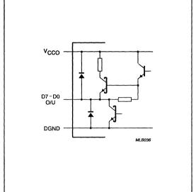
Fig.8 TTL data and overflow/underflow outputs.
