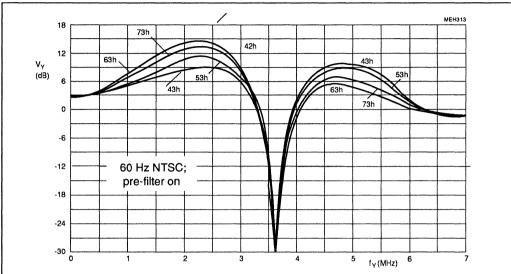
Fig.27 Maximum luminance peaking control as a function of <u>four different aperture centre frequencies</u> controllable by subaddress byte 06; aperture factor 1; coring off; chroma trap on; pre-filter on; and bandfilter on.
