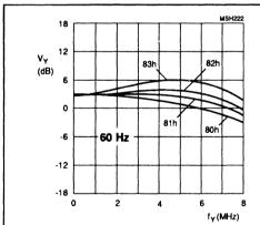
Fig.25 Luminance control in 60 Hz / S-VHS mode controllable by subaddress byte 06; pre-filter off and coring off; different aperture bandpass ffilter characteristics.
