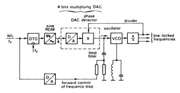
Fig. 10. Analog PLL as reconstruction filter.
