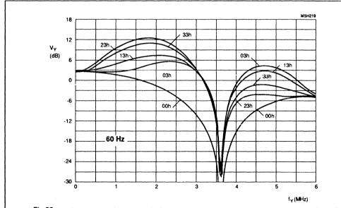
Fig.22 Luminance control in 60 Hz / CVBS mode controllable by subaddress byte 06; pre-filter off and coring off; maximum and minimum aperture bandpass filter characteristics.
