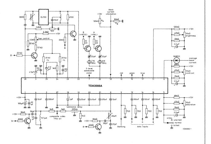
Fig.9 Application diagram showing the TDA3566A for a PAL/NTSC decoder.
