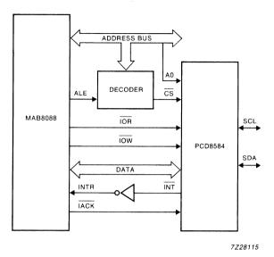
Fig.13 Application diagram using the 8088.
