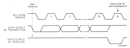
Fig.7 Acknowledgement on the I<sup>2</sup> C-bus.
