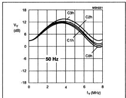
Fig.23 Luminance control in 50 Hz / S-VHS mode controllable by subaddress byte 06; pre-filter on and coring off; different aperture bandpass filter characteristics.
