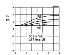
Fig.36 4.1 MHz luminance peaking control in 60 Hz / S-VHS mode as a function of four different aperture factors controllable by subaddress byte 06.
