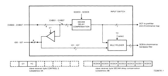
Fig.5 Schematic diagram of the input switch.
