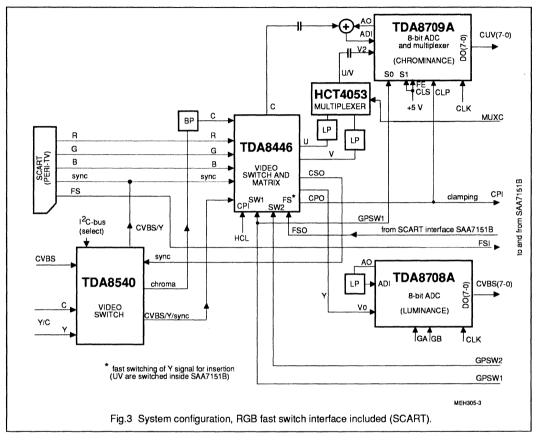
The SECAM signals are fed after de-emphasis to a cross-over switch, to provide the both serial-transmitted colour-difference signals. These signals are finally fed via the fast switch to the output formatter stages and to the output interface. Chrominance signals are output in parallel (4:2:2) on the YUV-bus. The data rate of Y signal (pixel rate) is 13.5 MHz. UV signals have a data rate of 13.5 MHz/2 for the 4:2.2 format (Table 2) respectively 13.5 MHz/4 for the 4:1.1 format (Table 3)
