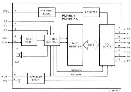
Fig.1 Block diagram.
