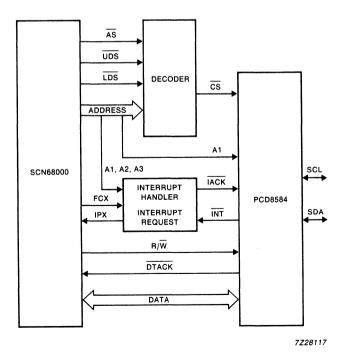
Fig.12 Application diagram using the SCN68000.
