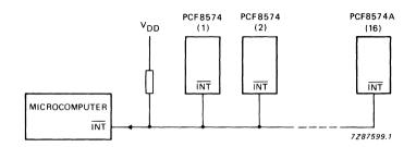
Fig. 12 Application of multiple PCF8574s with interrupt.
