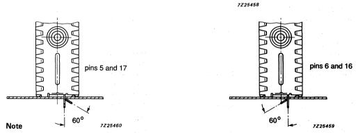
In order to prevent any stress to the printed-wiring board, the tuner should be supported at its aerial connector.
