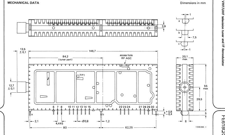
Fig. 3 Unless otherwise stated the tolerance is  $\pm$  0,05 mm.
