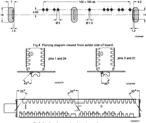
Fig.5 Bending of connecting pins and mounting tags.
