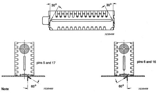
In order to prevent any stress to the printed-wiring board, the tuner should be supported at its aerial connector.
