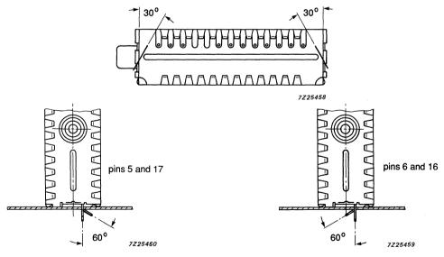
Note: In order to prevent any stress to the printed-wiring board, the tuner should be supported at its aerial connector.
