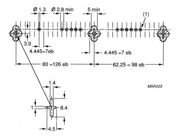
Fig.2 Piercing diagram viewed from solder side of board.
