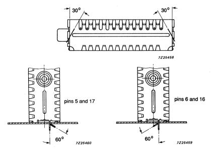
**Note:** In order to prevent any stress to the printed-wiring board, the tuner should be supported at its aerial connector.
