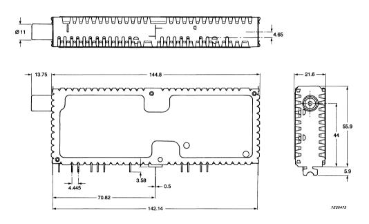
Fig. 3 Mechanical detail.
