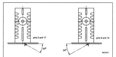
To prevent any stress on the PWB set, it is recommended to support the tuner at the aerial connector.
