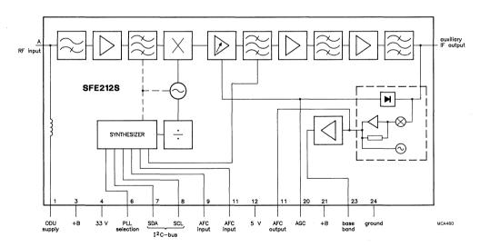
Fig.2 SFE212S block diagram.
