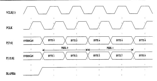
Figure 9.25 - DAC Interface - Attribute Mode 6 (32bpp, 16-bit port)
