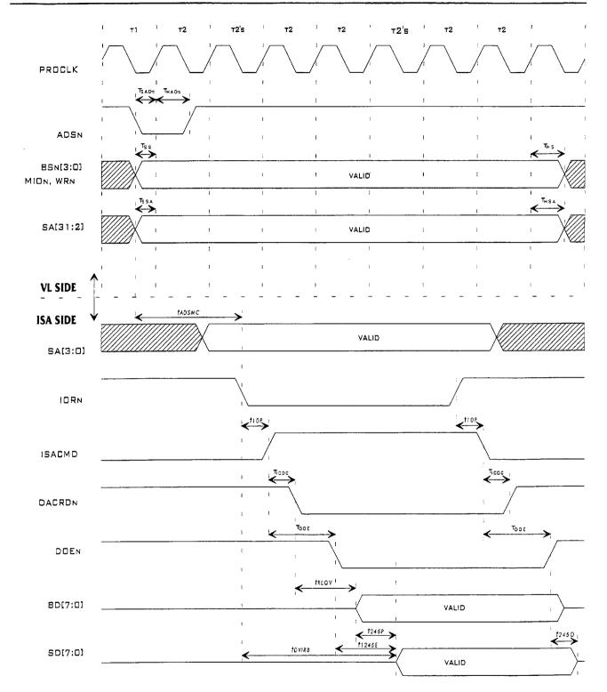
Figure 9.7 - VL DAC I/O Read Timing
