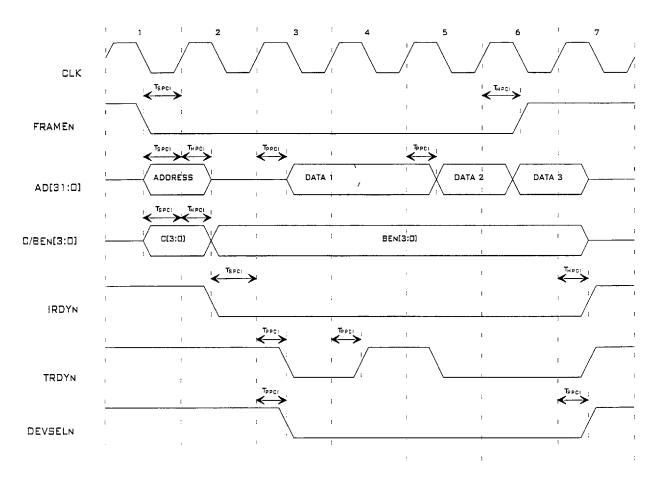
Figure 9.10 - PCI Bus Timing (Read Operation)
