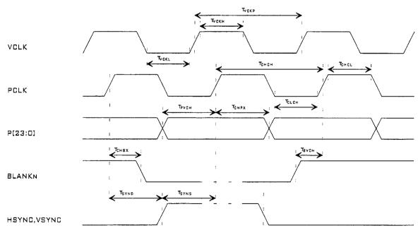
Figure 9.16 - DAC Pixel Port Interface Timing
