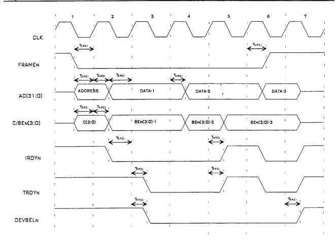
Figure 9.11 - PCI Bus Timing (Write Operation)
