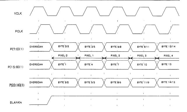
Figure 9.26 - DAC Interface - Attribute Mode 7 (24bpp, 24-bit port)
