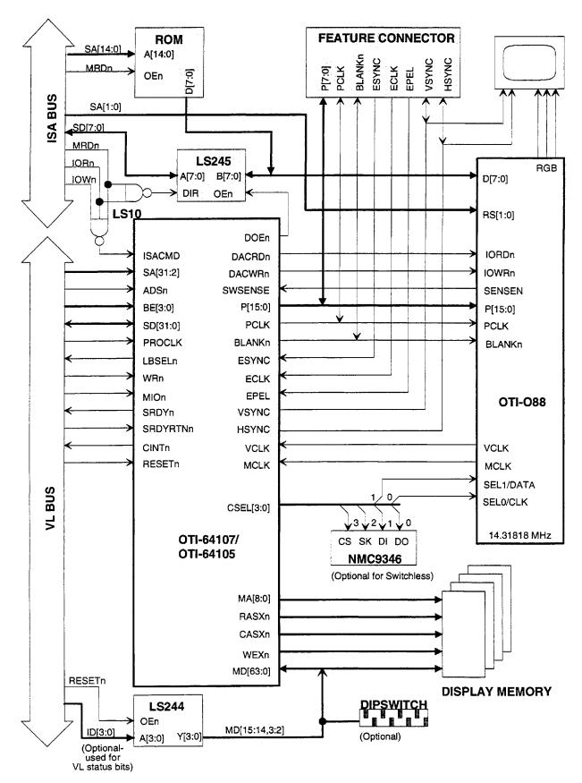
Figure 2.1 - VL Bus Block Diagram using OTI-088 ClkDAC
