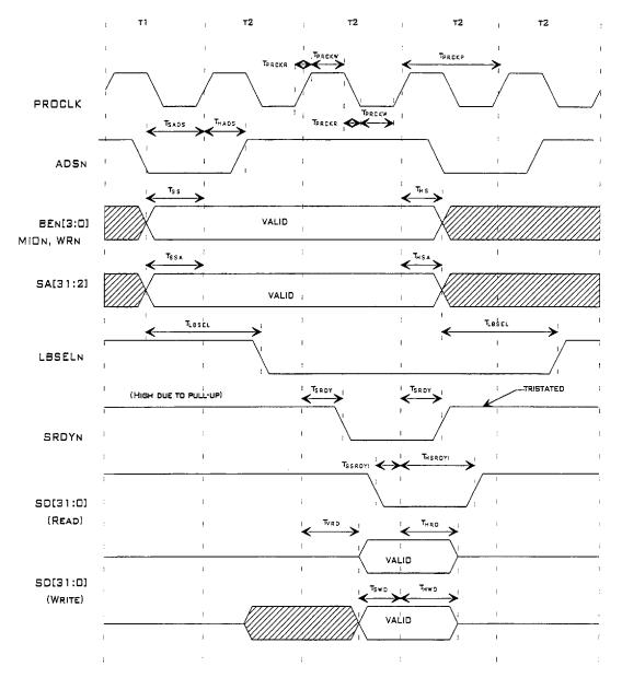
Figure 9.5 - VL Bus Interface Timing
