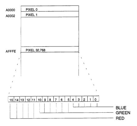
This figure shows the 16-bit (65,536 colors) Direct-color, Packed-pixel Mode organization. The RGB color information is stored in a 5-6-5 format comprising 5-bits of RED, 6-bits of GREEN, and 5-bits of BLUE. The color information (per pixel) is read from Display Memory, and used by the internal Palette DAC in Direct-color Mode to display 65,536 colors simultaneously.
