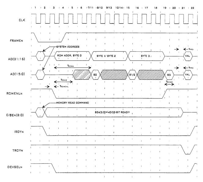
Figure 9.14 - PCI ROM Read Timing
