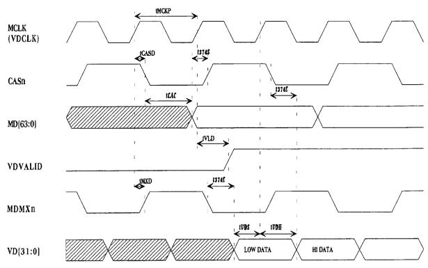
Figure 9.31 - Multimedia Output Port (Video Window) Timing - MD64
