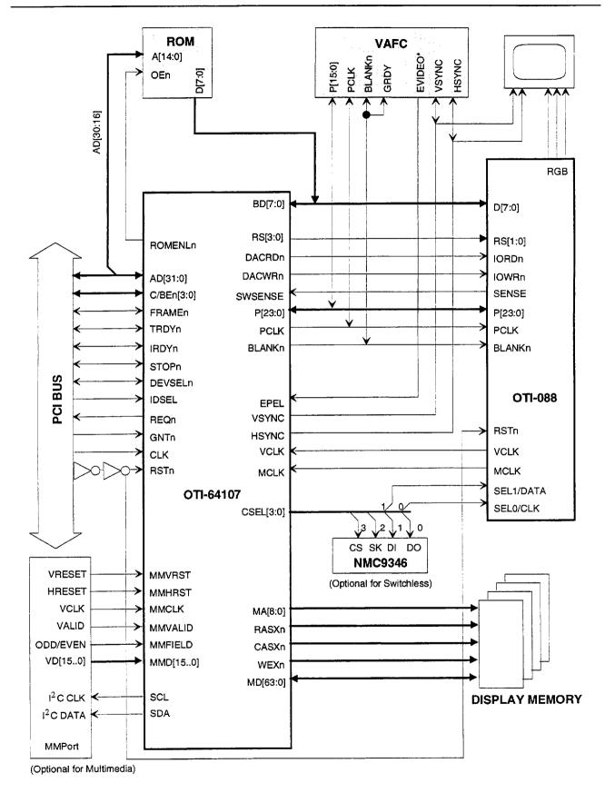
Figure 4.3 - Block Diagram of the Multi-Media Port and the VAFC using OTI-088 ClkDAC and PCI Bus (Glueless)
