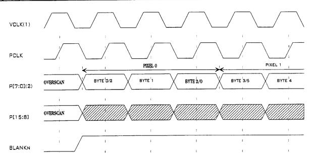
Figure 9.21 - DAC Interface - Attribute Mode 2C (24bpp, 8-bit port)
