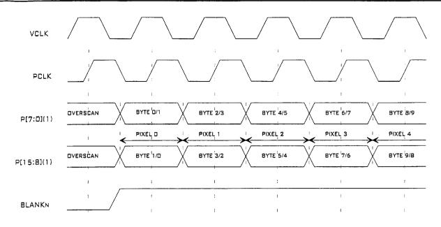
Figure 9.24 - DAC Interface - Attribute Mode 5 (15/16bpp, 16-bit port)
