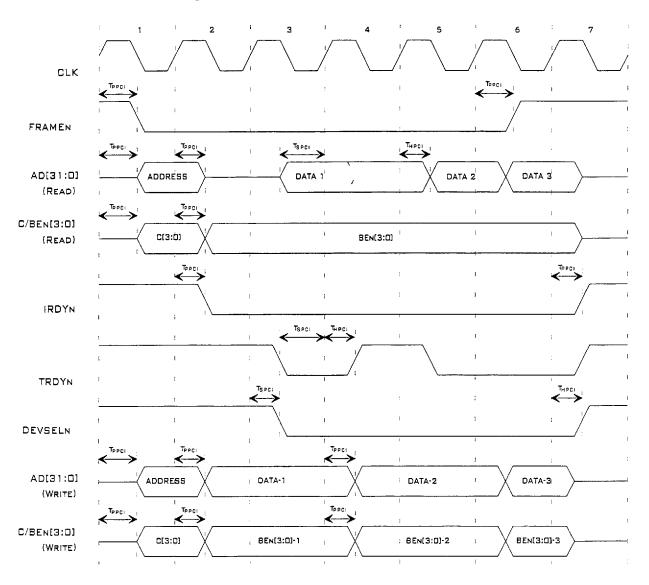
Figure 9.13 - PCI Bus Master Read/Write Timing
