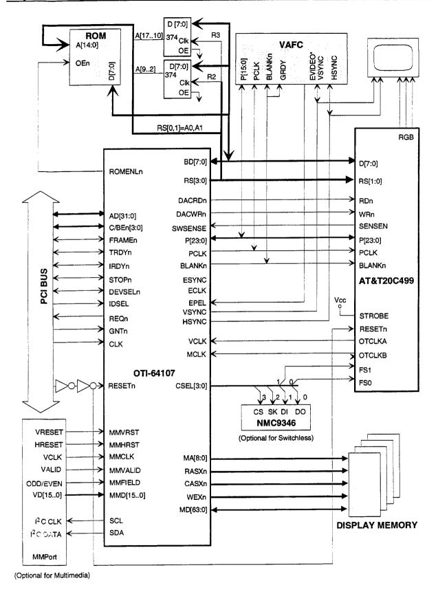
Figure 4.4 - Block Diagram of the Multi-Media Port and the VAFC using AT&T20C499 Precision DAC™ and PCI Bus (Glueless)
