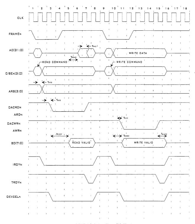
Figure 9.15 - PCI DAC & Auxiliary I/O Timing
