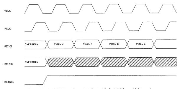
Figure 9.19 - DAC Interface - Attribute Mode 2A (8bpp, 8-bit port)
