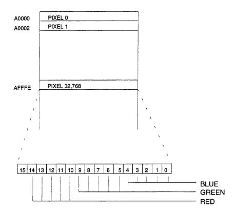
The figure shows the 15-byte (32,768 colors) Direct-color, Packed-pixel Mode organization. The RGB color information is stored in 5-5-5 format, and the MSB (Bit 15) is ignored. Two bytes per pixel are used for storing the color information. The CPU addressing is completely sequential. The 5-5-5 format represents most-significant bits of RED, GREEN, and BLUE of the 24-bit DAC output.
