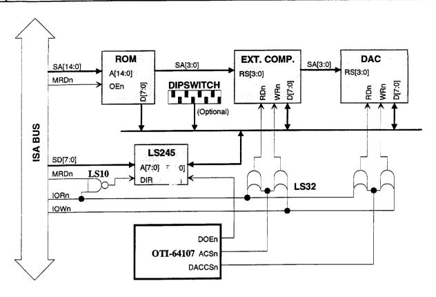
Figure 4.5 - Auxi ry I/O on VL Bus (via ISA Bus)
