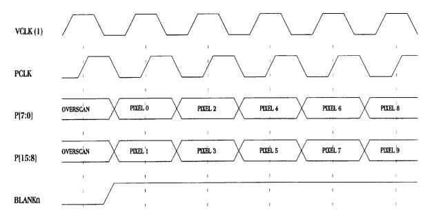
Figure 9.23 - DAC Interface - Attribute Mode 4 (8bpp, 16-bit port)
