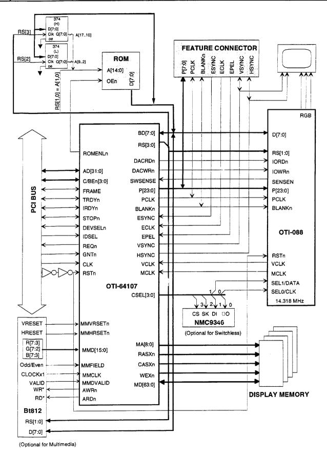
Figure 2.4 - PCI Bus Block Diagram (compliant) with the Multimedia Port
