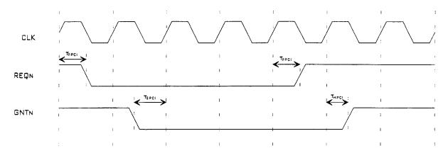
Figure 9.12 - PCI Bus Master Request Timing
