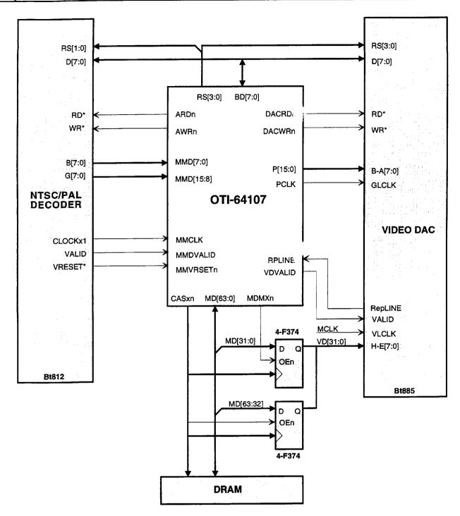
Figure 4.2 - Block Diagram of the Multi-Media Port with the Brooktree Bt885 Video DAC on the VL Bus
