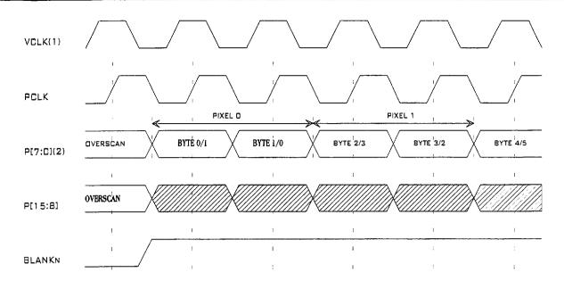
Figure 9.20 - DAC Interface - Attribute Mode 2B (15/16bpp, 8-bit port)
