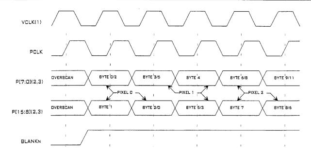
Figure 9.22 - DAC Interface - Attribute Mode 3 (24bpp, 16-bit port)
