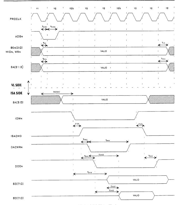
Figure 9.8 - VL DAC I/O Write Timing
