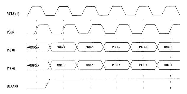
Figure 9.18 - DAC Interface - Attribute Mode 1 (4bpp, 8-bit port)
