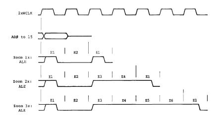
Figure 2.3 Zoom Magnified Display Cycles
