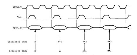
Figure 2.10 Mixed Mode Display Addressing, DAD
