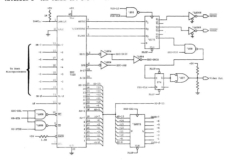
Figure B.1 One-Plane System, Part A
