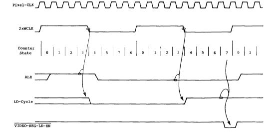
Figure 2.6 Video Register Load Timing Diagram
