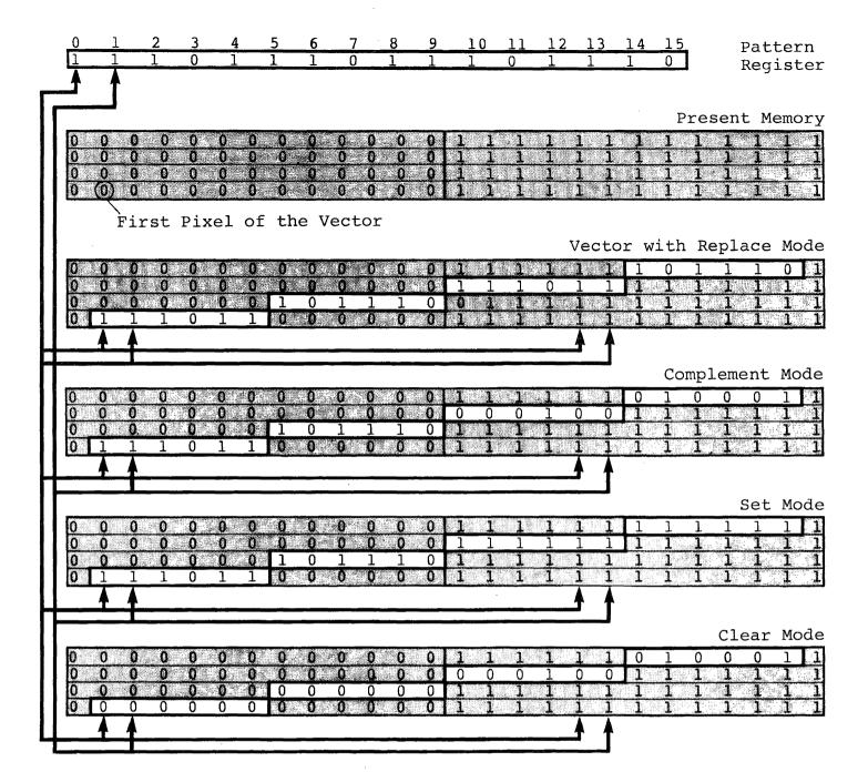
Figure 3.2 Pattern Register Operation During Different Logic Functions
