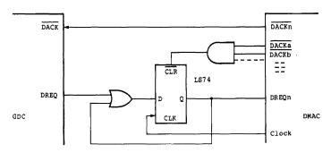
Figure 5.7 System Configuration for DMA Operation with µPD8237 DMA Controller
