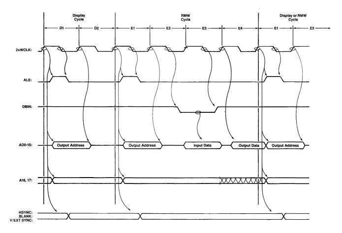
Figure 2.12 RMW Cycle Timing
