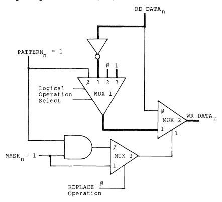
Figure 3.5c RMW Operation with:  $PATTERN_n = 1$ ,  $MASK_n = 1$ , Logic Operation = 1, 2, 3
