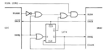
Figure 5.6 System Configuration for DMA Operation with Flashless Mode
