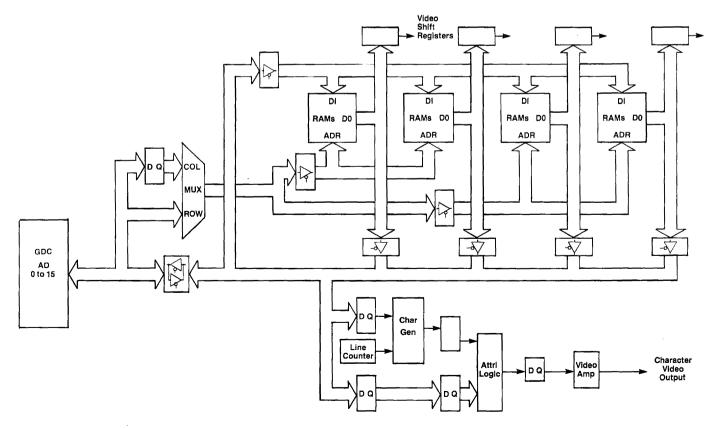
Figure A.2 4-Plane Display System with Character Mode Option
