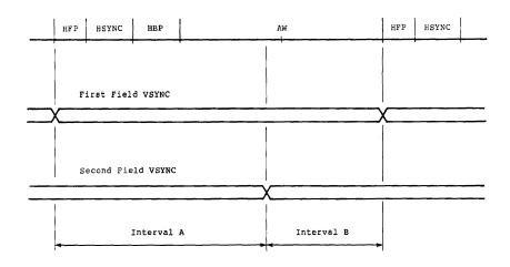
Figure 6.1 Horizontal Timing Relative to Vertical Sync Transitions
