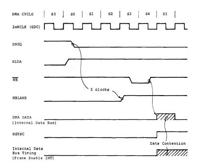
Figure 5.3 DMA Timing Waveforms
