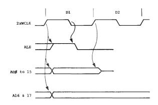
Figure 2.1 Outputting the Display Memory Address
