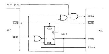
Figure 5.5 System Configuration with uPD8257 DMA Controller to Maintain T1, T2  $\geq$  TCLK
