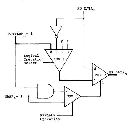
Figure 3.5e RMW Operation with:  $PATTERN_n = 1$ ,  $MASK_n = 1$ , Logic Operation = 0
