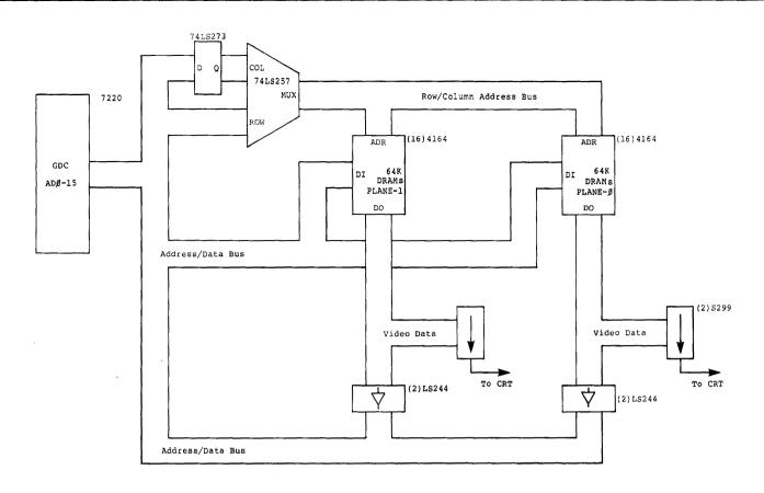
Figure A.1 Wide Display Cycle Memory Configuration
