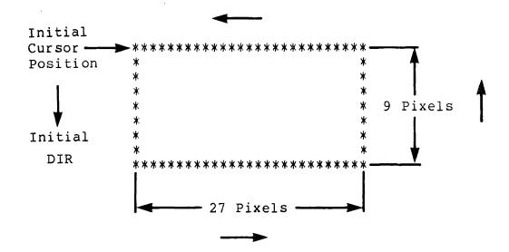
Figure 4.23 Example of Rectangle Drawing
