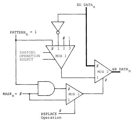
Figure 3.5b RMW Operation with:  $PATTERN_n = 1$ ,  $MASK_n = 0$ , Logic Operation = 1, 2, 3
