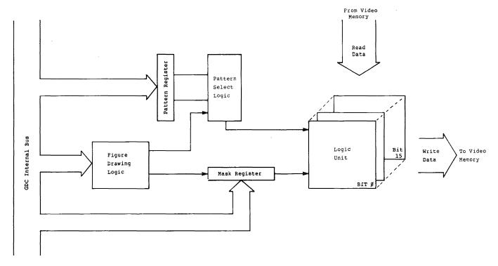
Figure 3.1 RMW Logic Block Diagram
