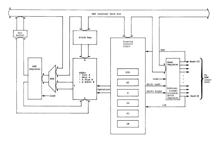
Figure 3.4 GDC Figure Drawing Hardware
