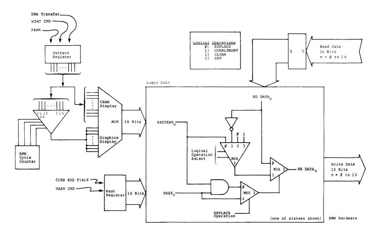
Figure 3.3 RMW Logic Block Diagram
