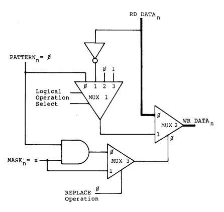
Figure 3.5a RMW Operation with:  $PATTERN_n = 0$ ,  $MASK_n = X$ , Logic Operation = 1, 2, 3
