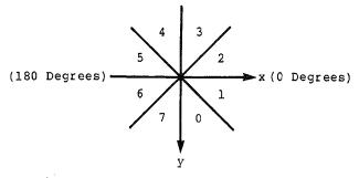
Figure 4.17 Octant Direction Definition
