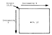
Figure 4.10 Direction of Increasing X,Y Values
