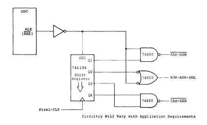
Figure 2.2 Memory Strobe Generation Logic
