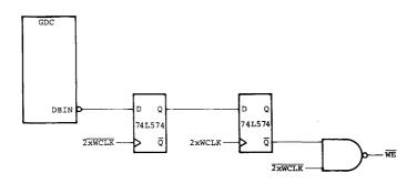
Figure 2.13 RMW Timing Generator
