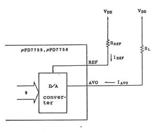
Fig. 3-2 D/A Converter Reference Current
