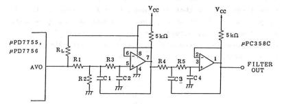
Fig. 4-4 Lowpass Filter Circuit Example
