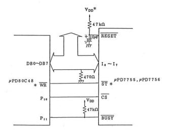
Fig. 4-1 Circuit Example when Control is by Host
