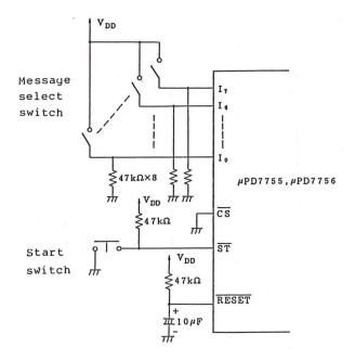
Fig. 4-3 Key Input Mode Circuit Example
