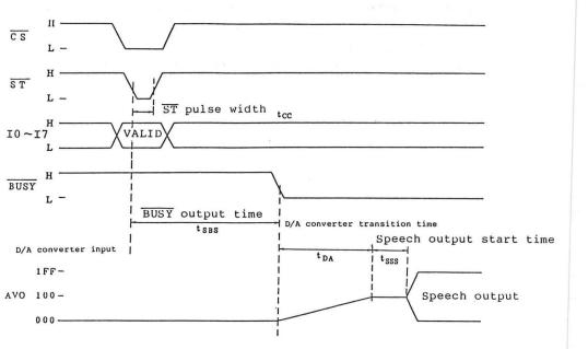
Fig. 3-10 Speech Synthesis Start Operation (Standby Mode)
