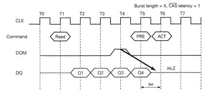
When CAS latency is 2, the read data will remain valid until one clock after the precharge command. Invalid data may appear one clock after valid data out.
