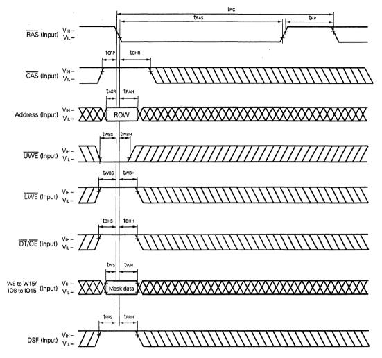
Caution After the falling edge of  $\overline{RAS}$ , the operations performed for the upper byte will be the same as the  $\overline{RAS}$  only refresh cycle.
