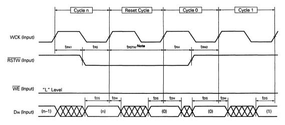
Note In write reset cycle, reset operation is executed even without a reset cycle (tnstw). WCK can be input any number of times in a reset cycle.
