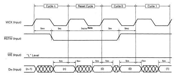
Note In write reset cycle, reset operation is executed even without a reset cycle (trstw). WCK can be input any number of times in a reset cycle.
