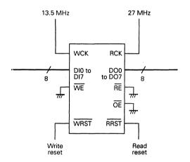
Fig. 5 Circuit of double speed conversion
