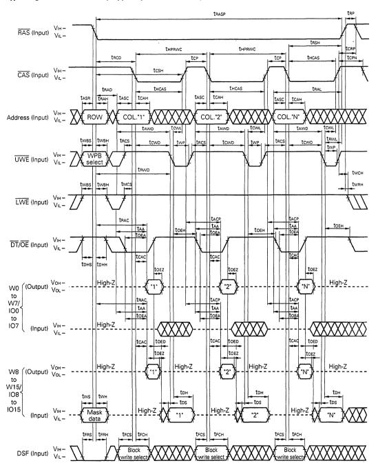
Hyper Page Mode Read Modify Upper Byte Write Cycle (Extended data output: μPD482445) Hyper Page Mode Read Modify Upper Byte Block Write Cycle (Extended data output: μPD482445) Remarks 1. When DSF is high level : Block write cycle
