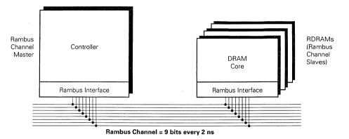
The Rambus Channel is a synchronous, high-speed, byte-wide bus that is used to directly connect Rambus devices together. Using only 13 high-speed signals, the Channel carries all address, data, and control information to and from devices through the use of a high level block-oriented protocol.
