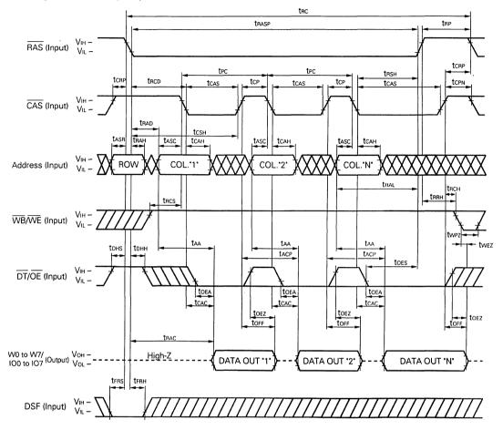
**Remark** Because the serial access port operates independently of the random access port, there is no need to control the SC, SE, SIO pins in this cycle.
