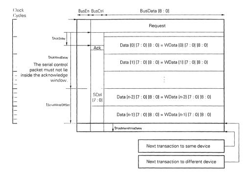
Figure 7-6. Write Transaction with Serial Control Packet
