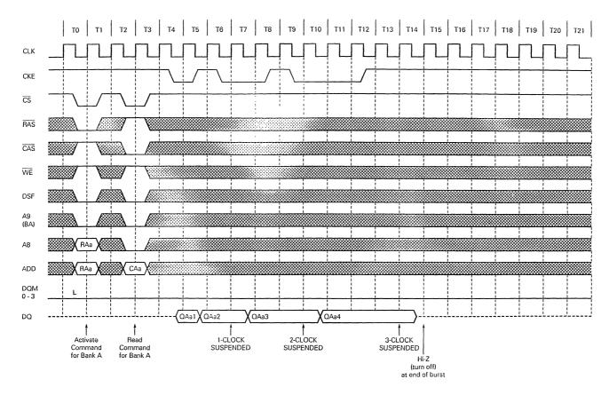
Clock Suspension during Burst Read (using CKE Function) (2/3) (Burst length = 4, CAS latency = 2)
