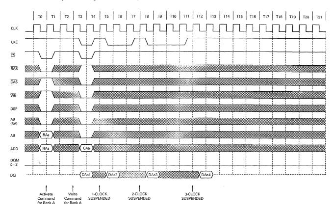
Clock Suspension during Burst Write (using CKE Function) (3/3) (Burst length = 4, CAS latency = 3)
