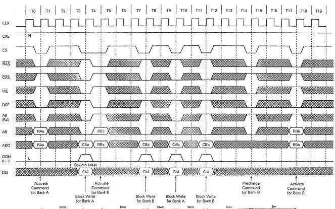
Interleaved Block Write (CAS latency = 3)
