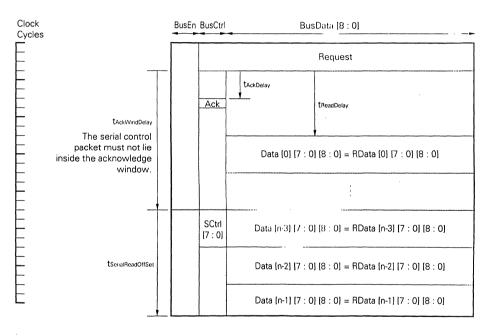
Figure 7-5. Read Transaction with Serial Control Packet
