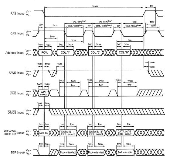
Fast Page, Hyper Page Mode Lower Byte Early Write Cycle/ Fast Page, Hyper Page Mode Lower Byte Early Block Write Cycle
