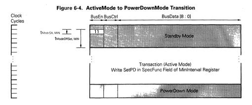
Power may be greatly reduced using the powerdown mode at the expense of moderate latency. In powerdown mode, the device's receivers and clock circuitry are inactive. The device may deactivate other power-hungry circuits also. Power-up enables all these circuits and makes the device available for transactions once the clock circuitry resynchronizes and stabilizes.
