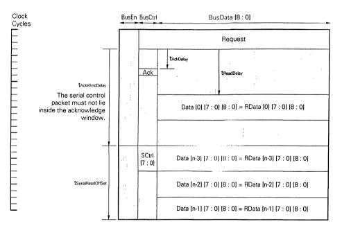
Figure 7-5. Read Transaction with Serial Control Packet
