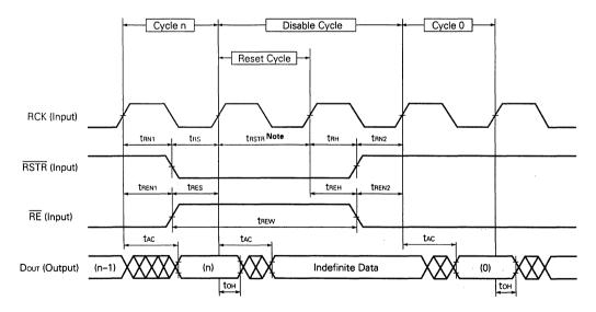
**Note** In read reset cycle, reset operation is executed even without a reset cycle (trstr). RCK can be input any number of times in a reset cycle.
