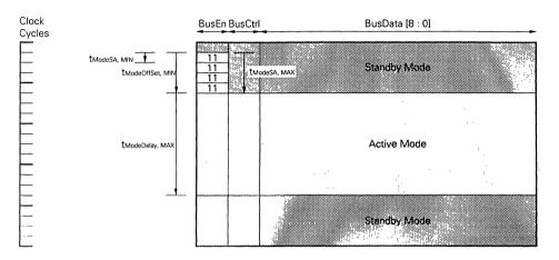
Figure 6-2. Basic ActiveMode/StandbyMode Transitions
