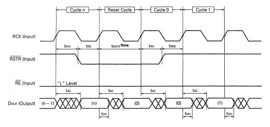
**Note** In read reset cycle, reset operation is executed even without a reset cycle (trstr). RCK can be input any number of times in a reset cycle.
