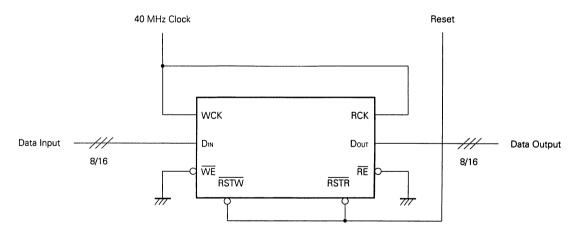
Fig. 1 1 H Delay Line Circuit
