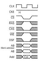
Fig. 6 Column address and read command
