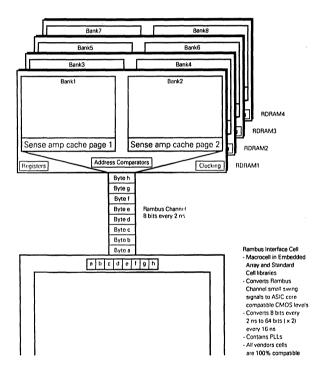
Figure 3-1. Converting the Channel Data Rate
