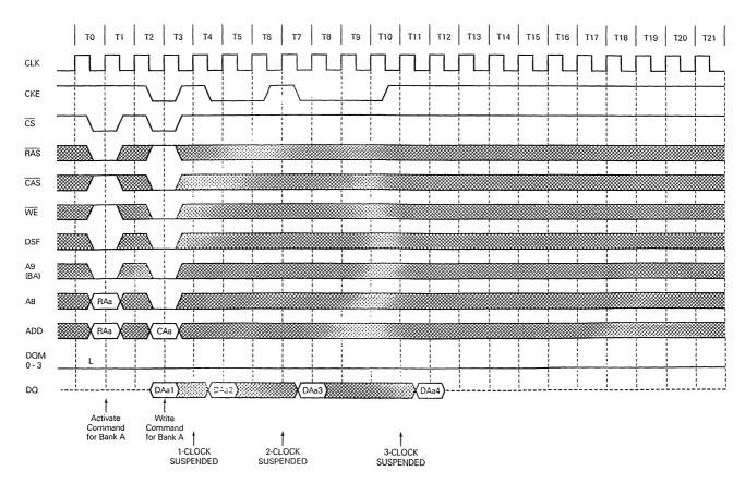
Clock Suspension during Burst Write (using CKE Function) (2/3) (Burst length = 4, CAS latency = 2)
