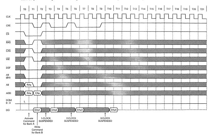
Clock Suspension during Burst Write (using CKE Function) (1/3) (Burst length = 4, CAS latency = 1)
