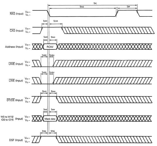
**Remark** Because the serial access port operates independently of the random access port, there is no need to control the SC, SE, SIO pins in this cycle.
