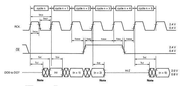
**Remark**  $\overline{\text{RRST}} = \text{"H" level, } \overline{\text{RE}} = \text{"L" level}$
