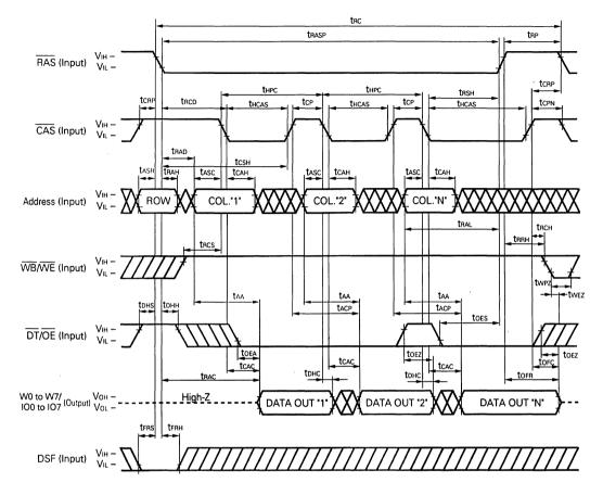
**Remark** Because the serial access port operates independently of the random access port, there is no need to control the SC,  $\overline{SE}$ , SIO pins in this cycle.
