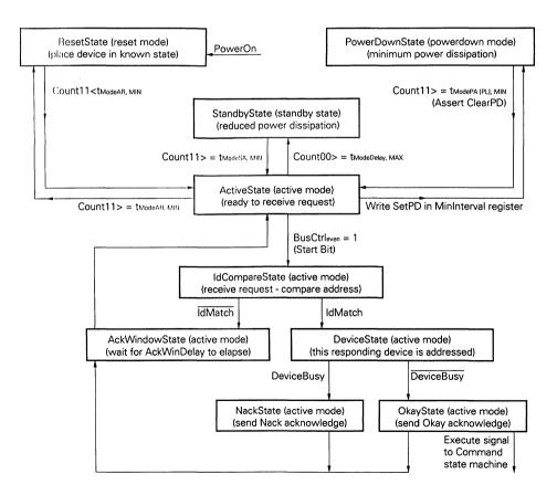
Figure 6-1. Frame State Machine - State Diagram
