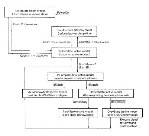
ActiveState is the state in which all decisions are made to transition to the states for the other operating modes. From here, the device will also enter the transaction-framing states. Refer to "Rambus DRAM user's manual (Reference Manual)".
