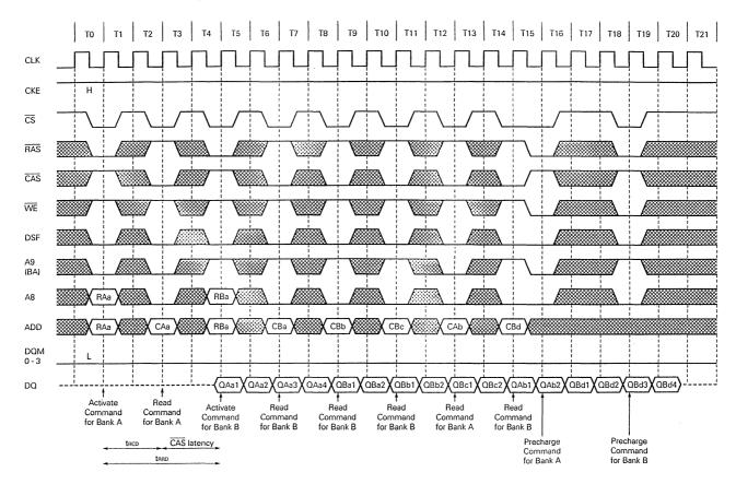
Interleaved Column READ Cycle (2/3) (Burst length = 4,  $\overline{CAS}$  latency = 2)
