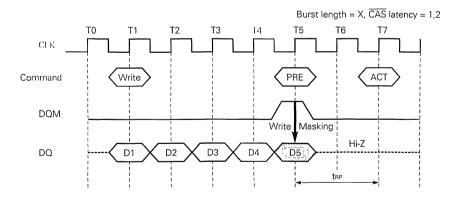
When  $\overline{CAS}$  latency is 3, the write data written more than one clock prior to the precharge command will be correctly stored.
