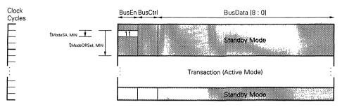
Figure 6-3. ActiveMode/StandbyMode Transition - Early Transaction
