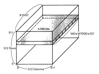
Figure 2-5. Memory Cell Range That Can be Written with Flash Write Cycle
