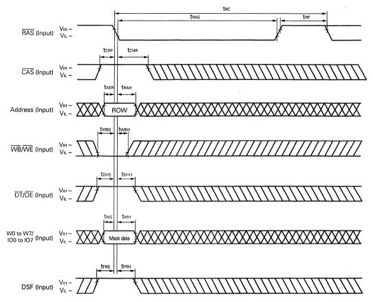
**Remark** Because the serial access port operates independently of the random access port, there is no need to control the SC, SE, SIO pins in this cycle.
