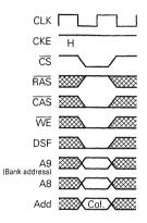
Fig. 5 Column address and write command
