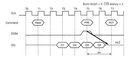
When CAS latency is 3, the read data will remain valid until one clock after the precharge command. Invalid data may appear one and two clocks after valid data out.
