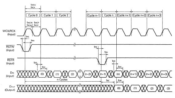
Fig. 4 n-Bit Delay Line Timing (2)
