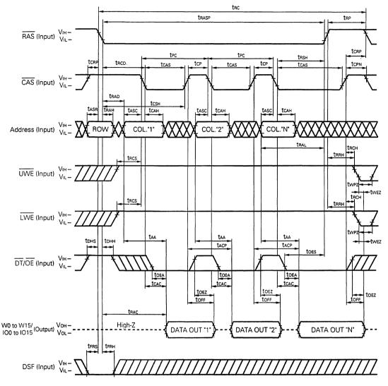
**Remark** Because the serial access port operates independently of the random access port, there is no need to control the SC, SE, SIO pins in this cycle.
