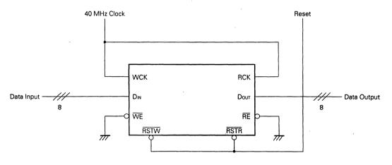
Fig. 1 1 H Delay Line Circuit
