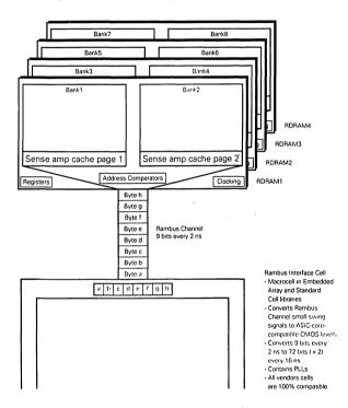
Figure 3-1. Converting the Channel Data Rate
