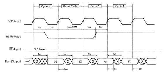
Note In read reset cycle, reset operation is executed even without a reset cycle (thsth). RCK can be input any number of times in a reset cycle.
