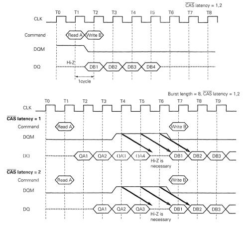
For  $\overline{CAS}$  latency of 3, the READ and WRITE command interval is [Burst length + 1] cycles. The data bus must be Hi-Z using DQM before WRITE to avoid data conflict. And DQM must be kept being High from at least 3 clocks to 1 clock before the WRITE command.
