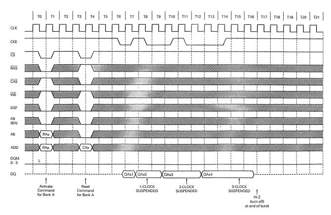
Clock Suspension during Burst Read (using CKE Function) (3/3) (Burst length = 4,  $\overline{CAS}$  latency = 3)
