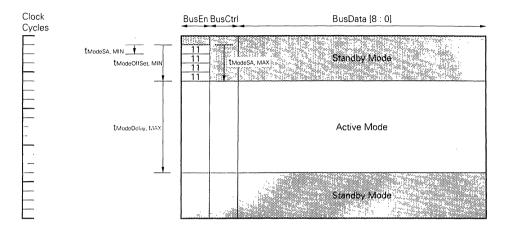
Figure 6-2. Basic ActiveMode/StandbyMode Transitions
