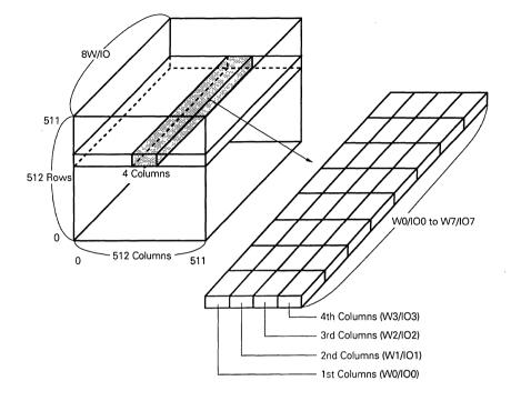
Figure 2-6. Memory Cell Range That Can be Written in Block Write Cycle
