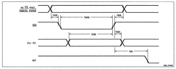
Figure. 6 DMA Operation
