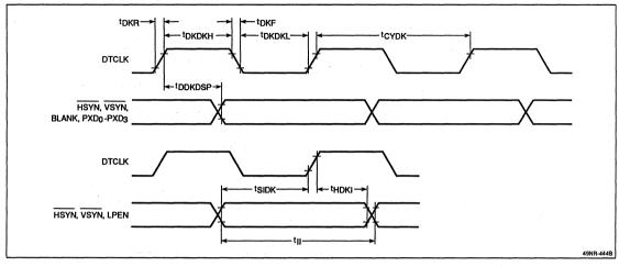
Figure 15. DMA Read Cycle
