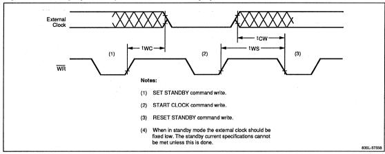
Figure 8. Standby Operation (With External Clock Input)
