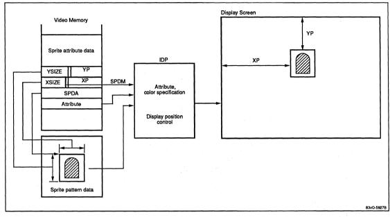
Figure 25. Data Flow During Sprite Image Display
