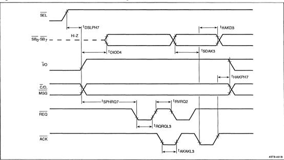
Figure 18. SCSI Bus; Transfer as Initiator in Sync Mode
