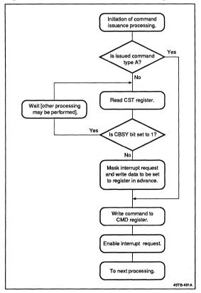
Figure 45. Interrupt Processing Flow
