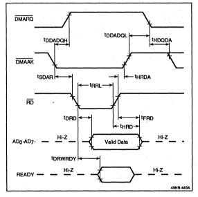
Figure 16. DMA Write Cycle
