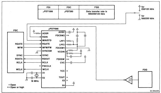
Figure 18. System Example 10: µPD71066 FDI and µPD7260 FDC
