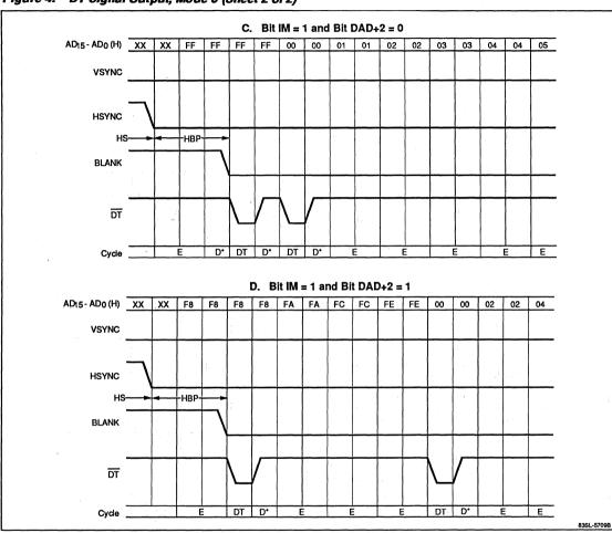
Figure 4. DT Signal Output, Mode 0 (Sheet 2 of 2)
