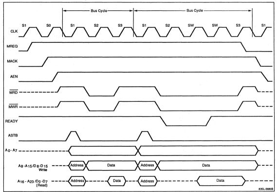
Figure 16. DMA Transfer Timing
