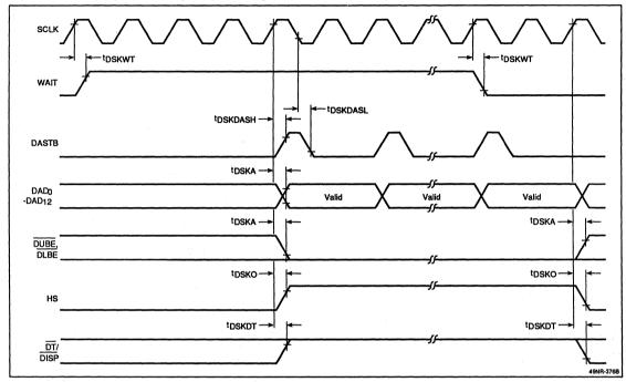
Figure 13. Display Refresh Cycle (CS Mode)
