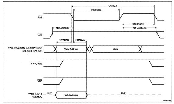
Figure 9. VRAM Request; Interleave Mode
