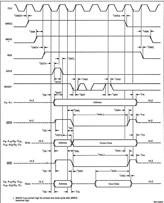
Figure 3. DMA Transfer Timing on Image Bus
