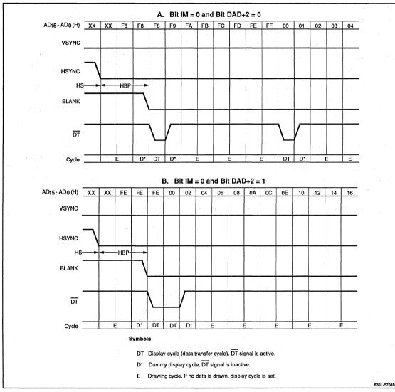
Figure 4. DT Signal Output, Mode 0 (Sheet 1 of 2)
