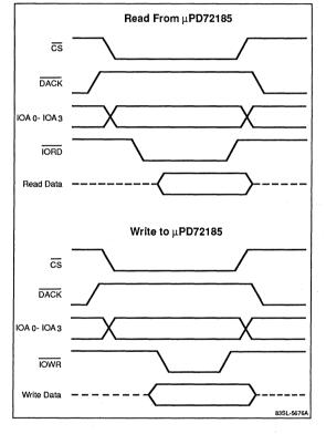
Figure 14. Read/Write Timing With External DMA Controller
