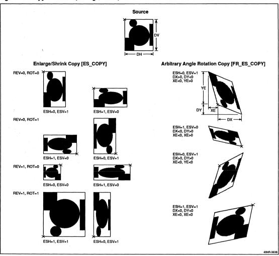
Figure 27. Copy Commands; Enlarge/Shrink, Rotate
