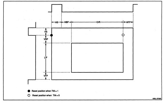
Figure 2. Horizontal Counter Reset Timing
