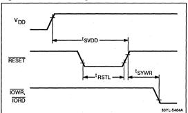
Figure 7. Read/Write Cycle Timing
