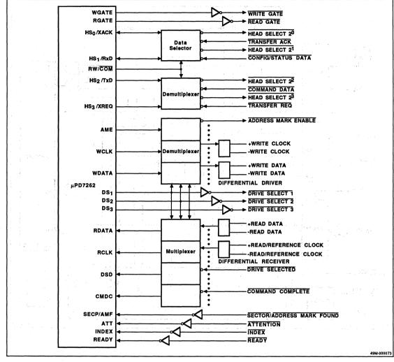
Figure 27. Example of the Interface Between the µPD7262 and a Hard-Disk Drive
