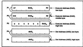
The execute address, EAD, points to the display memory word containing the pixel to be addressed.
