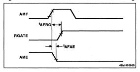
Figure 14. One-Bit Transfer Timing (to Drive)
