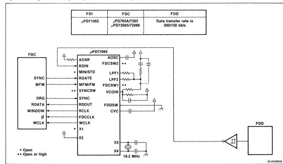
Figure 10. System Example 2: µPD71065 FDI and µPD765A FDC
