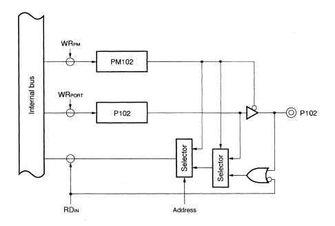
The input/output mode of port 10 is set by port mode register 10 (PM10). The control mode is set by port mode control register 10 (PMC10).
