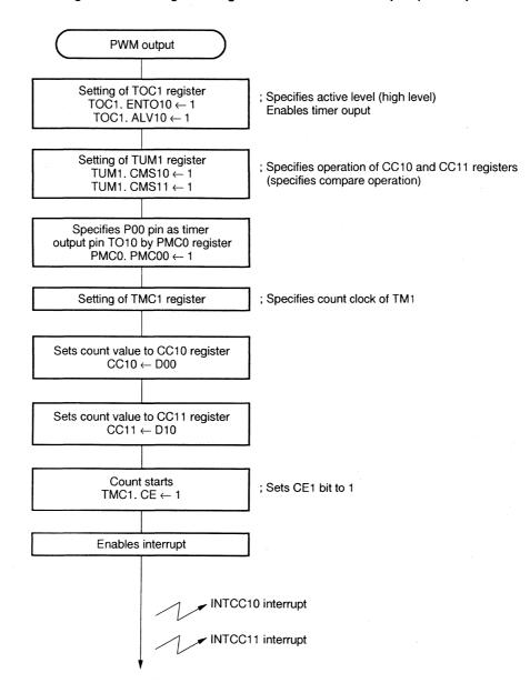
Figure 7-18. Programming Procedure of PWM Output (timer 1)
