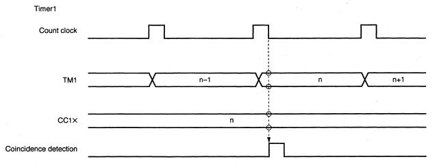
**Remark:** Note that the coincidence signal is generated immediately after TM1 is incremented as shown above.
