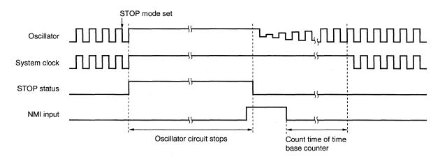
During inactivity, the NMI pin should be kept at the inactive level (e.g. at a logic "1" when the valid edge is specified to be the falling edge).
