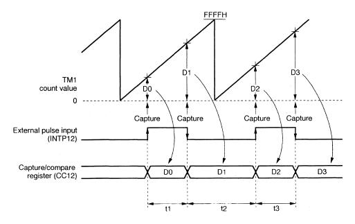
$t1= (D1-D0) \times count clock cycle$  $t2= {(FFFH-D1) +D2} \times count clock cycle$  $t3= (D3-D2) \times count clock cycle$
