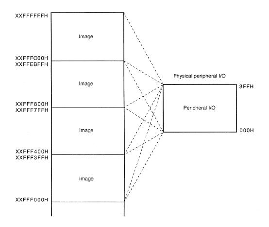
Peripheral I/O registers associated with the on-chip peripherals and the CPU are all memory-mapped to peripheral I/O area. Instruction fetches are not allowed in this area.
