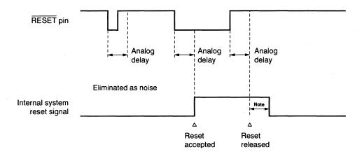
**Note:** The internal system reset signal remains active for the duration of at least 4 system clocks after the reset condition is removed from the RESET pin.
