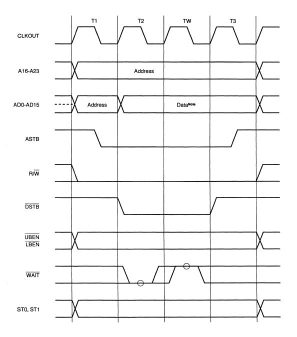
**Note:** AD0-AD7 output invalid data when odd address byte data is accessed. AD8-AD15 output invalid data when even address byte data is accessed.
