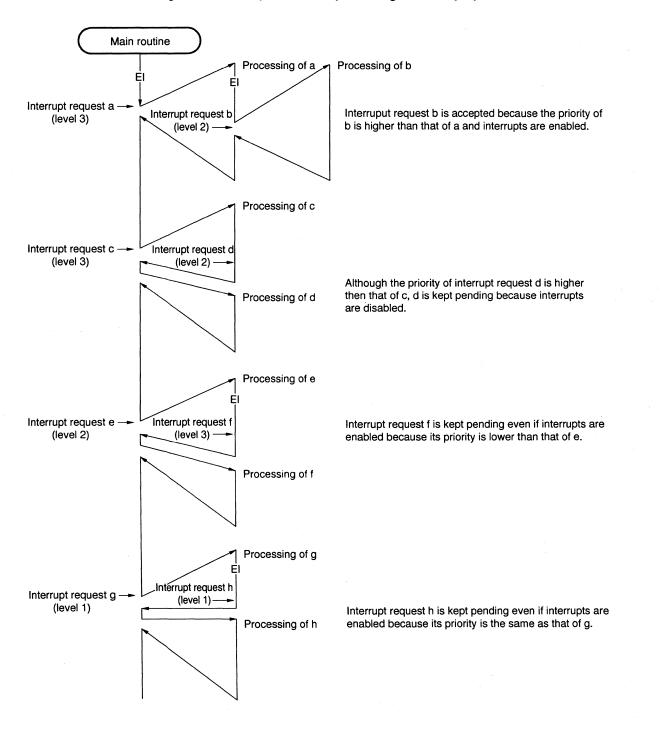
Figure 5-7. Example of Interrupt Nesting Process (1/2)
