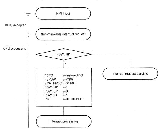
Figure 5-1. Non-Maskable Interrupt Processing
