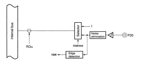
Figure 9-5. Block Diagram of P21-P24 (Port 2)
