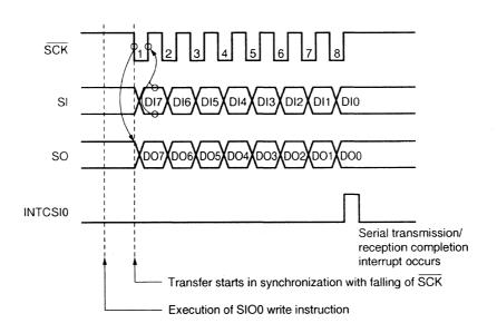
Figure 8-6. Timing of 3-Wire Serial I/O Mode (transmission)
