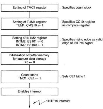
Figure 7-22. Interrupt Request Processing Routine Calculating Cycle (timer 1)
