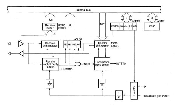
Figure 8-1. Block Diagram of Asynchronous Serial Interface
