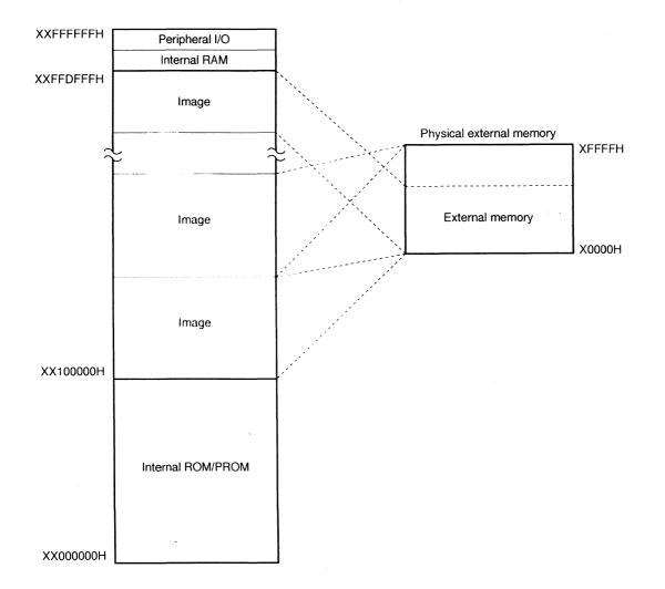
Figure 3-7. External Memory Area (when expanded to 64 KB, 256 KB, or 1 MB)
