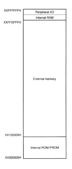
Figure 3-9. External Memory Area (when fully expanded)
