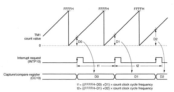
Figure 7-20. Frequency Measurement Timing(TM1)
