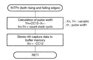
Caution: If an overflow occurs two times or more between (n-1)th capture and nth capture, the pulse width cannot be measured.
