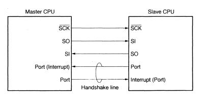
(3-wire serial I/O - 3-wire serial I/O)
