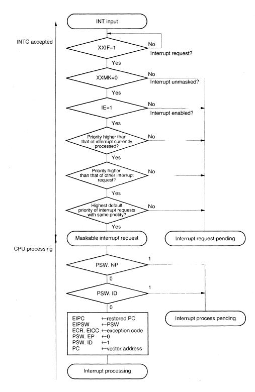
The INT input masked by the interrupt control registers and the automatic interrupt mask that occurs while a previous interrupt is being processed (when PSW.NP = 1 or PSW.ID = 1) are internally monitored by the interrupt controller. When the interrupts are unmasked, or when PSW.NP = 0 and PSW.ID = 0 by using the RETI and LDSR instructions, the pending maskable interrupts can then be acknowledge, by priority, and processed.
