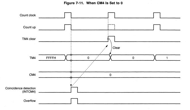
**Remark:** Interval time = (FFFFH + 2)  $\times$  count clock cycle
