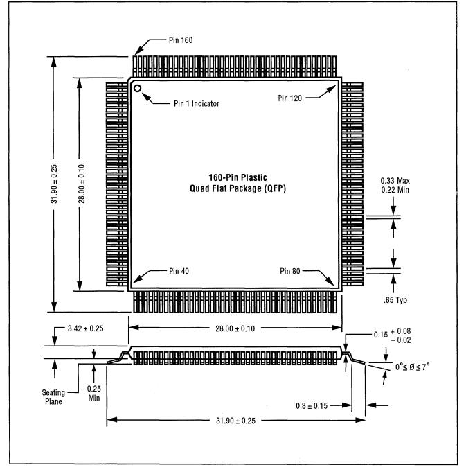
**Note:** All dimensions are in millimeters. This package is known as a Metric QFP, and should not be confused with the similiar JEDEC QFP.
