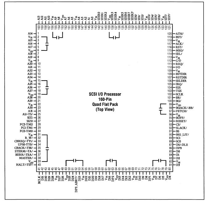
Note: The decoupling capacitor arrangement shown above is recommended to maximize the benefits of the internal split ground system. Capacitor values between 0.01 and 0.1 µF should provide adequate noise isolation. Because of the number of high current drivers on the 53C710, a multilayer PC board with power & ground planes is required.
