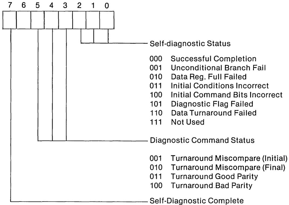
Bit 7 = 1 indicates that self-diagnostics have been completed. (NOTE: A reset will clear bits 6-3 if possible). After a reset to the chip, the microprocessor should make sure that the Diagnostic Status Register contains the following pattern before attempting any commands: 10000000. This code indicates self-diagnostics are complete and no errors were detected. After a diagnostic command has been executed, bits 6-3 will contain the resulting status, but bit 7 and bits 2-0 are not affected.
