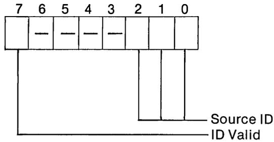
The ID Valid bit indicates that the source device placed its own ID bit on the SCSI bus during the Selection Phase. The SPC chip has encoded the source ID and placed it in bits 2-0. This information remains valid until the chip disconnects from the SCSI bus, at this time the ID Valid bit is reset.
