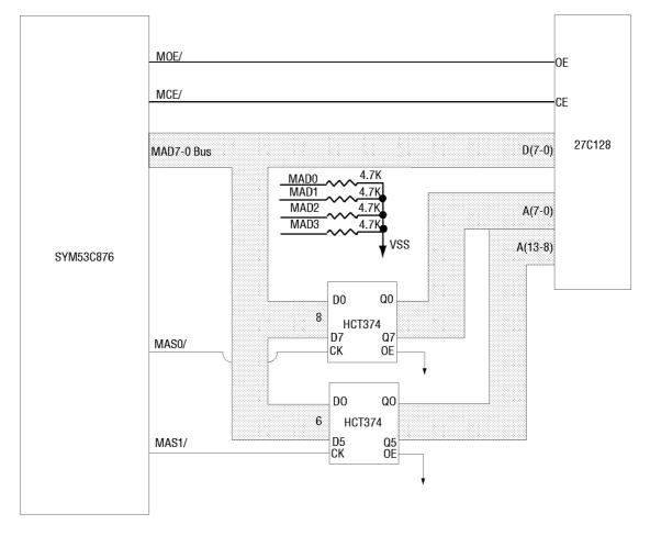
MAD3-1 pulled low internally. MAD Bus Sense Logic Enabled for 16 KB of slow memory (200 ns Device @ 33MHz)
