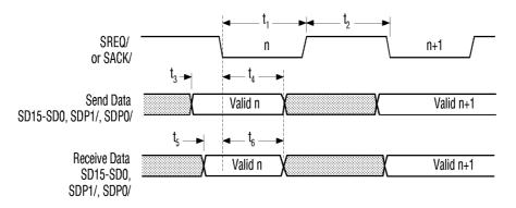
Figure 6-33: Initiator and Target Synchronous Transfers
