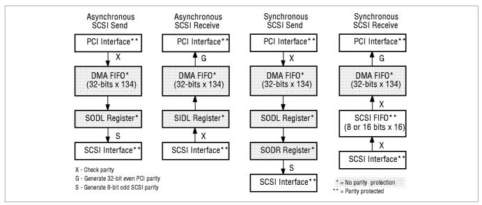
Figure 2-2: Parity Checking/Generation
