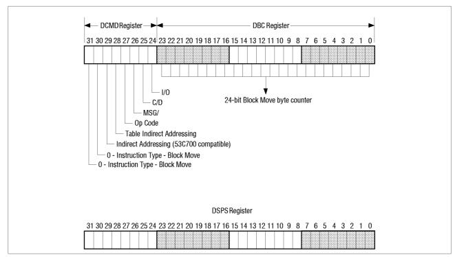
Figure 5-2: Block Move Instruction Register
