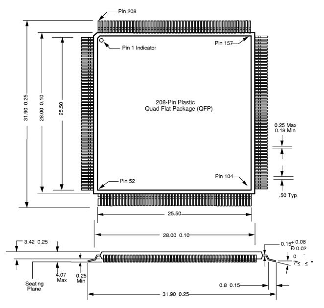
Figure B-1:SYM53C876 208-Pin PQFP Mechanical Drawing
