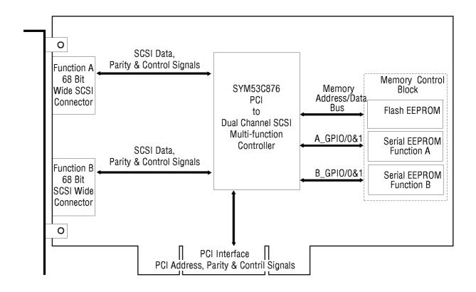
Figure 1-2: Typical SYM53C876 Board Application
