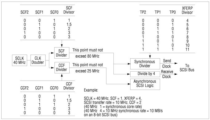
Figure 2-7: Determining the Synchronous Transfer Rate
