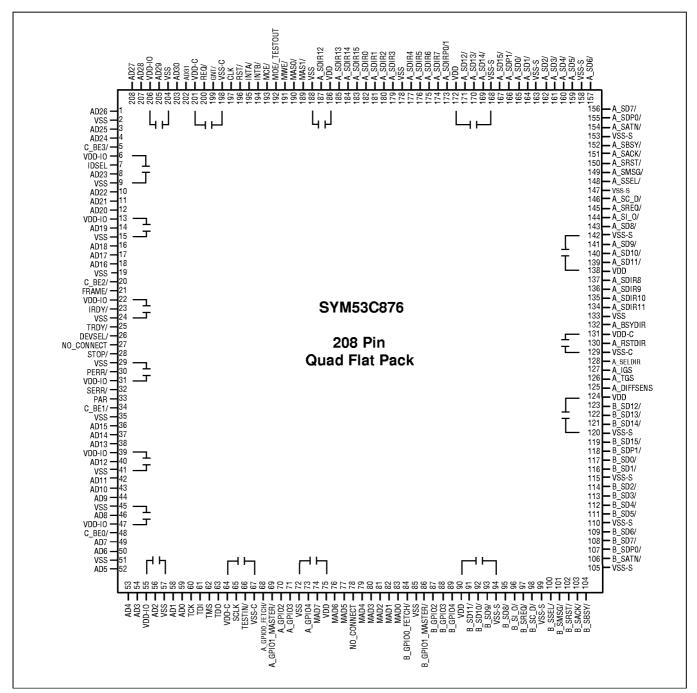
Figure 3-1: SYM53C876 208-Pin PQFP Diagram
