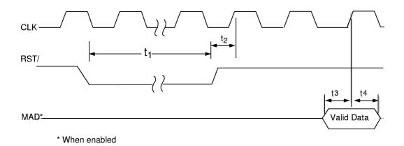
Figure 6-7: Reset Input
