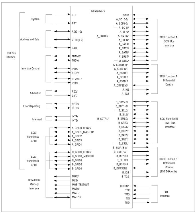
Figure 3-3: SYM53C876 Functional Signal Grouping
