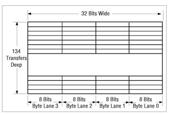
Figure 2-3: DMA FIFO Sections
