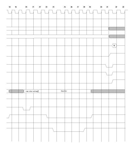
Figure 6-24: Write Cycle, Normal/Fast Memory (≥128 KB), multiple byte access (continued)
