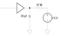
Figure 6-1: Rise and Fall Time Test Conditions
