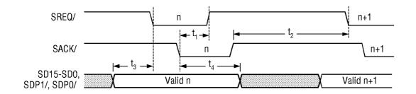
Figure 6-31: Target Asynchronous Send
