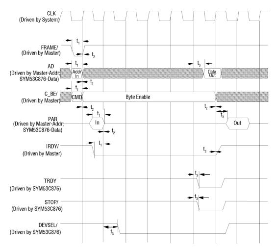
Figure 6-11: Target Read, not from external memory
