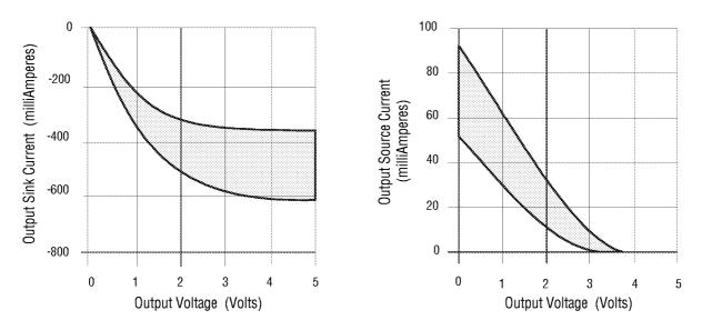
Figure 6-5: Output Current as a Function of Output Voltage
