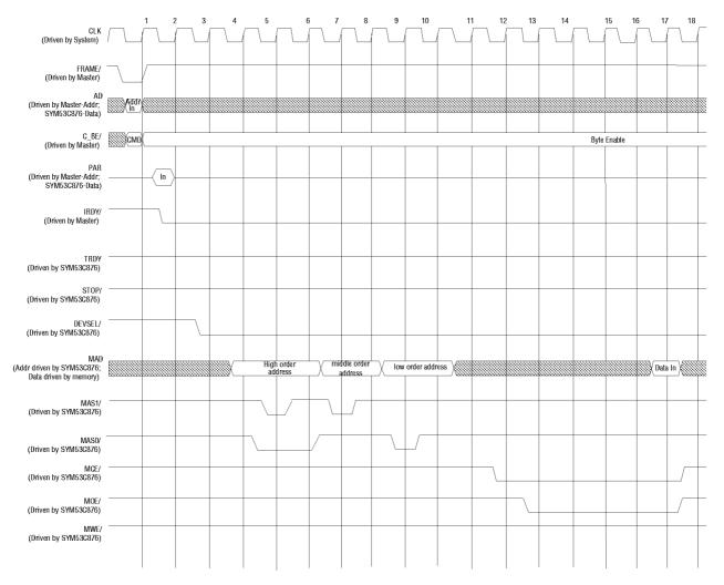
Figure 6-23: Read Cycle, Normal/Fast Memory (≥128 KB), multiple byte access
