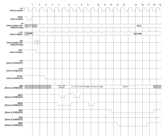
Figure 6-24: Write Cycle, Normal/Fast Memory (≥128 KB), multiple byte access
