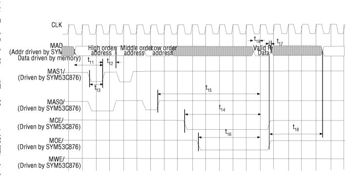
Figure 6-21: Read Cycle, Normal/Fast Memory (>128 KB), single byte access
