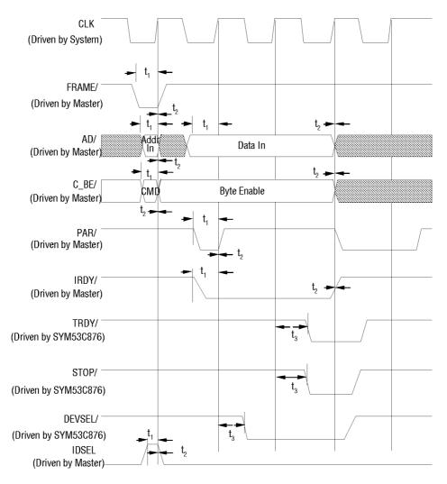
Figure 6-10: Configuration Register Write
