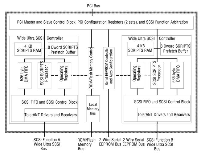
Figure 2-1: SYM53C876 Block Diagram
