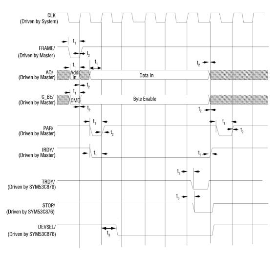
Figure 6-12: Target Write, not from external memory
