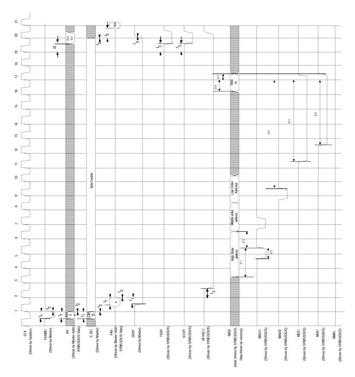
Figure 6-13: Target Read, from external memory
