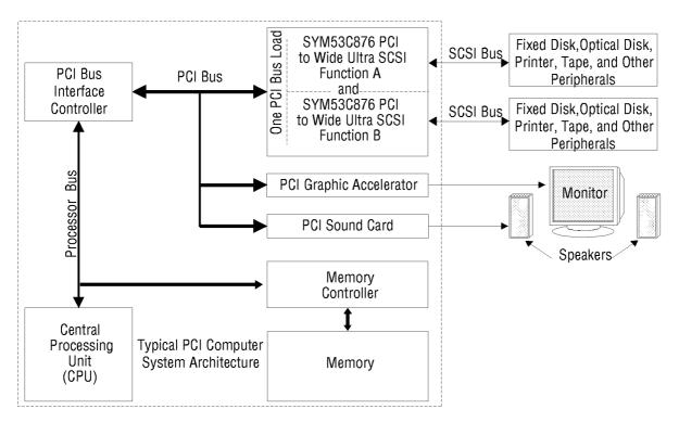
Figure 1-1: Typical SYM53C876 System Application
