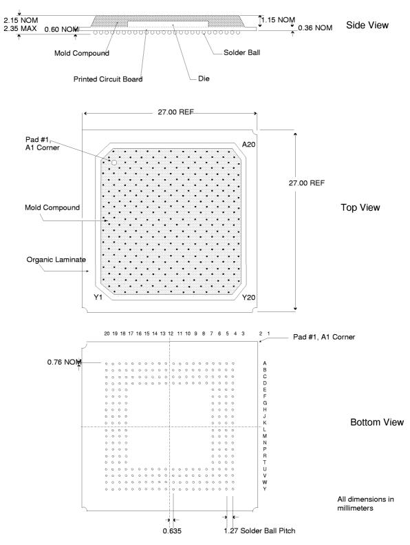
Figure B-2:SYM53C876 256-Bump PBGA Mechanical
