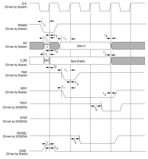
Figure 7-10: PCI Configuration Register Write
