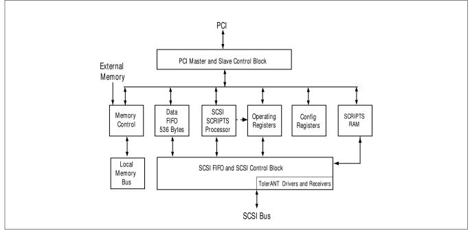
Figure 1-2: SYM53C825A Chip Block Diagram
