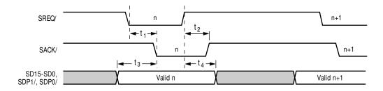
Figure 7-32: Initiator Asynchronous Receive
