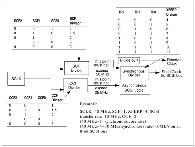
Figure 2-5: Determining the Synchronous Transfer Rate
