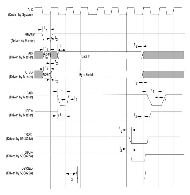
Figure 7-12: Operating Register/SCRIPTS RAM write
