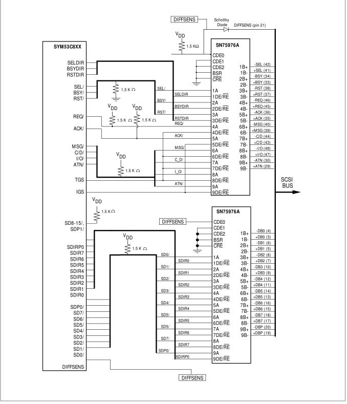
Figure 2-3: SYM53C825A Differential Wiring Diagram
