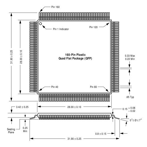
Figure B-1: SYM53C825A, 53C825AJ Mechanical Drawing
