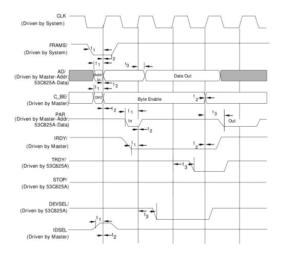
Figure 7-9: PCI Configuration Register Read
