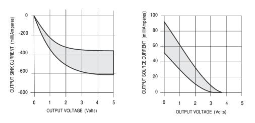
Figure 7-5: Output Current as a Function of Output Voltage
