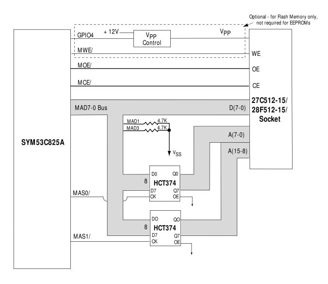
MAD Bus Sense Logic Enabled for 64 KB of fast memory (150 ns Device @ 33MHz)
