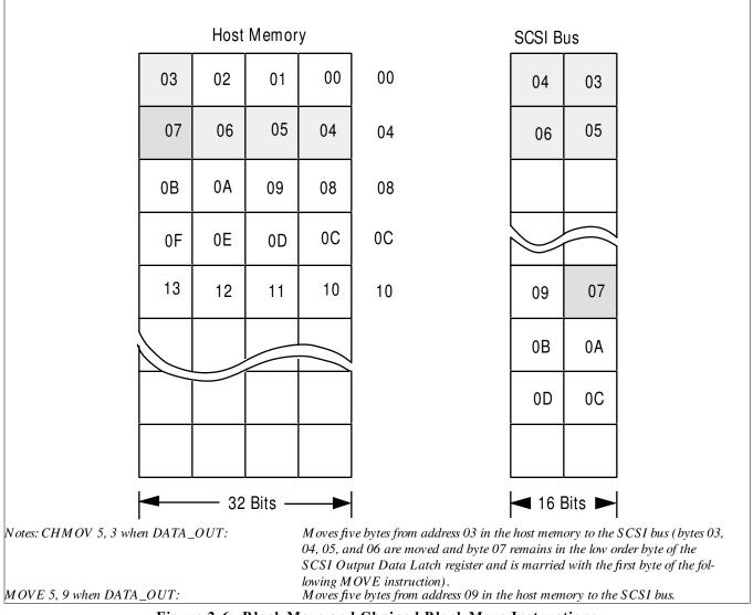
Figure 2-6: Block Move and Chained Block Move Instructions
