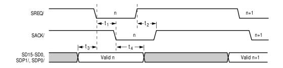
Figure 7-34: Target Asynchronous Receive
