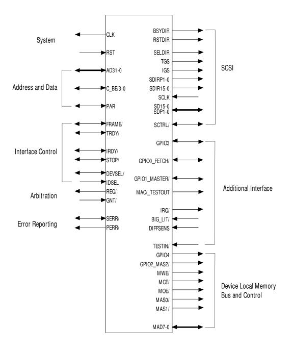
Figure 4-3: SYM53C825A Functional Signal Grouping
