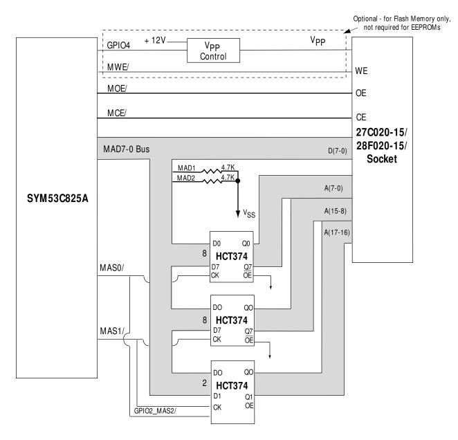
MAD Bus Sense Logic Enabled for 256 KB of fast memory (150 ns Device @ 33MHz). Address latch for the two most significant bits can be HCT74, HCT174, HCT175, etc.
