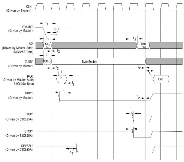
Figure 7-11: Operating Register/SCRIPTS RAM read
