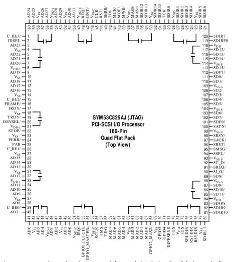
The decoupling capacitor arrangement shown above is recommended to maximize the benefits of the internal split ground system. Capacitor values between 0.01 and 0.1µF should provide adequate noise isolation. Because of the number of high current drivers on the SYM 53C825A, a multi-layer PC board with power and ground planes is required.
