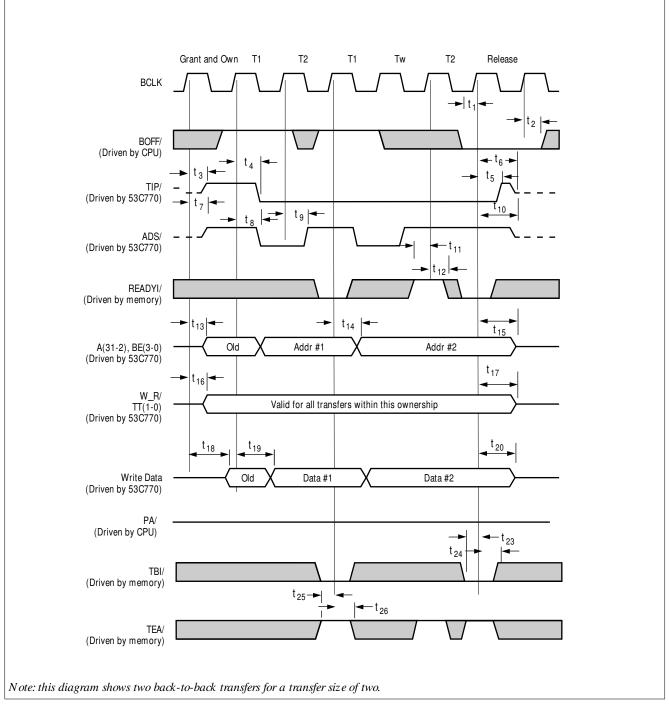
Figure 6-35: Bus Mode 3 and 4 Bus Master Write (Non-Preview of Address)
