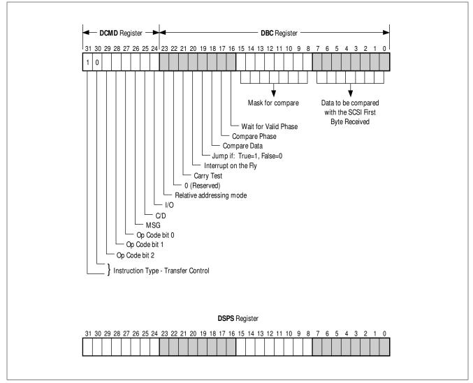
Figure 5-5: Transfer Control Instruction Register
