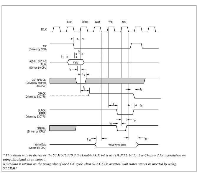
Figure 6-10: Bus Mode 1 Slave Write Waveforms
