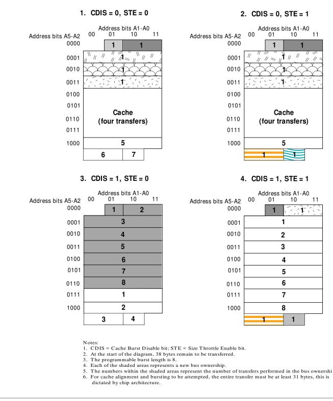
Figure 2-3: Transfer Size Throttling
