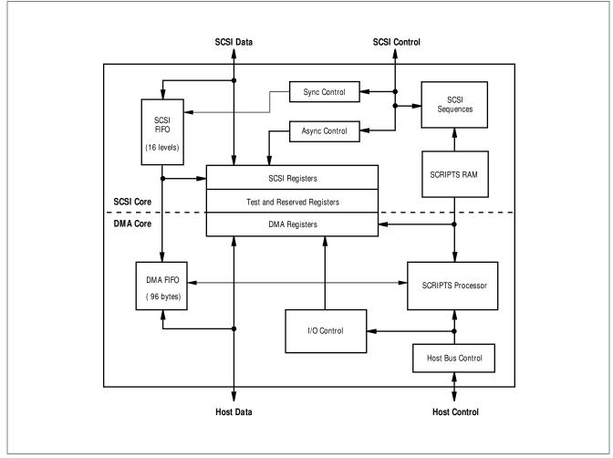
Figure 1-1: SYM53C770 Block Diagram
