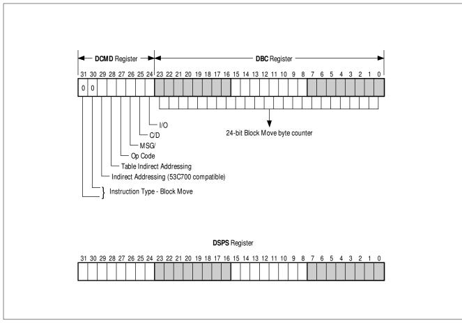
Figure 5-1: Block Move Instruction Register
