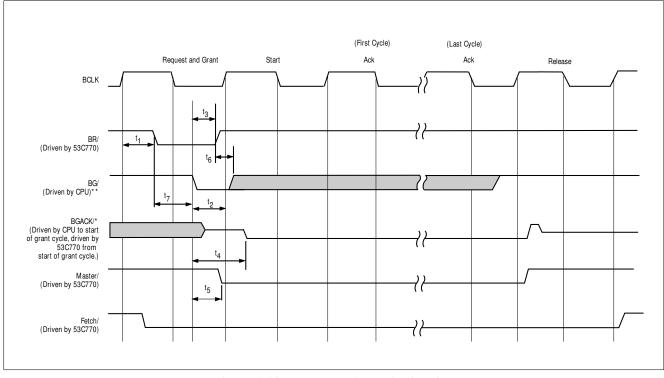
Figure 6-12: Bus Mode 1 Fast Arbitration
