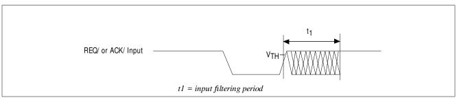
Figure 6-2: SCSI Input Filtering
