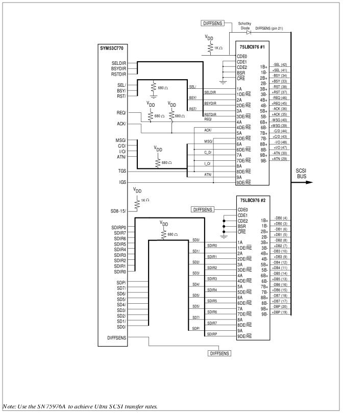
Figure 2-6: 53C770 Differential Wiring Diagram
