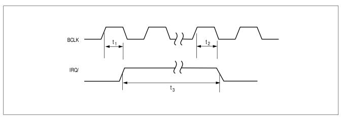
Figure 6-8: Interrupt Output Waveforms
