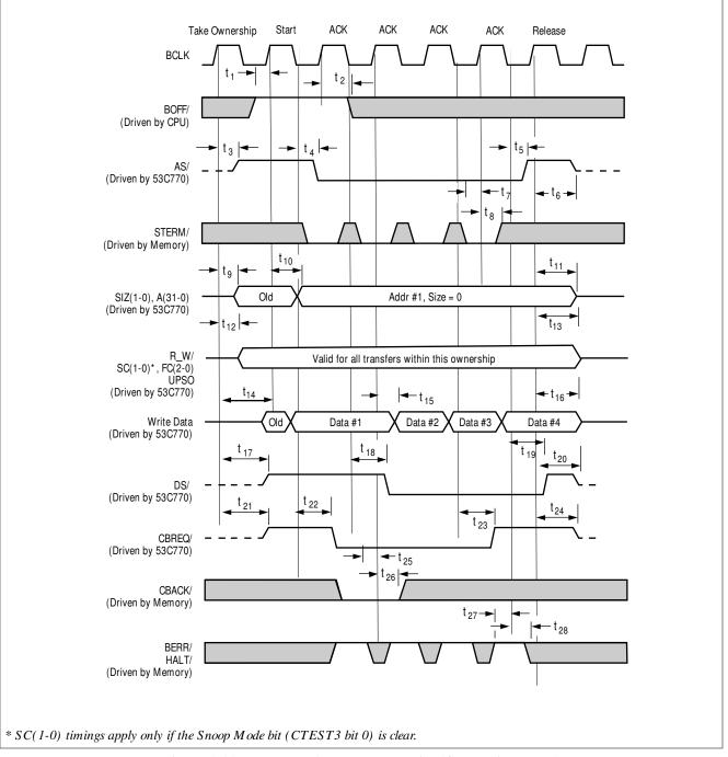
Figure 6-16: Bus Mode 1 Bus Master Write (Cache Line Burst)
