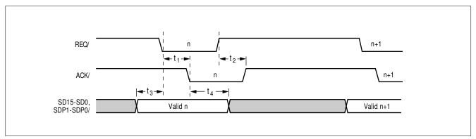
Figure 6-39: Initiator Asynchronous Receive
