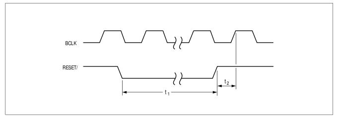
Figure 6-7: Reset Input Waveforms
