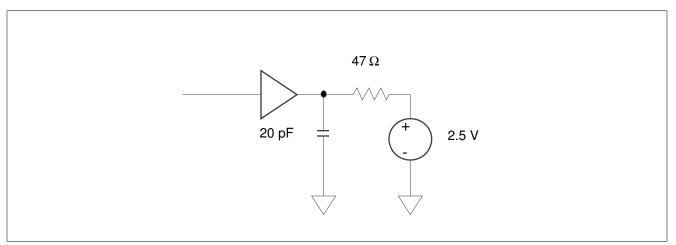
Figure 6-1: Rise and Fall Time Test Conditions
