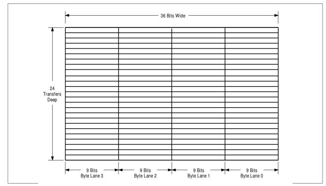
Figure 2-1: DMA FIFO Byte Lanes
