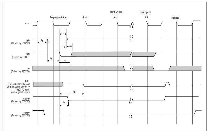
Figure 6-20: Bus Mode 2 Fast Arbitration
