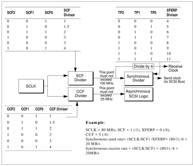
Figure 2-8: Determining the Synchronous Transfer Rate
