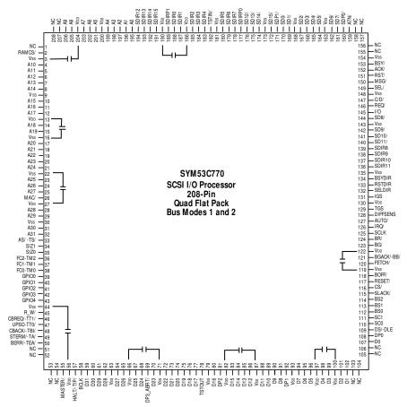
Note: the decoupling capacitor arrangements shown above are recommended to maximize the benefits of the internal split ground system. Capacitor values between 0.01 and 0.1  $\mu$ F should provide adequate noise isolation. Because of the number of high current drivers on the SYM 53C770, a multi-layer PC board with power and ground planes is required.
