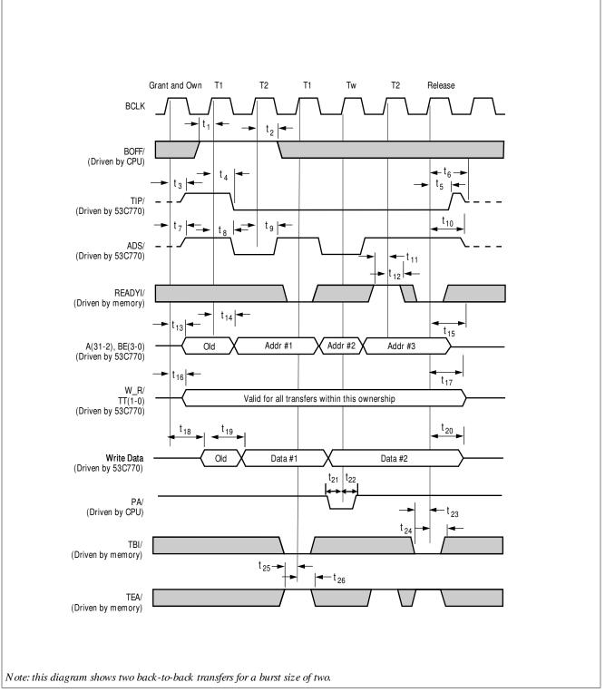
Figure 6-36: Bus Mode 3 and 4 Bus Master Write (Preview of Address)
