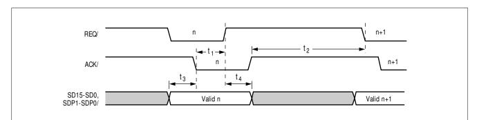
Figure 6-41: Target Asynchronous Receive
