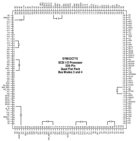
Note: the decoupling capacitor arrangements shown above are recommended to maximize the benefits of the internal split ground system. Capacitor values between 0.01 and 0.1 µF should provide adequate noise isolation. Because of the number of high current drivers on the SYM 53C770, a multi-layer PC board with power and ground planes is required.
