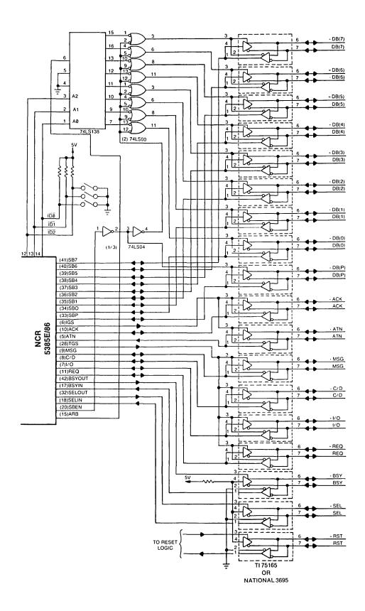
Figure 6.1 Suggested Interface to SCSI Differential Transceivers
