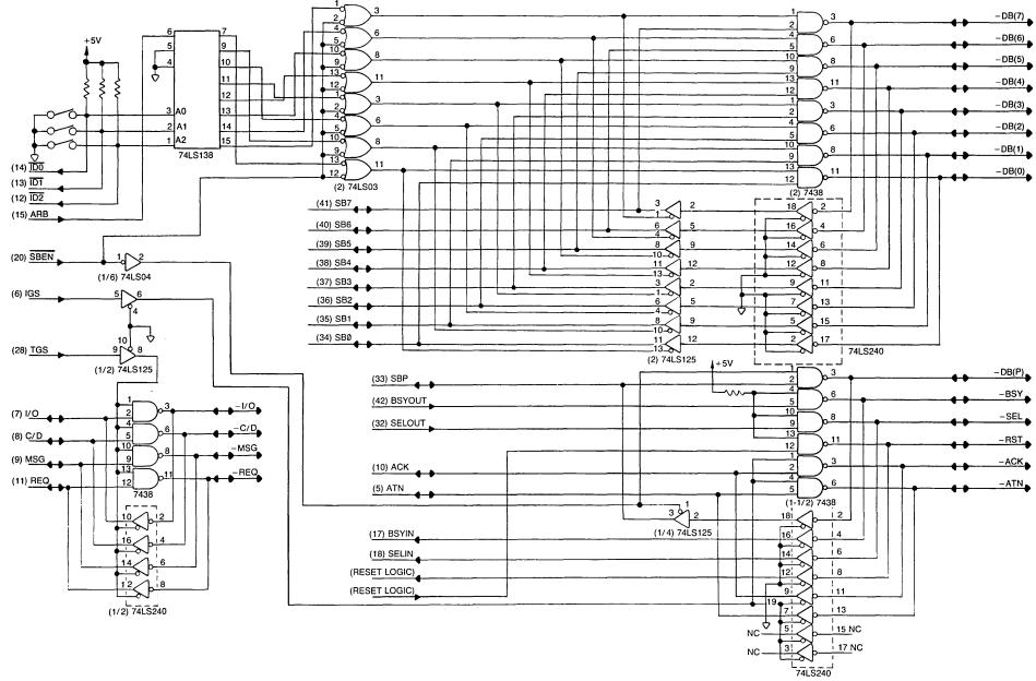
Figure 6.2 NCR 8310 Equivalent Circuit
