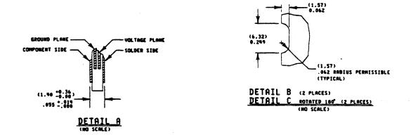
Figure 9. Dimensional Drawing of ADP-55
