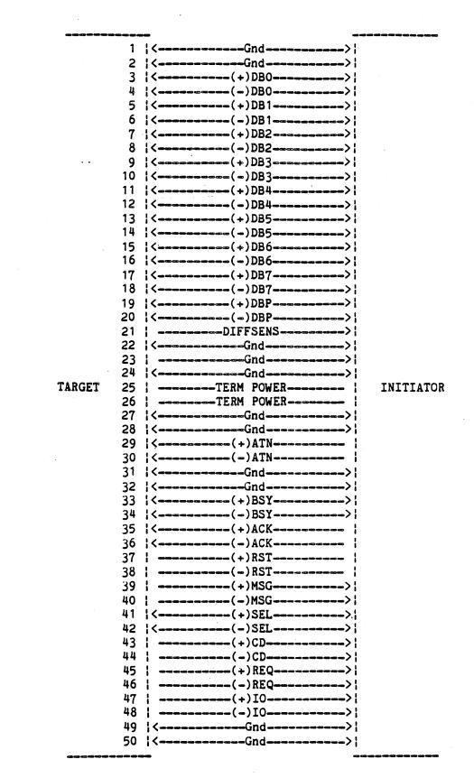
Figure 2. Differential pin assignments
