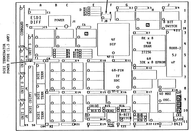
Figure 4-11 NCR ADP-47-04 ESDI Differential Controller board
