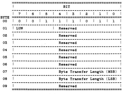
Figure 3-42 Write Buffer command descriptor
