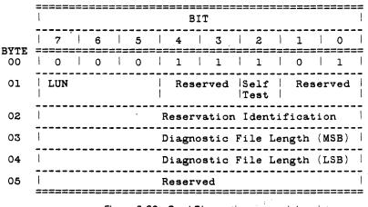
Figure 3-30 Send Diagnostic command descriptor
