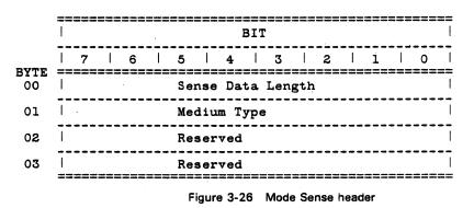
The Sense Data Length byte specifies the length in bytes of the following Mode Sense data available for transfer during the Data-In phase. The Sense Data Length byte does not include itself. If the command descriptor Allocation Length is not large enough to transfer all the Sense Data Length, the Sense Data Length does not adjust to reflect the truncation.
