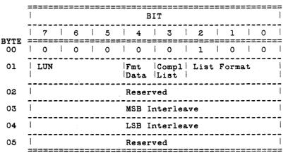
Figure 3-4 Format Fixed Unit command descriptor
