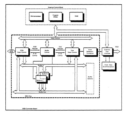
Figure 1-1 ADP-47 block diagram
