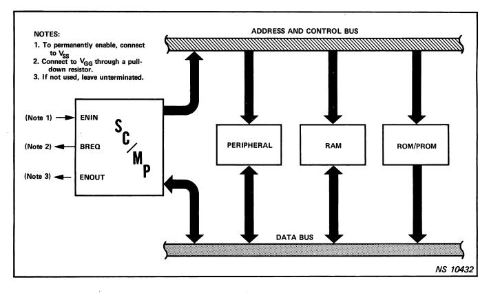
Figure 2-3. SC/MP-Controlled Bus Access
