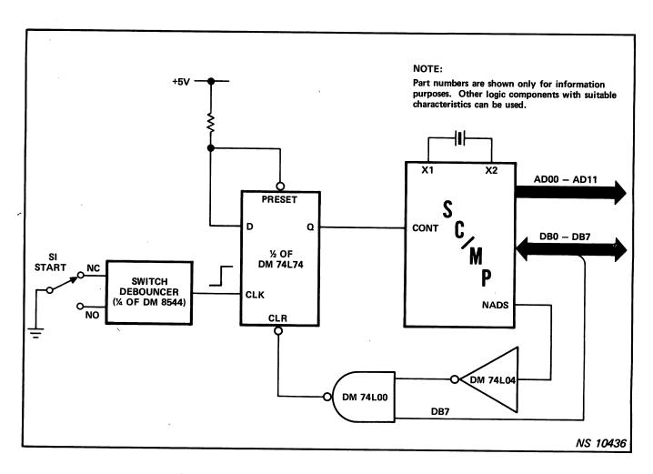
Figure 2-7. Using "H" Flag To Generate a Programmed Halt
