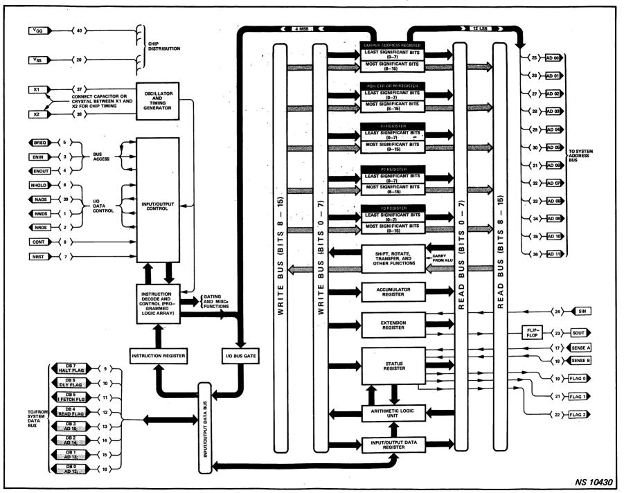
Figure 2-1. SC/MP Functional Block Diagram with Pinouts
