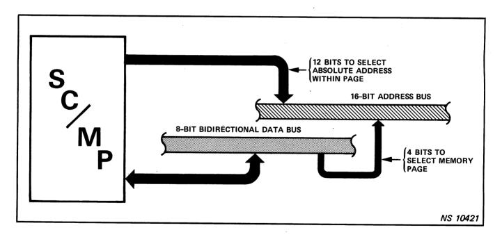
Figure 1-4. Memory-Access Capabilities of SC/MP
