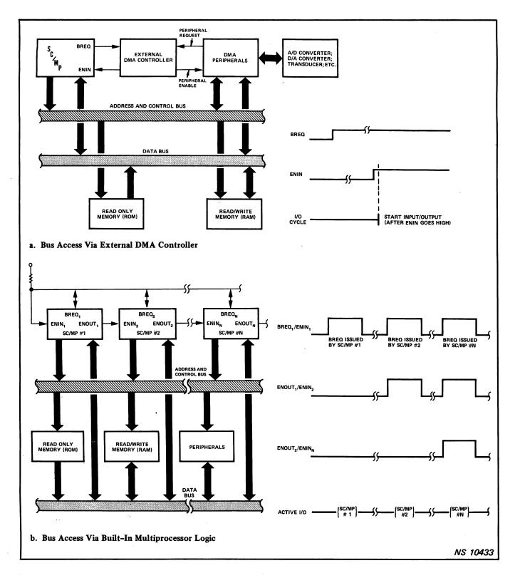
Figure 2-4. Typical DMA Configurations
