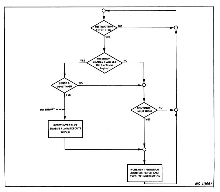
Figure 2-12. SC/MP Interrupt/Instruction-Fetch Process
