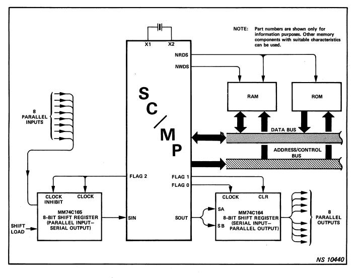
Figure 2-11. Using SC/MP With a Simple Serial Interface
