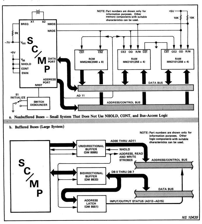
Figure 2-10. Nonbuffered and Buffered Bus Interfaces
