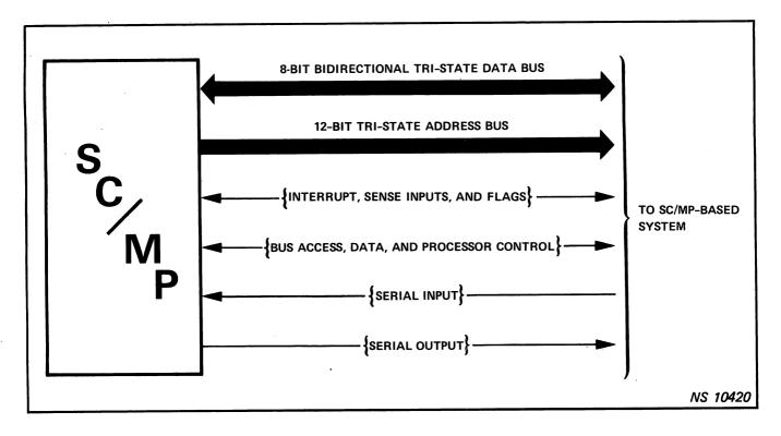
Figure 1-3. Input/Output Capabilities of SC/MP
