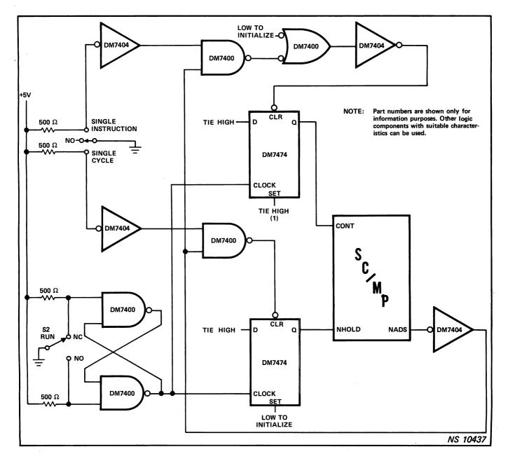
Figure 2-8. Circuit Detail To Implement Single-Cycle/Single-Instruction Control
