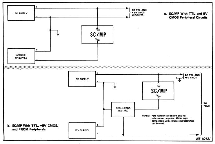
Figure 2-2. SC/MP Power Requirements, Typical Configurations
