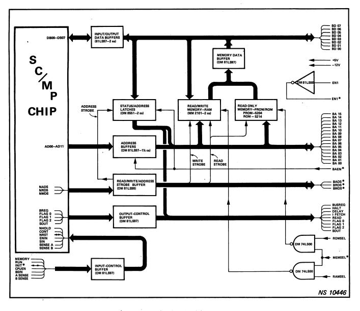
Figure 3-2. SC/MP CPU Application Module, Functional Block Diagram
