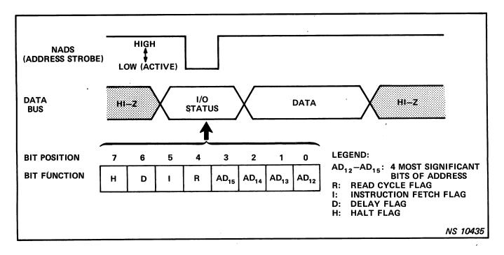
Figure 2-6. Data Bus at Address Strobe Time
