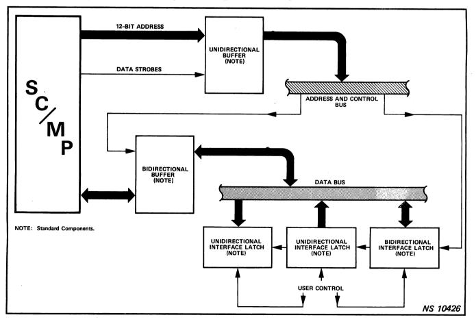
Figure 1-9. SC/MP Using Interface Latch For Input/Output Device
