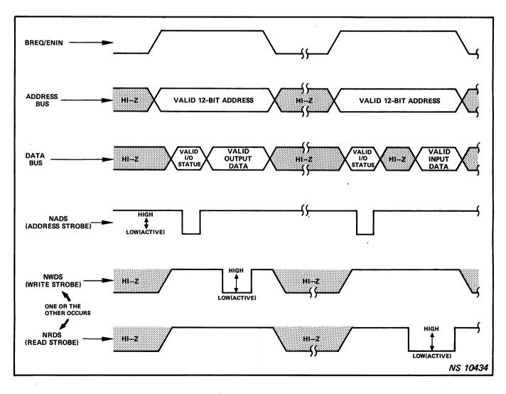
Figure 2-5. Typical Input/Output Sequence Showing Relative Timing
