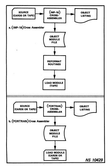
Figure 1-12. SC/MP Cross Assemblers—Operational Flow Diagrams
