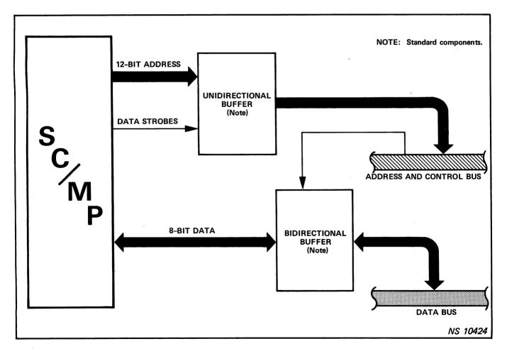
Figure 1-7. Fanout Buffering of SC/MP to System Buses
