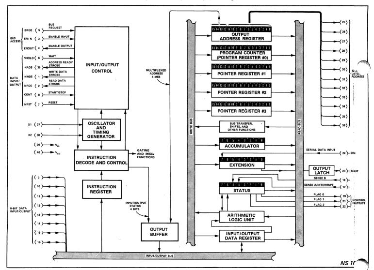
Figure 1-2. CPU Architecture and Pinouts of SC/MP
