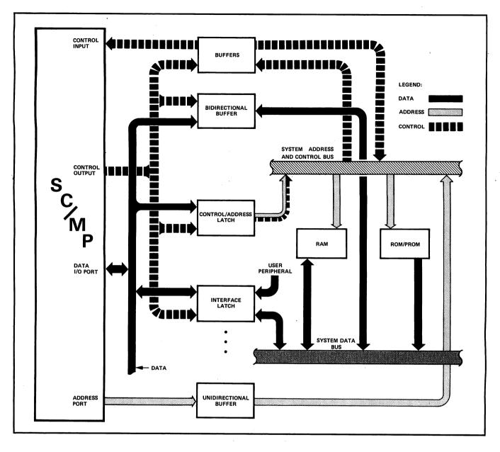
Figure 1–11. Typical Configuration of SC/MP with Supporting Chips
