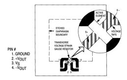
Figure 1. Basic Uncompensated Sensor Element — Top View
