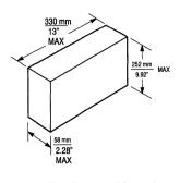
Figure 4. Fan Fold Box Dimensions
