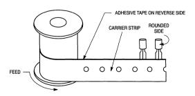
Rounded side of transistor and carrier strip visible (adhesive tape on reverse side).
