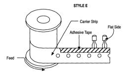
Flat side of transistor and adhesive tape visible.
