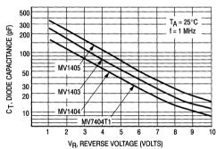
Figure 11. Diode Capacitance versus Reverse Voltage
