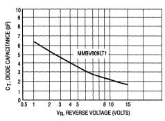
Figure 4. Diode Capacitance
