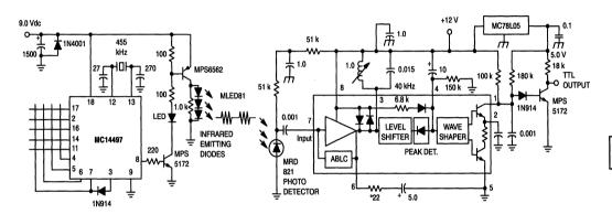
Figure 4. Remote Control Application 40 kHz Carrier
