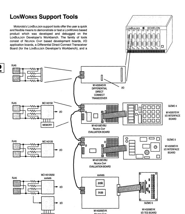
Figure 20. Evaluation and I/O Interface Boards
