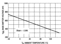
Figure 2. Base–Emitter Voltage versus Ambient Temperature
