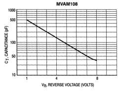
Figure 7. Capacitance versus Reverse Voltage
