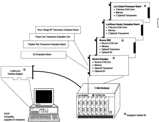
Figure 19. LonBuilder Developer's Workbench and Starter Kit
