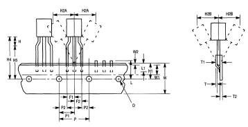
Figure 1. Device Positioning on Tape
