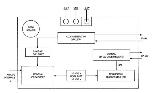
Figure 22. MC145537EVK Block Diagram
