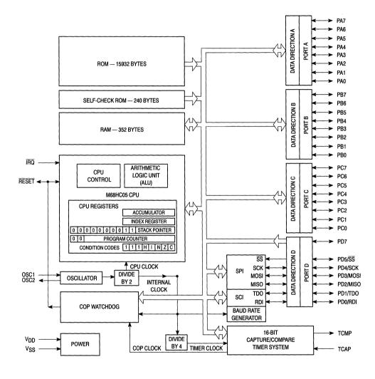
Figure 2. MC68HC05C9 Block Diagram
