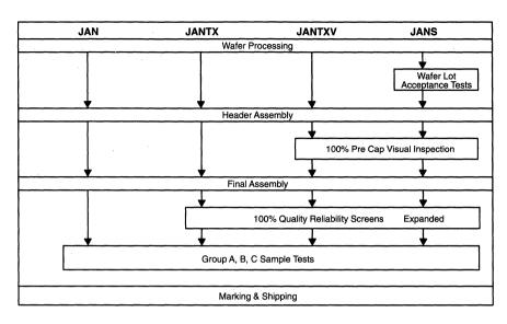
Figure 1. The MIL-S-19500 Semiconductor Process Flow
