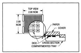
Figure 3. MIL-tested discrete semiconductor chips are now available off the shelf for high reliability hybrid (multi-chip) circuits.
