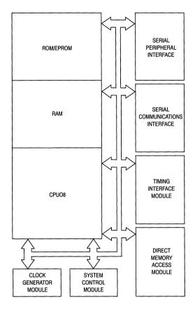
Figure 5. Block Diagram of Typical M68HC08 MCU
