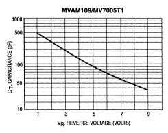
Figure 8. Capacitance versus Reverse Voltage
