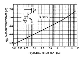
Figure 1. Base–Emitter Voltage versus Collector–Emitter Current
