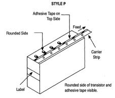
Style P ammo pack is equivalent to Styles A and B of reel pack dependent on feed orientation from box.
