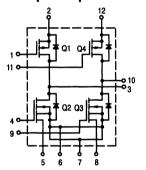
H-Bridge with Current Sensing MPM3002/MPM3010
