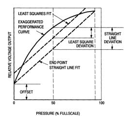
Figure 2. Linearity Specification Comparison
