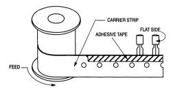
Flat side of transistor and adhesive tape visible.
