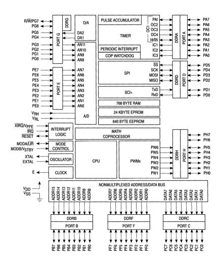
Figure 8. MC68HC711N4 Block Diagram
