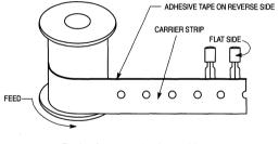
Flat side of transistor and carrier strip visible (adhesive tape on reverse side).
