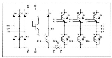
Includes optional sense resistor and temperature sensor.
