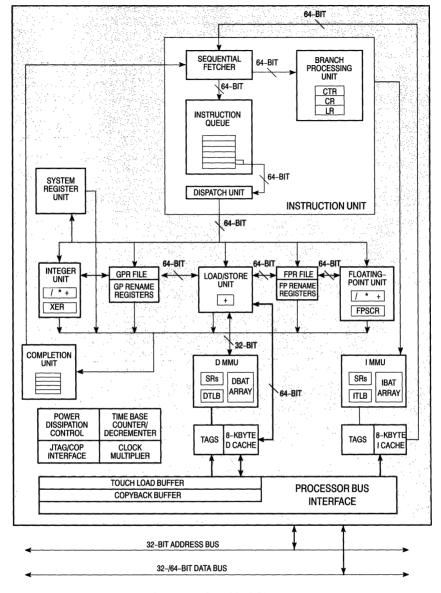
Figure 2. MPC603 Block Diagram
