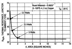
Figure 3. Thermal Resistance versus Drain Pad Area for the D<sup>2</sup>PAK Package (Typical)
