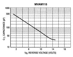
Figure 9. Capacitance versus Reverse Voltage
