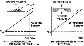
Motorola sensing elements can withstand pressure inputs as high as four times their rated capacity, although accuracy at pressures exceeding the rated pressure will be reduced. When excessive pressure is reduced, the previous linearity will immediately be restored.
