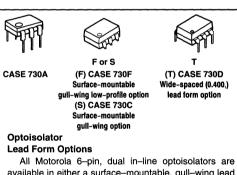
All Motorola 6-pin, dual in-line optoisolators are available in either a surface-mountable, gull-wing lead form or a wide-spaced 0.400" lead form, which is used to satisfy 8 mm PC board spacing requirements.
