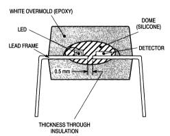
Figure 2. Geometric Design for Optoisolators
