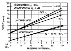
Figure 6. Typical-Output Voltage versus **Pressure and Temperature for Compensated** and Uncompensated Devices
