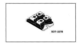
This new internally isolated high power package achieves low  $\mathsf{R}_{\mathsf{DS(on)}}$  by paralleling multiple die. Rated at 460 watts, the Isotop package exceeds the power dissipation ratings of all other power MOSFET packages. This package has a 2.5 kV isolation voltage.
