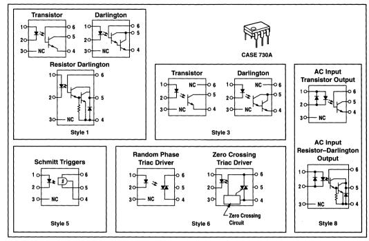
An optoisolator consists of a gallium arsenide infrared emitting diode, IRED, optically coupled to a monolithic silicon photodetector in a wide array of standard devices and encourages the use of special designs and selections for special applications. All Motorola optoisolators have VISO rating of 7500 Vac(pk), exceeding all other industry standard ratings.
