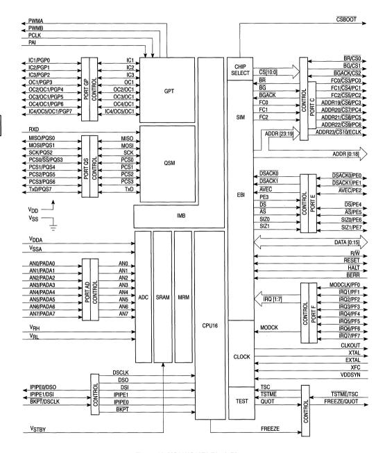
Figure 10. MC68HC16Z2 Block Diagram
