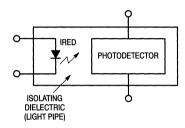
Figure 1. Block Diagram of Optoisolator
