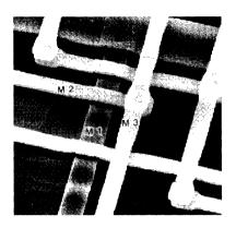
Figure 3. Triple—Layer Metal Signal Routing Enhances Utilization
