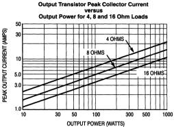
Another important parameter that must be considered before selecting the output transistors is the safe–operating area these devices must withstand. For a complete discussion on these see Application Notes AN484A and AN485.
