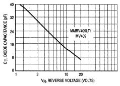
Figure 3. Diode Capacitance
