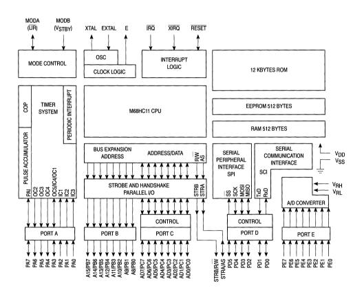
Figure 7. MC68HC11E9 Block Diagram
