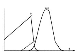
Figure A. Dynamic Desaturation
