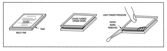
Figure 4. Care in removing the filter paper from the multi-pak will prevent loss of chips adhering to the paper.
