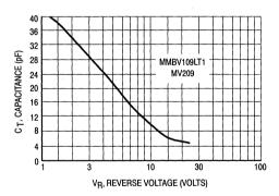
Figure 2. Diode Capacitance
