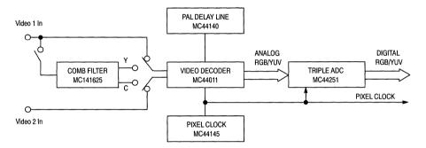
Figure 2. Video Input Processing
