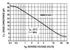
Figure 5. Diode Capacitance
