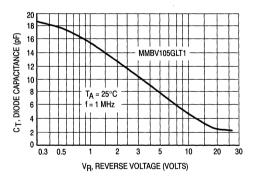
Figure 1. Diode Capacitance
