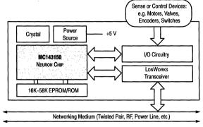
Figure 17. MC143150 in a Typical Node Block Diagram
