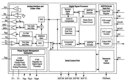
Figure 21. MC145540 ADPCM Codec Block Diagram
