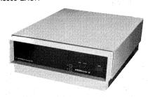
The EXORciser is an expandable development system that allows development of any 8-bit Motorola microprocessor or microcomputer configuration, from the simplest to the most elaborate. It comes with an MPU Module that provides system timing and a DEbug Module that contains system firmware. Both MC68B00 or MC68B09 MPU versions are offered in the EXORciser Development System.
