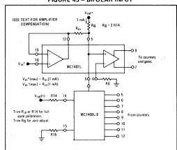
FIGURE 43 – BIPOLAR INPUT
