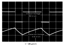
$(R_A = 5.1 \, k\Omega, C = 0.01 \, \mu F, R_L = 1.0 \, k\Omega;$  $R_B = 3.9 \, k\Omega, V_{CC} = 15 \, V)$
