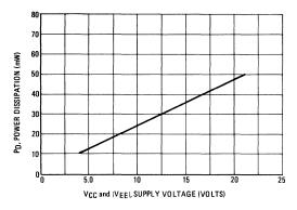
FIGURE 9 – POWER DISSIPATION versus POWER SUPPLY VOLTAGES
