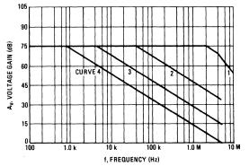
FIGURE 9 - MC1531/MC1431 OPEN LOOP VOLTAGE GAIN
