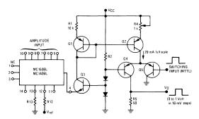
Fast rise and fall times require the use of high speed switching transistors for the differential pair, Q4 and Q5. Linear ramps and sine waves may be generated by the appropriate reference input.
