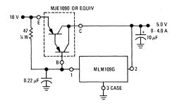
FIGURE 20 – 5.0-VOLT, 10-AMPERE REGULATOR (with Short-Circuit Current Limiting for Safe-Area Protection of pass transistors)
