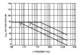
FIGURE 3 - VOLTAGE GAIN versus FREQUENCY
