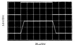
Clock Frequency increases from 5.0 MHz to 20 MHz with voltage controlled MC4024 in Panic Mode operation.
