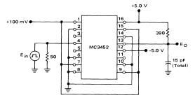
Output of Channel B shown under test, other channels are tested similarly.
