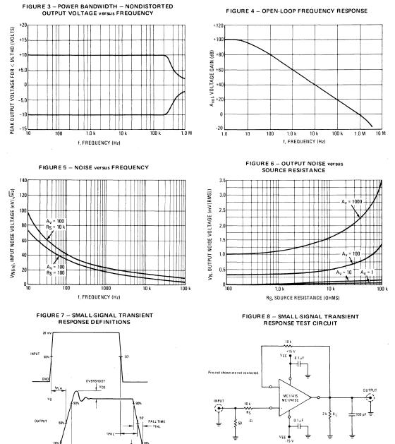
$\label{eq:VCC} \begin{array}{l} \textbf{TYPICAL CHARACTERISTICS} \\ (V_{CC} = +15 \ Vdc, \ V_{EE} = -15 \ Vdc, \ T_A = +25^o C \ unless \ otherwise \ noted.) \end{array}$
