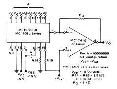
Decrease  $R_O$  to 2.5 k  $\Omega$  for a 0 to -5.0-volt output range. This application provides somewhat lower speed, as previously discussed in the Output Voltage Range section of the General Information.
