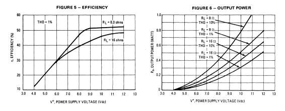
TYPICAL CHARACTERISTICS (V<sup>+</sup> = 9.0 V, f = 1.0 kHz,  $T_A$  = +25<sup>o</sup>C unless otherwise noted)
