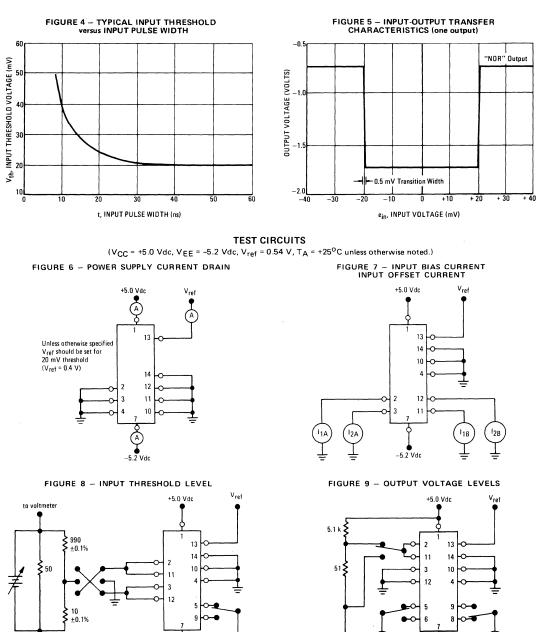
TYPICAL CHARACTERISTICS (continued) (V<sub>CC</sub> = +5.0 Vdc, V<sub>EE</sub> = -5.2 Vdc, V<sub>ref</sub> set for 20 mV Threshold, T<sub>A</sub> = +25<sup>o</sup>C unless otherwise noted.)
