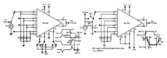
FIGURE 7 - INPUT COMMON-MODE CHARACTERISTICS
