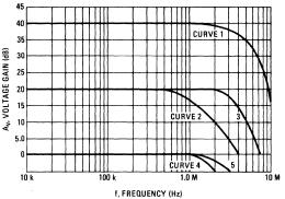
FIGURE 8 - MC1530/MC1430 OPEN LOOP VOLTAGE GAIN versus FREQUENCY
