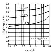
FIGURE 7 – LOW OUTPUT VOLTAGE @  $V_{CC} = 5.0 \, Vdc$
