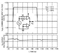
FIGURE 7 - COMMON-MODE PULSE RESPONSE
