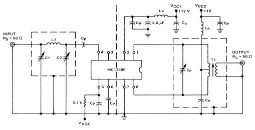
FIGURE 4 – UNTUNED INPUT (PIN 3 BYPASSED TO GROUND)
