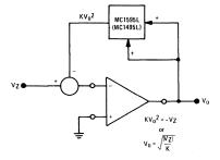
as indicated in Figure 26. This circuit may suffer from latch-up problems similar to those of the divide circuit. Note that only one polarity of input is allowed and diode clamping (see Figure 27) protects against accidental latch-up.
