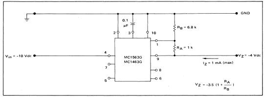
FIGURE 34 - An Adjustable "Zero-TC" Voltage Source
