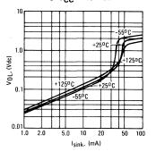
FIGURE 9 – LOW OUTPUT VOLTAGE @ V<sub>CC</sub> = 15 Vdc
