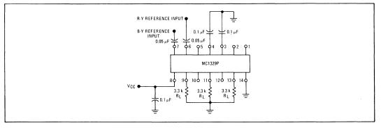
FIGURE 3 – DETECTED OUTPUT
