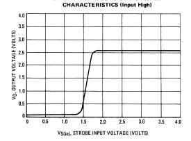
FIGURE 16 – CHANNEL SELECT versus OUTPUT TRANSFER CHARACTERISTICS
