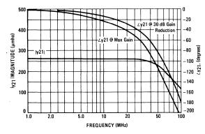
FIGURE 10 - MC1352 AGC CHARACTERISTICS
