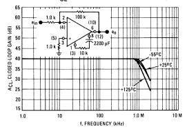
FIGURE 16 - ACL = 1000 RESPONSE versus TEMPERATURE
