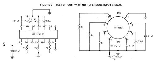
$\label{eq:test} \begin{array}{c} \textbf{TEST CIRCUITS} \\ (V^{+}=24 \; Vdc, \; R_{L}=3.3 \; k\Omega, \; T_{A}=+25^{o}C \; unless \; otherwise \; noted) \end{array}$
