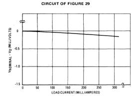
FIGURE 30 - LOAD REGULATION FOR
