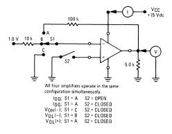
FIGURE 7 – INPUT BIAS CURRENT AND CURRENT MIRROR GAIN
