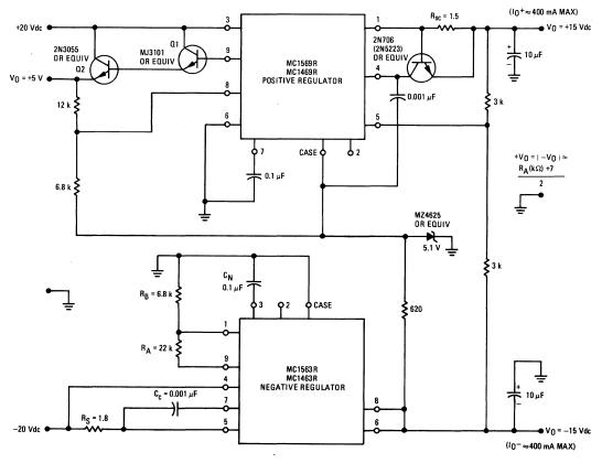
FIGURE 33 - A ±15 Vdc COMPLEMENTARY TRACKING REGULATOR WITH AUXILIARY +5.0 V SUPPLY
