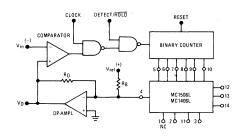
Positive peaks may be detected by inserting a hex inverter between the counter and MC1506L, reversing the comparator inputs, and connecting the output amplifier for unipolar operation.
