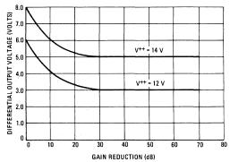
FIGURE 11 – MC1353 AGC CHARACTERISTICS
