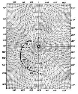
FIGURE 23 – s<sub>12</sub>, REVERSE TRANSMISSION COEFFICIENT (FEEDBACK)
