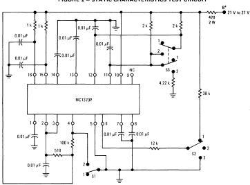
FIGURE 2 – STATIC CHARACTERISTICS TEST CIRCUIT
