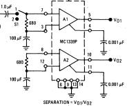
FIGURE 2 - POWER SUPPLY REJECTION
