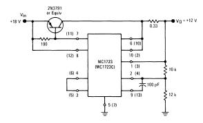
Pin numbers adjacent to terminals are for the metal and ceramic flat packages; pin numbers in parenthesis are for the ceramic dual in-line package.
