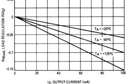
FIGURE 6 – LOAD REGULATION CHARACTERISTICS WITH CURRENT LIMITING
