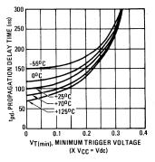
FIGURE 10 – DELAY TIME versus SUPPLY VOLTAGE
