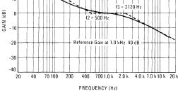
for RIAA equalization. Figure 12 illustrates the RIAA response of the amplifier in Figure 11. The dashed line shows the ideal response with the corner frequencies indicated. The lower corner frequency (f1) is determined by the input capacitance C1 and the equation
