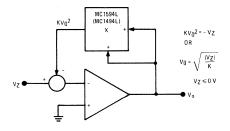
nator voltage. As a result, if  $V_X$  is set to 10 volts and 0.5% accuracy is available, then 5% accuracy can be expected when  $V_X$  is only 1 volt.
