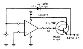
$\label{eq:VO} \begin{array}{l} V_0 = V_Z + 0.6 \ Vdc \\ NOTE 1: \ R is used to bias the zener. \\ NOTE 2: \ If the Zener TC is positive, and equal in magnitude to the negative TC of the input to the operational amplifier (\approx 2.0 mV/°C), the output is zero-TC. A 7.0-Volt Zener will give approximately zero-TC. \end{array}$
