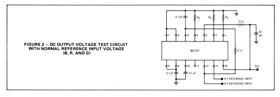
$\label{eq:test} \begin{array}{l} \textbf{TEST CIRCUITS} \\ (V_{CC} = 24 \; \text{Vdc}, \; \textbf{R}_L = 3.3 \; \text{kilohms}, \; \textbf{T}_A = +25^{o} \text{C} \; \text{unless otherwise noted}) \end{array}$
