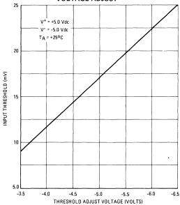
FIGURE 4 - TYPICAL INPUT THRESHOLD versus V<sup>-</sup>
