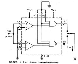
2. Not more than one output should be tested at one time.
