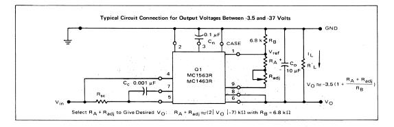
PARTS LIST Component Value Description Select 1/4 or 1/2 watt carbon 6.**8** k Select IRC Model X-201, Mallory Model MTC-1 or equivalent Select 1/2 watt carbon Select For minimum current of 1 mAdc 10 µF Sprague 1500 Series, Dickson D10C series or equivalent 0.1 µF Ceramic Disc - Centralab DDA 104, or equivalent Sprague TG-P10, or equivalent 0.001 µF Jumper MC1563R or MC1463R
