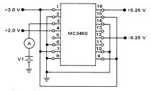
Output of Channel A shown under test, other outputs are tested similarly for V1 = 0.4 V and +2.4 V.
