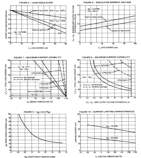
TYPICAL CHARACTERISTICS (V<sub>CC</sub> = +20 V, V<sub>EE</sub> = -20 V, V<sub>O</sub> =  $\pm$ 15 V, T<sub>A</sub> = +25<sup>o</sup>C unless otherwise noted.)
