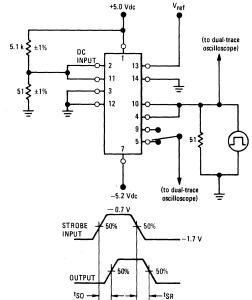
FIGURE 13 – DIFFERENTIAL MODE RECOVERY TIME (See definition section)
