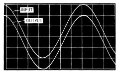
FIGURE 38 – BASIC 8-BIT TRACKING A-TO-D CONVERTER SINE WAVE RESPONSE
