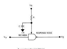
C, capacitor is for noise filtering. R, resistor is for threshold shifting.
