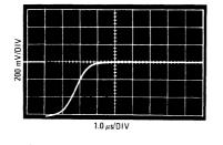
FIGURE 12 - WAVEFORM AT FALSE SUMMING NODE
