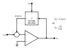
$V_{\boldsymbol{X}}$  being near zero is a result of the transfer through the multiplier being near zero. The op-ampl. is then operating with a very high closed loop gain and error voltages can thus become effective in causing latch-up.
