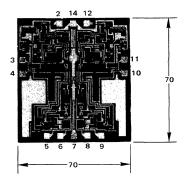
All dimensions are nominal and in mils  $(10^{-3} \text{ inches})$ . Die Dimensions Thickness = 8.0 Bonding Pads =  $4.0 \times 4.0$
