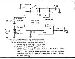
FIGURE 3 - GENERAL TEST CIRCUIT
