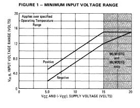
TYPICAL CHARACTERISTICS ( $V_{CC} = +15 V$ ,  $V_{EE} = -15 V$ ,  $T_{A} = +25^{\circ}C$  unless otherwise noted.)
