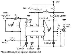
Connect to ground for maximum power gain test. All power-supply chokes  $(L_p)$ , are self-resonate at input frequency.  $L_p \ge 20 k\Omega$ See Figure 10 for frequency response curve.
