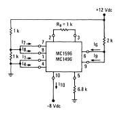
Pin number references pertain to this device when packaged in a metal can. To ascertain the corresponding pin numbers for a ceramic packaged device refer to the PIN CONNECTION CHART on the first page of this specification.
