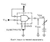
(Arrows indicate actual direction of current flow. Current into a terminal is a positive value.)
