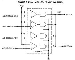
The MC3452 can be used for address decoding as illustrated above. All outputs of the MC3452 are tied together through a common resistor to  $\pm50$ , volts. In this configuration the MC3452 provides the "AND" function. All addresses have to be true before the output will go high. This scheme eliminates the need for an "AND" gate and enhances speed throughput for address decoding.
