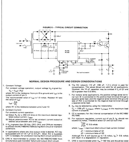
11. CR6 is recommended when  $V_{0}\!>\!150$  Vdc and should be rated such that Peak Inverse Voltage  $\!>\!V_{0}.$
