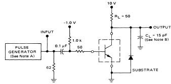
NOTES: A. The pulse generator has the following characteristics:  $t_W = 0.3 \ \mu s$ , duty cycle  $\leq 1\%$ ,  $z_0 \approx 50 \ \Omega$ . B. CL includes probe and jig capacitance.
