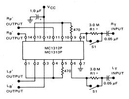
\*R1 is used for input impedance measurement. S1 is normally closed.
