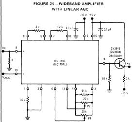
Notice that the resistor values for R<sub>X</sub>, R<sub>Y</sub>, and R<sub>L</sub> have been modified. This has been done primarily to increase the bandwidth by lowering the output impedance of the MC1594 and then lowering R<sub>X</sub> and R<sub>Y</sub> to achieve a gain of 1. The e<sub>c</sub> can be as large as 1 volt peak and e<sub>m</sub> as high as 2 volts peak. No output offset adjust is employed since we-are interested only in the ac output components.
