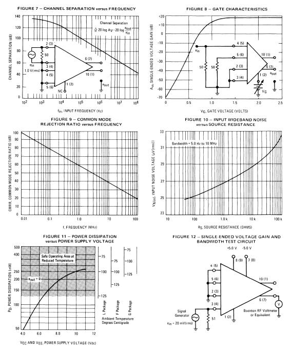
Number in parenthesis denotes pin for F and L packages, number at left in each case denotes corresponding pin for G package.
