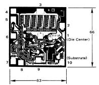
All dimensions are nominal and in mils  $(10^{-3} \text{ inches})$ . Die Dimensions Thickness = 8.0 Bonding Pads =  $4.0 \times 4.0$
