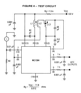
The number without parenthesis is the pin number for the metal package. The number in parenthesis is the pin number for the plastic package. Metal Package, Pin 9 - no connection
