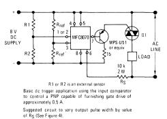
R2 must be the external sensor for the internal short and open protection to be operative.
