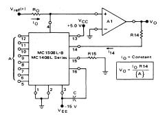
This circuit yields the inverse of a digital word scaled by a constant. For minimum error over the range of operation, I<sub>0</sub> can be set at 16  $\mu$ A so that I<sub>14</sub> will have a maximum value of 3.984 mA for a digital bit input configuration of 00000001.
