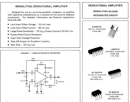
Pin numbers adjacent to terminals apply to 8-pin packages, numbers in parenthesis apply to 14-pin packages.
