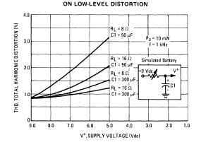
FIGURE 8 - EFFECT OF BATTERY AGING
