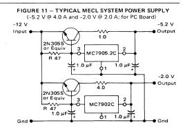
When current-boost power transistors are used, 47-ohm base-toemitter resistors (R) must be used to bypass the quiescent current at no load. These resistors, in conjunction with the VBE of the NPN transistors, determine when the pass transistors begin conducting. The 1-ohm and 4-ohm dropping resistors were chosen to reduce the power dissipated in the boost transistors but still leave at least 2.0 V across these devices for good regulation.
