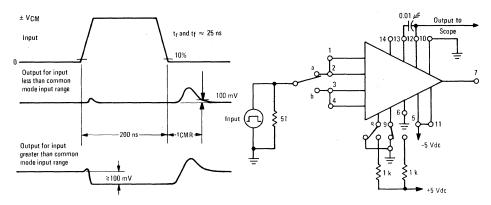
FIGURE 14 – DIFFERENTIAL RECOVERY AND DIFFERENTIAL RANGE
