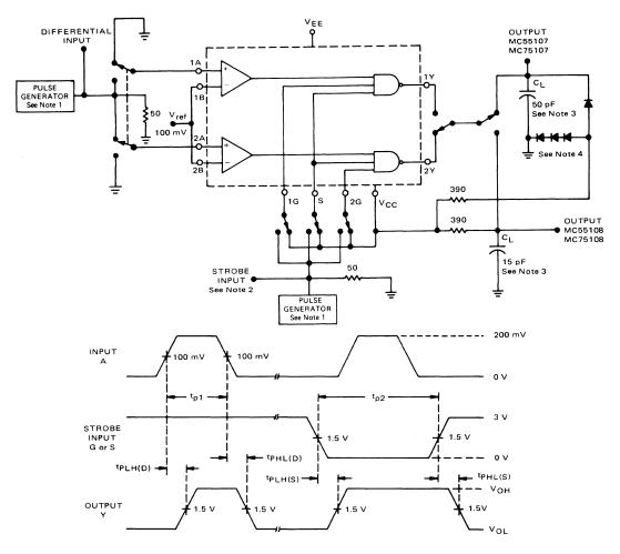
TEST CIRCUITS (continued) FIGURE 7 – PROPAGATION DELAY TIME TEST CIRCUIT AND WAVEFORMS
