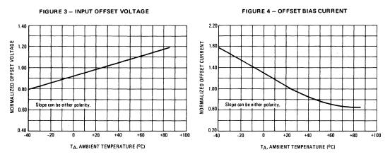
$$\label{eq:transformation} \begin{split} & \textbf{TYPICAL CHARACTERISTICS} \\ (V_{CC} = +15 \mbox{ Vdc}, \mbox{T}_{A} = +25^{o} \mbox{C} \mbox{ (each comparator) unless otherwise noted.}) \end{split}$$
