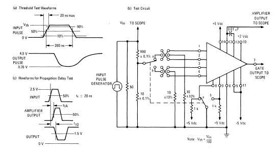
Number at terminal end denotes the pin number for flat package only; to ascertain the corresponding pin number for the dual in line packages refer to the circuit schematic on the second page.
