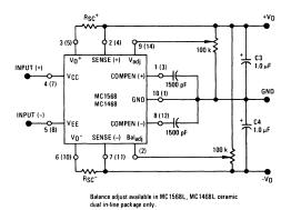
FIGURE 4 -- OUTPUT VOLTAGE ADJUSTMENT FOR 8.0 V  $\leq |\pm V_0| \leq 14.5$  V (Ceramic-Packaged Devices Only, L Suffix.)
