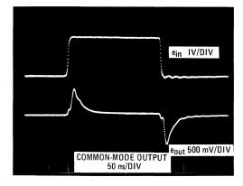
FIGURE 12 - DIFFERENTIAL-MODE RECOVERY TIME
