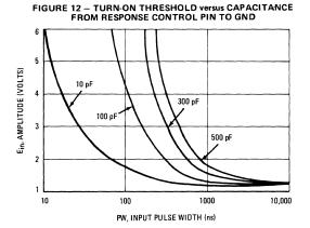
rejection. The MC1489L input has typical turn-on voltage of 1.25 volts and turn-off of 1.0 volt for a typical hysteresis of 250 mV. The MC1489AL has typical turn-on of 1.95 volts and turn-off of 0.8 volt for typically 1.15 volts of hysteresis. Each receiver section has an external response control node in
