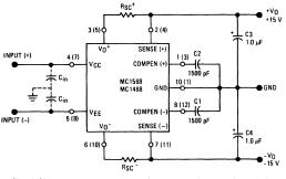
C1 and C2 should be located as close to the device as possible. A 0.1  $\mu F$  ceramic capacitor (Cin) may be required on the input lines if the device is located an appreciable distance from the rectifier filter capacitors.
