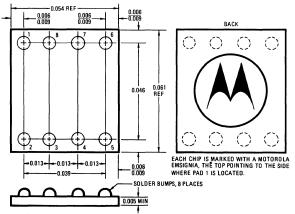
Bump Dia, at Base: 0.006 ± 0.001 in. Bump Height: 0.0040 ± 0.0005 in. Each bump centerline to be located within 0.001 in. of its true position with respect to any other bump centerline.
