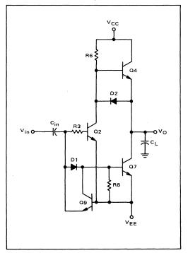
The complete circuit, Figure 1, basically creates Darlington devices of transistors Q7, Q4 and Q2 in the simplified circuit of Figure 17. Note in Figure 1 that when the input goes negative with respect to VEE, diodes D7 through D10 turn "on" assuring faster turn "off" of transistors Q1, Q2, Q6 and Q7. Resistor R6 insures that the output will charge to within one V<sub>BE</sub> voltage drop of the V<sub>CC</sub> supply.
