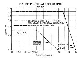
exceed the maximum junction temperature rating during this fault condition and, in addition, the dc safe operating area limit (see Figure 41).
