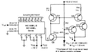
Current pulses, ramps, staircases, and sine waves may be generated by the appropriate digital and reference inputs. This circuit is especially useful in curve tracer applications.
