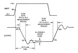
FIGURE 11 – SLEW RATE AND SETTLING TIME TEST CIRCUIT
