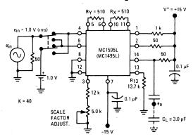
FIGURE 9 – BANDWIDTH (R  $_L$  = 11 k  $\Omega$ )
