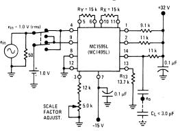
FIGURE 11 – COMMON-MODE GAIN and COMMON-MODE INPUT SWING
