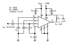
FIGURE 2 - VOLTAGE GAIN AND BANDWIDTH TEST CIRCUIT
