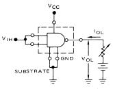
Both inputs are tested simultaneously.
