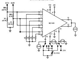
FIGURE 4 – CHANNEL SELECT AND STROBE INPUT CURRENTS
