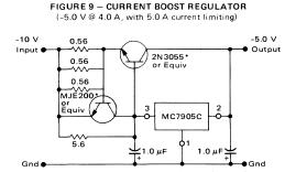
\*Mounted on common heat sink, Motorola MS-10 or equivalent.
