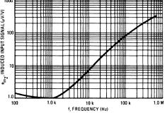
Induced input signal ( $\mu V$  of induced input signal in amplifier #2 per volt of output signal at amplifier #1)
