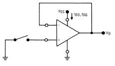
IDO is total supply current with "+" input open. IDG is total supply current with "+" input grounded.
