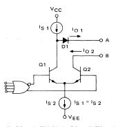
If Q1 is "on", Q2 is "off", Diode D1 is "off" and current IS 1 flows through Q1 and IS 2 to VEE. However, if Q1 is "off", and Q2 is "on", the current IS 1 flows through diode D1 to output A and current from output B flows through Q2 to current sink IS 2.
