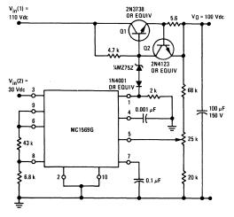
Figure 34 shows how the regulator can be controlled by a logic gate. Here, it is assumed that the regulator operates in its normal mode – as a positive regulator referenced to ground – and that the logic gate is of the saturating type, operating from a positive supply to ground. The high logic level should be greater than about 1.5 V and should source no more than 10 mA into pin 2.
