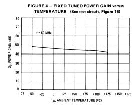
$\label{eq:VCC} \begin{array}{l} \textbf{TYPICAL CHARACTERISTICS} \\ (V_{CC} = 12 \mbox{ Vdc}, \mbox{ T}_{A} = +25^{o} \mbox{C} \mbox{ unless otherwise noted}) \end{array}$
