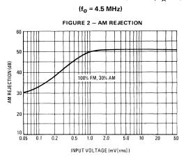
TYPICAL CHARACTERISTICS  $(V^+ = 24 V, T_A = +25^{\circ}C \text{ unless otherwise noted})$
