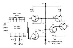
Current pulses, ramps, staircases, and sine waves may be generated by the appropriate digital and reference inputs. This circuit is especially useful in curve tracer applications.
