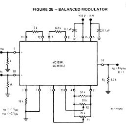
The adjustment procedure for this circuit is quite simple. (1) Place the carrier signal at pin 10. With no signal applied to pin 9, adjust potentiometer P1 such that an ac null is obtained at the output.
