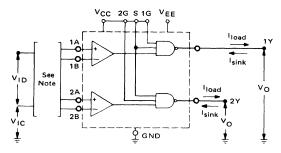
NOTE: When testing one channel, the inputs of the other channel are grounded.
