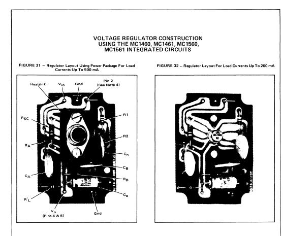
There is a general tendency to consider a voltage regulator as simply a dc circuit and to prepare circuit layout accordingly. The excellent high-frequency performance and fast response capability of this integrated-circuit regulator, however, makes extra layout care worthwhile. Since short, well-dressed leads must be used, printed-circuit boards provide an excellent component interconnection technique.
