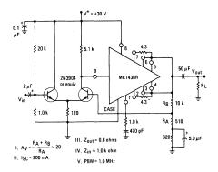
FIGURE 15 - NON-INVERTING POWER AMPLIFIER
