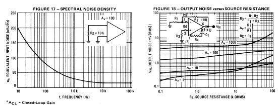
Pin numbers adjacent to terminals apply to 8-pin packages, numbers in parenthesis apply to 14-pin packages.
