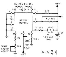
FIGURE 10 – BANDWIDTH (RL = 50  $\Omega$ )
