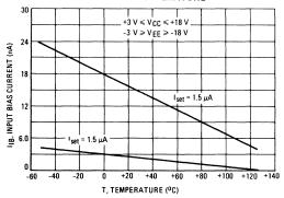
FIGURE 4 - INPUT BIAS CURRENT versus SET CURRENT
