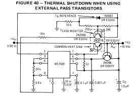
In the case where an external pass transistor is employed, its temperature, rather than that of the IC regulator, requires control. A technique similar to the one just discussed can be used by directly monitoring the case temperature of the pass transistor as is indicated in Figure 40. The case of the normally "OFF" thermal monitoring transistor, Q2, should be in thermal contact with, but electrically isolated from, the case of the boost transistor, Q1.
