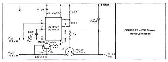
$(R_A = 13 \text{ k}\Omega)$  supply and operating with a – 15 V input, with a  $R_{sc}$  of 0.1  $\Omega$ , will yield a change in output voltage of only 26 mV over a load current range of from 1 mA to 3.5 A. This corresponds to a dc output impedance of only 7.5 milliohms or a percentage load regulation of 0.26% for a full 3.5-ampere load current change. Figure 27 indicates how the short circuit current varies with the value of  $R_{sc}$  for this circuit.
