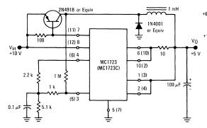
FIGURE 18 - +5 V, 1-AMPERE SWITCHING REGULATOR
