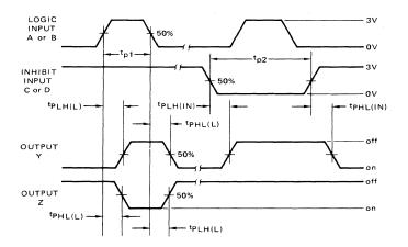
NOTES: 1. The pulse generators have the following characteristics:  $z_0 = 50 \ \Omega$ ,  $t_r = t_f = 10 \pm 5 \ ns$ ,  $t_{p1} = 500 \ ns$ , PRR = 1 MHz,  $t_{p2} = 1 ms, PRR = 500 kHz.$ 2. C<sub>L</sub> includes probe and jig capacitance.
