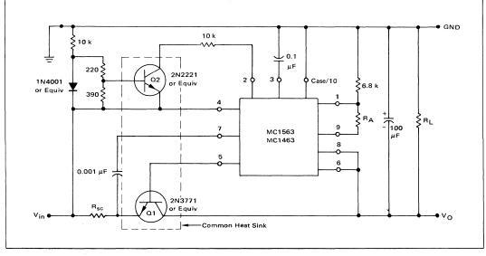
FIGURE 36 - Thermal Shutdown When Using External Pass Transistors
