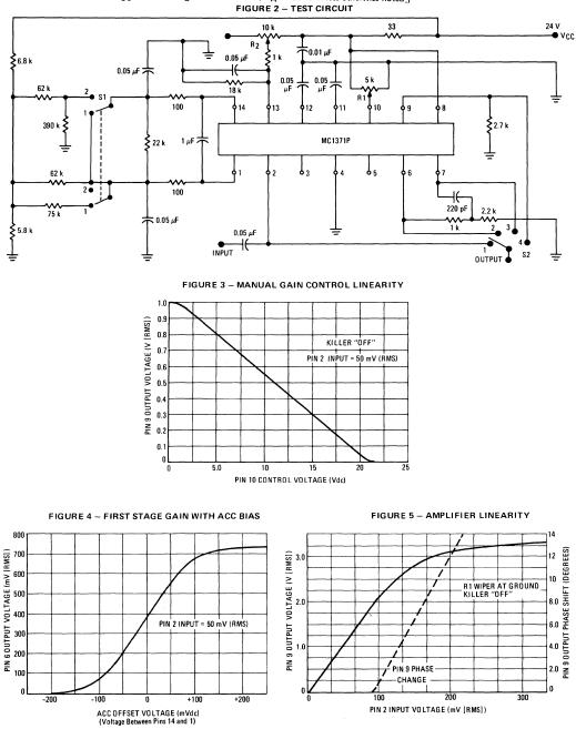
TYPICAL CHARACTERISTICS ( $V_{CC}$  = +24 Vdc, f<sub>O</sub> = 3.579545 MHz, T<sub>A</sub> = +25<sup>o</sup>C unless otherwise noted.)
