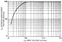
FIGURE 4 – DETECTOR "S" CURVE @ f = 4.5 MHz, BW = 200 kHz, Q = 24
