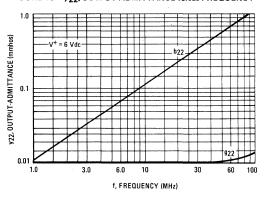
FIGURE 18 - y22, OUTPUT-ADMITTANCE versus FREQUENCY
