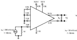
FIGURE 13 - OUTPUT VOLTAGE SWING TEST CIRCUIT
