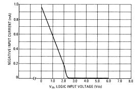
FIGURE 13 – LOGIC INPUT CURRENT versus INPUT VOLTAGE
