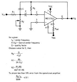
where  $f_0$  and GBW are expressed in Hz. GBW is available from Figure 6 as a function of Set Current,  $I_{\text{set}}.$
