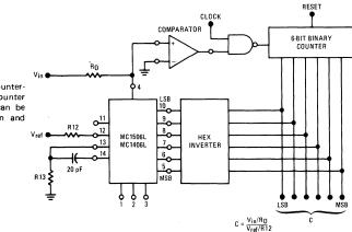
The circuit shown is a simple counterramp converter. An UP/DOWN counter and dual threshold comparator can be used to provide faster operation and continuous conversion.
