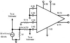
FIGURE 15 - OUTPUT IMPEDANCE TEST CIRCUIT
