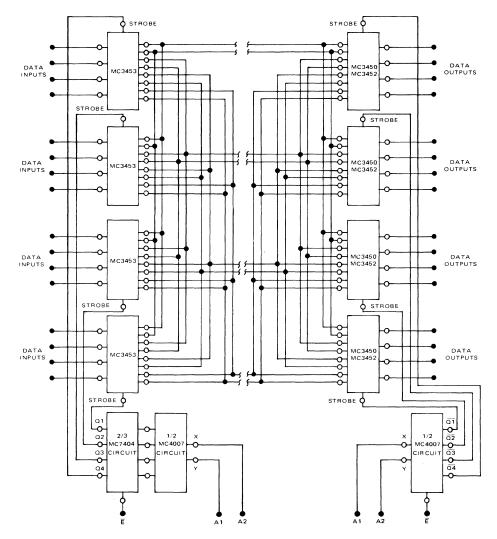
FIGURE 17 - PARTY-LINE DATA TRANSMISSION SYSTEM WITH MULTIPLEX DECODING
