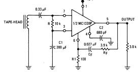
The lower -3.0 dB corner frequency (f1) is determined by the value for capacitor C1 in accordance with equation 1.
