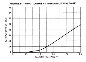
$\label{eq:transformation} \begin{array}{c} \textbf{TYPICAL CHARACTERISTICS} \\ (\textbf{V}_{CC} = + \ 20 \ \textbf{V}, \ \textbf{V}_{EE} = 0 \ \textbf{V}, \ \textbf{T}_{A} = + 25^{o} C \ \textbf{unless otherwise noted.}) \end{array}$
