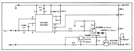
FIGURE 32 - Voltage Boosting Circuit
