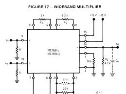
shows a typical ac multiplier circuit with a scale factor  $K\!\approx\!1.$  Again, resistor  $R_X$  and  $R_Y$  are chosen as outlined in the previous section, with  $R_L$  chosen to provide the required scale factor.
