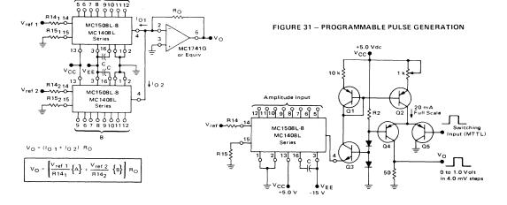
Fast rise and fall times require the use of high-speed switching transistors for the differential pair, Q4 and Q5. Linear ramps and sine waves may be generated by the appropriate reference input.
