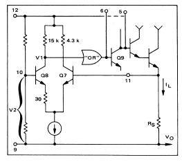
This level is further boosted by the output stage such that in the constant voltage mode overall transconductance is about 300 mA/volt.
