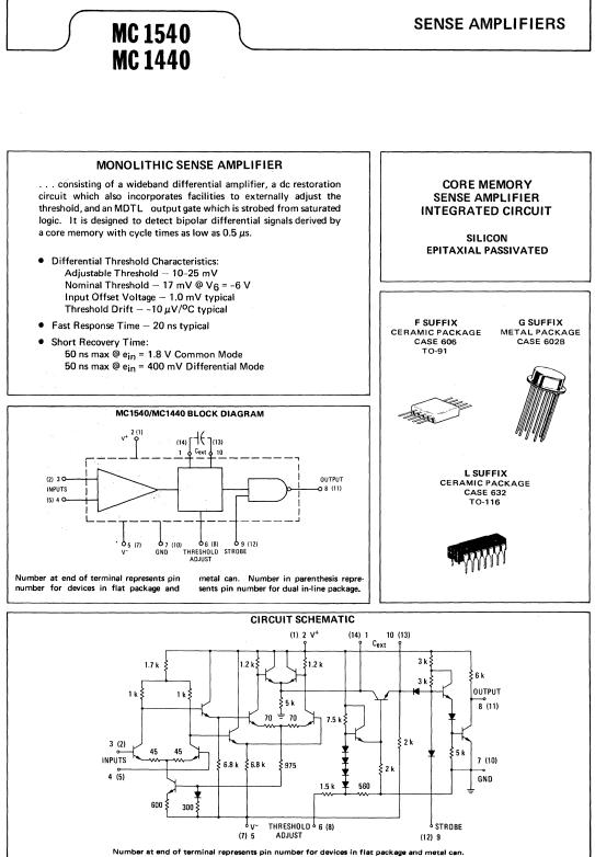
Number in parenthesis represents pin number for ceramic dual in-line package.
