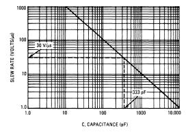
fast for this requirement. The current limited output of the device can be used to control this slew rate by connecting a capacitor to each driven output. The required capacitor can be easily determined by using the relationship C =  $I_{SC} \times \Delta T / \Delta V$  from which Figure 12 is derived. Accordingly, a 330-pF capacitor on each output will guarantee a worst case slew rate of 30 volts per microsecond.
