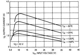
FIGURE 6 - PEAK OUTPUT CURRENT (K PACKAGE)
