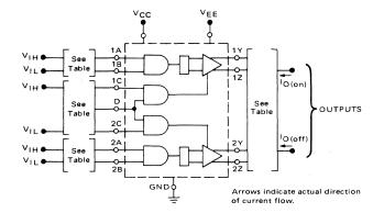
TEST TABLE TEST Ground all output pins not under test. INHIBITOR INPUTS LOGIC INPUTS 1B or 2B 1A or 2A 1C or 2C D VIL VIL at output VIH VIH VIL  $v_{1H}$ lO(on) 1 Y or 2 Y VIH VIL at output  $v_{1H}$ <sup>1</sup>O(on)  $v_{1H}$  $v_{\mathsf{IH}}$ v<sub>IH</sub> 1Z or 2Z at output <sup>I</sup>O(off) ⊻ін ViH VIH VIH 1Y or 2Y VIL V<sub>IL</sub> at output VIH lO(off) VIL  $v_{1H}$ ۷ін 1Z or 2Z VIH VIL VIL VIL at output Either Either O(off) VIL VIH 1Y, 2Y, 1Z, or 2Z state state VIL VIH
