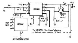
FIGURE 34 - ELECTRONIC SHUT-DOWN USING A MDTL GATE
