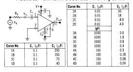
FIGURE 5c - CAPACITIVE COUPLED INPUT (R<sub>s</sub> < 500  $\Omega$ )
