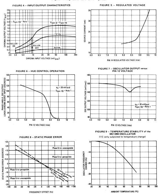
**TYPICAL CHARACTERISTICS** ( $T_A = +25^{\circ}C$  unless otherwise noted) (Figures 4 through 9, See Test Circuit of Figure 2.)
