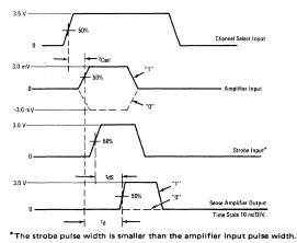
FIGURE 21 - TYPICAL TIMING SEQUENCE
