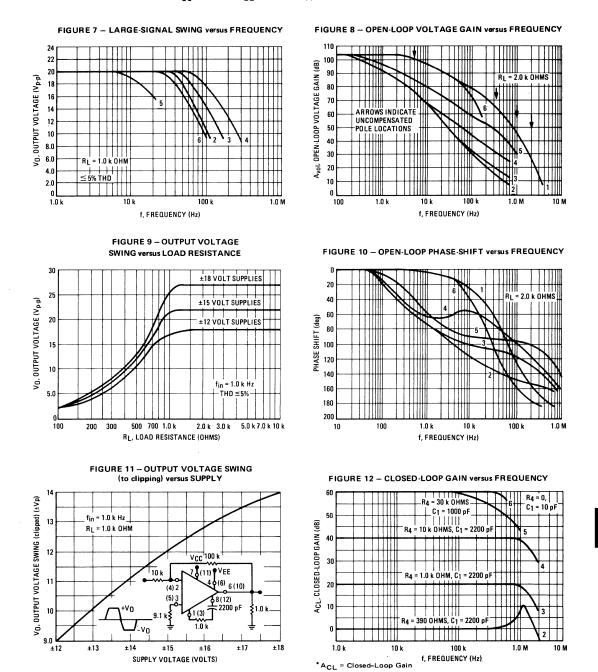
$$\label{eq:transformation} \begin{split} \textbf{TYPICAL CHARACTERISTICS} \ (continued) \\ (V_{CC} = +15 \ Vdc, \ V_{EE} = -15 \ Vdc, \ T_{A} = +25^{o}C, \ unless \ otherwise \ noted.) \end{split}$$
