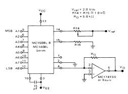
FIGURE 17 – OUTPUT CURRENT TO VOLTAGE CONVERSION
