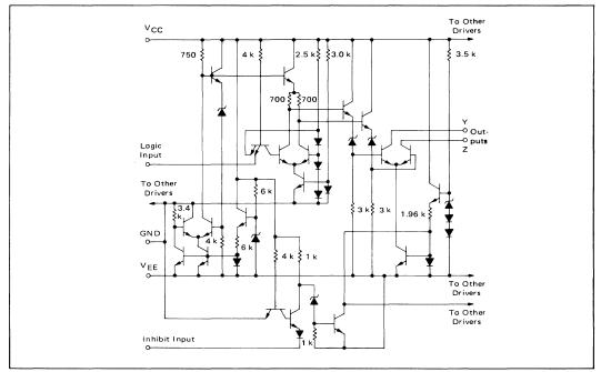
FIGURE 6 – CIRCUIT SCHEMATIC (1/4 Circuit Shown)
