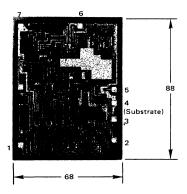
All dimensions are nominal and in mils  $(10^{-3} \text{ inches})$ . Die Dimensions Thickness = 8.0 Bonding Pads =  $4.0 \times 4.0$
