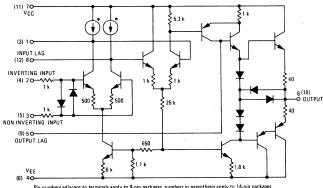
Pin numbers adjacent to terminals apply to 8 pin packages, numbers in parenthesis apply to 14 pin packages. Pin 7 is electrically connected to the substrate and VEE for Case 646 only. \*Patent pending.
