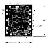
All dimensions are nominal and in mils  $(10^{-3} \text{ inches})$ . Die Dimensions Thickness = 8.0 Bonding Pads =  $4.0 \times 4.0$
