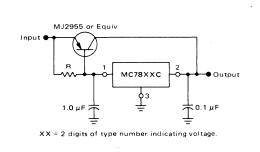
The MC7800C series can be current boosted with a PNP transistor. The MJ2955 provides current to 5.0 amperes. Resistor R in conjunction with the V<sub>BE</sub> of the PNP determines when the pass transistor begins conducting; this circuit is not short-circuit proof. Input-output differential voltage minimum is increased by V<sub>BE</sub> of the pass transistor.
