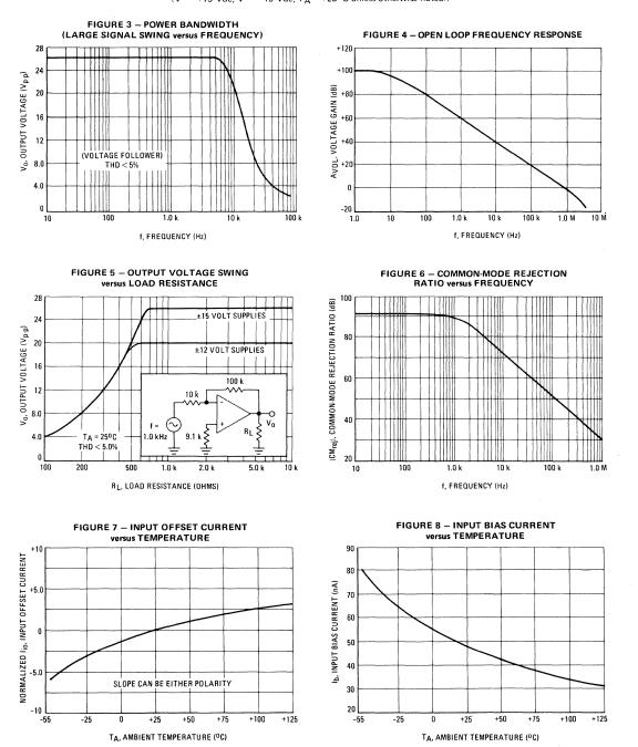
$\label{eq:transformation} \begin{array}{l} \textbf{TYPICAL CHARACTERISTICS} \ (continued) \\ (V^+ = +15 \ Vdc, \ V^- = -15 \ Vdc, \ T_A = +25^oC \ unless \ otherwise \ noted.) \end{array}$
