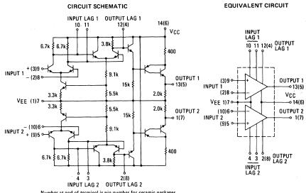
Number at end of terminal is pin number for ceramic packages. Number in parenthesis is pin number for metal package. Input Lag available only in ceramic packages.
