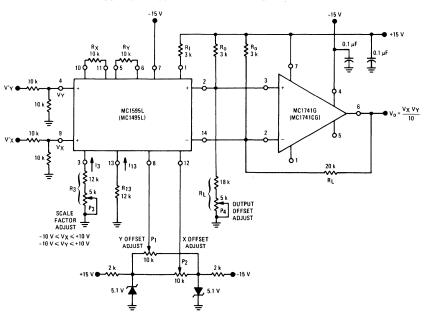
FIGURE 21 - MULTIPLIER WITH OP-AMPL. LEVEL SHIFT
