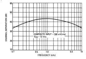
FIGURE 7 – CHANNEL SEPARATION
