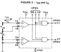
NOTE: Each pair of differential inputs is tested separately. The inputs of the other pair are grounded
