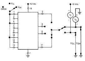
FIGURE 3 - OUTPUT SHORT CIRCUIT CURRENT
