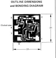
All dimensions are nominal and in mils ( $10^{-3}$  inches). Die Dimensions Thickness = 8.0 Bonding Pads = 4.0 x 4.0
