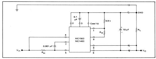
FIGURE 33 - Remote Sensing Circuit
