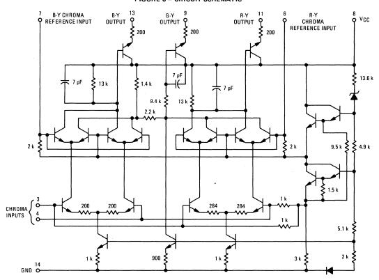
FIGURE 6 - CIRCUIT SCHEMATIC
