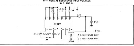
TEST CIRCUITS (V<sub>CC</sub> = 24 Vdc, R<sub>L</sub> = 3.3 Kilohms, T<sub>A</sub> = +25<sup>o</sup>C unless otherwise noted.)
