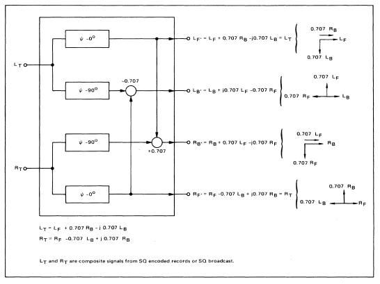
FIGURE 4 - DECODING PROCESS DIAGRAM
