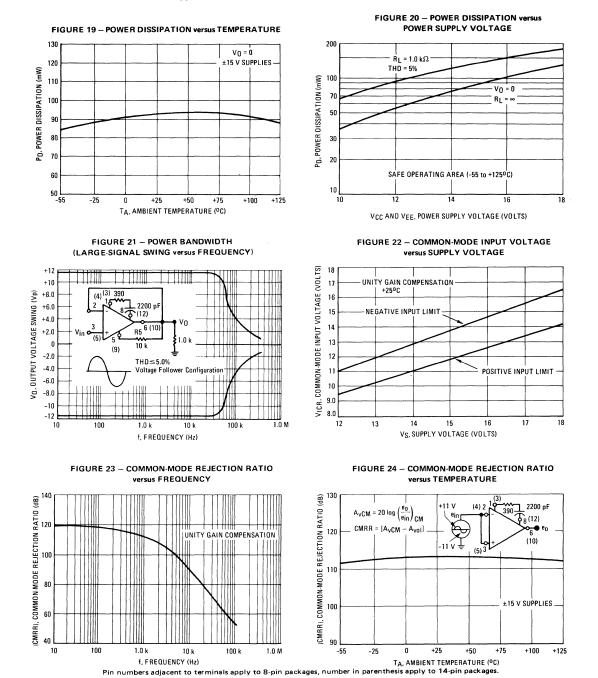
TYPICAL CHARACTERISTICS (continued) ( $V_{CC}$  = +15 Vdc,  $V_{EE}$  = ~15 Vdc,  $T_A$  = +25<sup>o</sup>C, unless otherwise noted.)
