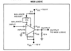
FIGURE 6 - ZERO-CROSSING DETECTOR DRIVING
