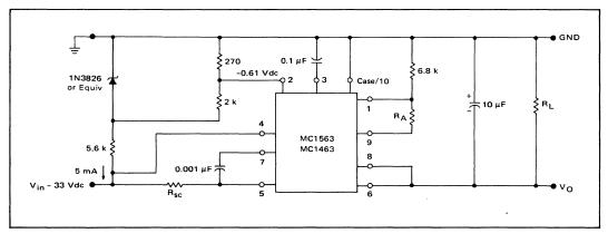
FIGURE 35 - Junction Temperature Limiting Shutdown Circuit
