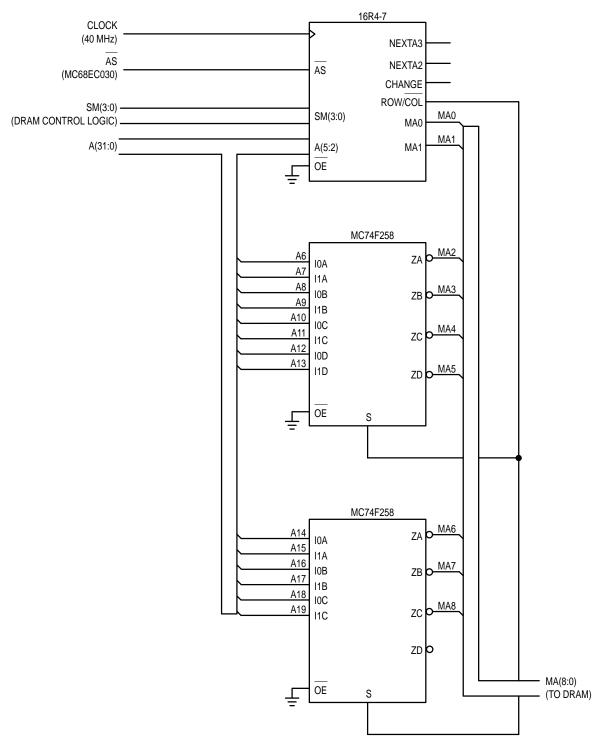
Figure 7. Address Multiplexing Logic
