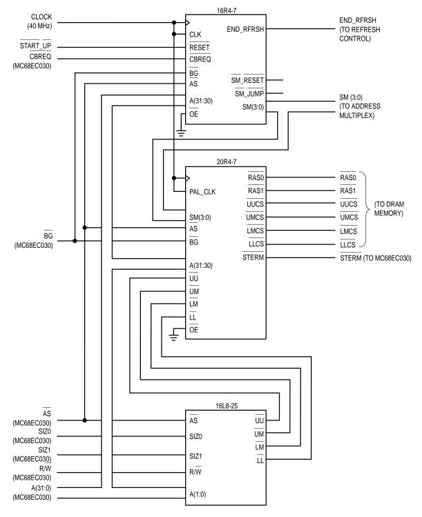
Figure 6. Memory Control Logic
