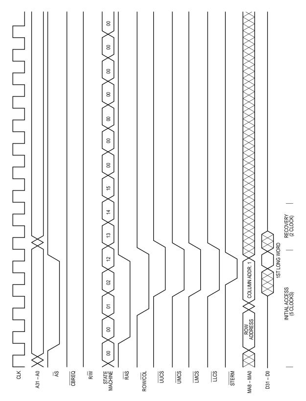
Figure 2. Non-Burst Read Access Followed by Idle Clocks
