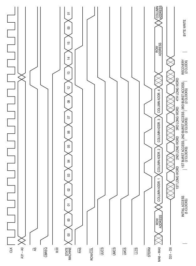
Figure 4. Burst Read Access Followed Immediately by a Byte Write Access
