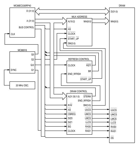
Figure 5. MC68EC030 System with DRAM Control
