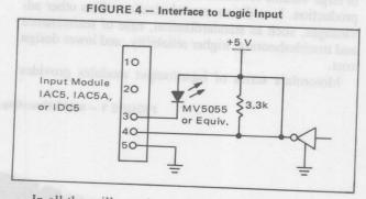
In all three illustrations, an indicator LED is added to indicate the status of the device. If a mounting board such as the MS16 is used, both the indicator LED and the  $3.3 \text{ k}\Omega$  resistor are installed on the board at the factory.
