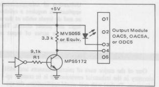
of an NPN transistor, which, in turn, drives the output module. By changing the value of R1 to 39 k $\Omega$ , this configuration may be used to interface CMOS operating at 15 volts with 15-volt logic modules OAC15, OAC15A, and ODC15.
